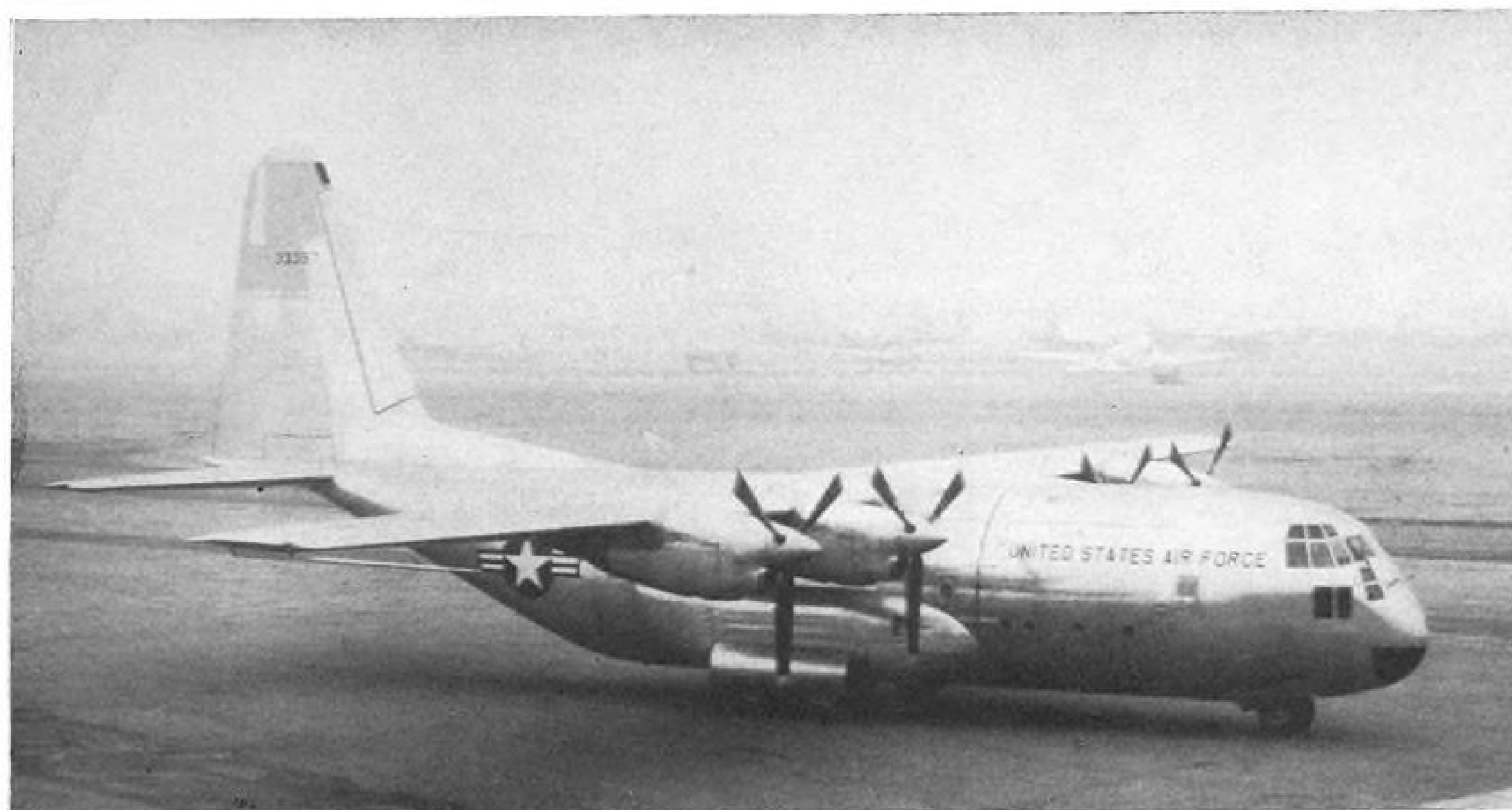
LOCKHEED YC-130 transport, forerunner of production C-130A, made its first flight Aug. 23. Powerplants are four Allison T56s.
