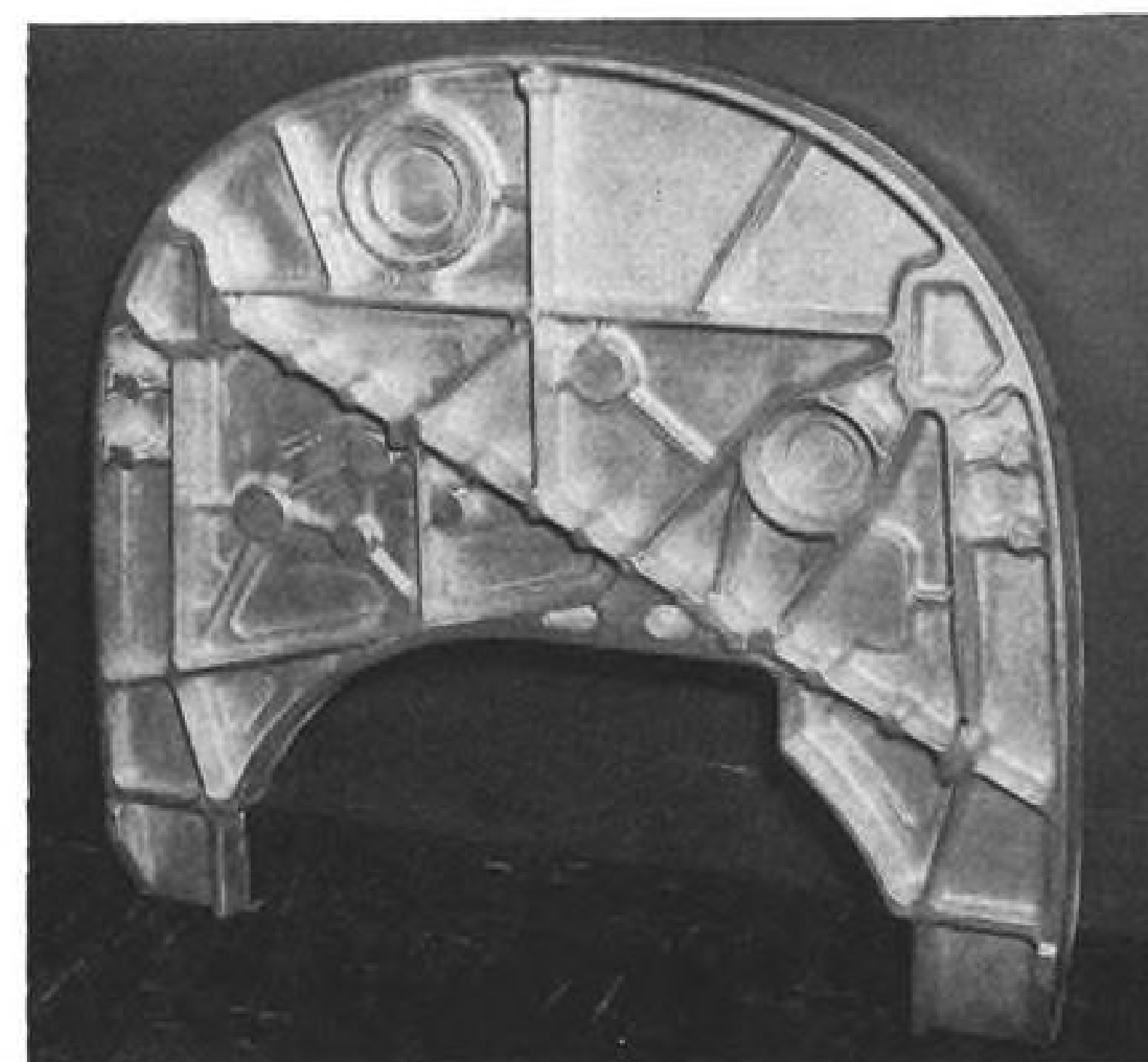
BIG FORGING—C-130A nacelle bulkhead has 775 sq. in. area.
