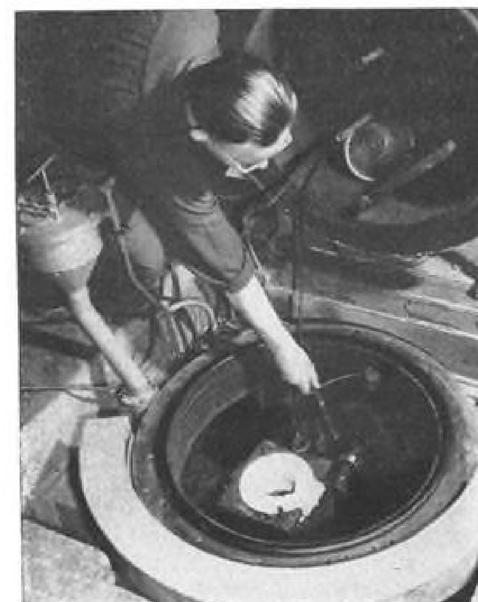
CRUCIBLE in GE experimental furnace holds metal for vacuum melting.
