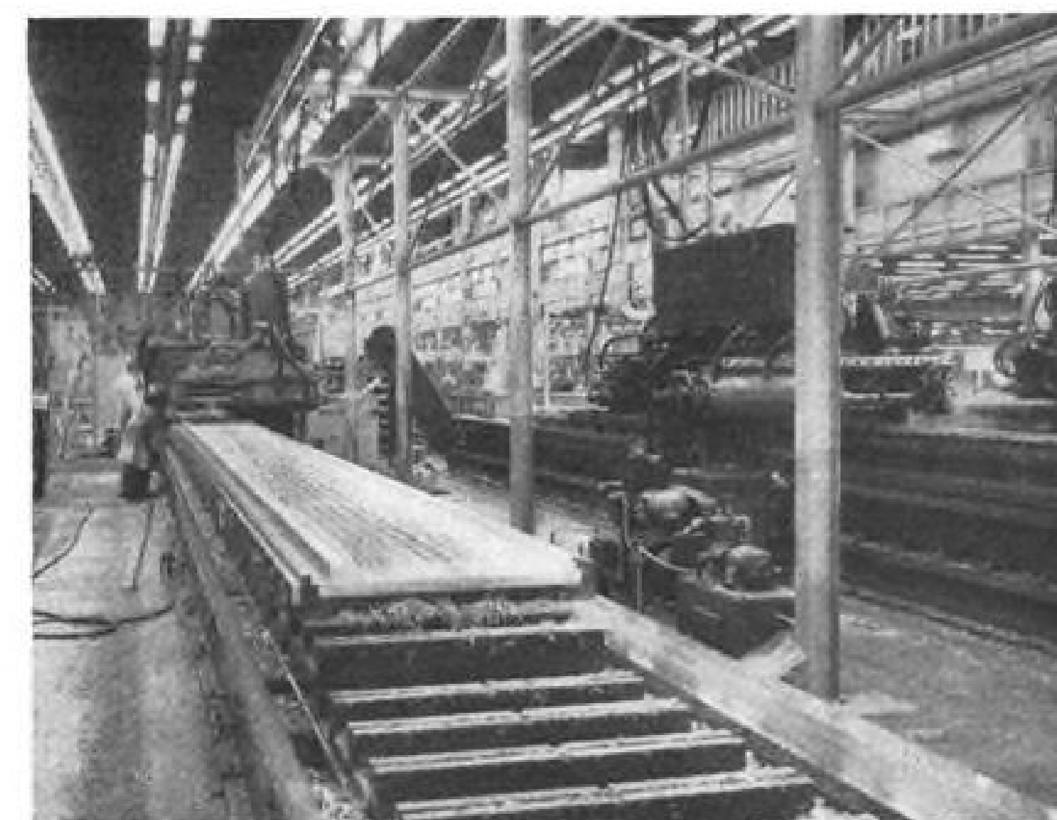
BIG MACHINES—Onsrud skin mill (left) produces integrally stiffened wing interbeam skin; then Giddings and Lewis mill cuts taper.
