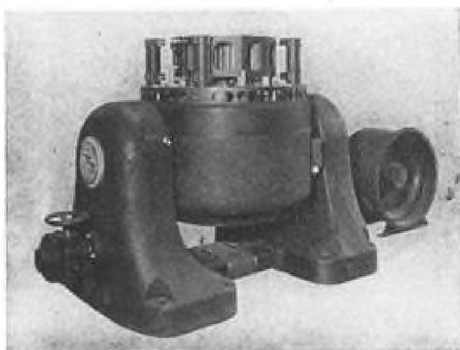
C-100 exciter produces 12,500 lb. force.
