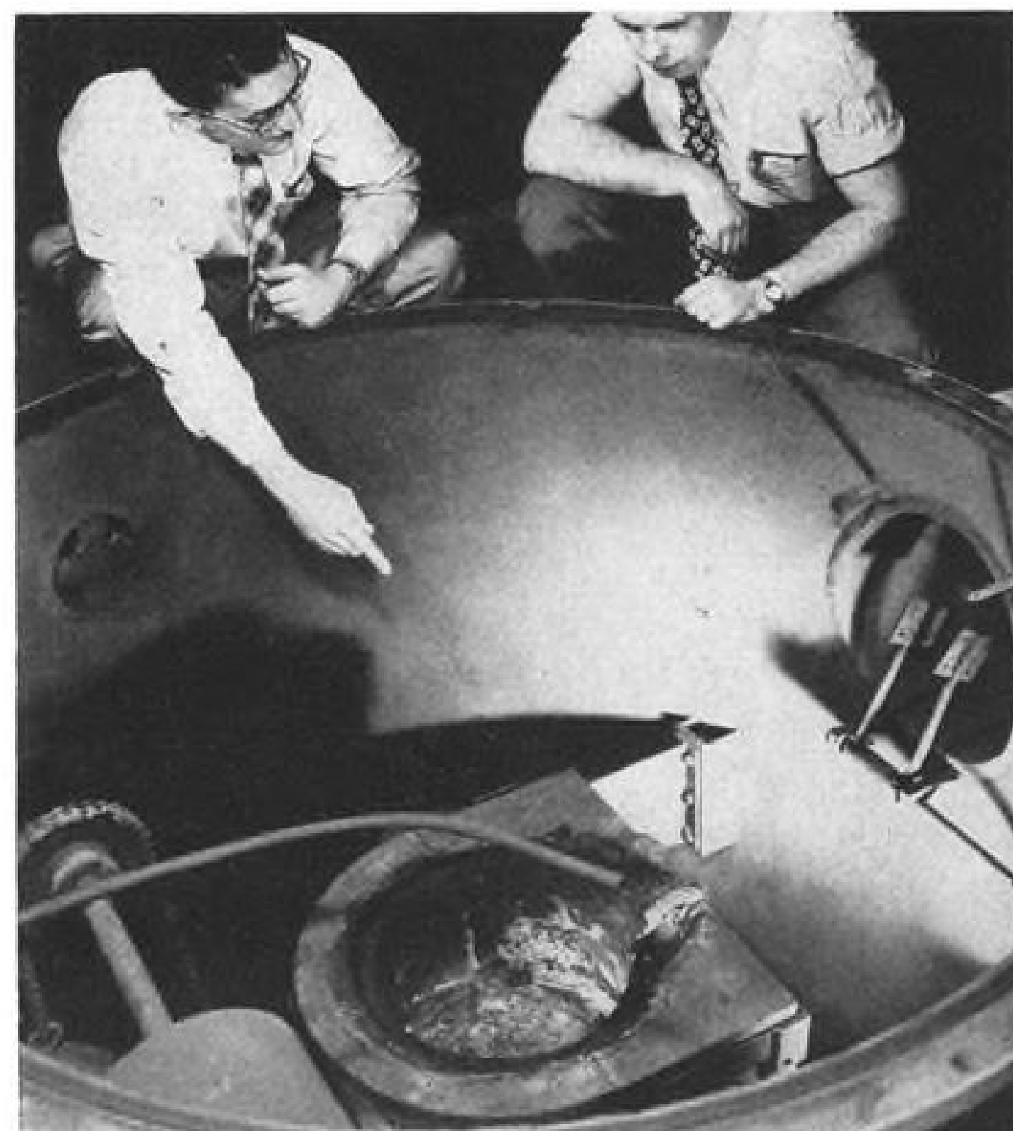
HIGH-PURITY, HIGH-HEAT-RESISTANT jet alloys are produced in vacuum furnaces at Utica Drop Forge (left) and GE (right). The Utica unit, designed and built by F. J. Stokes Machine Co., has 1,000-lb. capacity, is said to be the largest of its type ever constructed.
