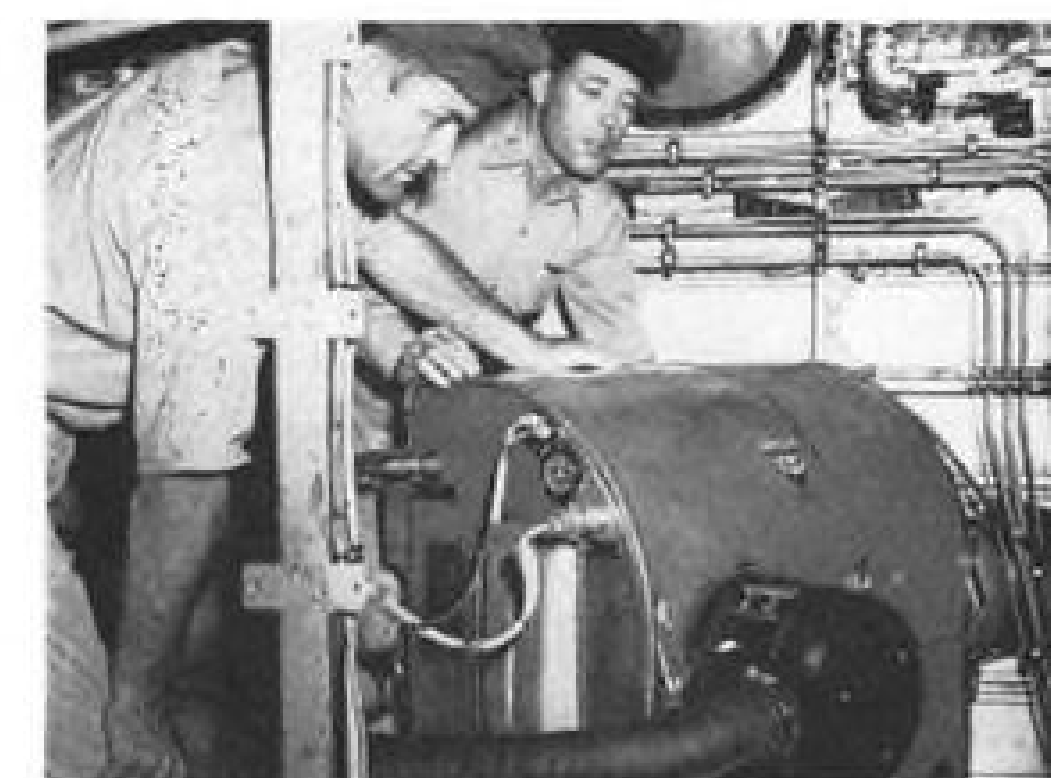
A flick of a switch in the Douglas Globemaster starts Solar APU (above); below, Air Force officers check gas turbine generator set installation in the huge transport.
