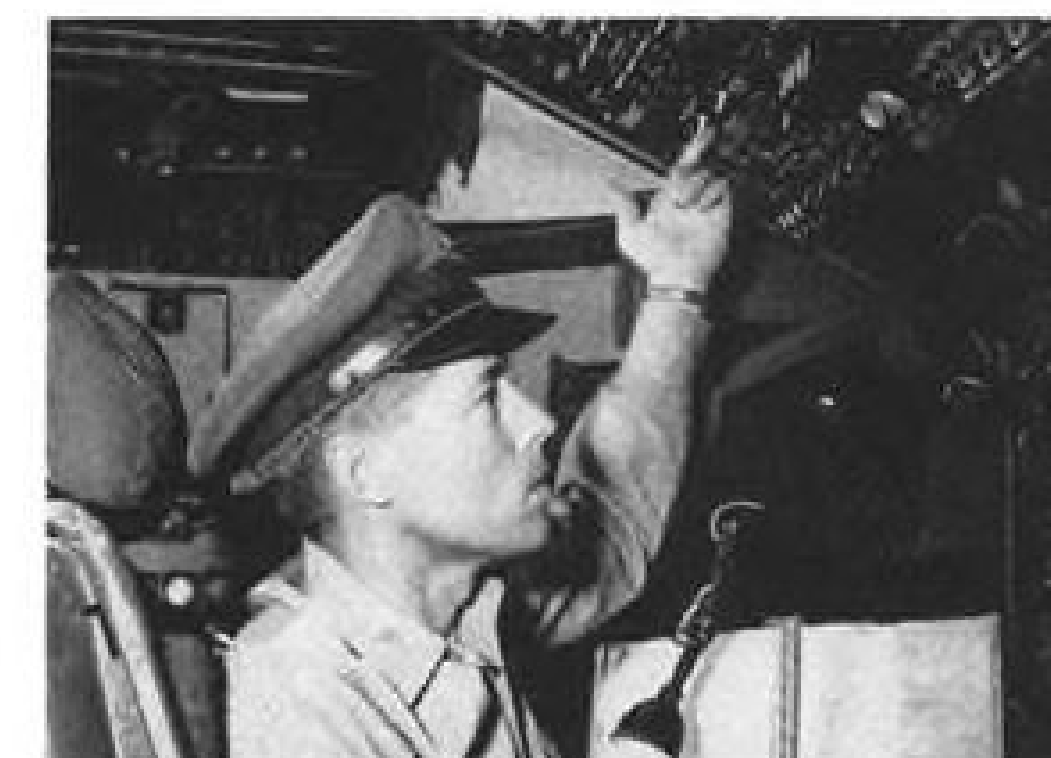
A flick of a switch in the Douglas Globemaster starts Solar APU (above); below, Air Force officers check gas turbine generator set installation in the huge transport.
