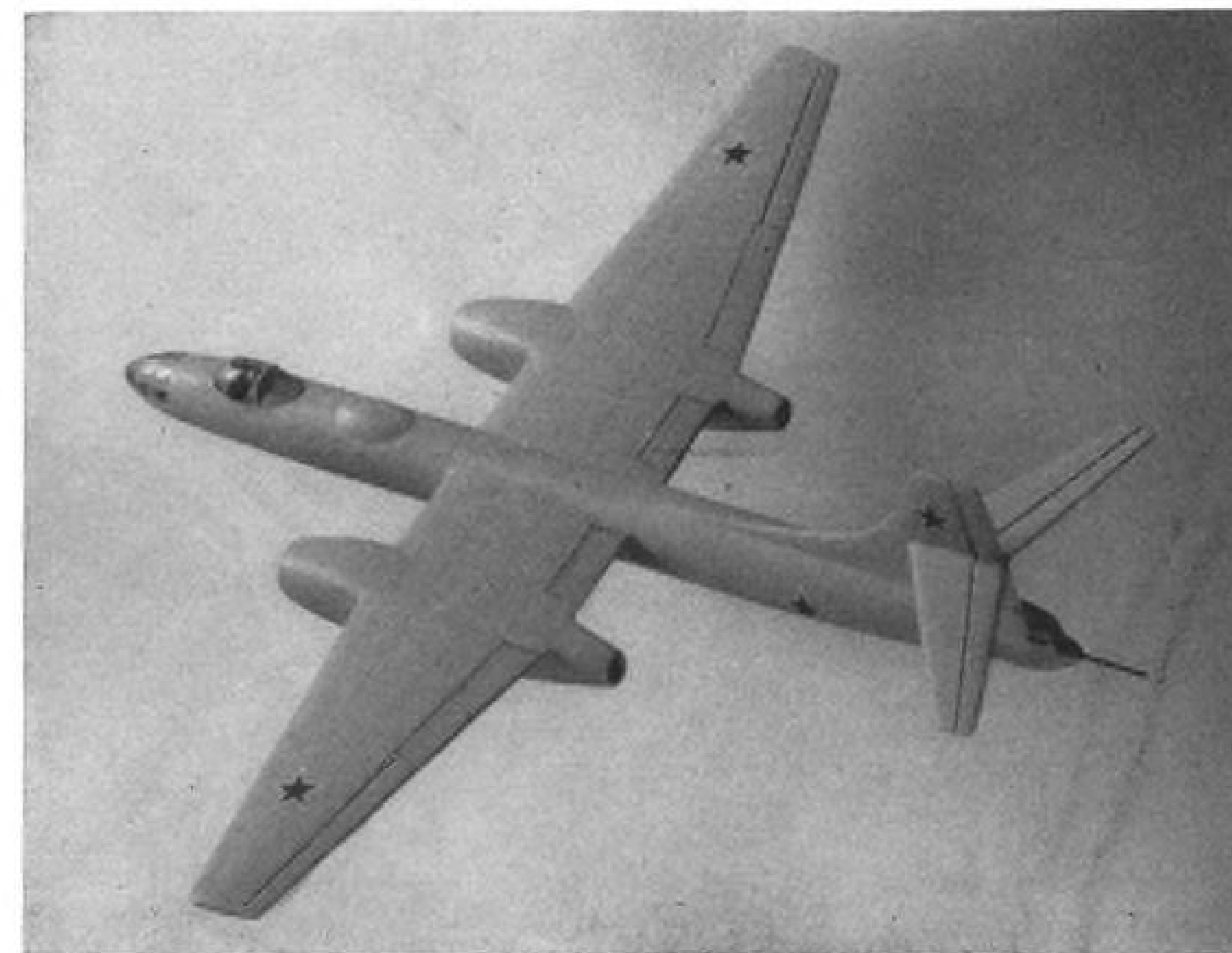
BOSUN is twin-jet naval bomber with more than 600-mi. radius, designed to harass shipping.
