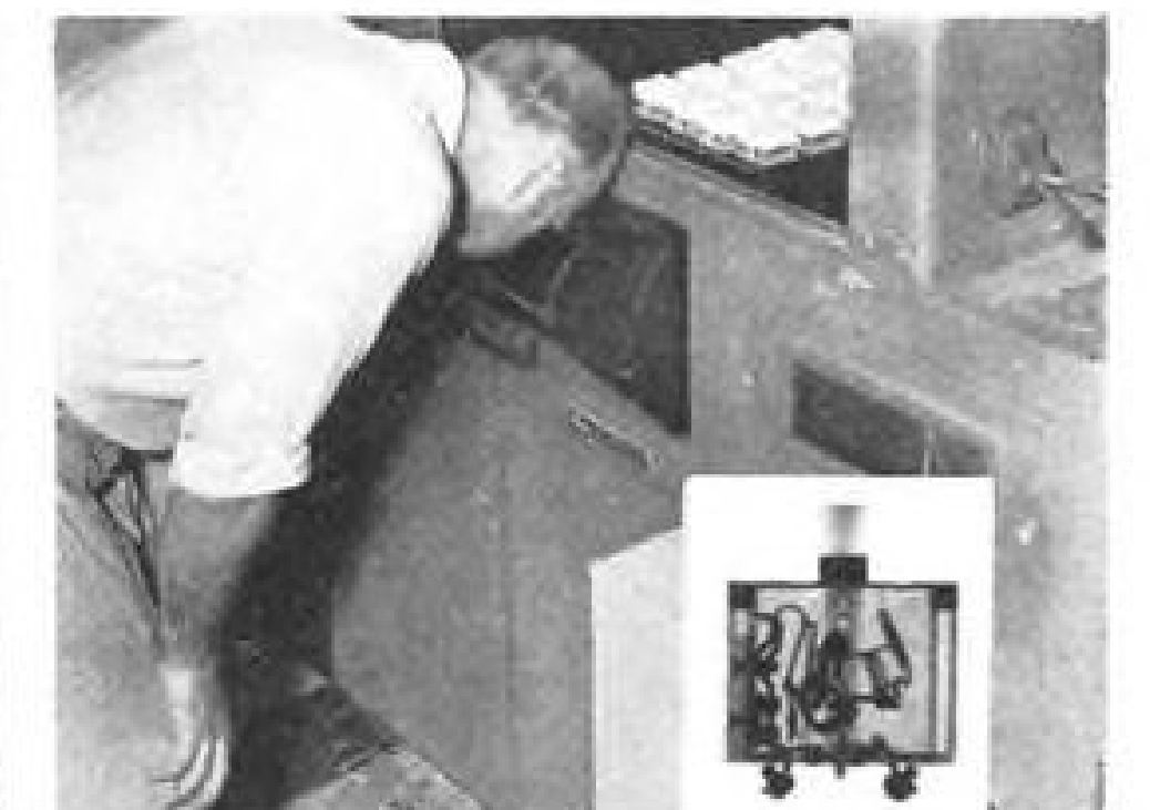
Here Klixon Breakers are X-ray inspected to assure accuracy and quality of workmanship.
