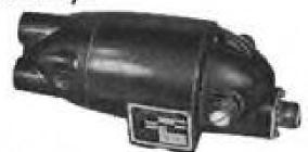
Fluid Metering Pump Series "M" with capacities from 5 to 15 GPH at 20 psi, 271/2 V.D.C. Width 31/6", length 6%". Weight 2.75 lbs. Single and dual outlet types. Meets all anti-icing requirements.
