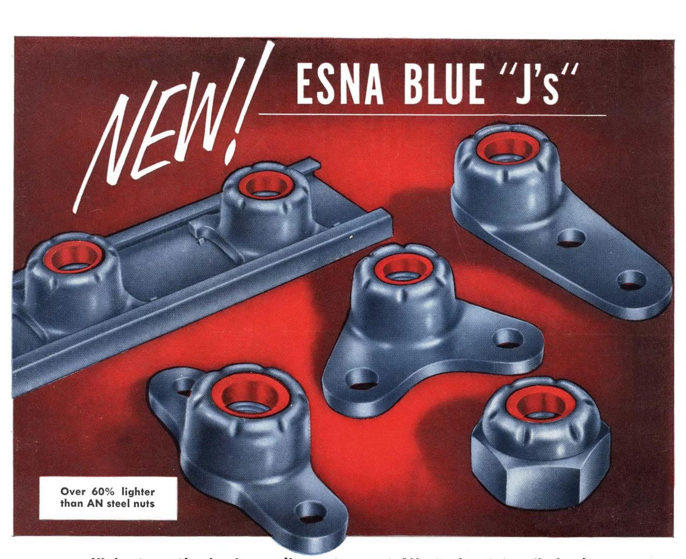
High-strength aluminum-alloy nuts meet AN steel nut tensile loads. Nylon locking inserts guarantee reusability through 50 on-off cycles.
