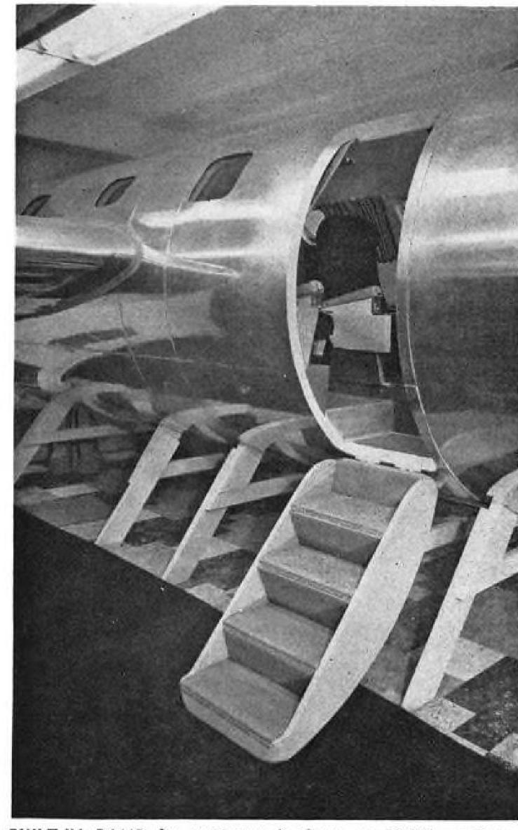
BUILT-IN RAMP for passengers is shown on B-57B mockup. EIGHT-PASSENGER mockup includes four-place divan.
