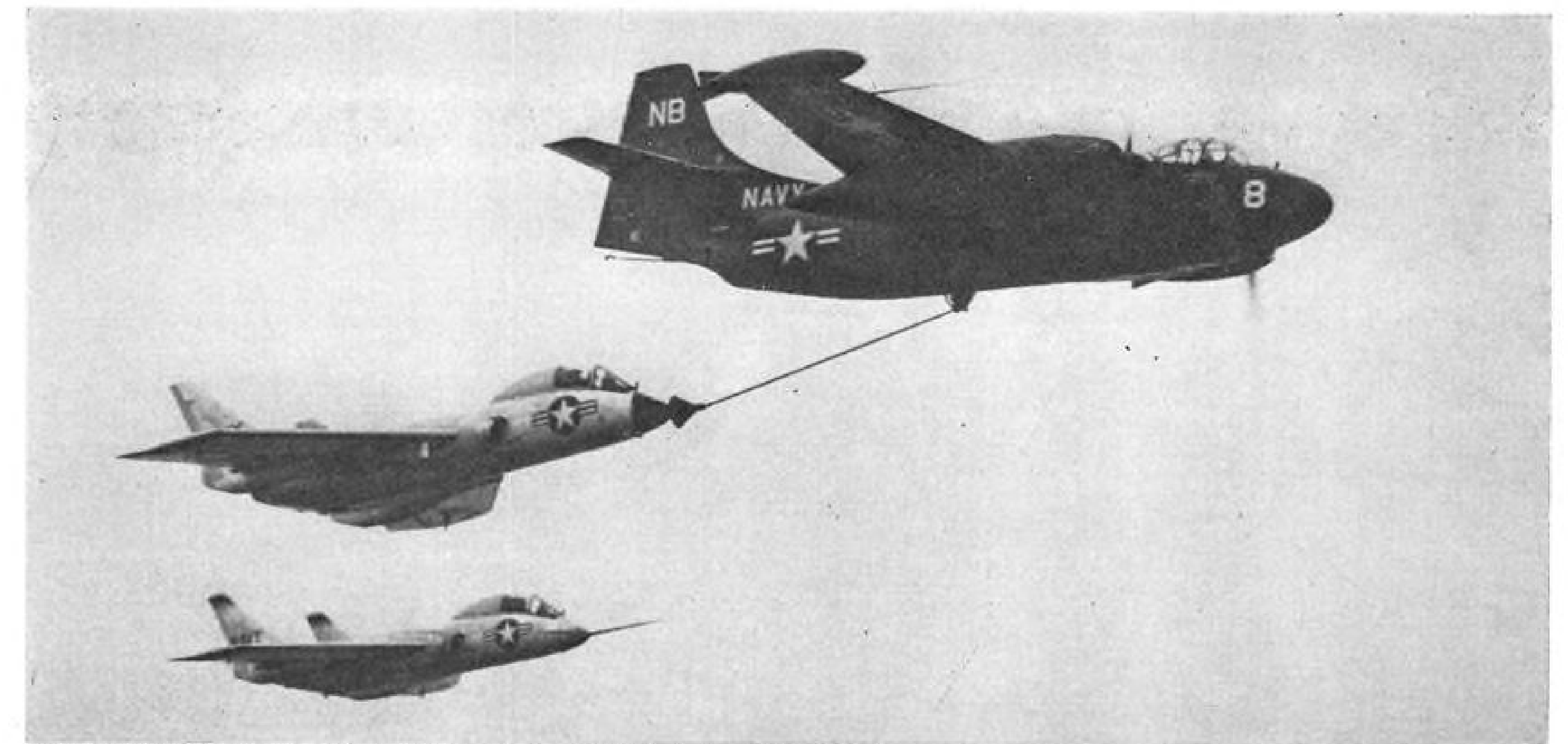
AJ-1 TANKER-BOMBER refuels F7U-3s during inflight tests of the Navy's new concept of quickly convertible carrier-based tankers.
