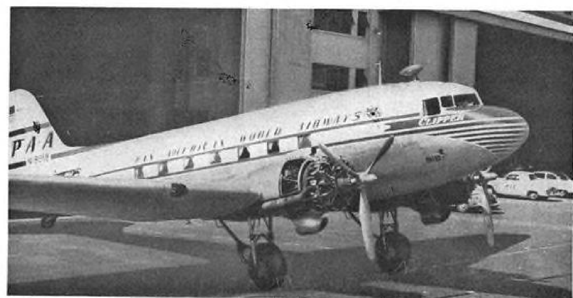
HI-PER DC-3 modification of Douglas transport, which mounts R2000 powerplants.
