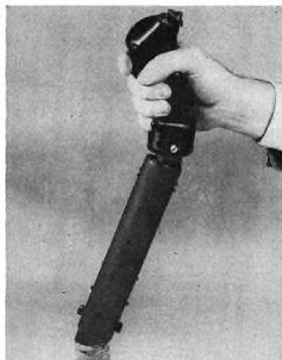
DOUBLE-DUTY STICK is used for both autoflight and manual control maneuvers.
