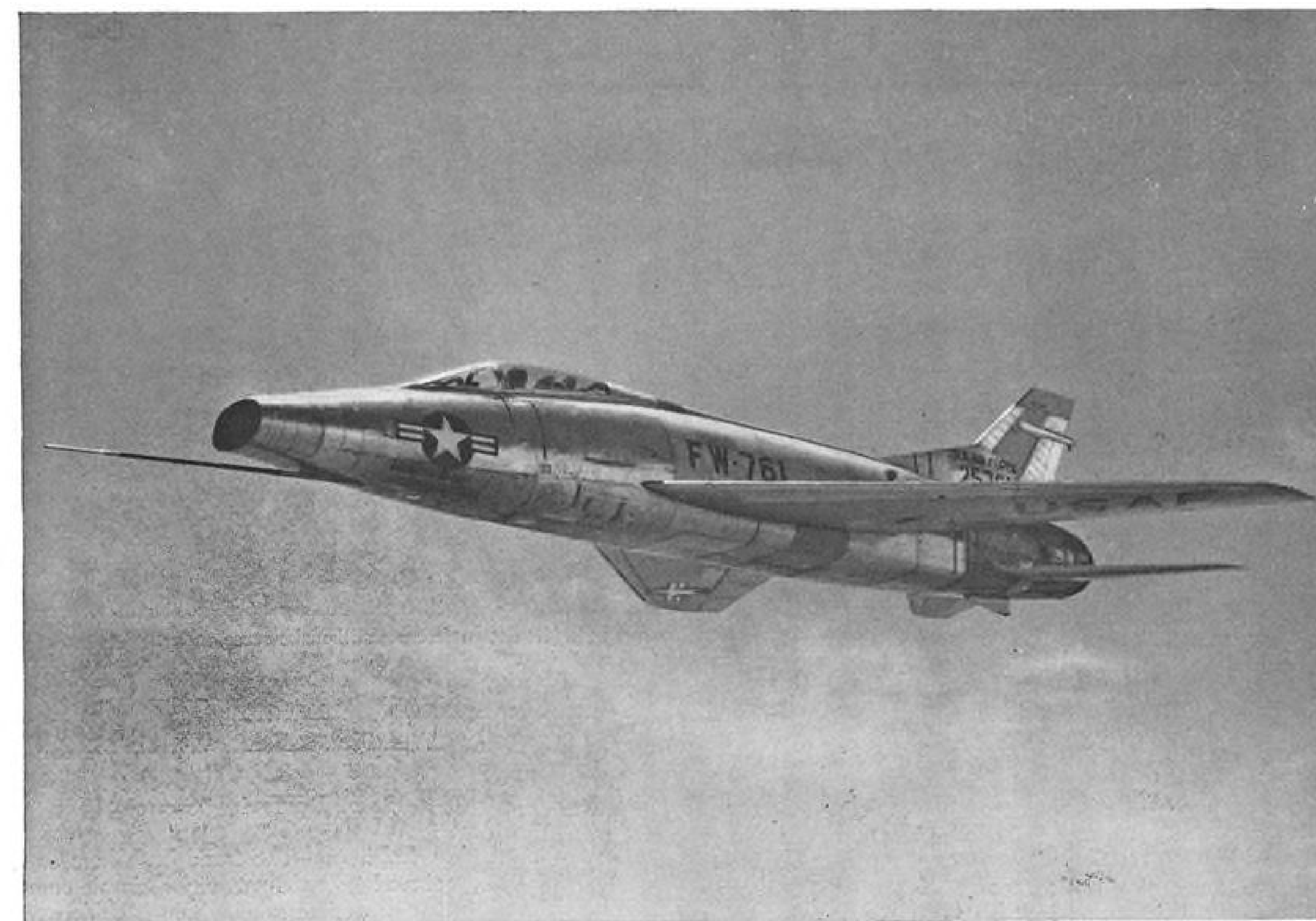
Sharply swept-back wings and tail surfaces mark the North American F-100 Super Sabre. Built around one Pratt & Whitney Aircraft J-57 turbojet and afterburner, the Super Sabre is the Air Force's first operational supersonic jet fighter.
