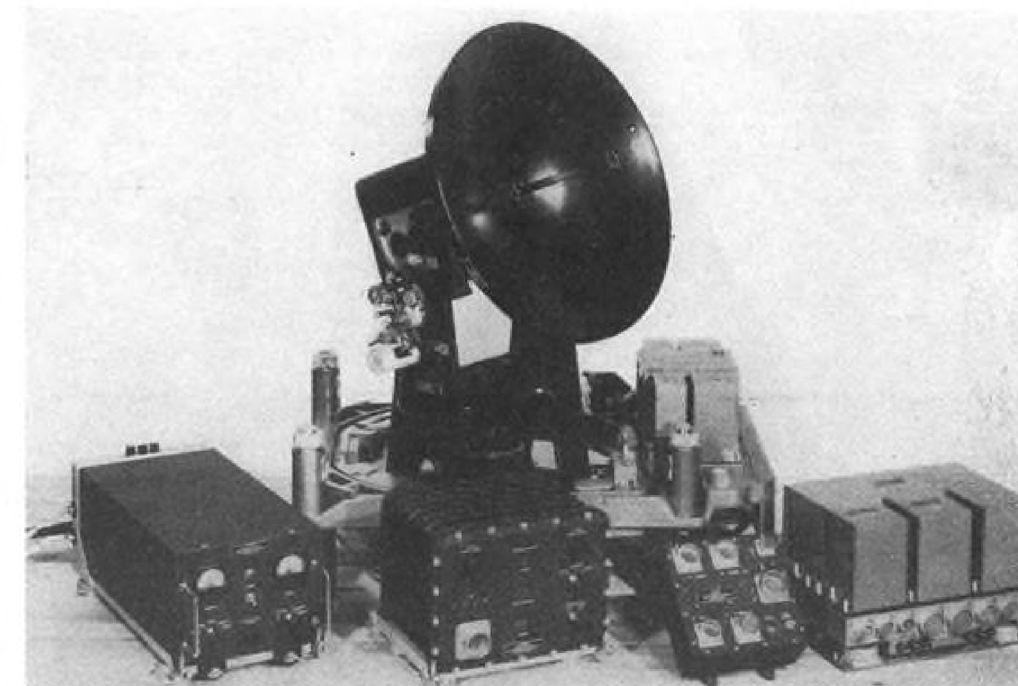
AIRBORNE RADIO SEXTANT , mounted on stabilized platform, could be used for longrange navigation of aircraft and missile. Photo shows components of airborne unit.
