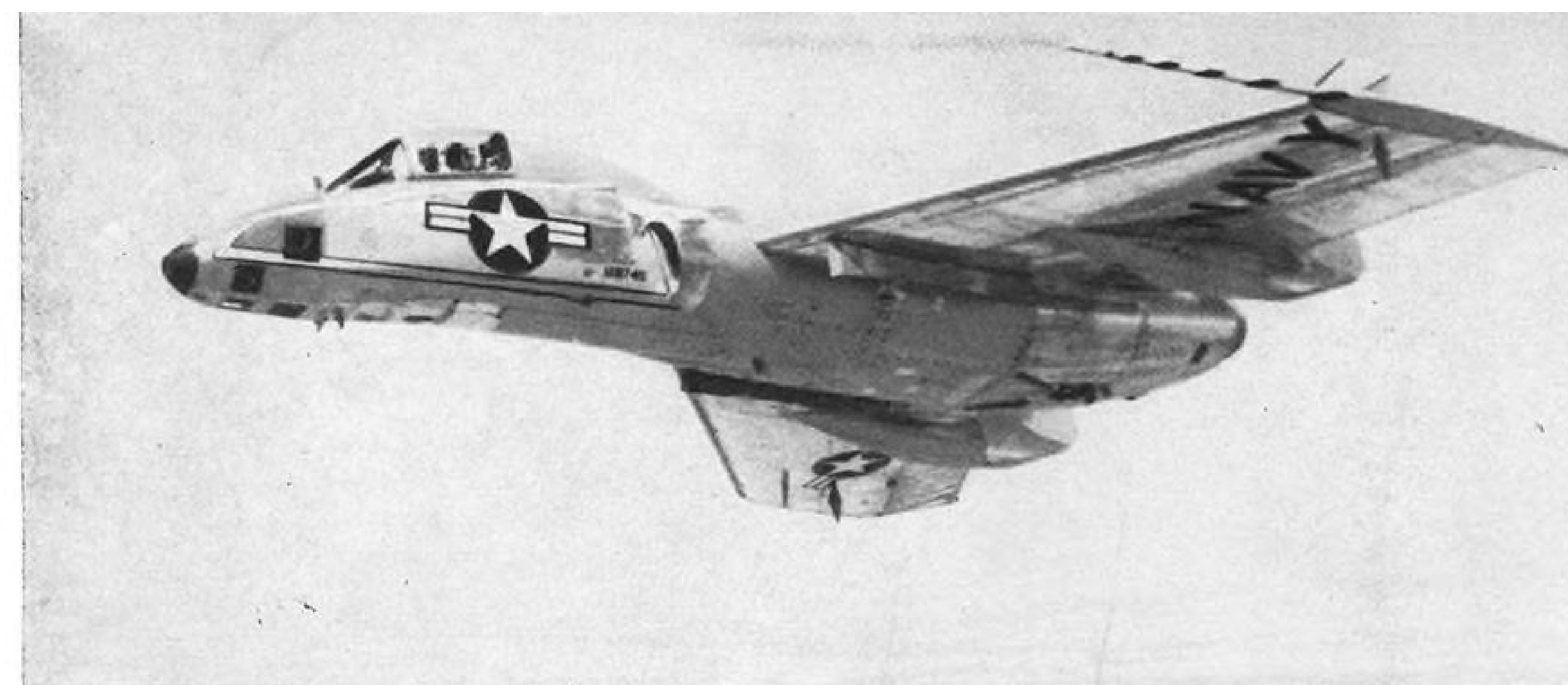
CUTLASS WITH CAMERAS, designated F7U-3P, has 25 in. longer nose than fighter versions and carries 104 flash flares for night photographs in the top of its twin jet intakes. The Cutlass normally carries multiple 20-mm. cannon above intakes.
