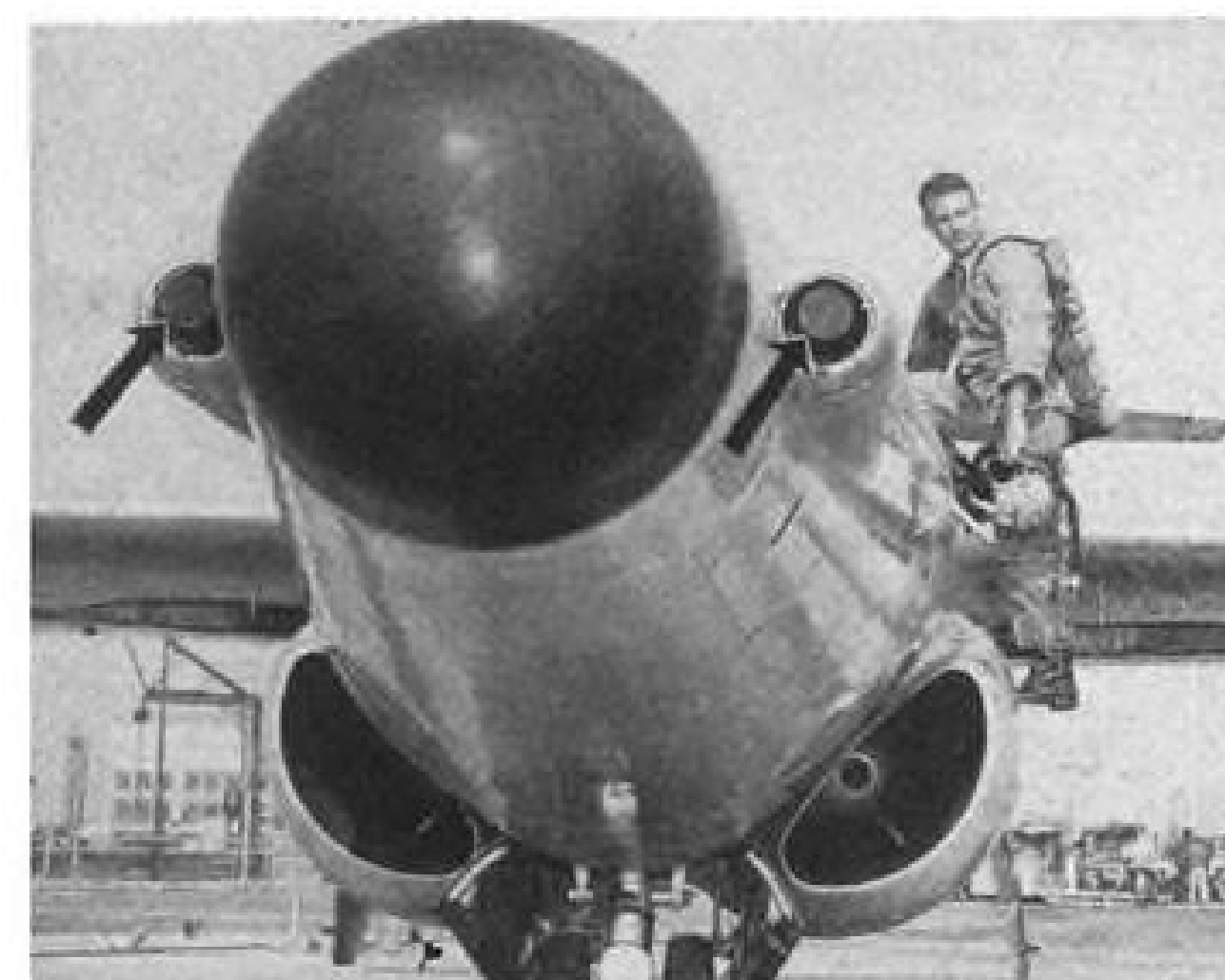
AUTOMATIC ROCKET GUNS on either side of Northrop F-89C Scorpion test bed's nose are product of Armour Research Foundation. Developed under Army Ordnance contract, they are designated T-110 launchers. Units are tested on F-89 mockup in photo at right.
