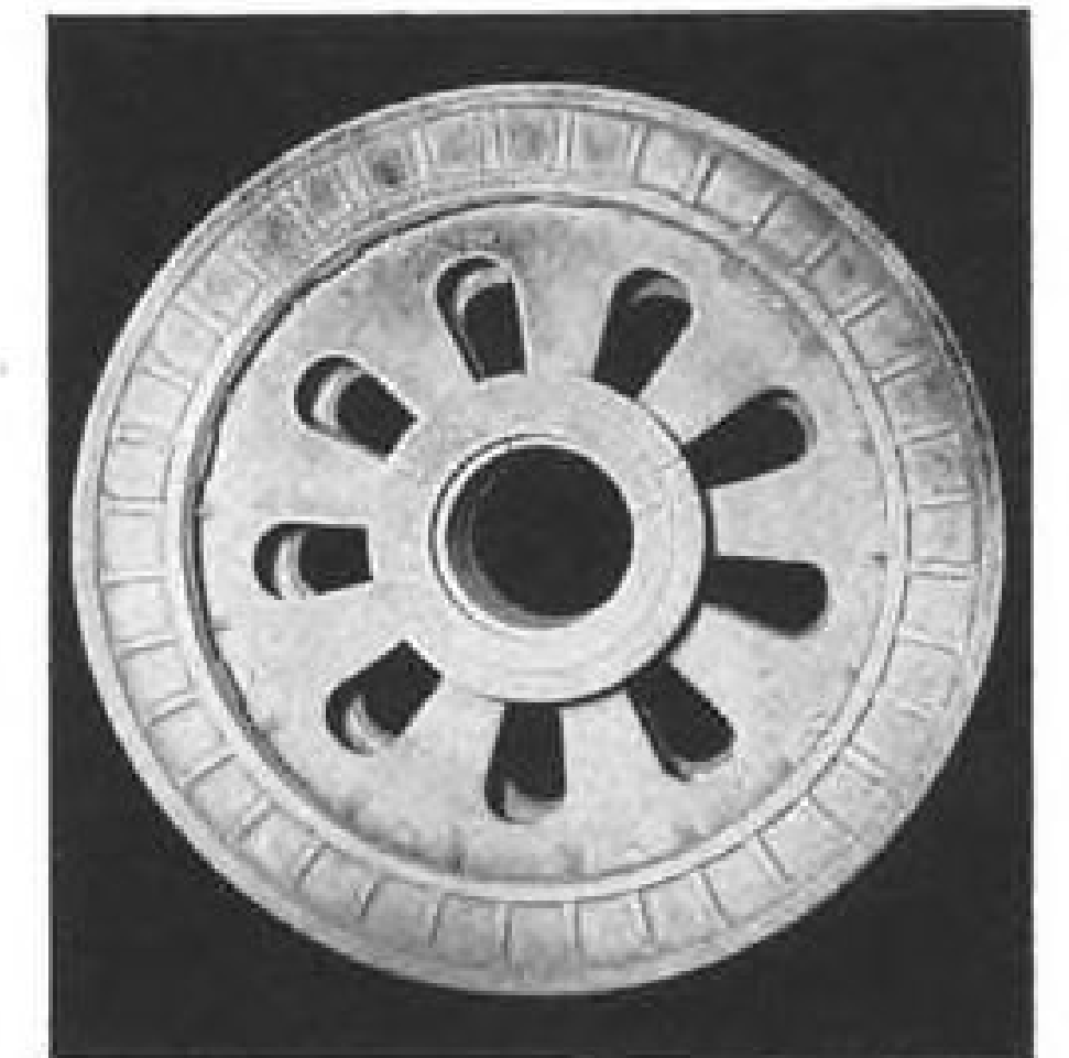
Extra-light aircraft wheels of Alcoa Magnesium—like this type, used on the Air Force's B-47 "Stratojet" bomber.
