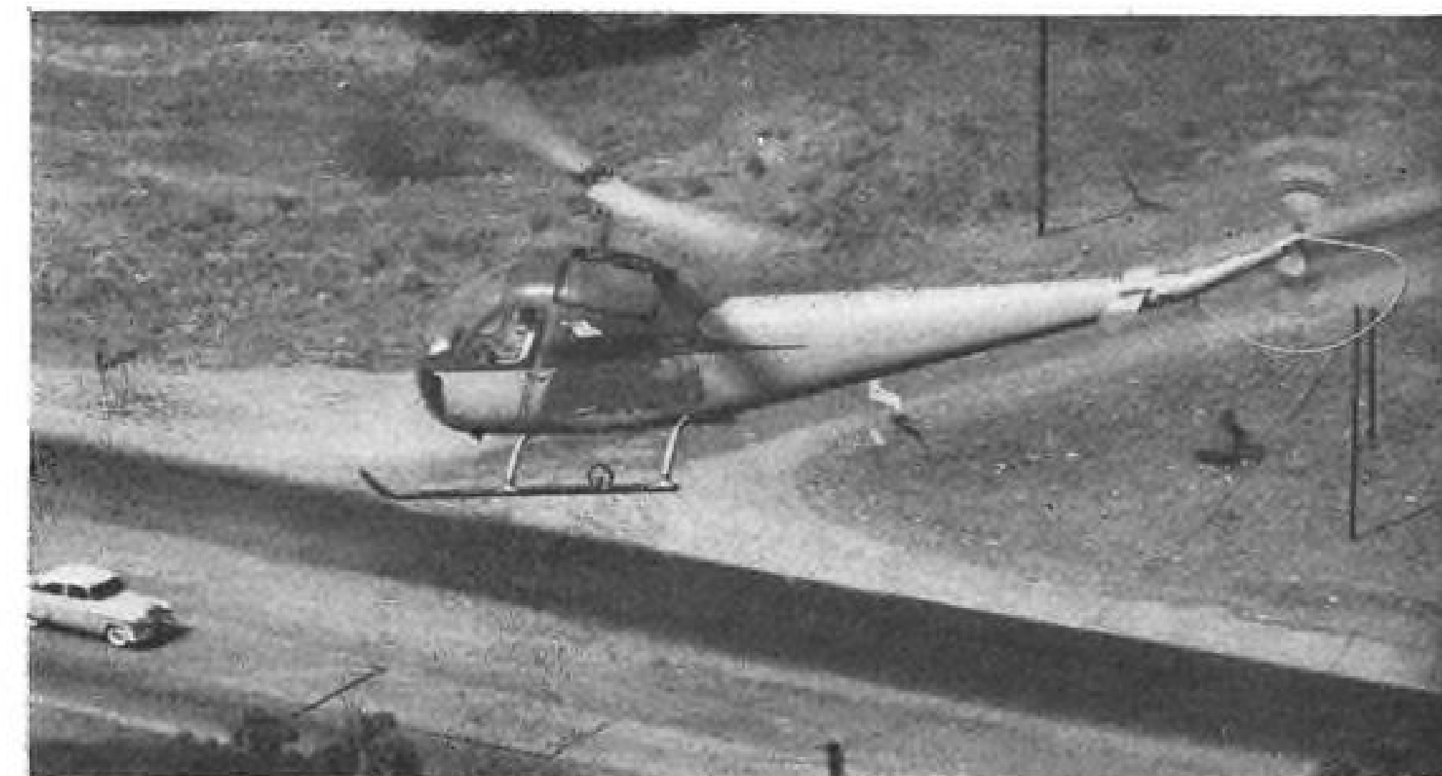
STREAMLINING of basic Bell 47G gives new 47H (above) about 20% higher speed and proportionate reduction in fuel consumption. Now undergoing CAA certification trials, the copter's general configuration is similar to the 47G (Aviation Week Sept. 13, p. 17).
