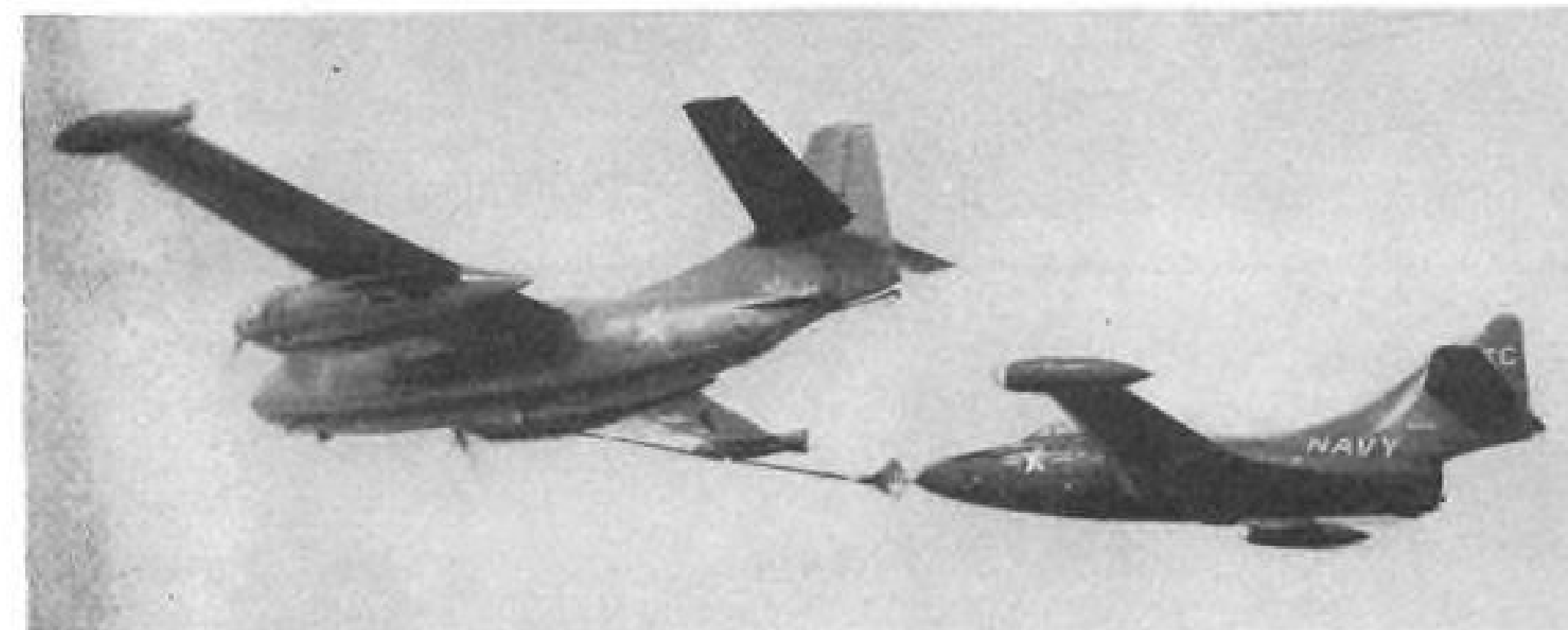
IN NAVY TESTS, North American AJ-1 tanker refuels Grumman F9F Panther at sea.
