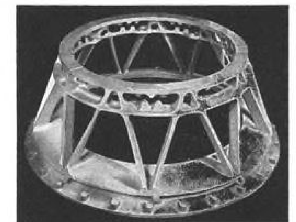
Another intricate job, this one a light weight engine support for a Pratt & Whitney Aircraft turbojet engine.
