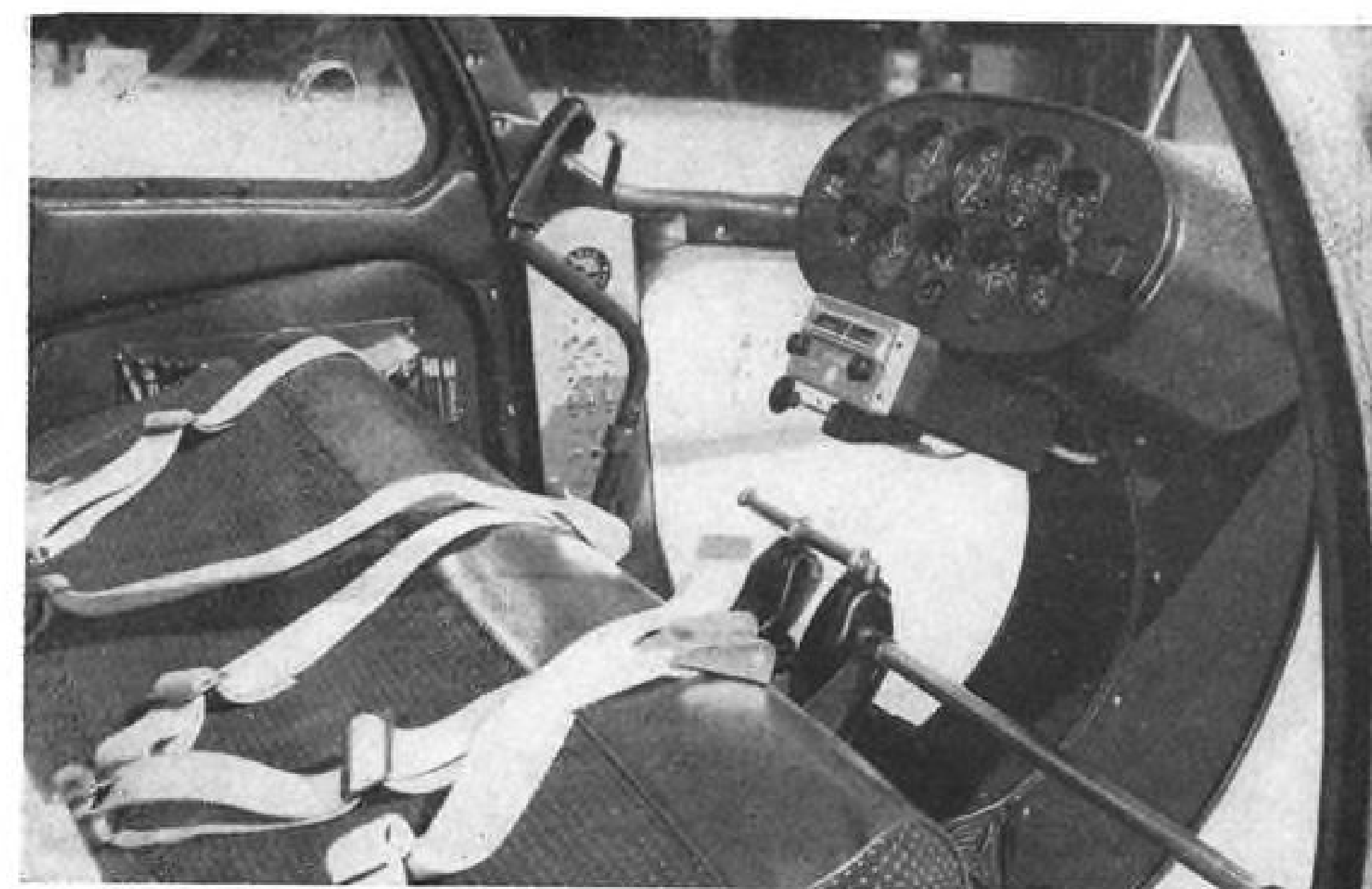
INSTRUMENT CONSOLE is located at pilot's left to give him and passengers more room in the 47H's enlarged 60-in. wide, side-by-side cabin. Seats are automobile size.
