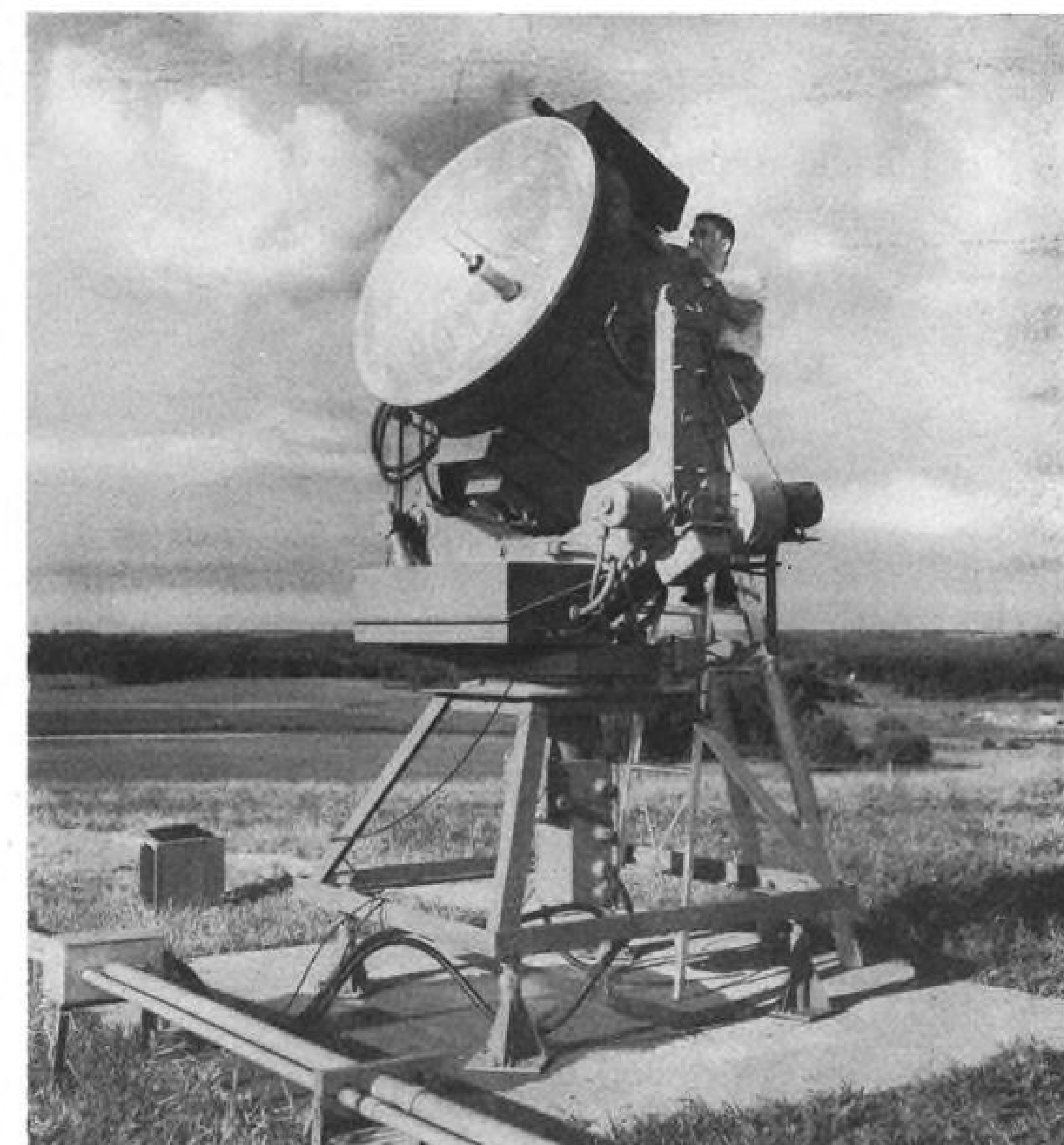
EXPERIMENTAL RADIO SEXTANT , under test by Collins Radio near Cedar Rapids, is housed in a war-surplus Navy searchlight. Sextant tracks sun, even through overcast.
