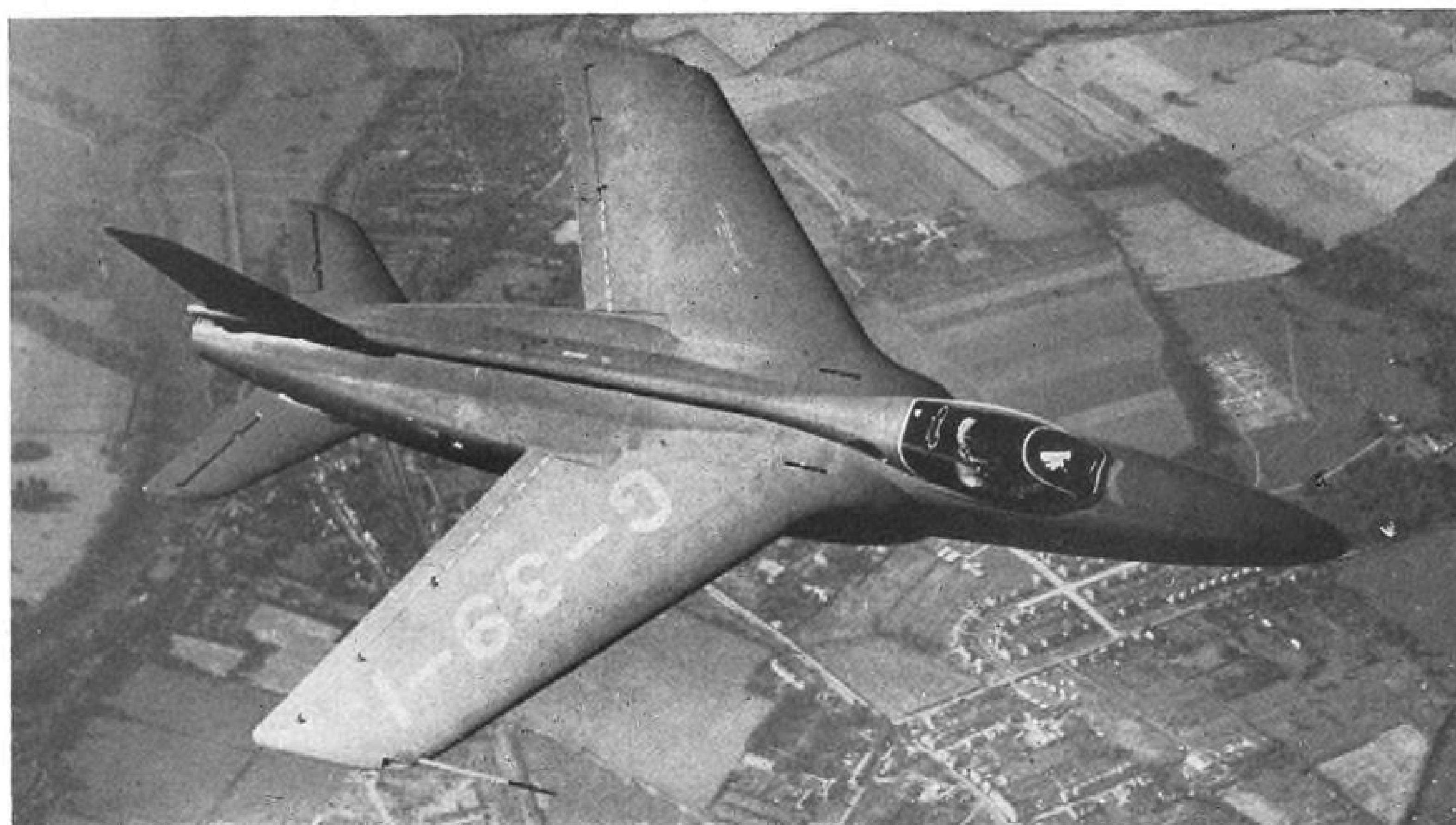
MIDGE is flying with Viper jet in place of higher-thrust Orpheus that will power production Gnats. Dorsal spine houses control cables.
