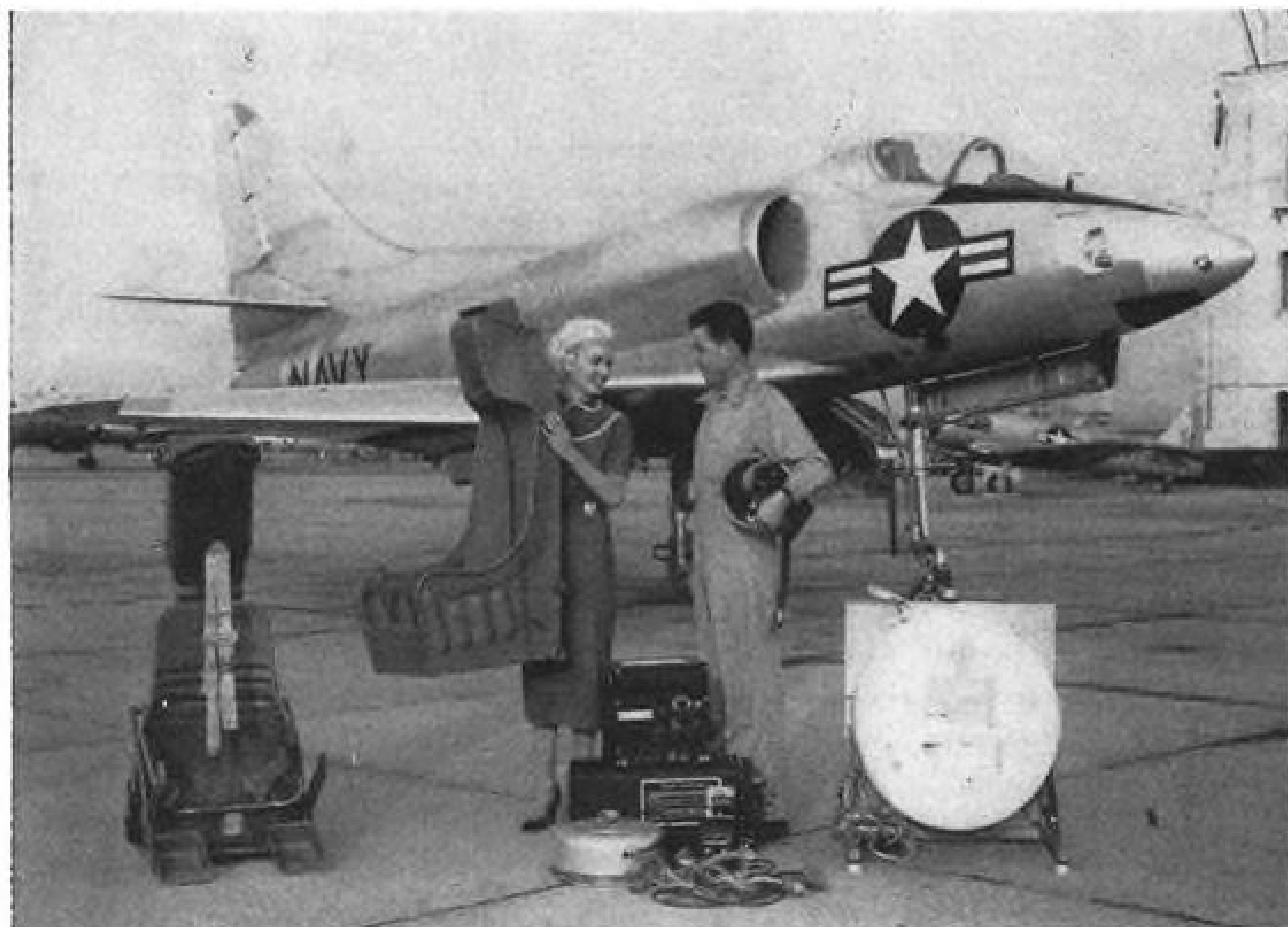
DOUGLAS XA4D-1 SKYHAWK shows weight savings: seat at left has 240 parts, weighs 98 lb.; A4D's seat has 80 parts weighs 40 lb. Conventional complex avionics gear (center) has been completely repackaged for Skyhawk (right) at saving of 48 lb.
