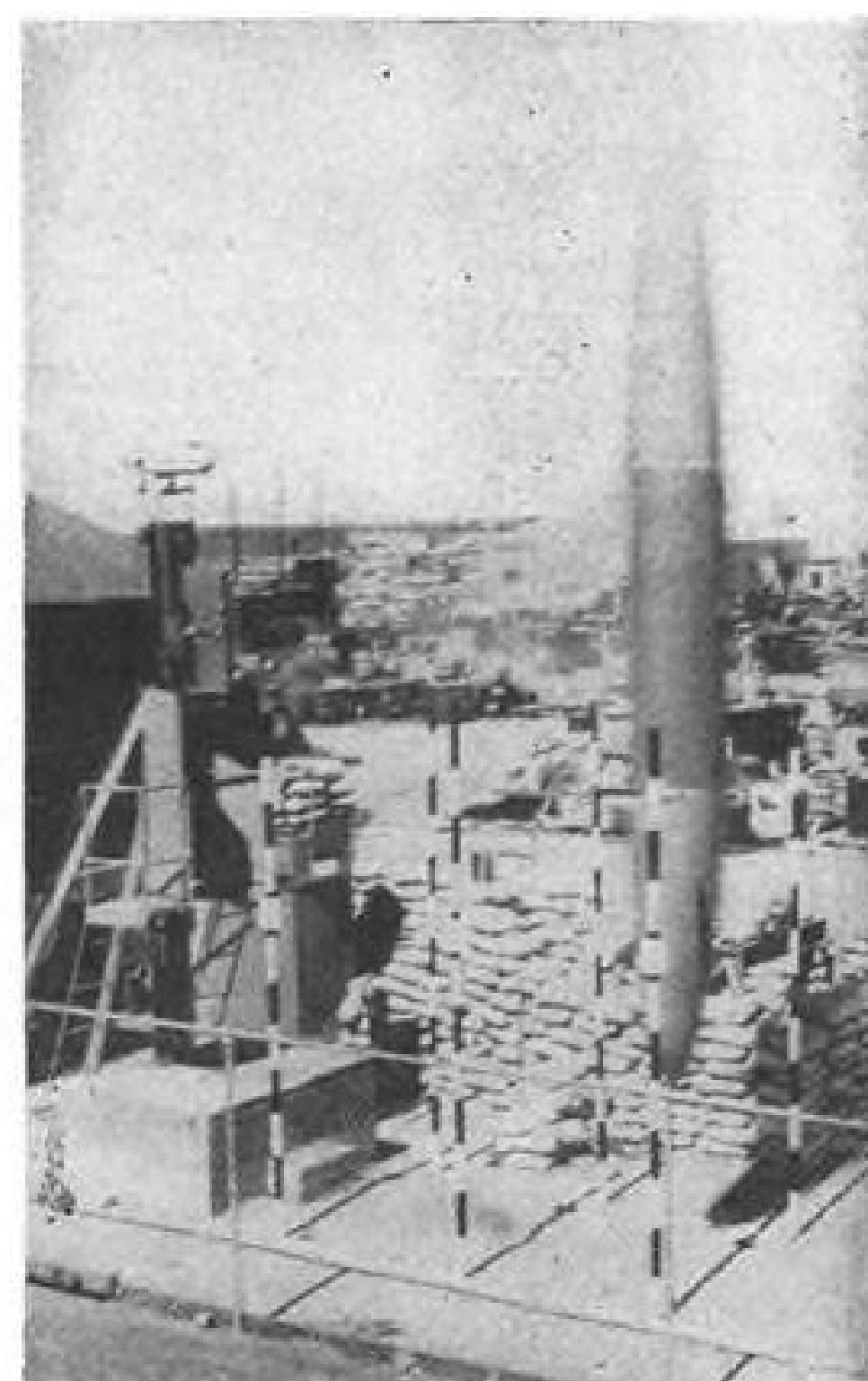
FORCE EJECTION separates tank from pylon using explosive. Tank is fixed vertically (left) to ejection tester, is hurled (right) between rows of calibrated poles.
