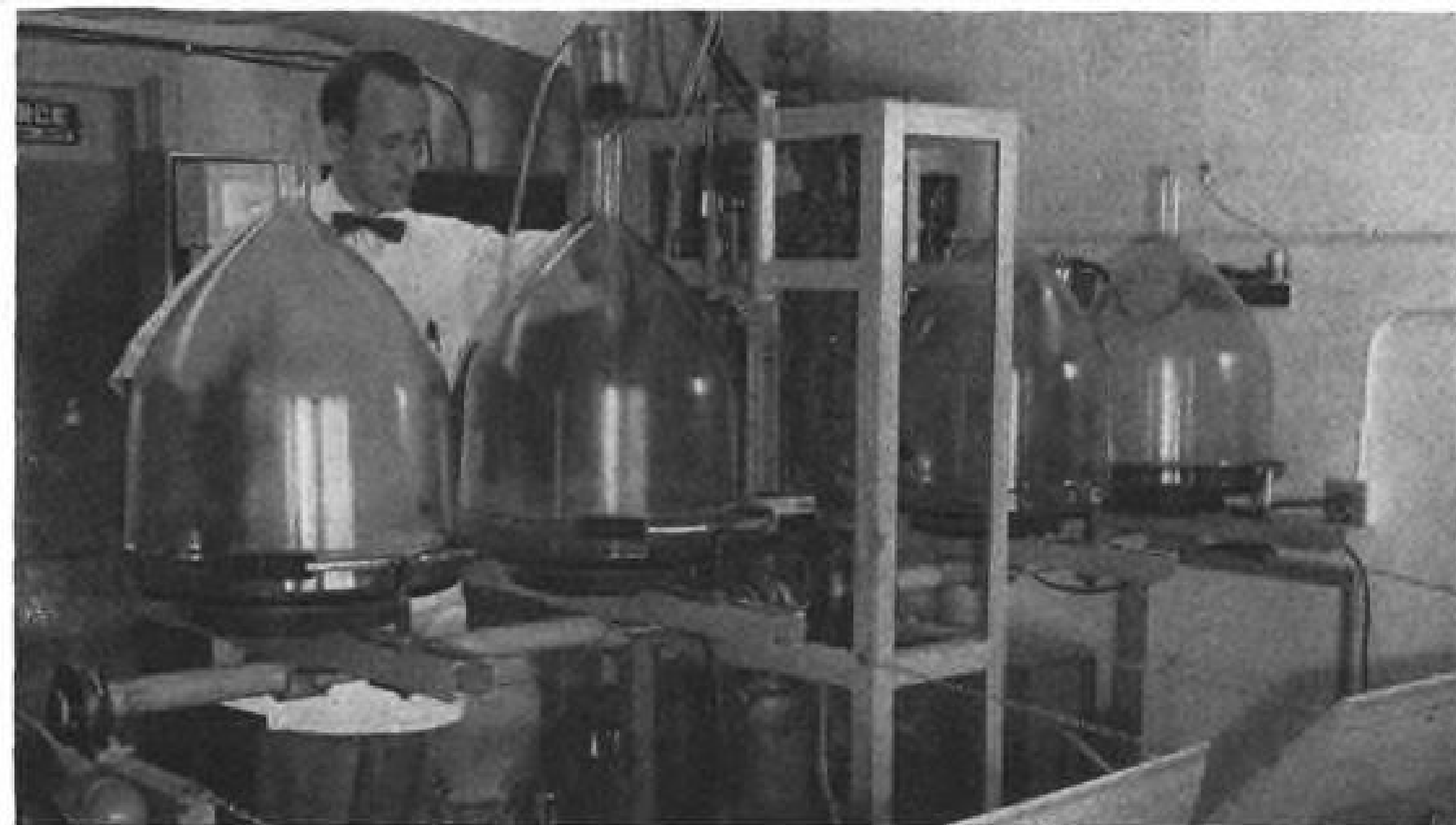
CHARACTRON CATHODE RAY TUBE has vacuum of 2 \times 10^{-7} microns. That is one reason the 19-in. tube costs so many more times than a TV tube of the same size.
