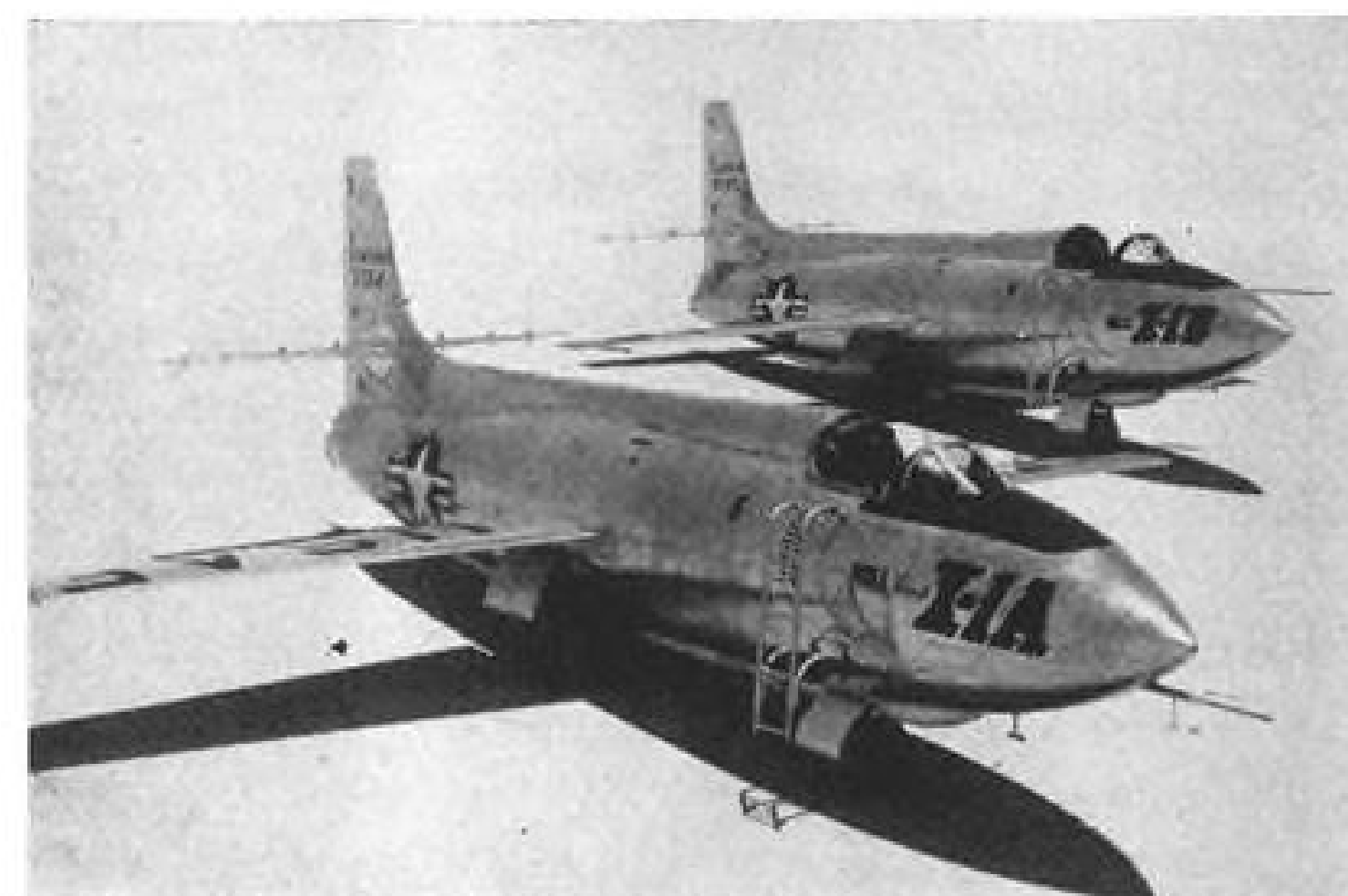
SUPERSONIC TWINS are USAF Bell X-1A, foreground, and X-1B, identical except for instrumentation. Rocket-powered planes are at Edwards AFB, Calif. X-1A attained 1,650-mph. speed, 90,000-ft altitude.
