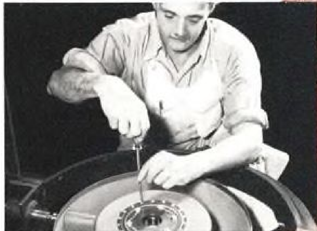
The simplicity of the J44 construction means easy field maintenance using only standard equipment.
