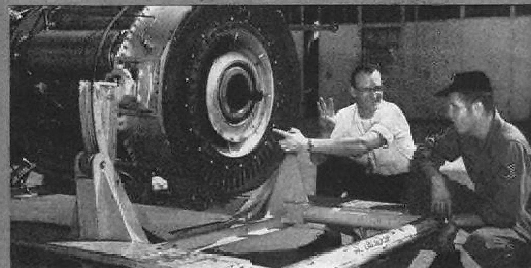
IMPROVED RELIABILITY in the J47-GE-33 engine is illustrated by the new "floating" shim shroud visible above. It reduces the possibility of shroud ring rub on turbine wheel buckets. G-E tech rep is pointing to new adjustable turbine baffle.
