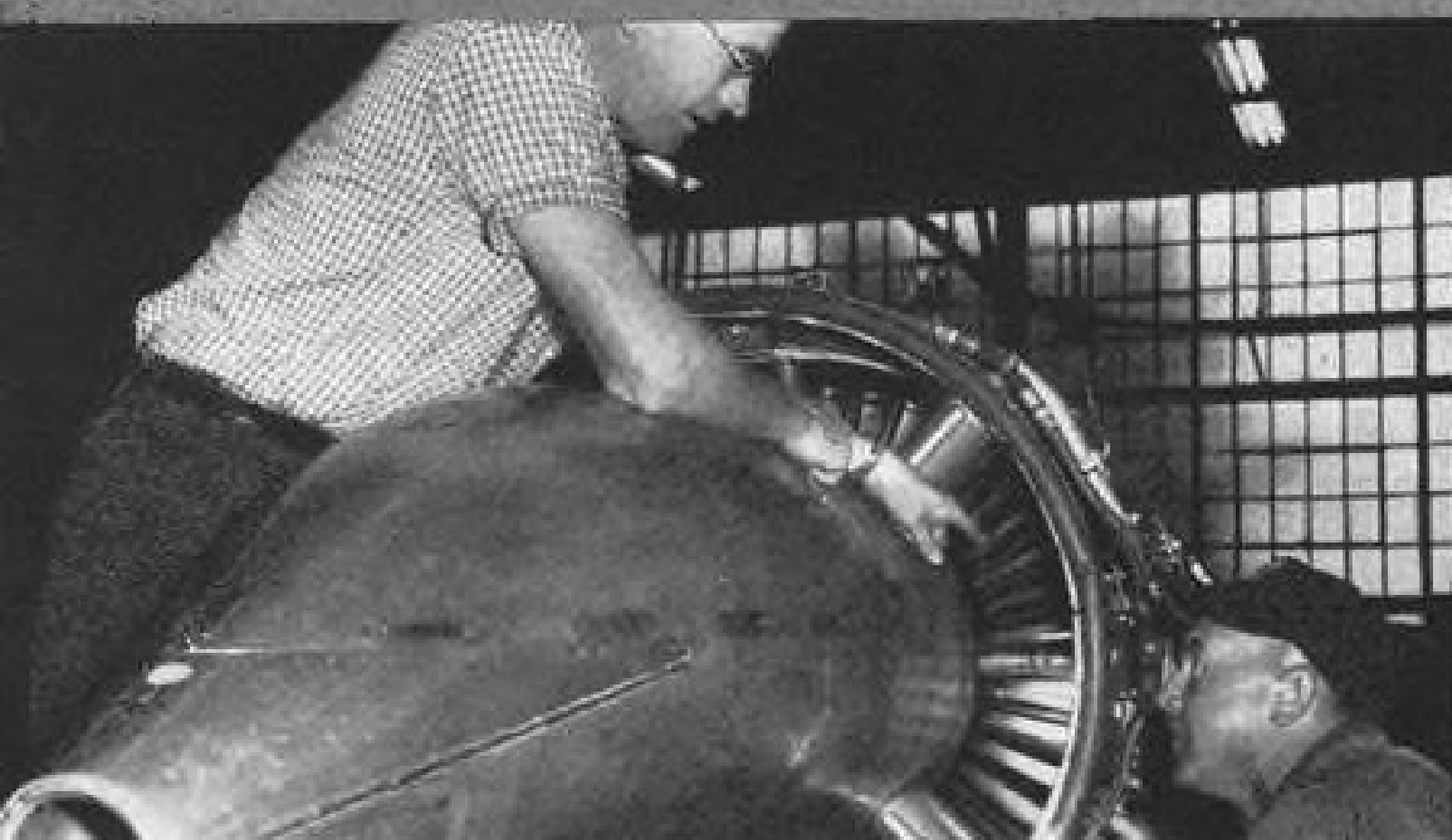
NEW INLET GUIDE VANES allow more air to enter compressor of J47-GE-33 engine. New vanes have same configuration as those used on J47-GE-17, but pay off in increased thrust during dry and afterburner operation.
