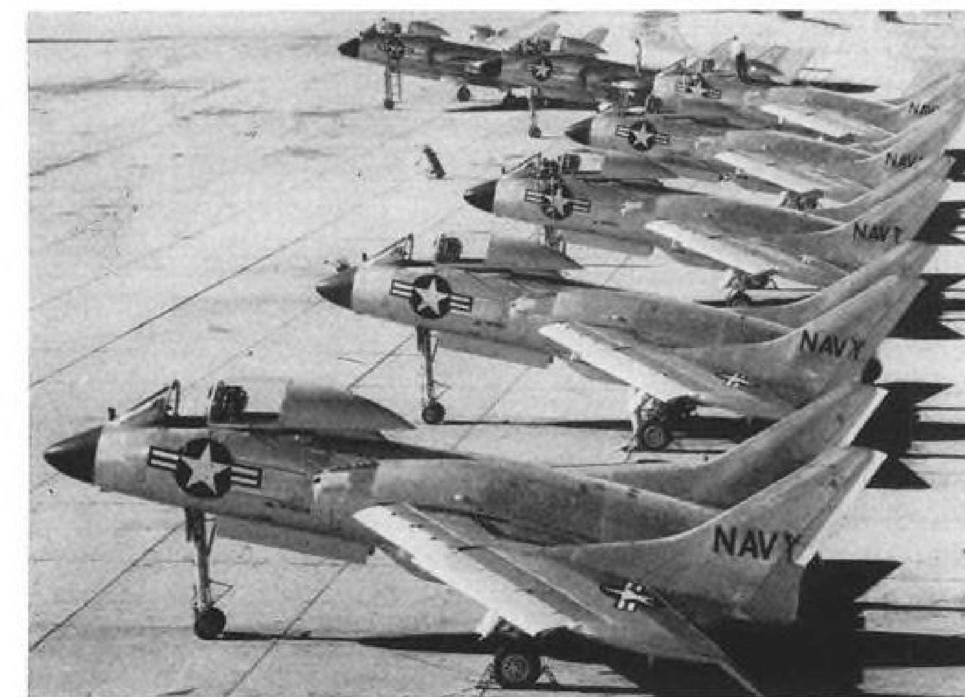
BEVY OF CUTLASSES, with underbelly rocket pods, await delivery at Chance Vought's Dallas plant to Navy squadrons on both coasts. The F7U-3's two Westinghouse J46-WE-2 turbojets have afterburners. Stencil on lower portion of F7U-3's tail reads: Experimental finish. Do not paint.
