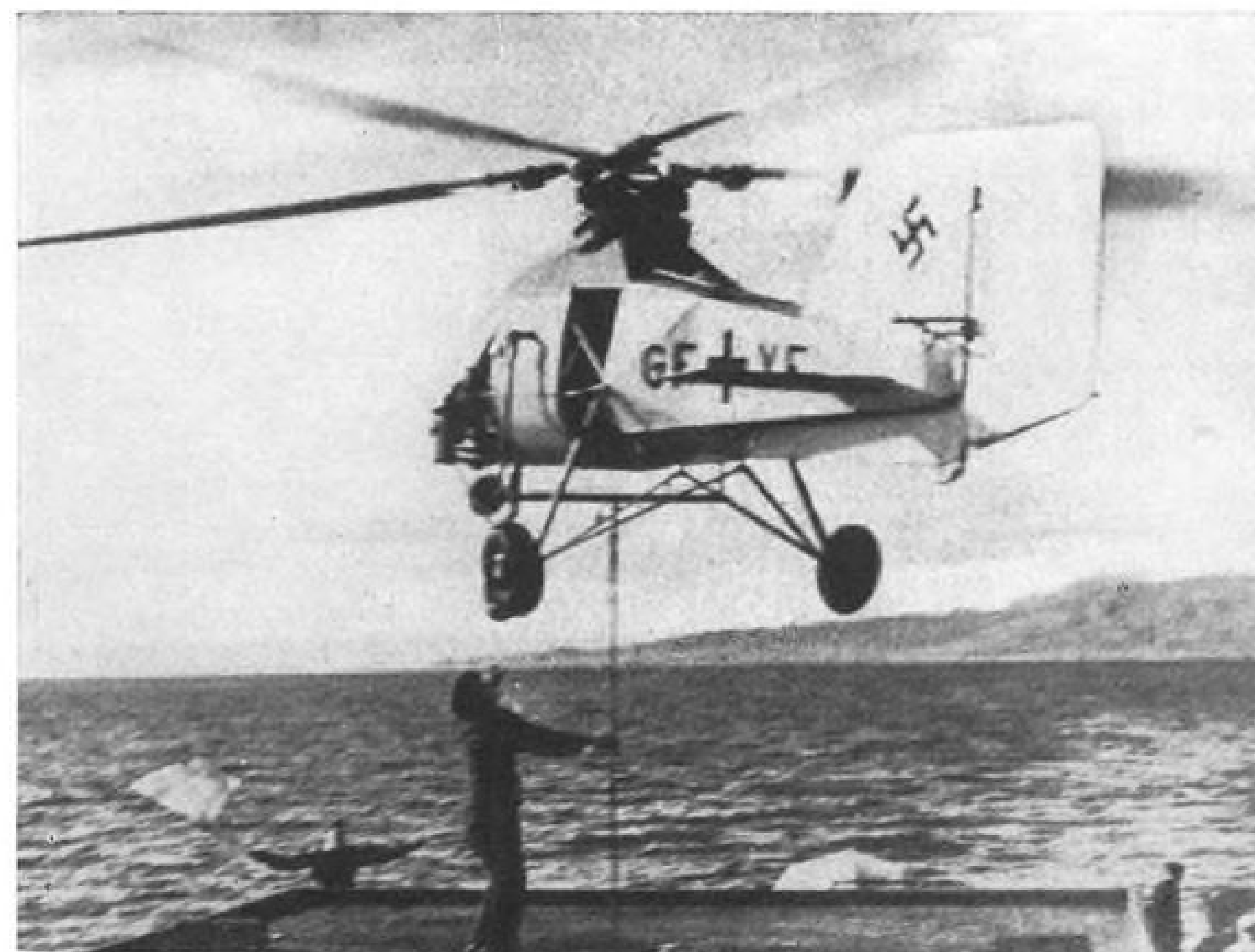
HOOKS ON to hovering craft. Pilot increases lift to maintain tension in cable and copter is winched down. Technique was developed for rough-sea operations.
