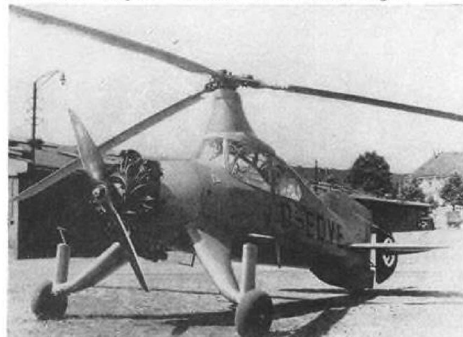
FL-184 AUTOGYRO: First flown in 1935, this pioneering aircraft featured cyclic-pitch control for the rotor.
