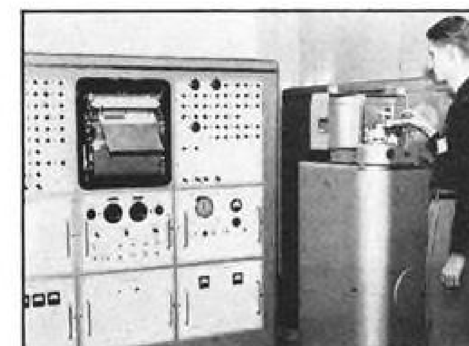
Every production step is subject to strict quality control at Bridgeport Aluminum. This spectroscopy detects alloy elements as low as 0.001 per cent.
