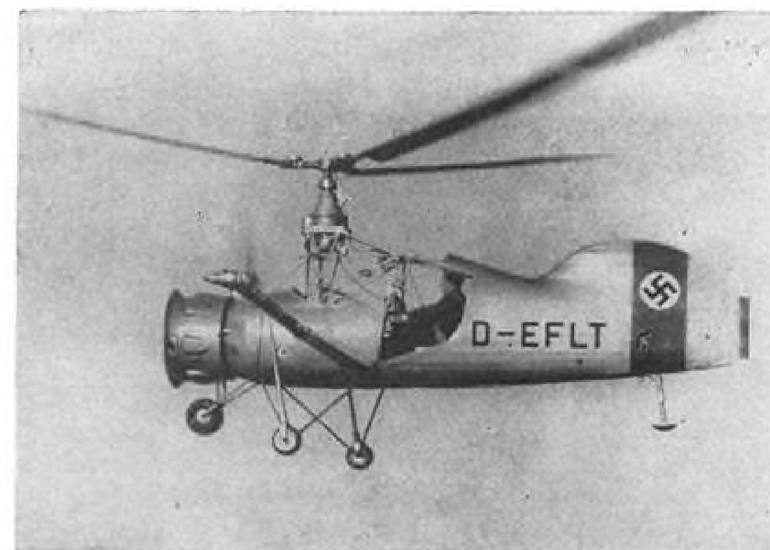
FL-185 HELIGYRO: Two gyro-controlled props automatically counteracted torque and added thrust for forward flight.
