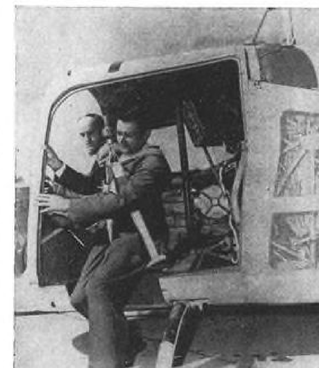
INTERNAL HOIST lifts man into cabin at rate of 90 fpm. Pilot can operate copter and hoist controls from a single console.
