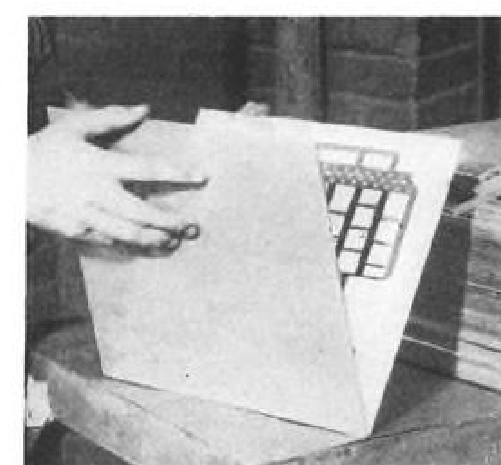
2. 'PRINTED' SHEET and plain sheet make a sandwich for roll bonding operation.
