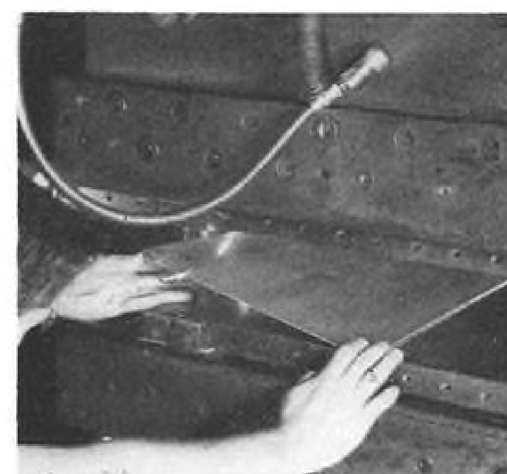
4. NEEDLE has been inserted in left corner of sheet at lead-in of stop-weld pattern.
