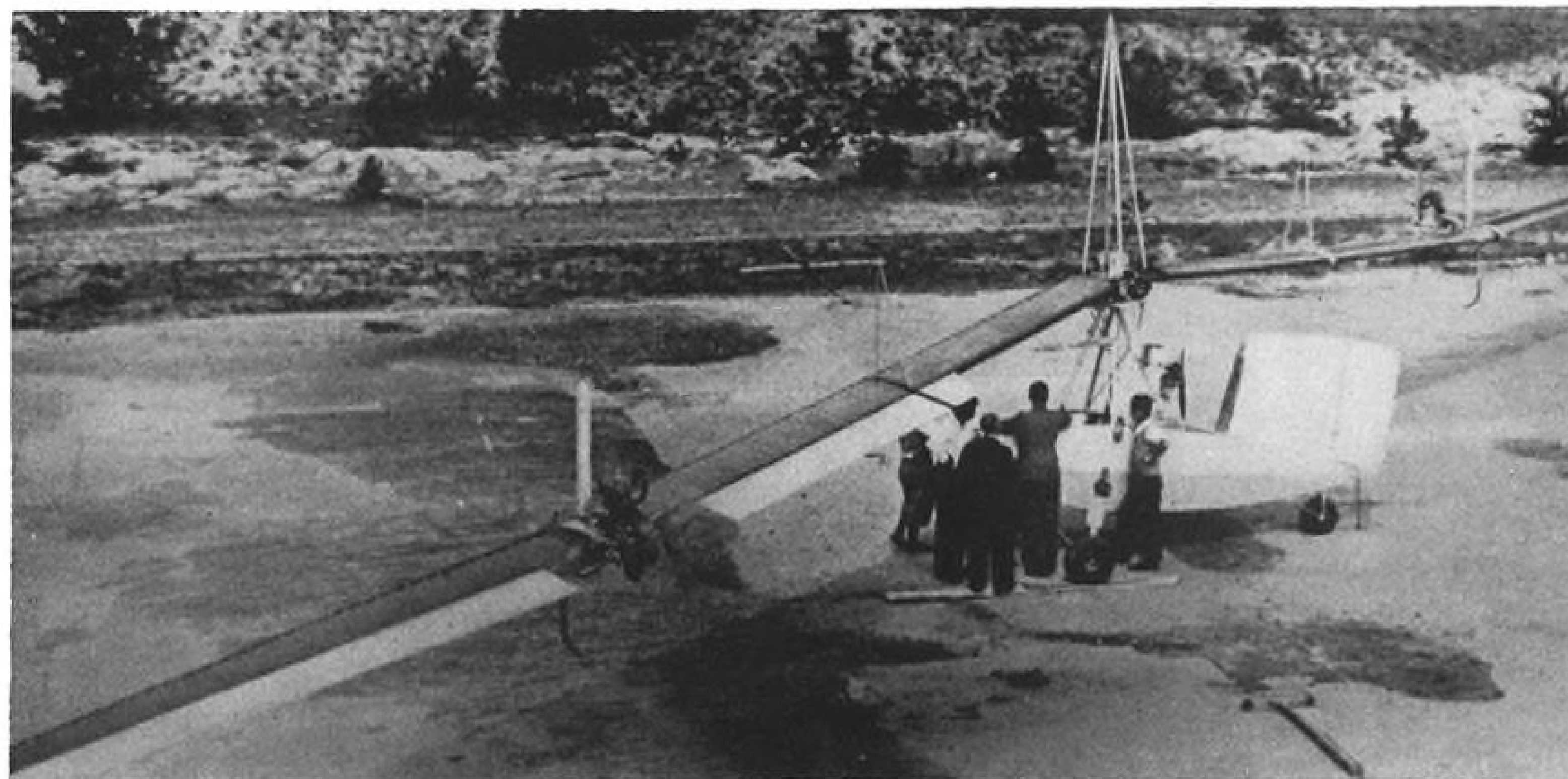
FLETTNER GIANT with 100-ft.-dia. rotors flew tethered in 1933; blades were hinged at root and outboard of engines.
