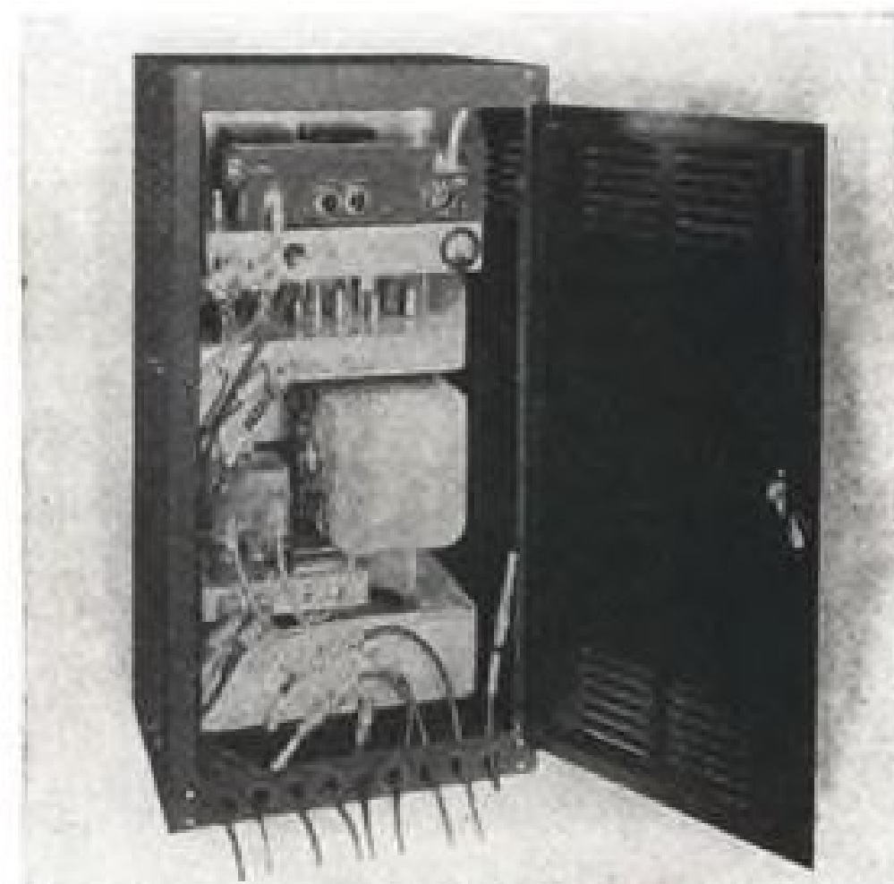
REAR VIEW of aural bearing generator, with door open, shows compact layout.
