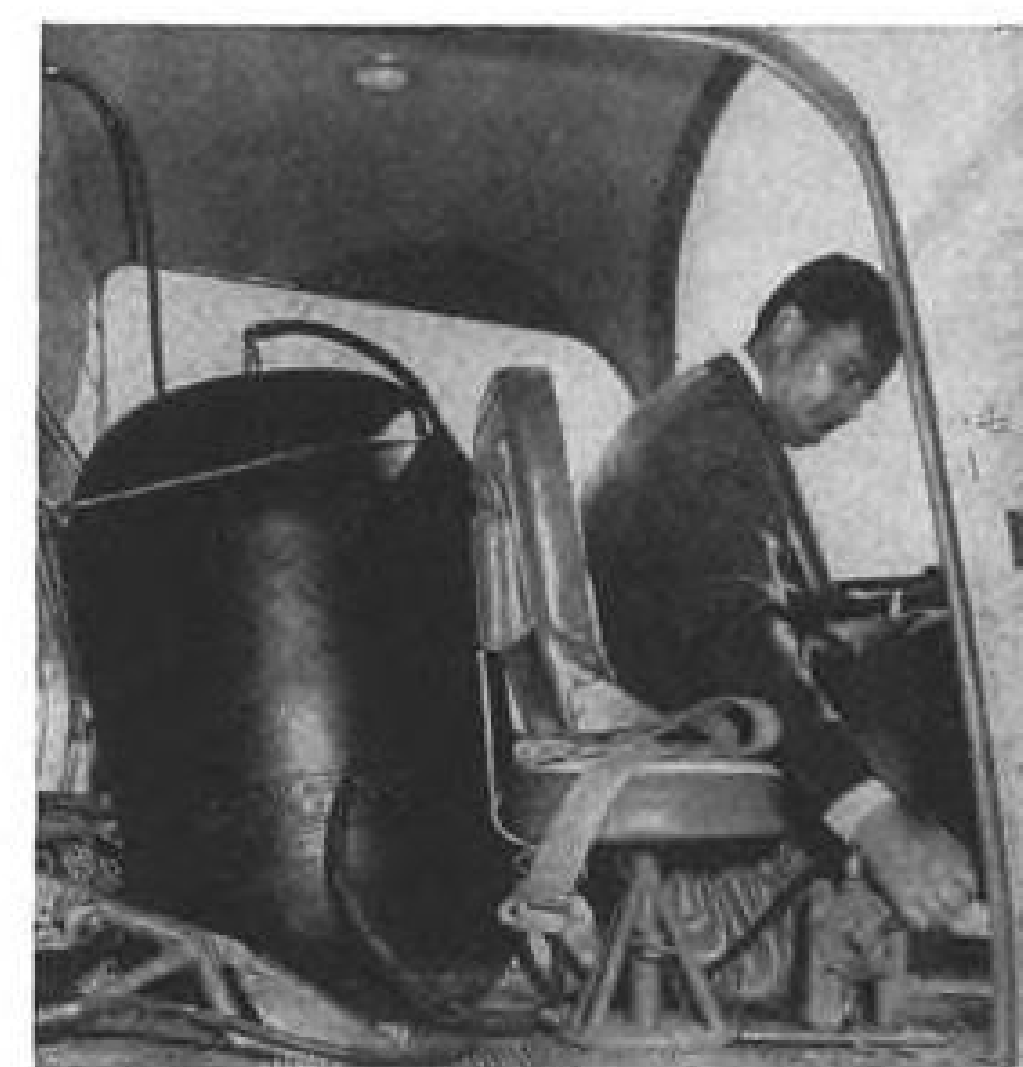
AUXILIARY FUEL CELL is 52-gal. U. S. rubber bag, part of kit that includes wobble pump and quick-disconnect lines.
