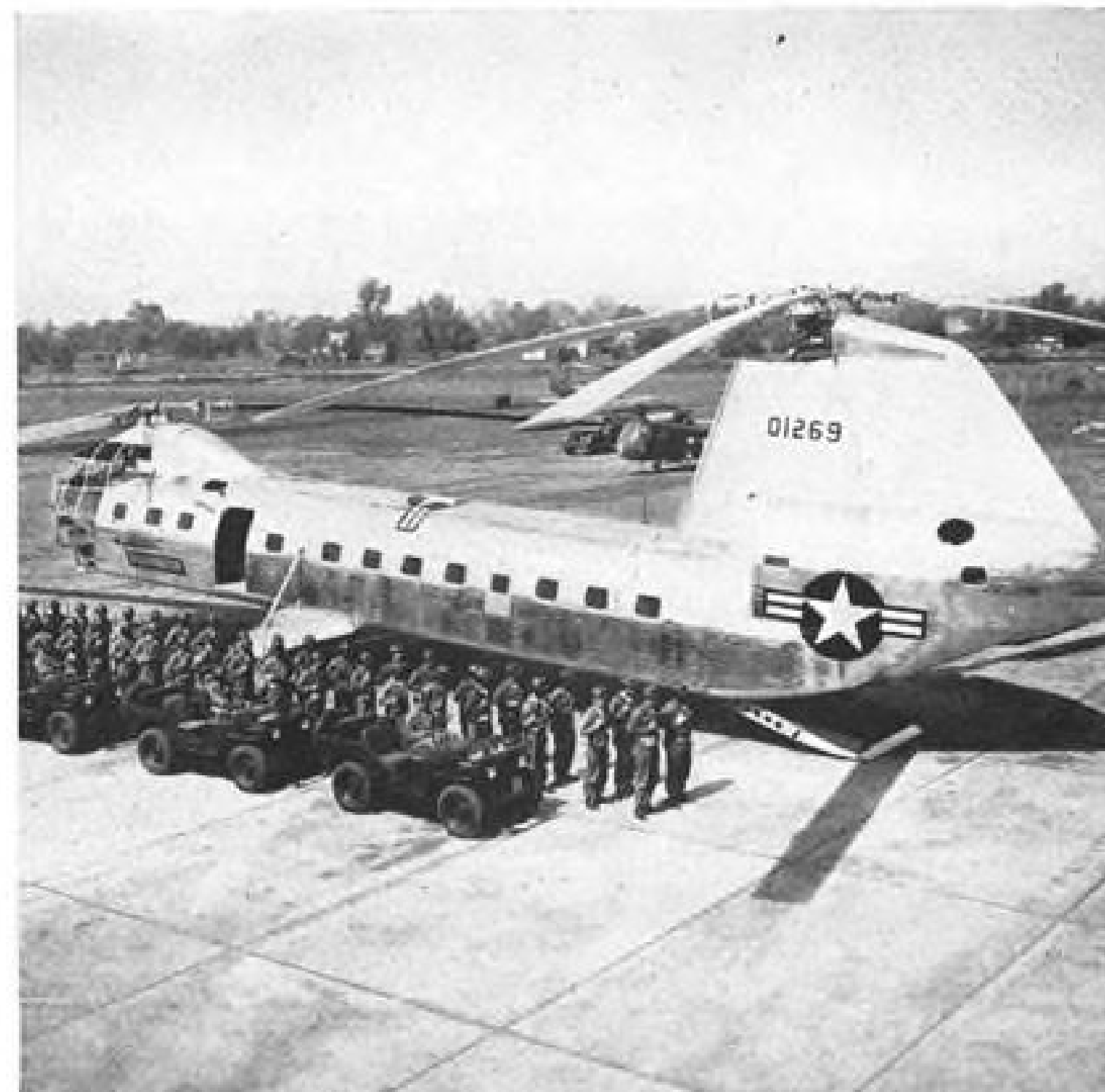
2. WORLD'S LARGEST TRANSPORT HELICOPTER is this twin-engine, tandem-rotor Piasecki H-16, recently unveiled by the U. S. Air Force. It carries 40 troops, 32 litter patients or three jeeps. The H-16 depends on Fenwal Midget THERMOSWITCH units to warn of overheating in transmission gear boxes, and THERMOSWITCH heater controls for cabin combustion heaters.
