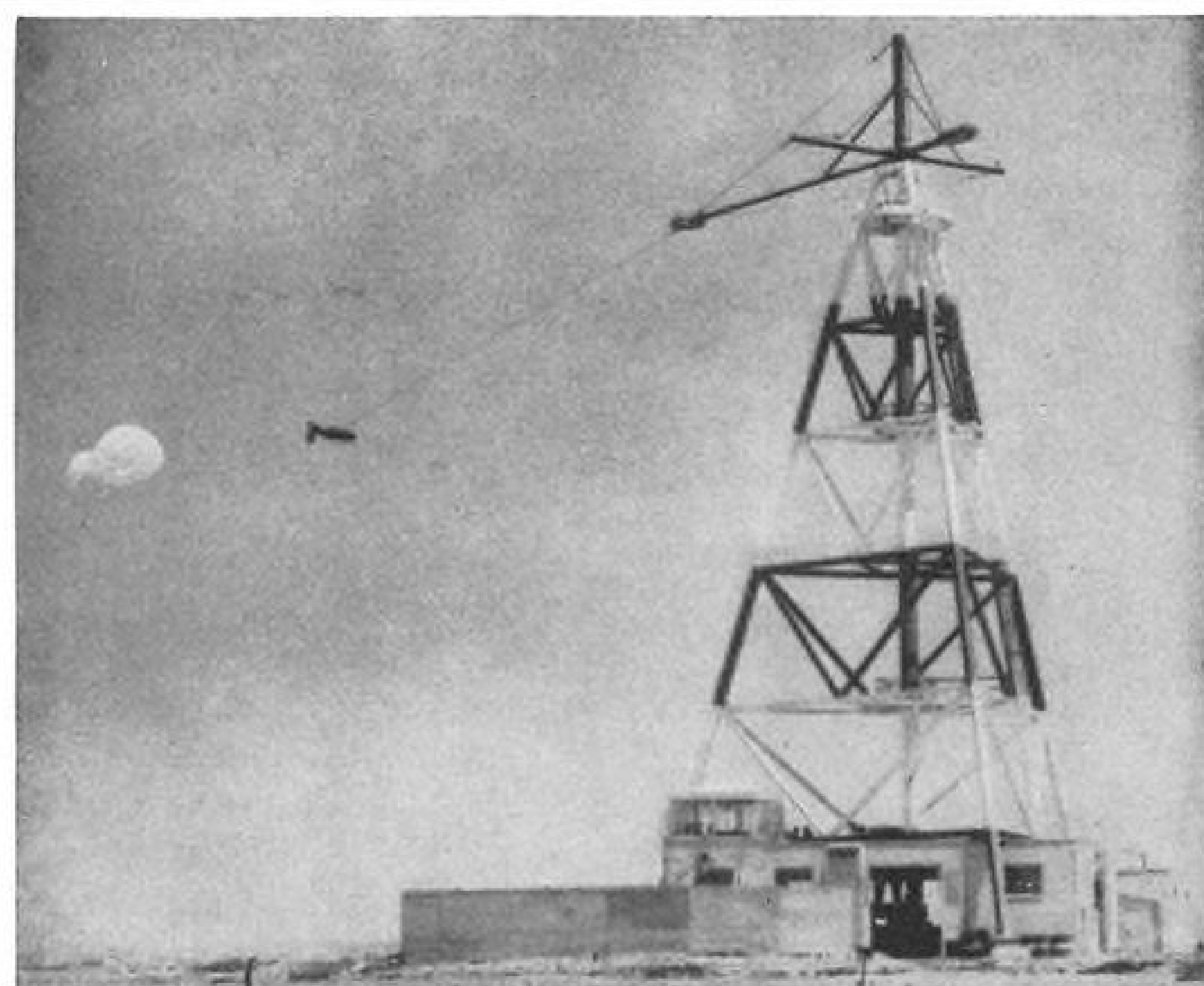
TEST CHUTE is released from gondola whipping around at end of cable.
