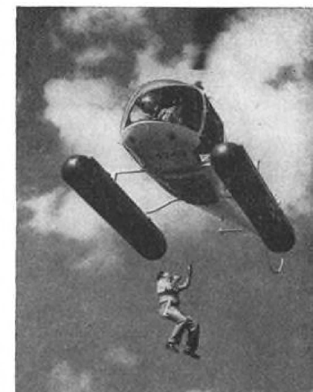
AIR-RESCUE capability is demonstrated by new Bell 47J. Its Navy-type hoist can lift two men simultaneously if necessary.
