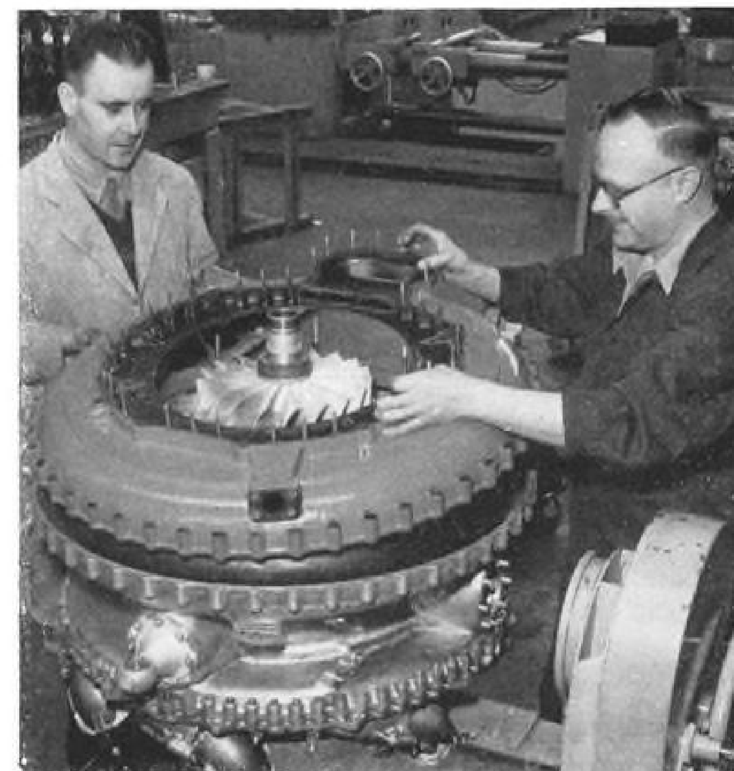
FRONT CASING is shown being fitted to first stage of two-stage centrifugal compressor on Dart engine.
