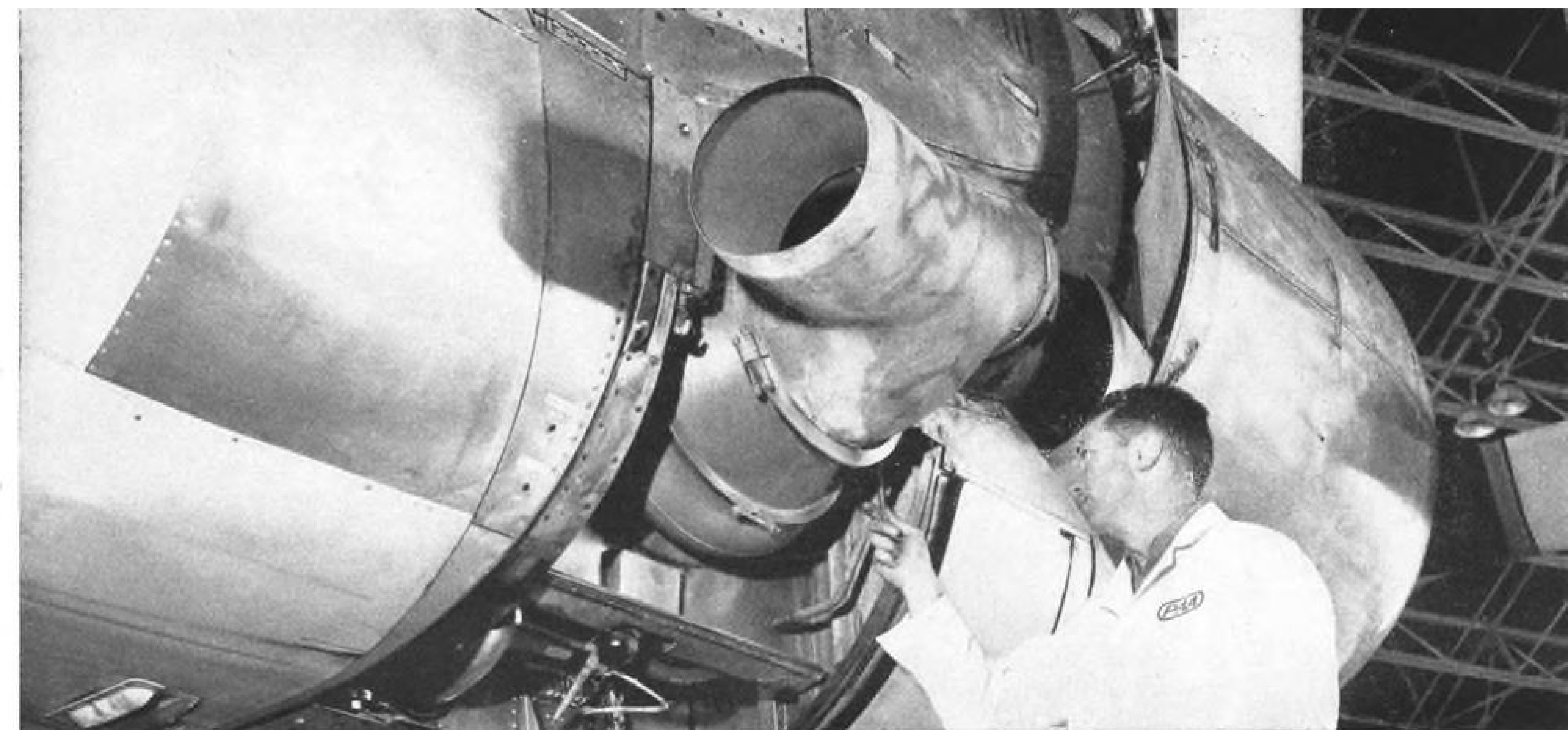
FIRST PAN AM SUPER STRATOCRUISER to use the new G-E turbosupercharger is the "Clipper Mayflower." Improved turbo allows cowl flaps above mechanic's head to be drawn in closer to the engine to reduce drag.
