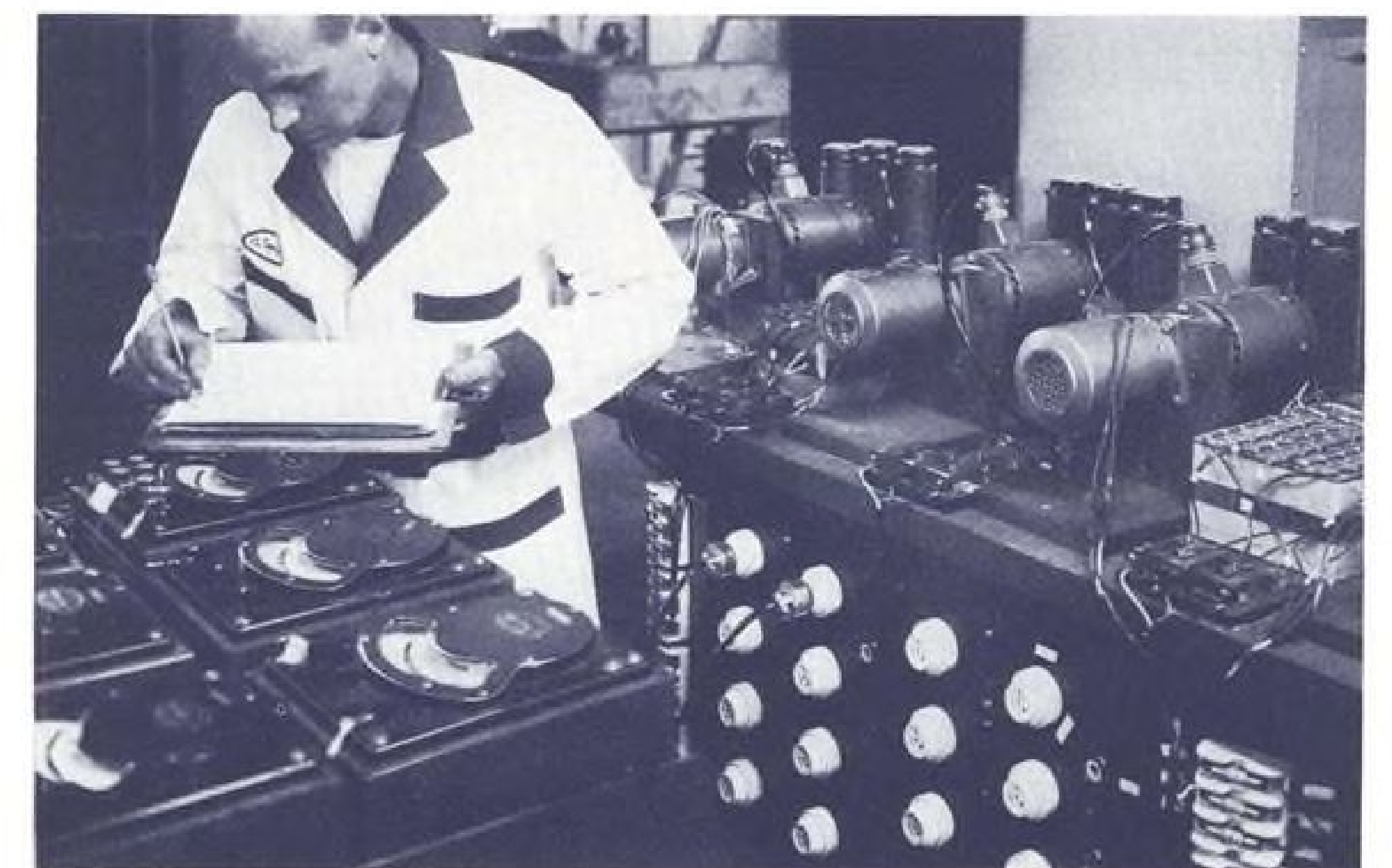
Life testing of all electrical apparatus plays a vital part in the Aircraft Department of the Small Motor Division. Highly specialized facilities—similar to the one shown above—test generators and motors under full load to determine brush life and stamina. The results are then cross-checked with other evaluations, such as high altitude chamber tests. Complete systems and their components can be tried and proved for performance under any climatic or mechanical environment.
