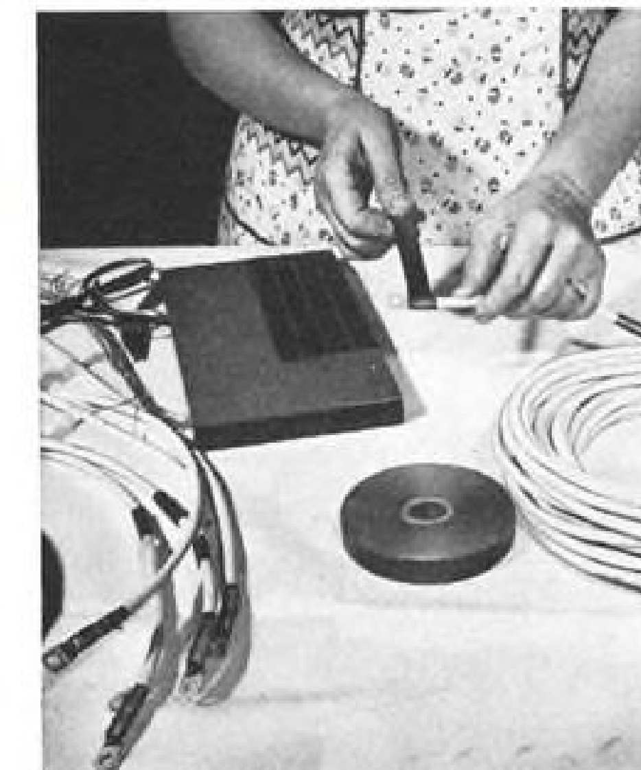
ELECTRICAL TERMINALS insulated with Permacel 30 Heavy Duty Plastic Tape for exceptionally high dielectric strength.
