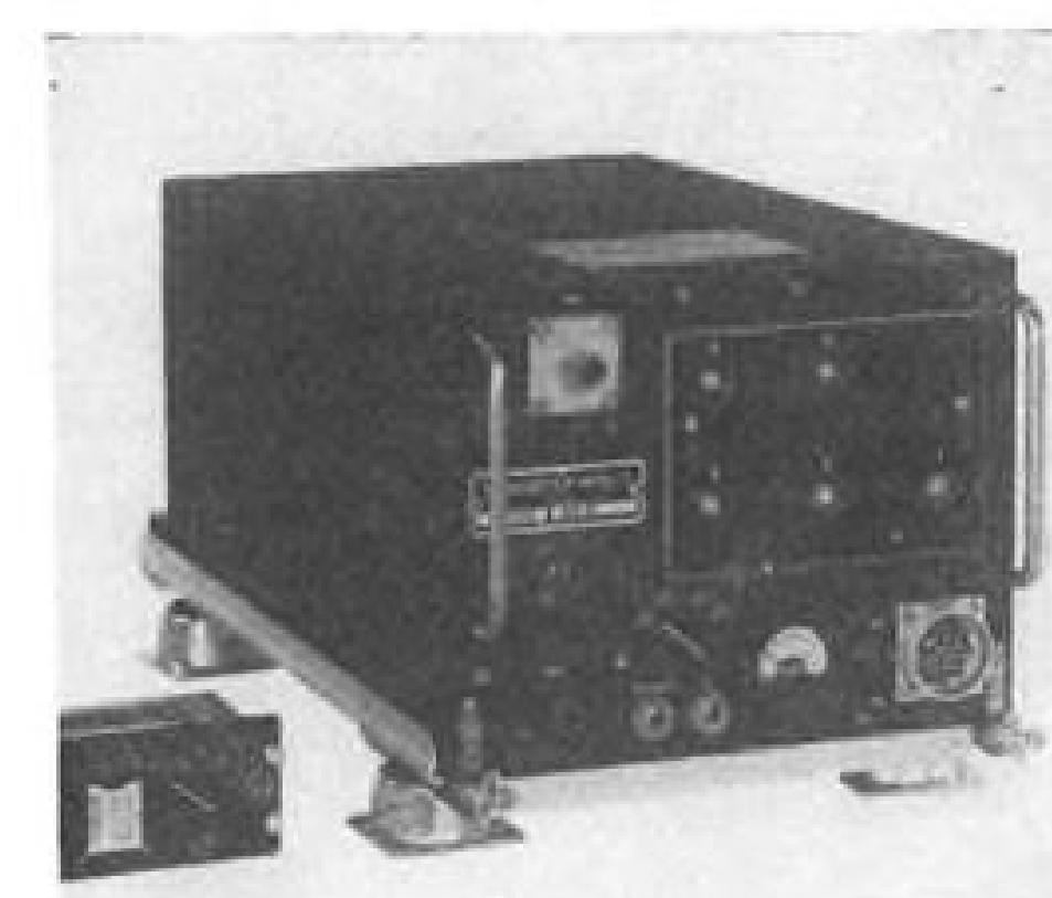
LIGHTPLANE transmitter-receiver weighs 35 lb., provides five pre-set channels.
