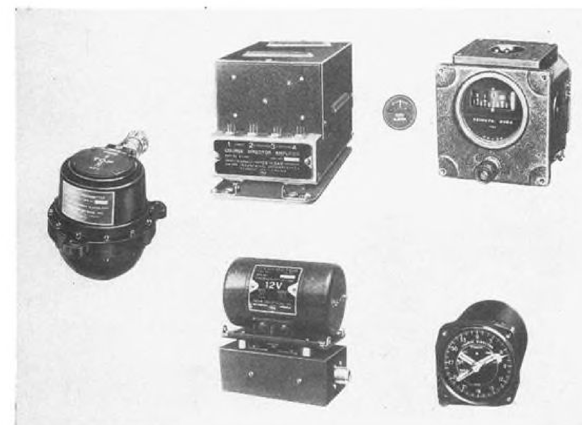
COMPLETE ORION SYSTEM includes remote compass transmitter, course director computer, slaving amplifier and inverter, slaved directional gyro and course and function selector.
