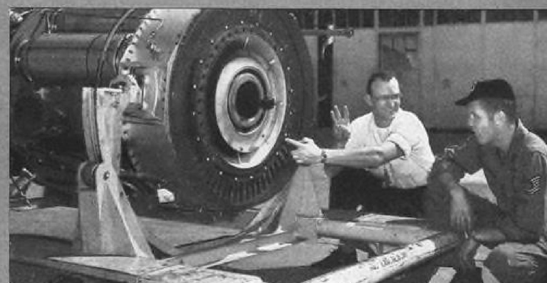
IMPROVED RELIABILITY in the J47-GE-33 engine is illustrated by the new "floating" shim shroud visible above. It reduces the possibility of shroud ring rub on turbine wheel buckets. G-E tech rep is pointing to new adjustable turbine baffle.
