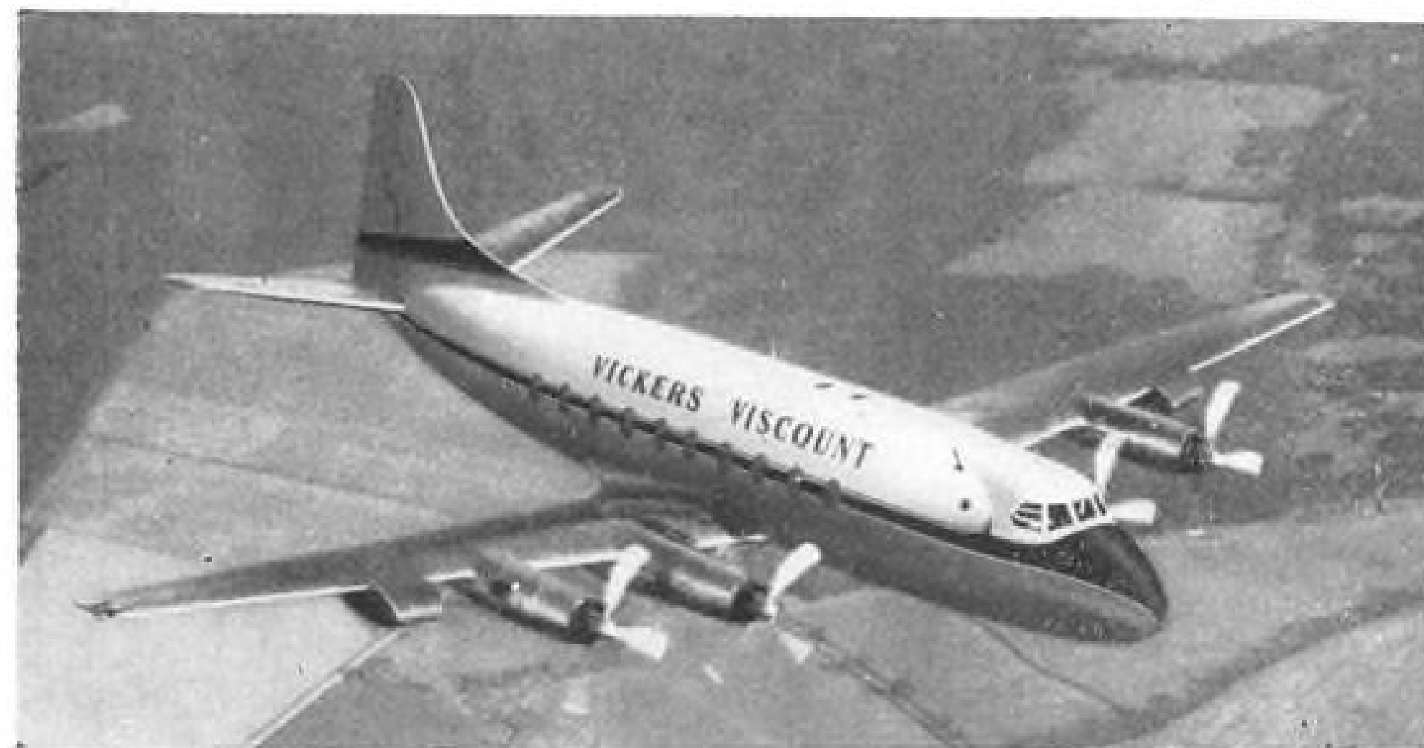
VISCOUNT 700D fitted with Dart 510s and fuel slipper tanks would look like this.
