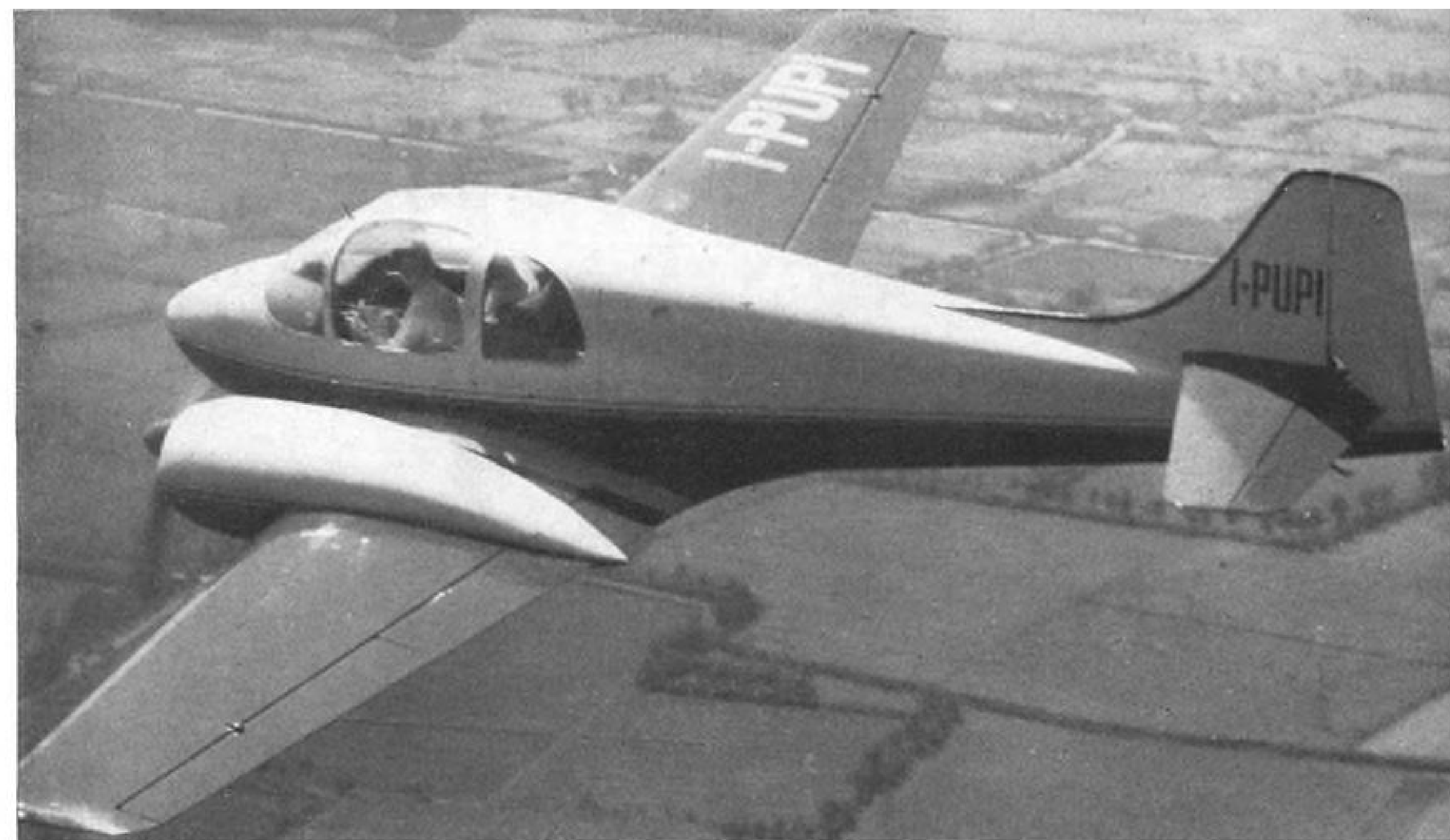
ITALIAN Pasotti F.6 Airone all-wood four-placer is powered by 140-hp. Lycomings. Its speed is about 190 mph.
