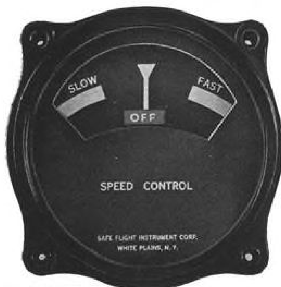
SAFE FLIGHT Speed Control Indicator Plane is being operated at proper speed when pointer is centered. Fail safe flag alarm guards against any malfunctioning.
