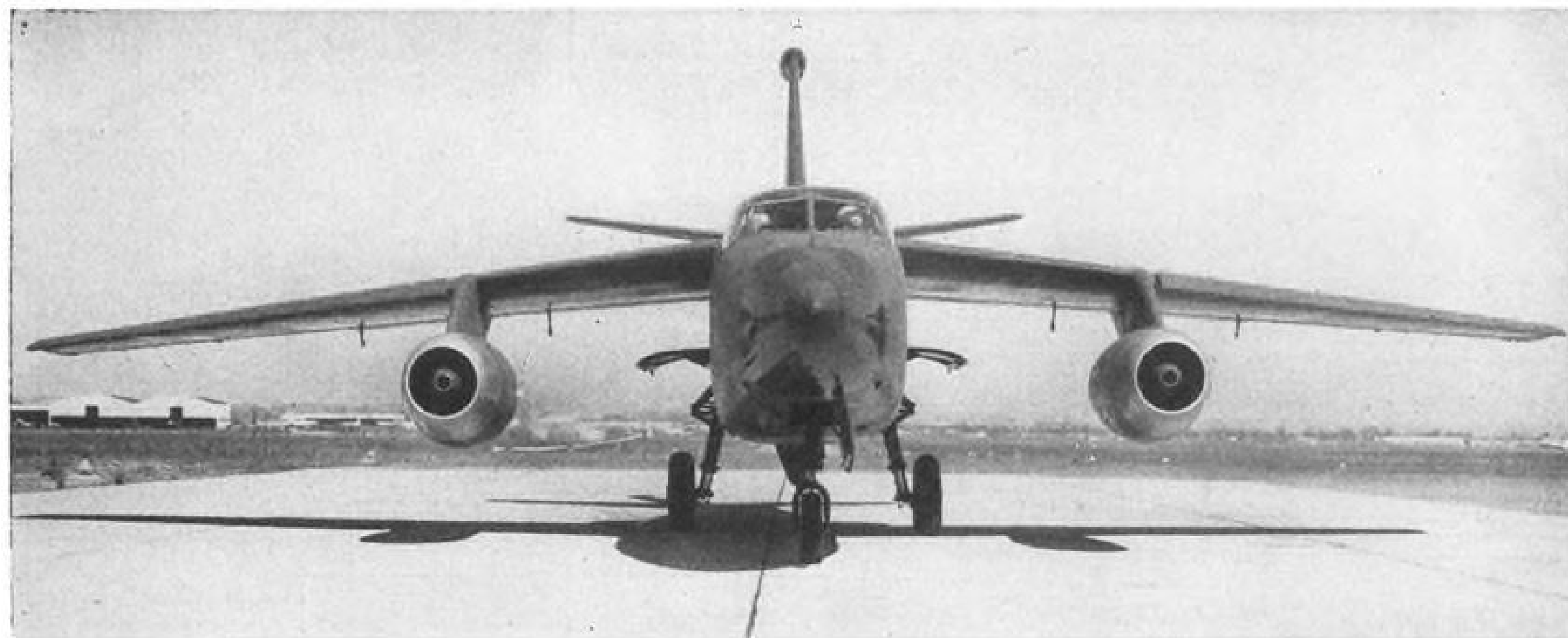
FRONT VIEW OF A3D SKYWARRIOR emphasizes its compactness. Narrow tread of landing gear is noteworthy.
