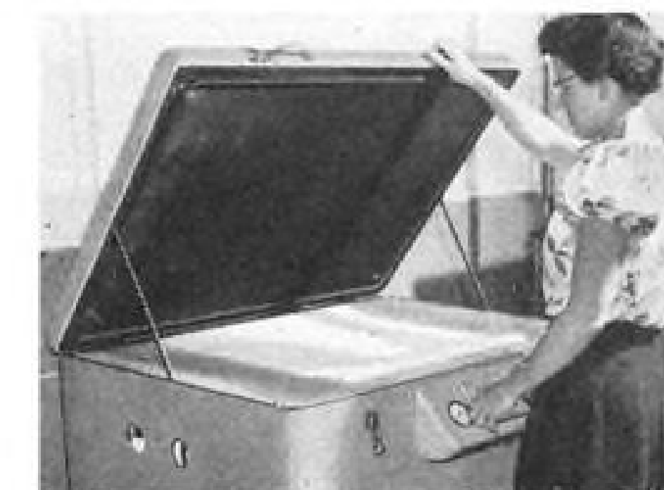
A positive photographic intermediate is produced directly by exposing the "paste-up" in contact with Kodagraph Autopositive Paper, then processing the print in standard photographic solutions. No negative step . . . easy room light operation.
