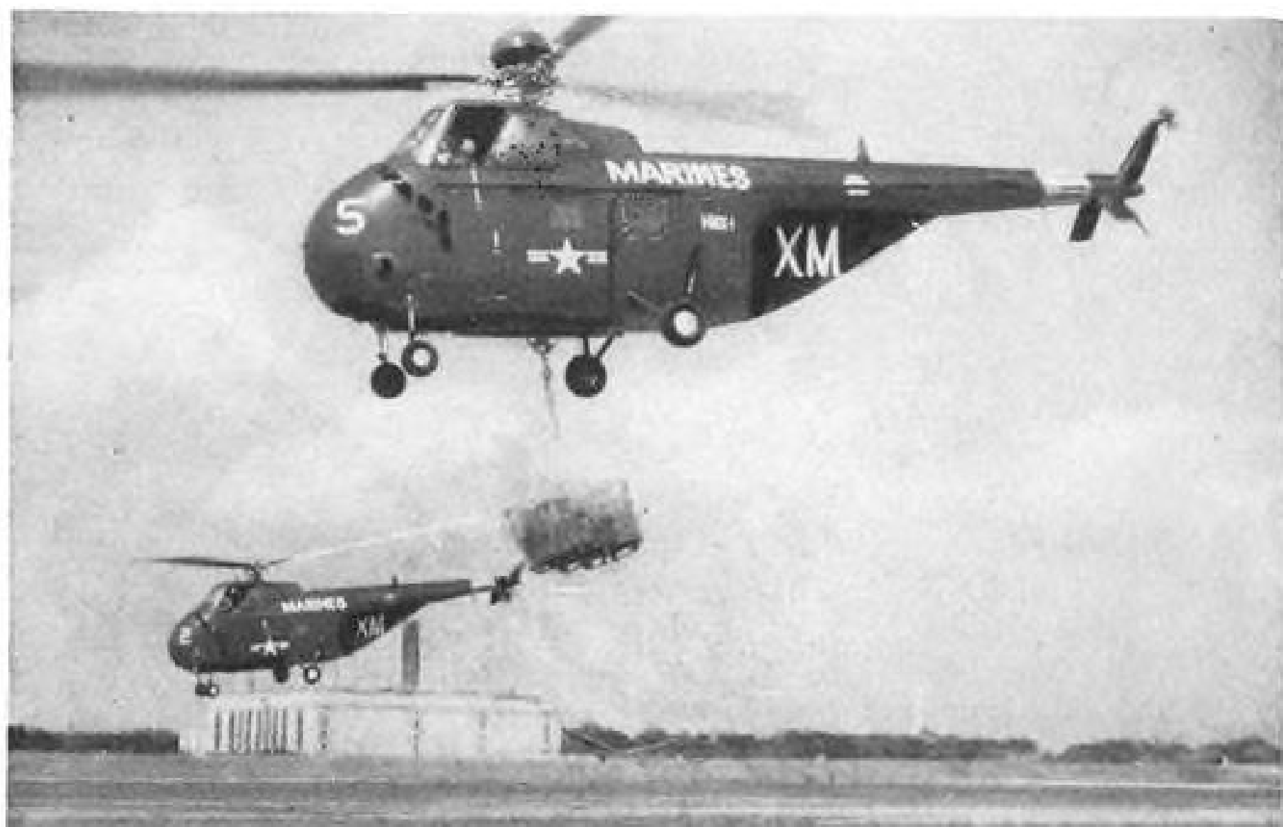
ROCKET MOTORS ON ROTORTIPS of Sikorsky HRS-2 in foreground give extra power, allowing it to match takeoff performance of conventional HRS-2 in background even when carrying 650-lb. additional load in basket slung under the fuselage. Dome above main rotor on nearer copter carries hydrogen-peroxide fuel for Reaction Motors' engines (Aviation Week Sept. 27, p. 17).
