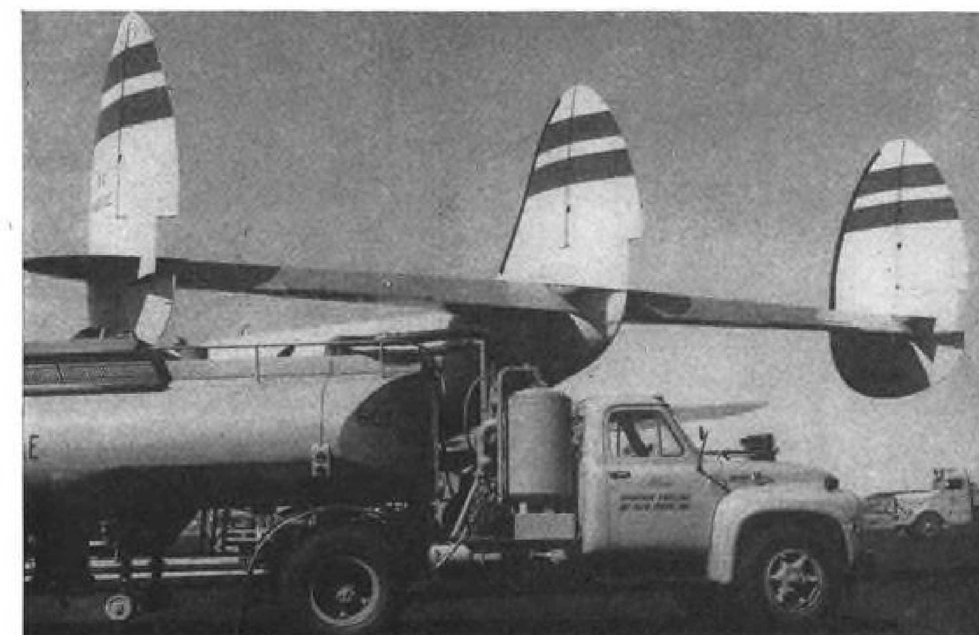
TANK-TYPE filter sits behind cab of $17,000 fueling truck at Idlewild Airport.
