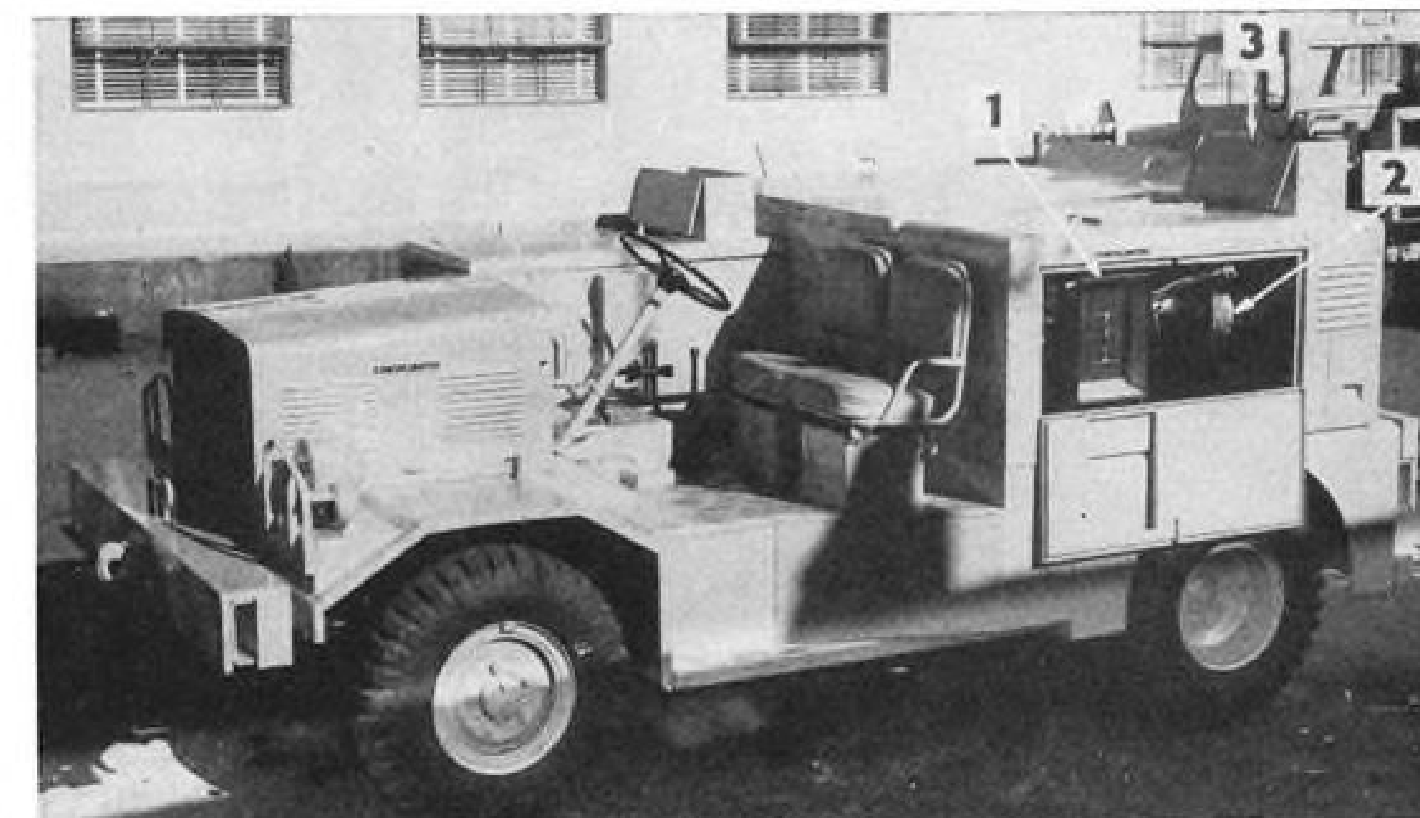
MODEL 3000—(1) Air intake for gas turbine; (2) turbine; (3) turbine exhaust stack.
