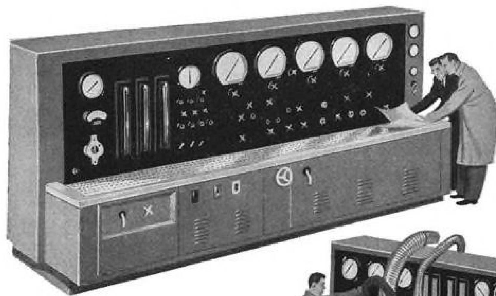
Universal Hydraulic Test Machine for high pressure, high output pumps and accessories. Made in pressures up to 5,000 psi, flows to 100 gpm, with variable speed drives up to 4500 rpm.
