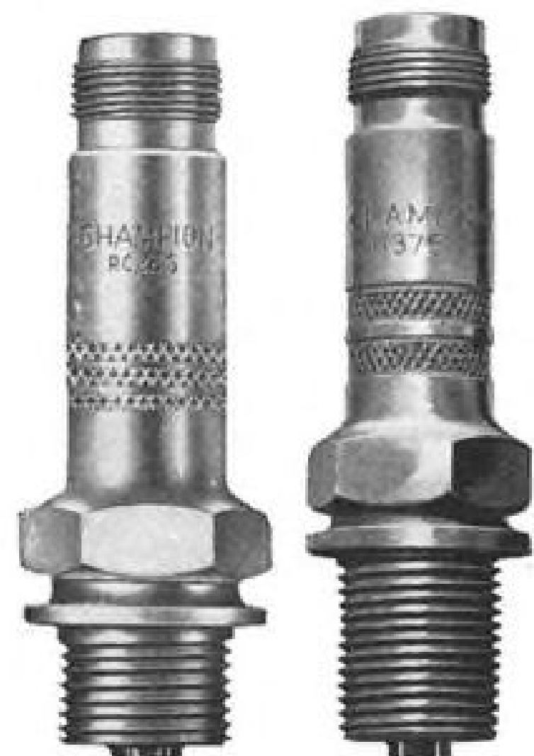
The RC 26S and R 37S-1 are most widely used of Champion's many types of aircraft spark plugs.
