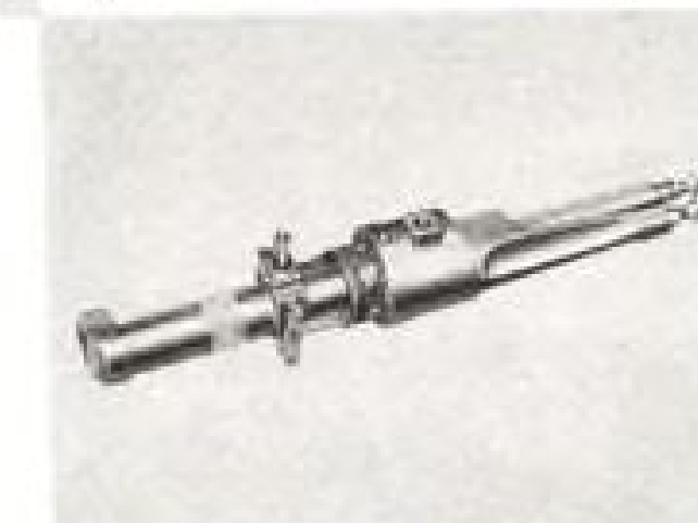
Powerplant Door Cylinder—1000 psi air cylinder 1-1/4" bore x 8-1/2" stroke w/mech. locks at both ends of stroke
