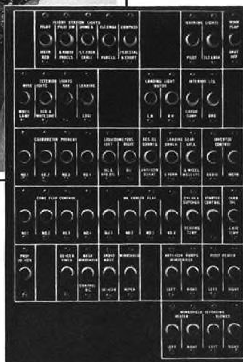
A typical Klixon Circuit Breaker Panel in the Super Constellation.
