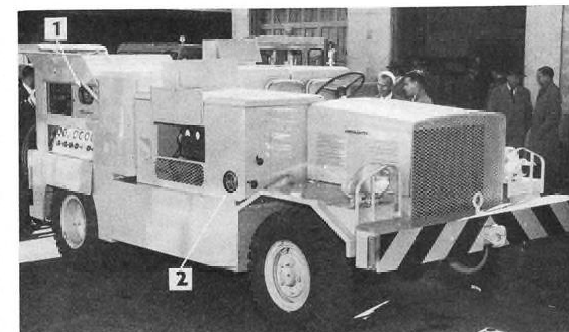
OTHER SIDE—(1) Low-pressure (50 psi.) air outlet; (2) cooling air outlet.
