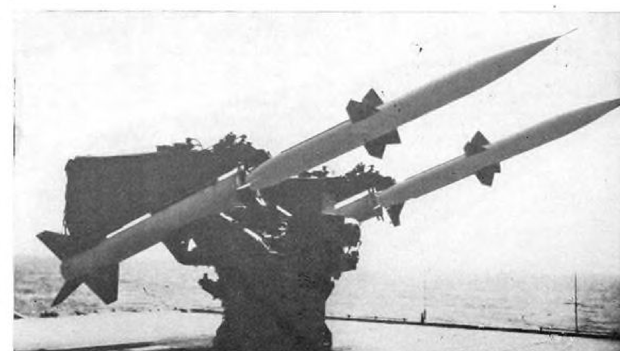
TWIN-MOUNT LAUNCHER is loaded with two Convair Terrier anti-aircraft missiles. In service, loading procedure probably would be automatic for speediest, safest handling.
