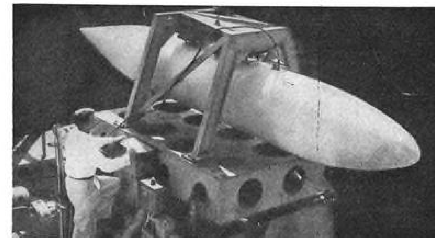
450-GAL. Zenith tank gets slosh-vibration test at Century.
