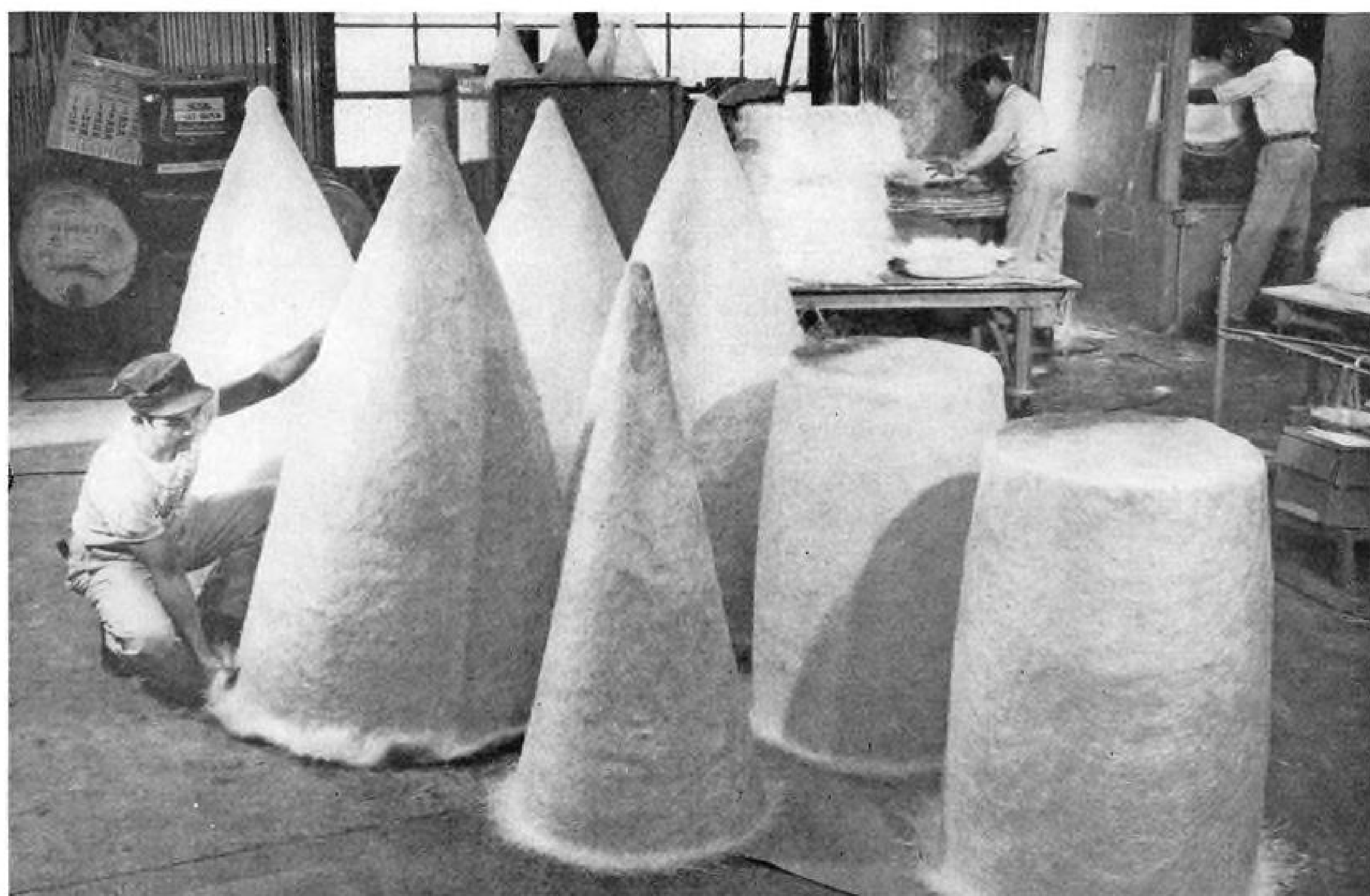
FUEL TANKS IN THE RAW. Fibrous-glass preforms for 450-gal. tanks are prepared at Zenith Plastics. Closed ends on cylindrical portions (right) are later cut out; these portions become center sections of completed tanks. Finished units require no painting or treatment.
