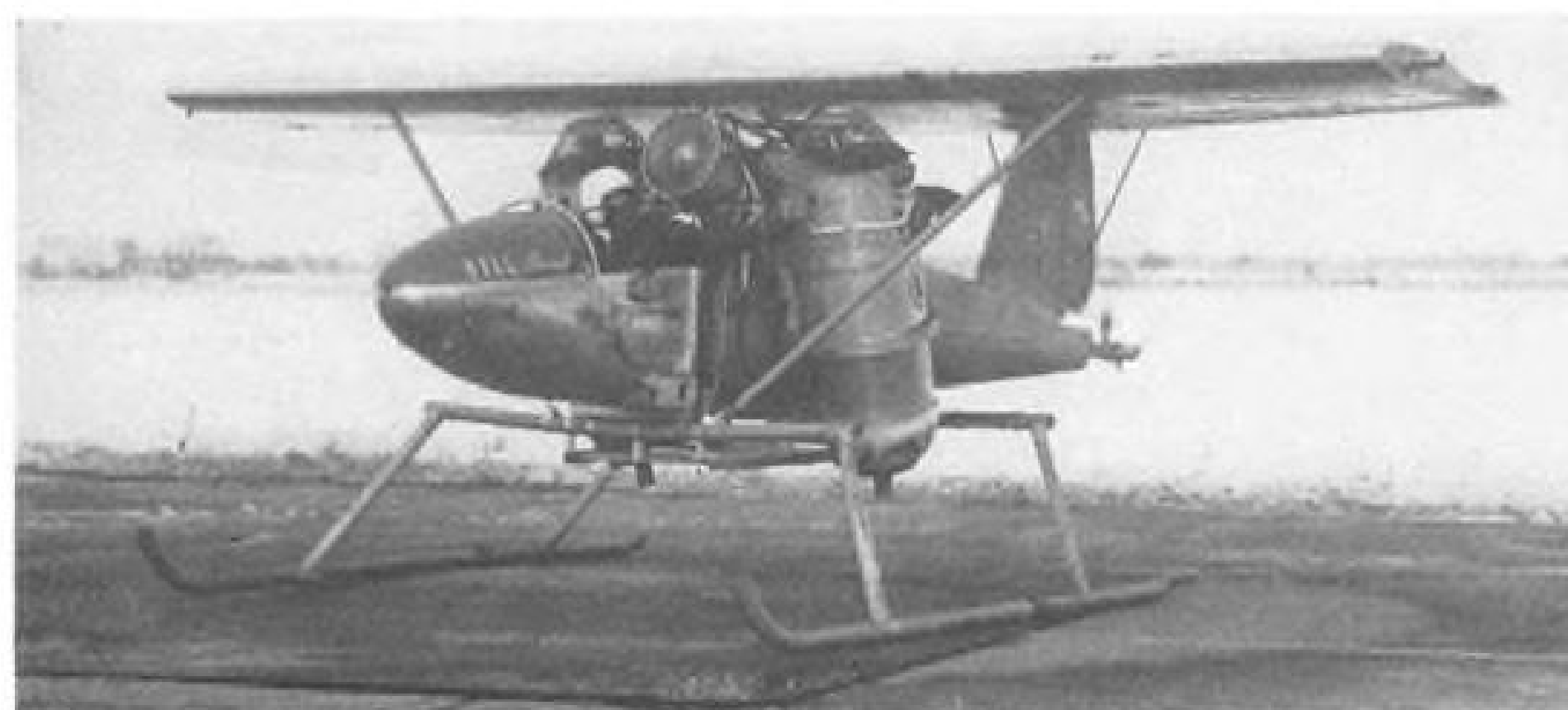
JETS ARE ROTATED from horizontal to vertical position for a straight-up takeoff. Inlet for modified Turbomeca Palouste used for three-axes control is visible just behind cockpit.
