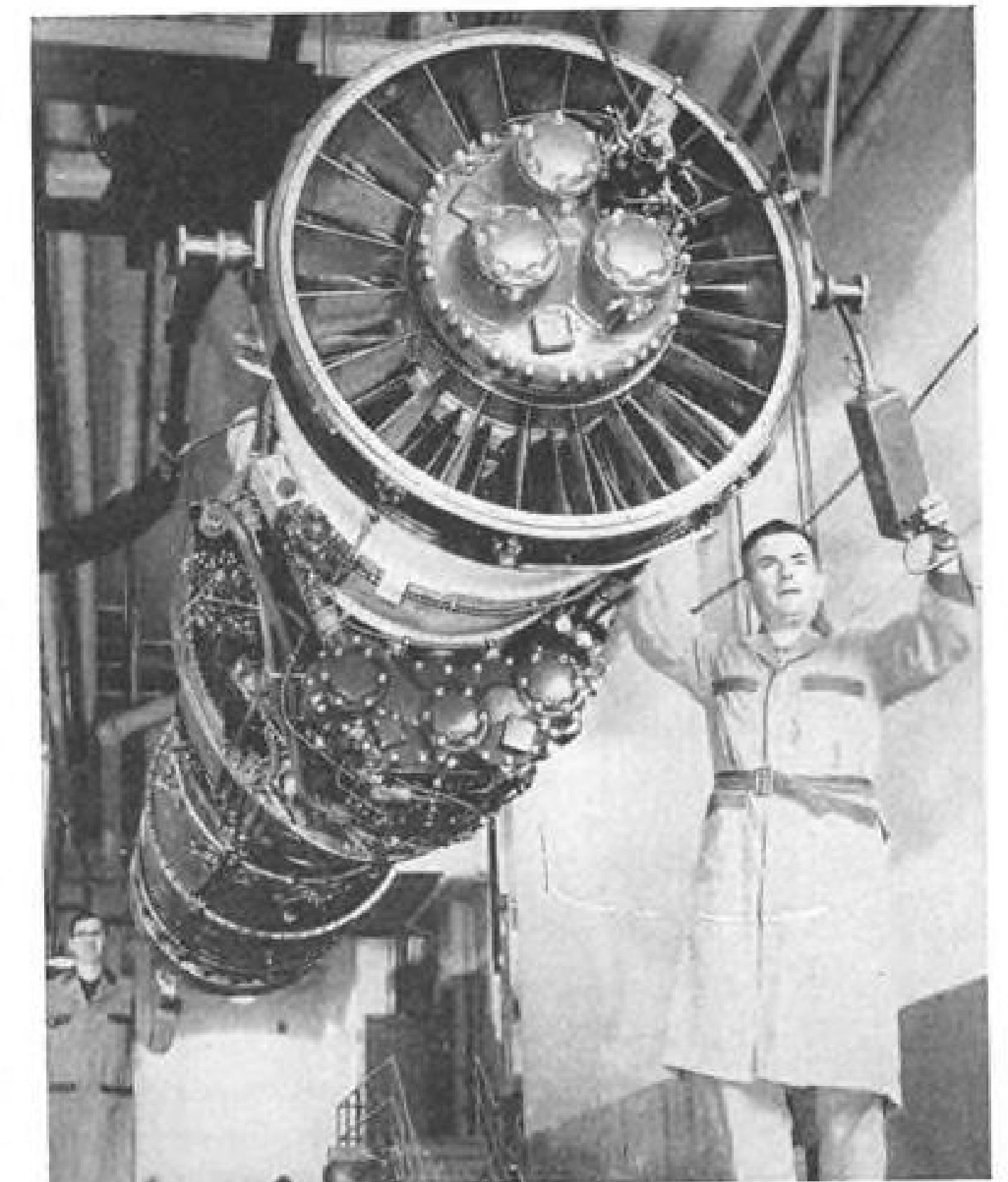
THE MIGHTY J-57 —More than 10,000 pounds of thrust is provided by Pratt & Whitney Aircraft's J-57. After-burners increase this basic thrust tremendously for short periods of operation. The engine offers outstanding fuel economy and high acceleration, vital to fighter operations, in addition to the huge thrust needed for supersonic speed. A year ago Pratt & Whitney Aircraft's J-57 was the basis for the Collier Trophy award.
