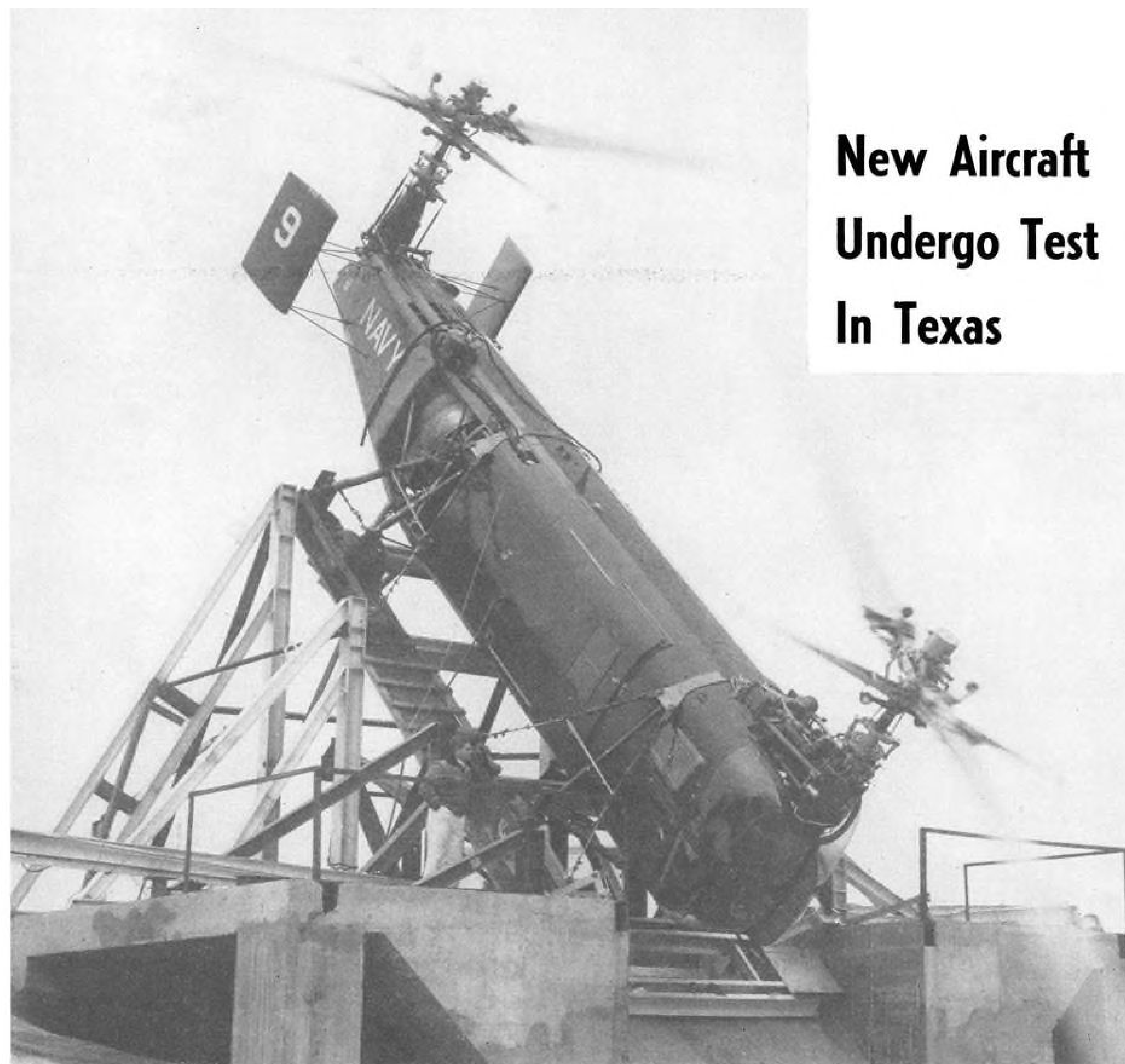
ARMAMENT-TOW ATTITUDE TESTS conducted by Bell Aircraft Corp., Ft. Worth, on its big tandem-rotor HSL-1 involve tilting the anti-sub copter to 45-deg. nosedown in the special rig to gather simulated flight data. Details of these trials are in classified category.
