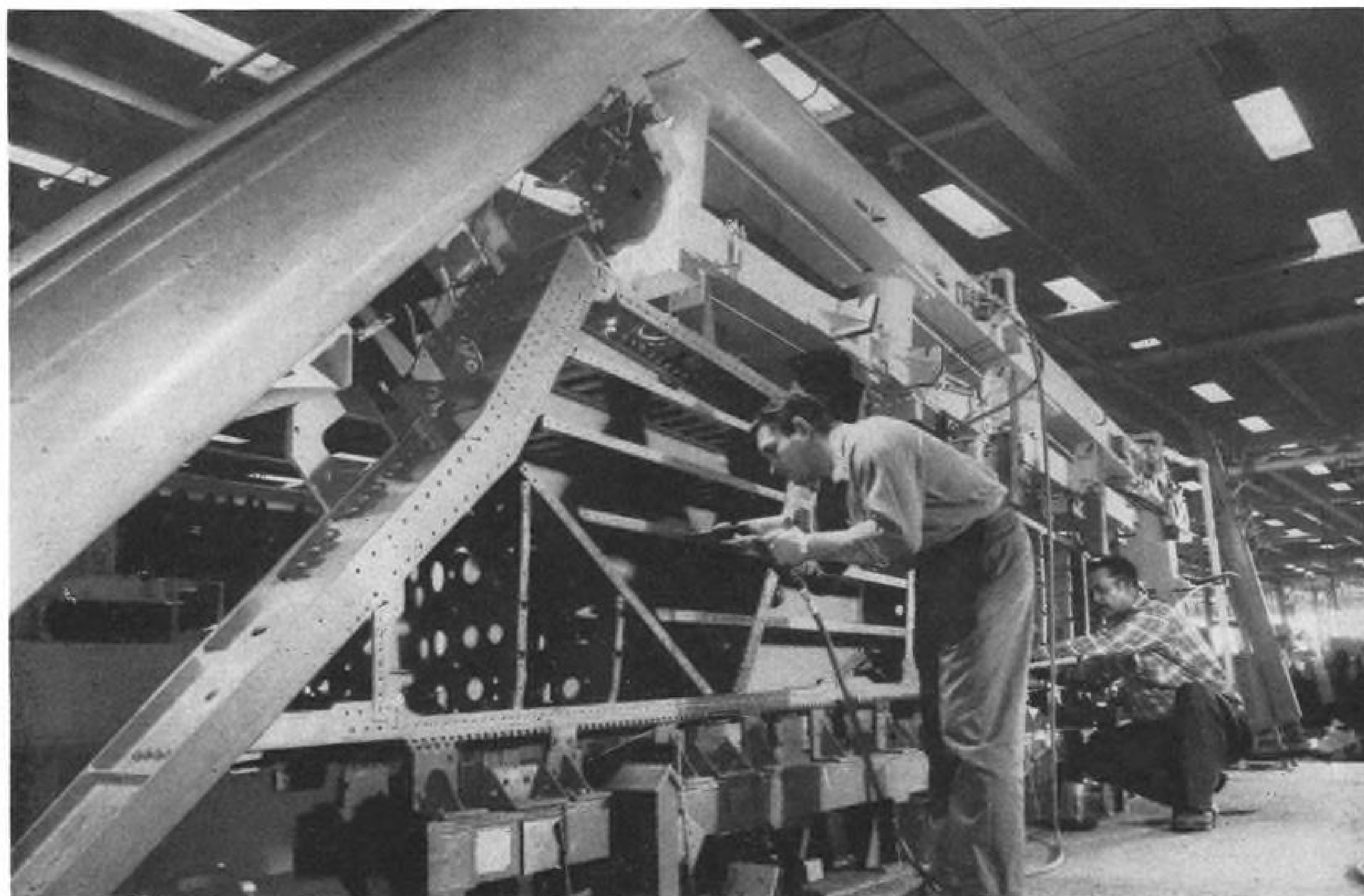
F-100 WING STRUCTURE reveals large forged root rib, leading edge spar with piano hinge, and rugged intermediate members.
