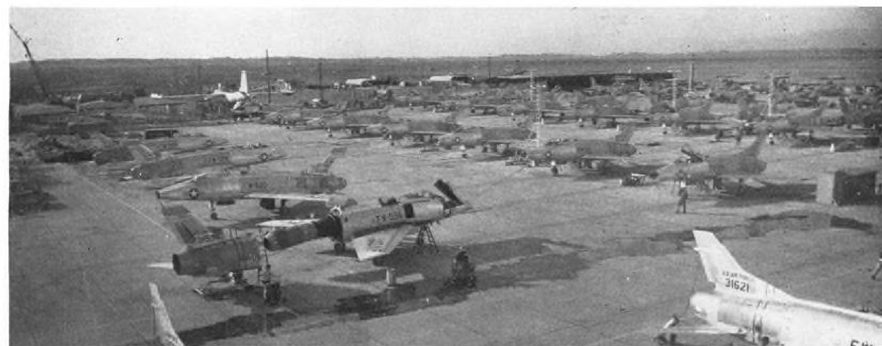
ROLLOUT AREA is spotted with the fighters getting final adjustments. Plane in left foreground has fuselage split at breakpoint.
