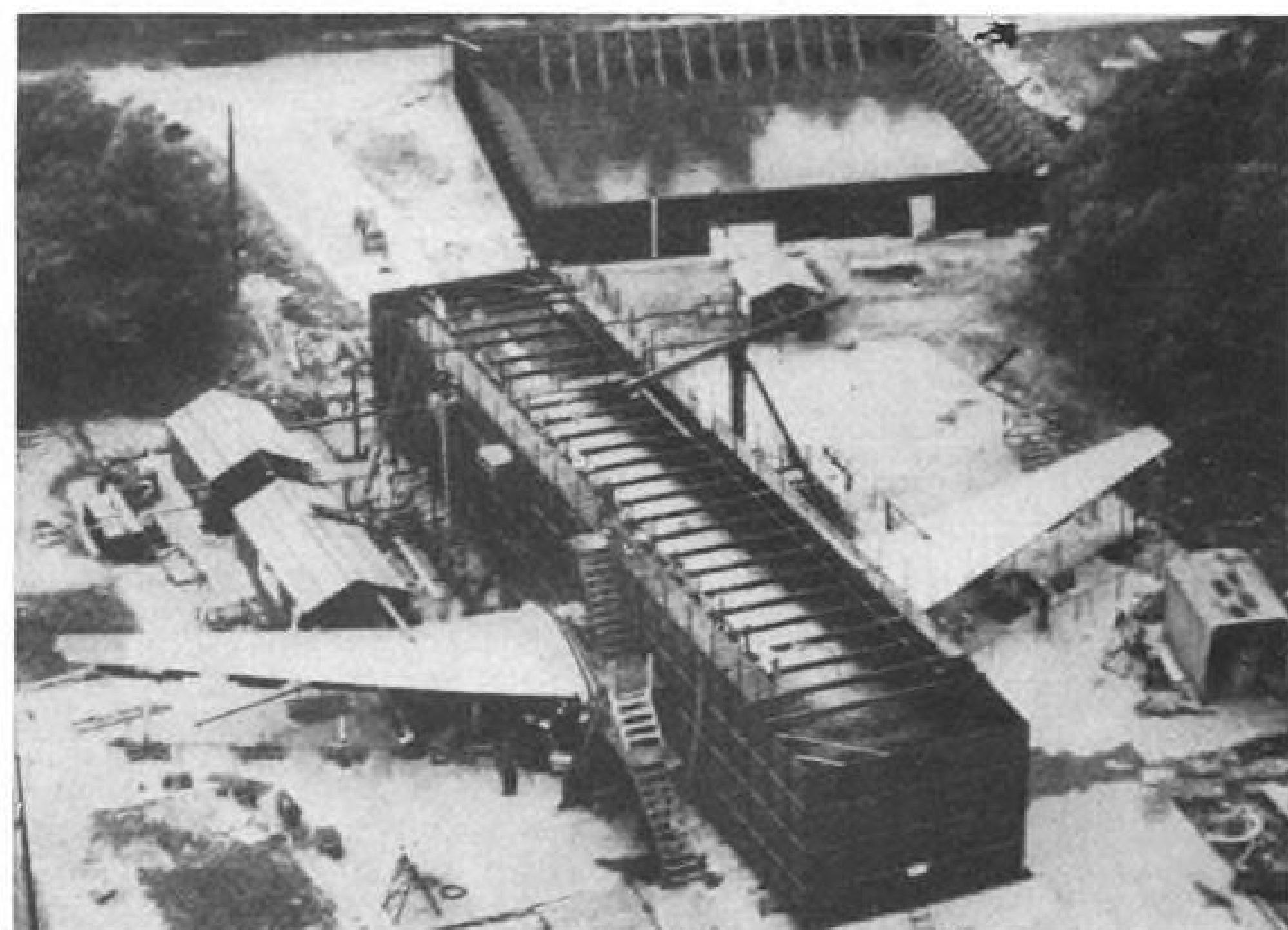
TANK TEST was one phase of intensive investigation at RAE Farnborough. Complete Comet fuselage was submerged; protruding wings were loaded to simulate flight plan.
