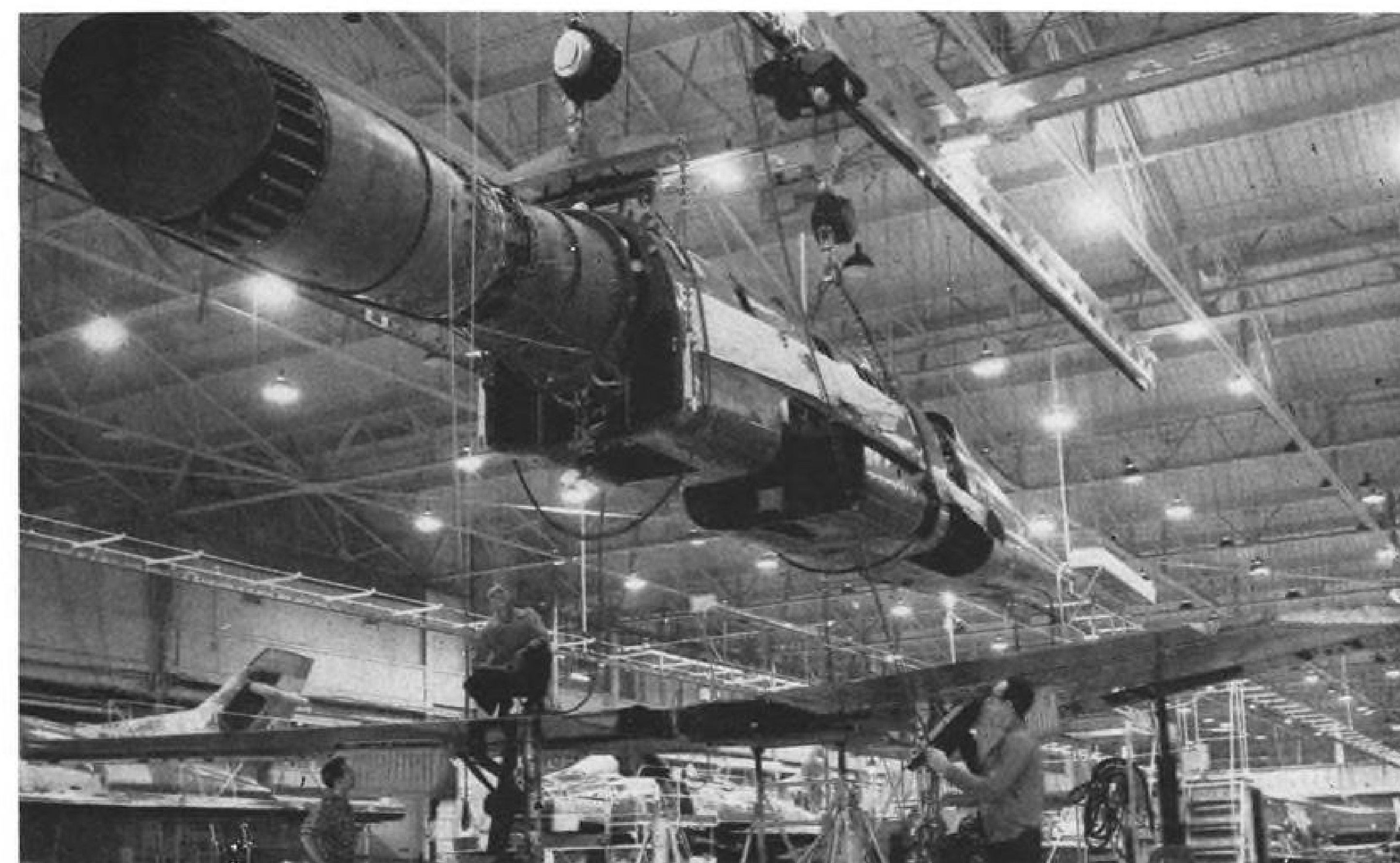
AFTERBURNER-FITTED J57 JET extends from fuselage as it is lowered over wing of the Super Sabre in major assembly job.
