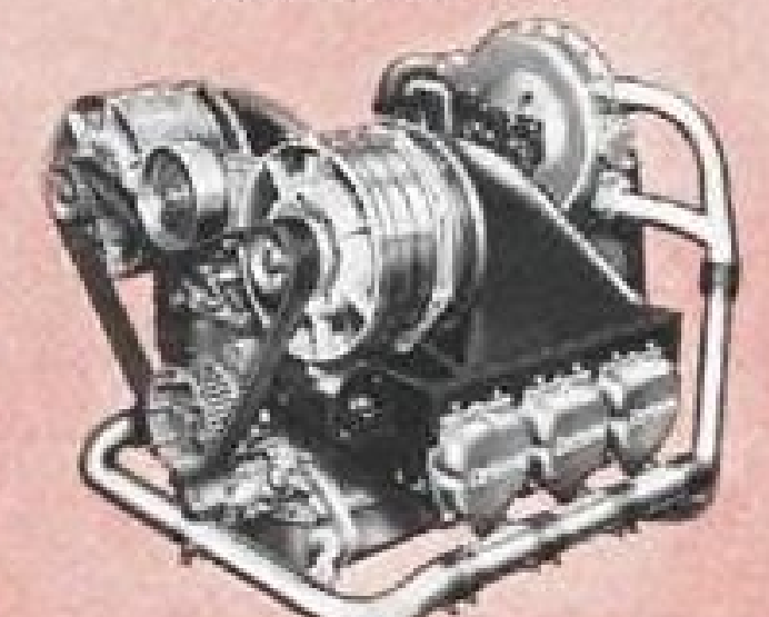
CMC MODEL F50470 SUPERCHARGED AND FAN-COOLED HELICOPTER ENGINE— 260 H.P.
