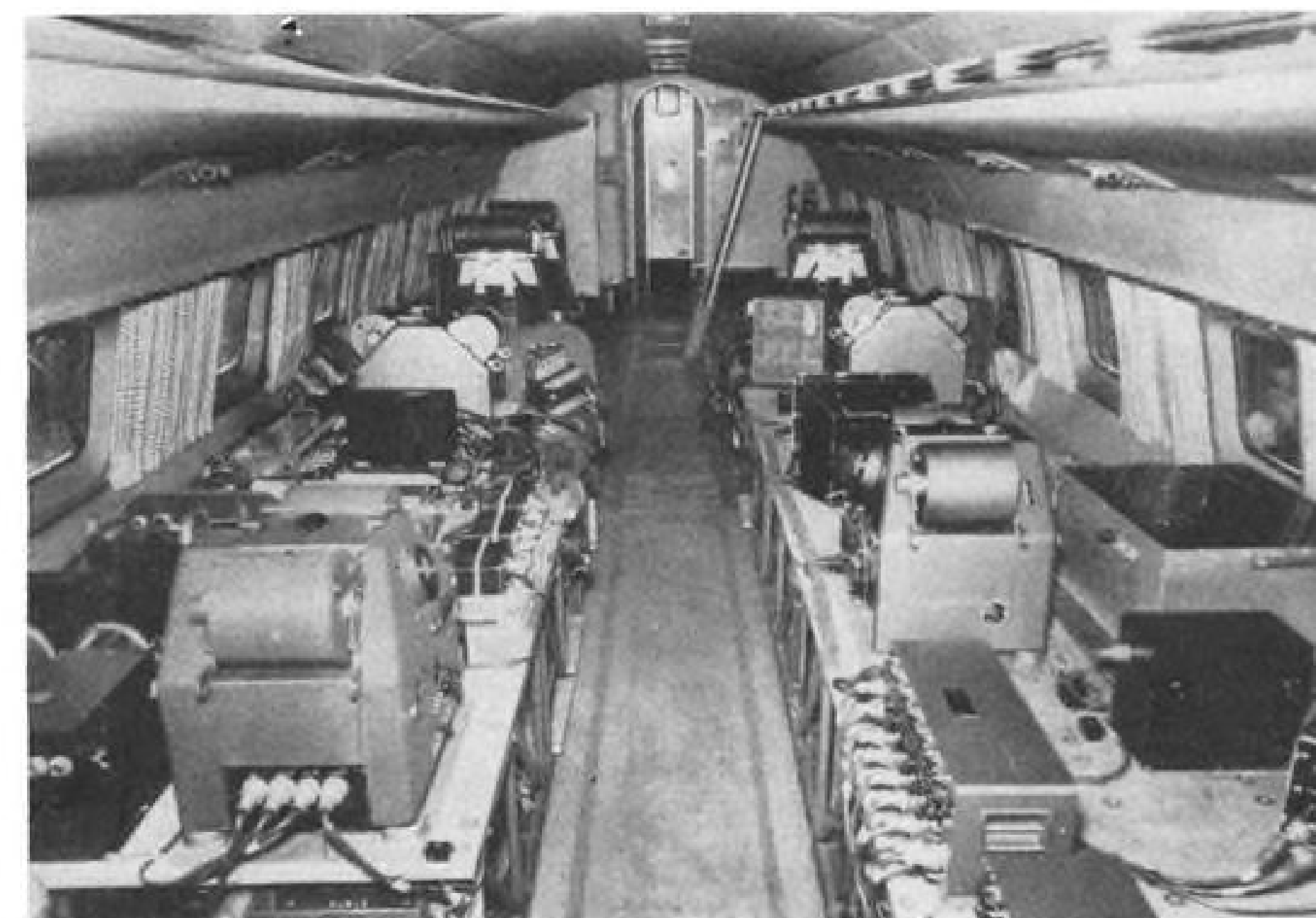
INTERIOR of Comet G-ALAV shows some of the 100-plus special flight-test instruments.
