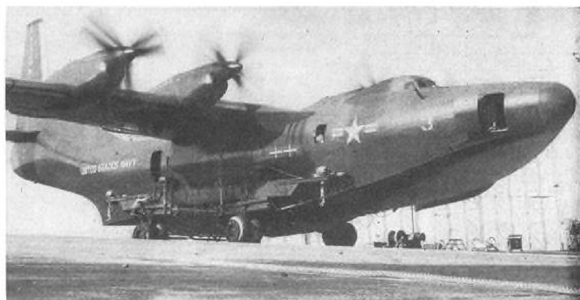
ON BEACHING CRADLE, Convair R3Y-1 Tradewind taxis down ramp under own power.
