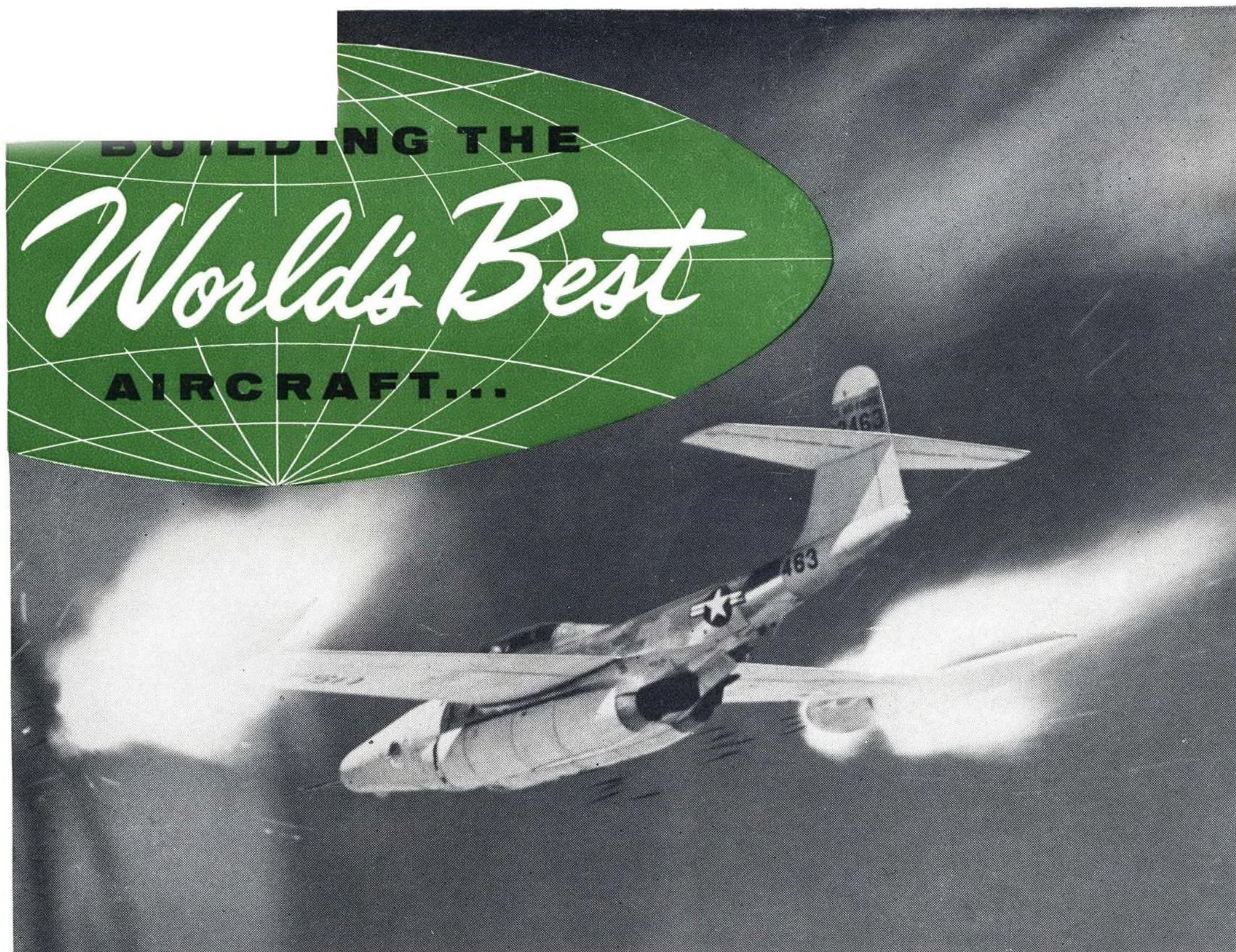
U.S. Air Force's New F-89D all-weather interceptor is powered by two Allison-built J-35 jet engines
