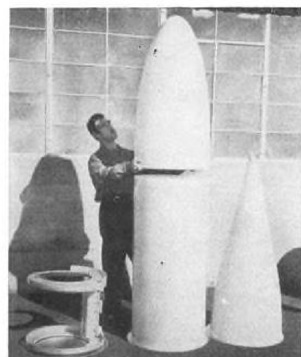
COMPONENTS of three-piece glass-plastic tank at variable capacity.
