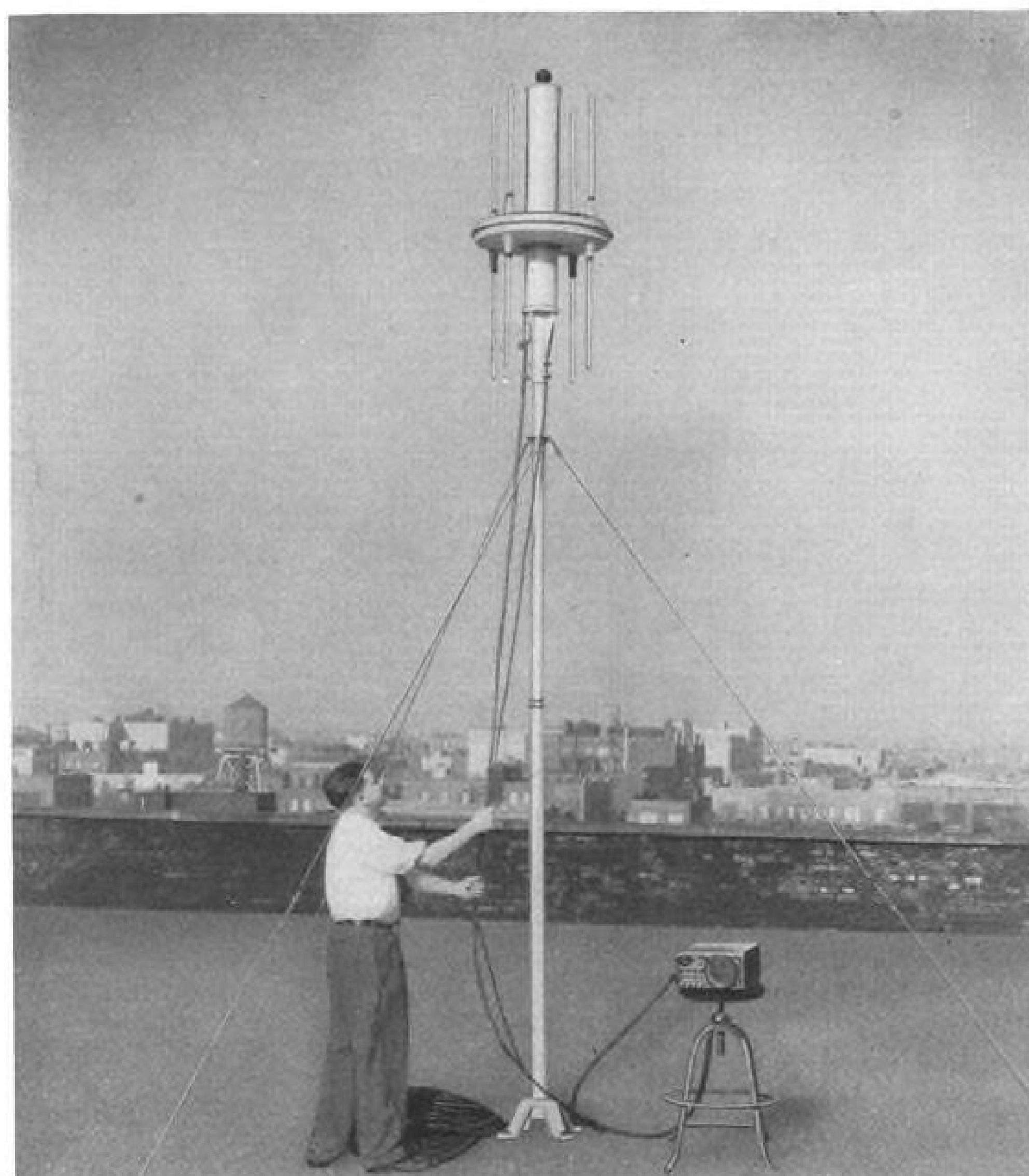
LOW-COST VHF direction finder for small airports consists of antenna (l.) and indicator (r.).
