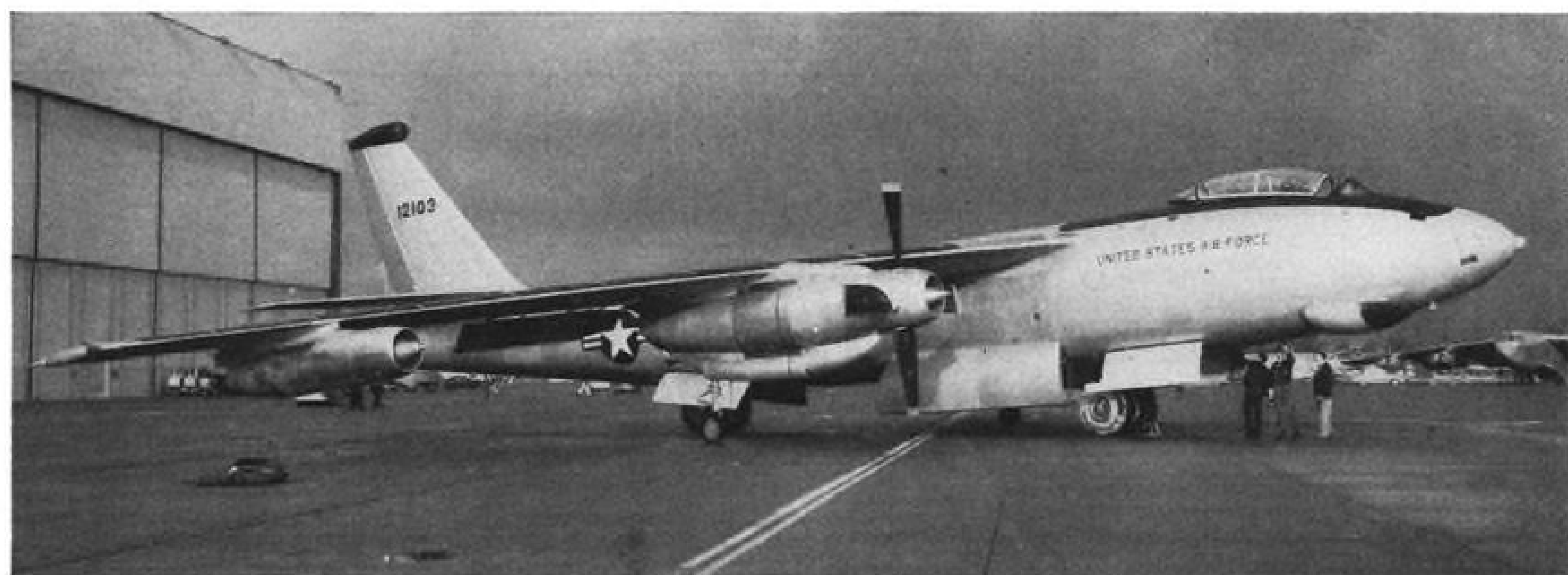
GROUND CLEARANCE was installation problem; nacelles replaced twin-jet pods, were mounted flush with wing undersurface.
