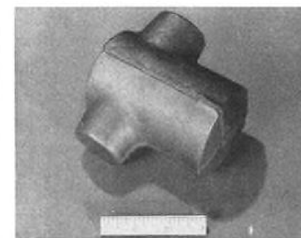
SMOOTH PORTION (front) of steel forging cap material shows fine Chem-Mill finish.
