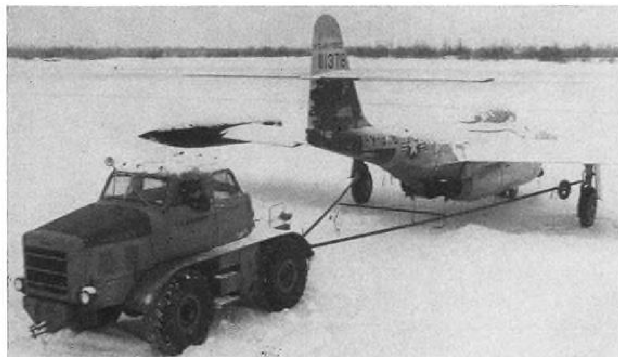
TOW BAR is used to move F-89D tail-first. Nose-first towing is difficult in snow.
