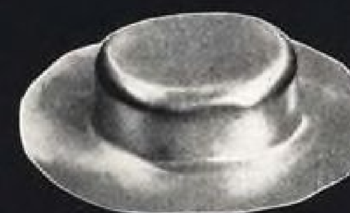
One operation 0.025" RC70 Titanium
