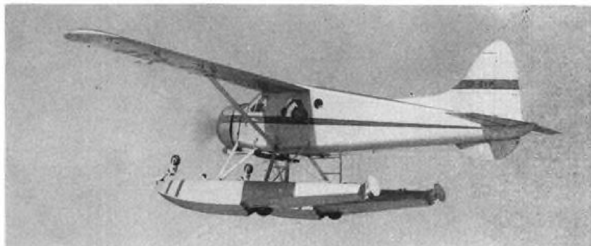
DH BEAVER amphibian retracts main wheels into float bottoms, nosewheels over bows.
