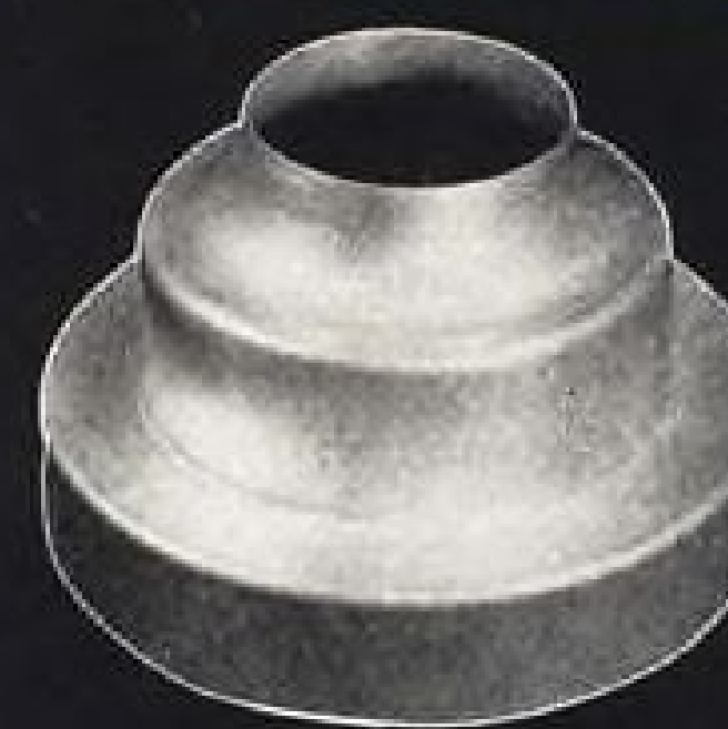
Three operations 0.032" 61SO Aluminum
