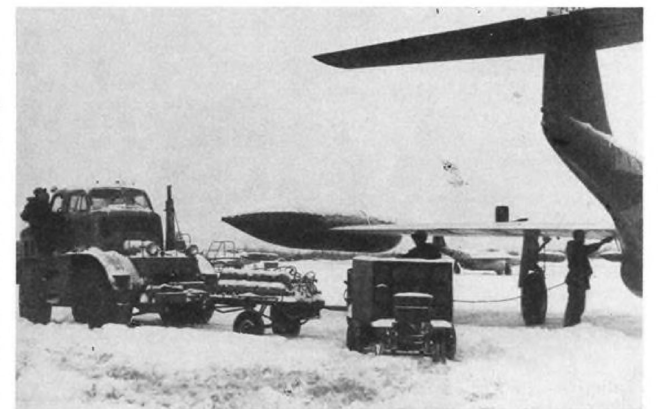
PRE-FLIGHT and post-flight gear with hydraulic fluid, oxygen and nitrogen by F-89D.
