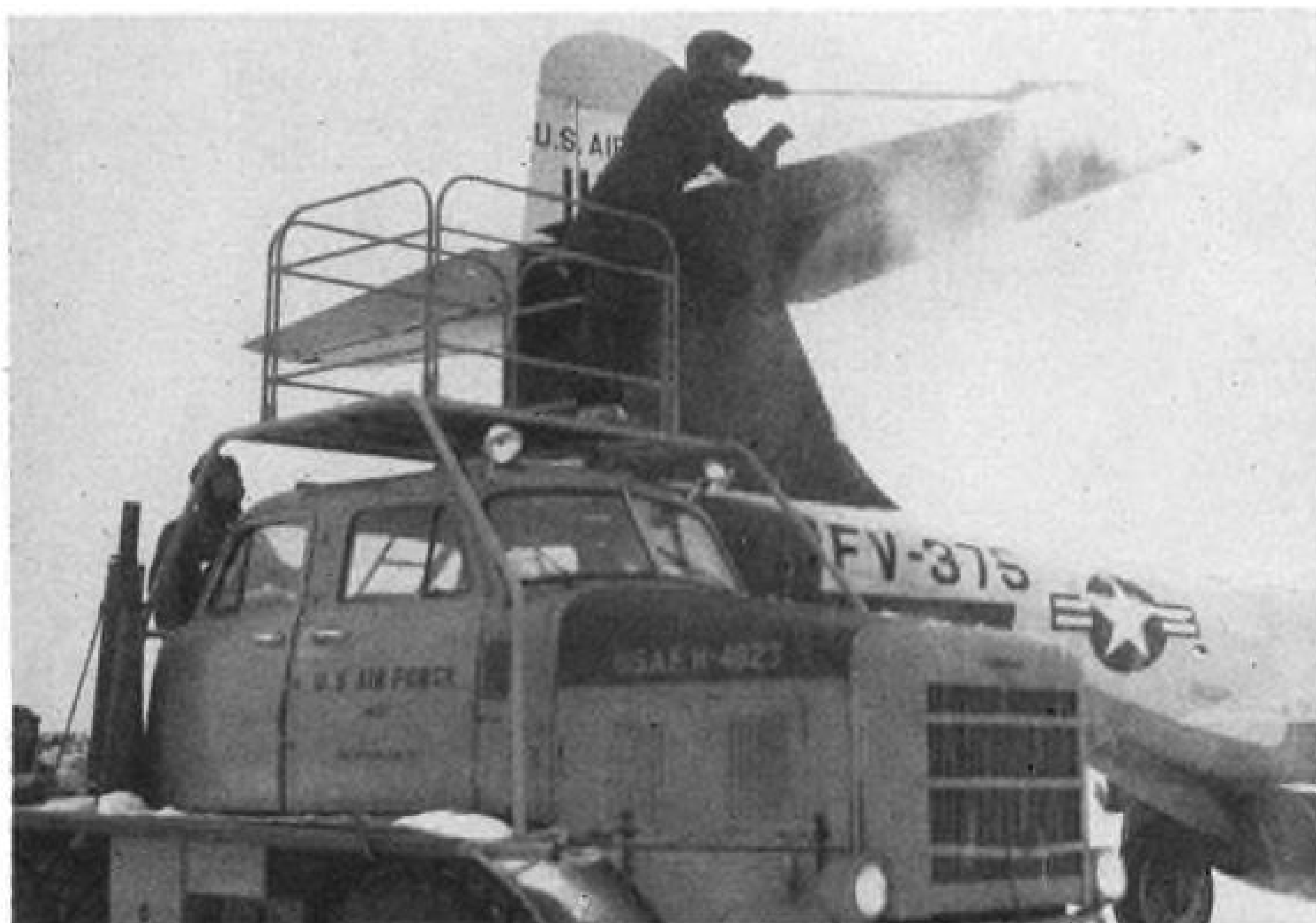
DETACHABLE WORK STAND atop Coleman tractor is handy for cleaning off stabilizers.
