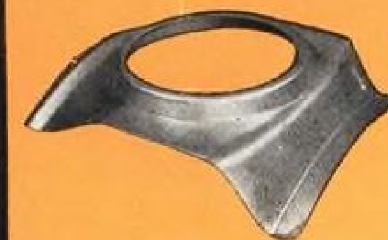
Drop Hammer combined with one Hydroform operation. 0.064" 61SO Aluminum
