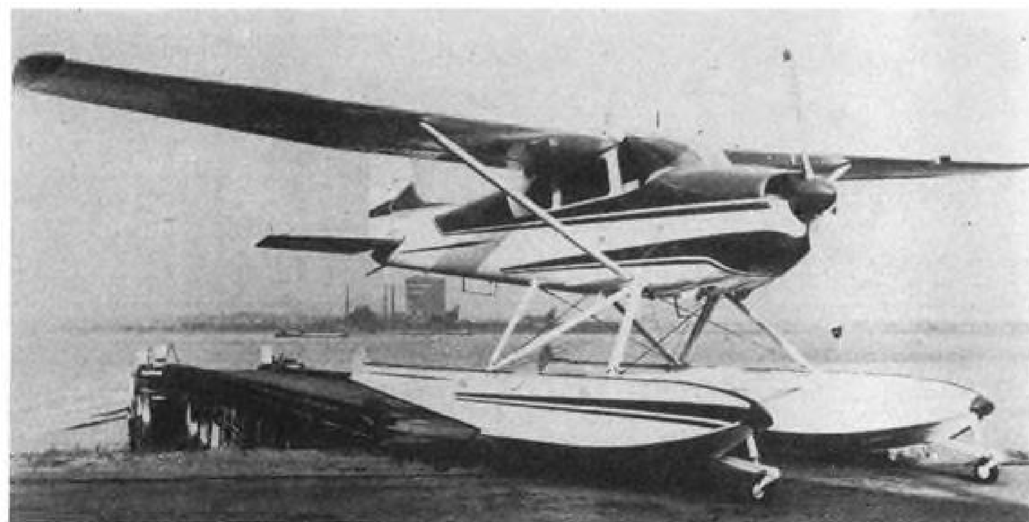
CESSNA 180 amphibian can land in the water, extend its wheels and taxi up ramp.
