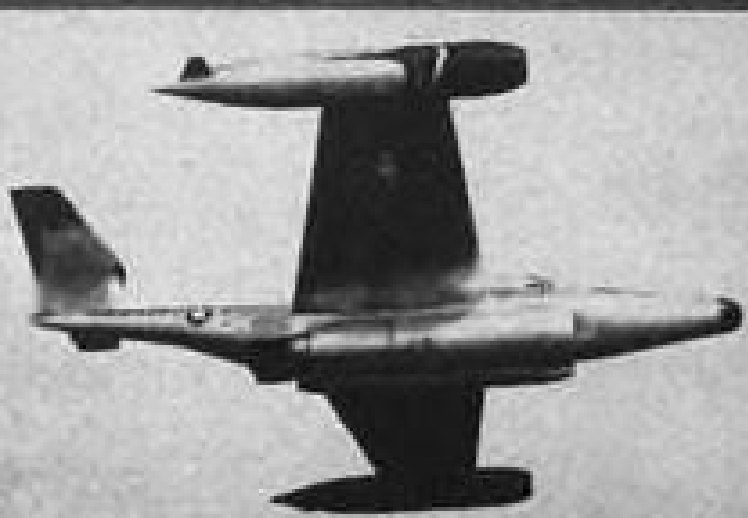
Northrop's Scorpion is the Air Force's most heavily armed all weather interceptor. A rugged fighter, it is powered by two Allison J-35 jet engines with afterburners that put it in the 600 mph class and altitude capabilities of 45,000 feet.
