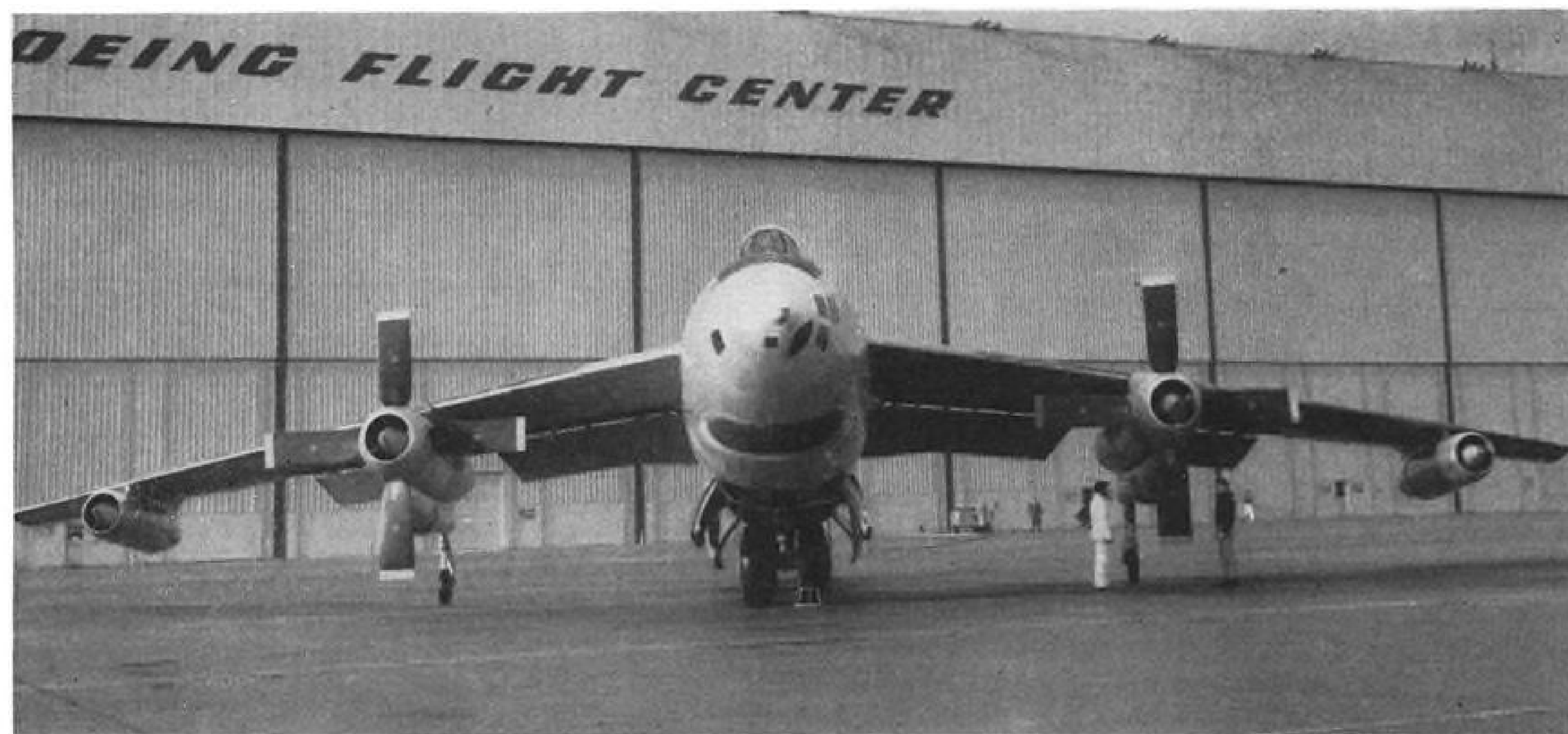
PADDLE BLADES absorb 10,000 hp. of Wright T49 turboprops in Boeing XB-47D flying test bed. Prop diameter is about 15 ft.
