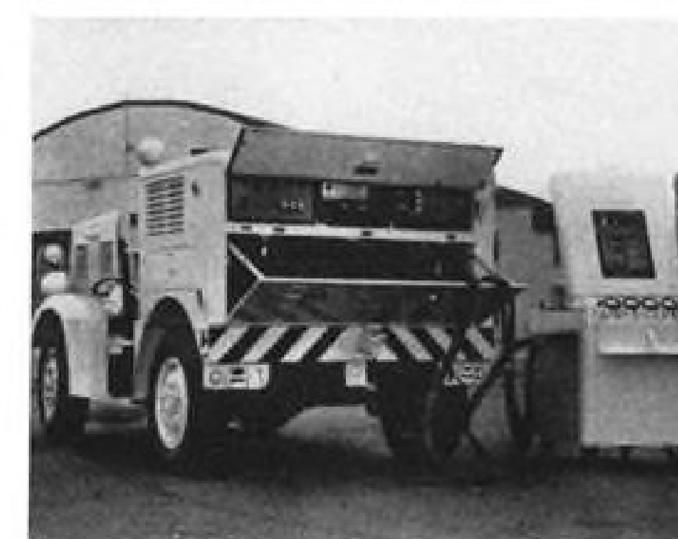
LOAD BANK (right) being used with multi-purpose starter (left).
