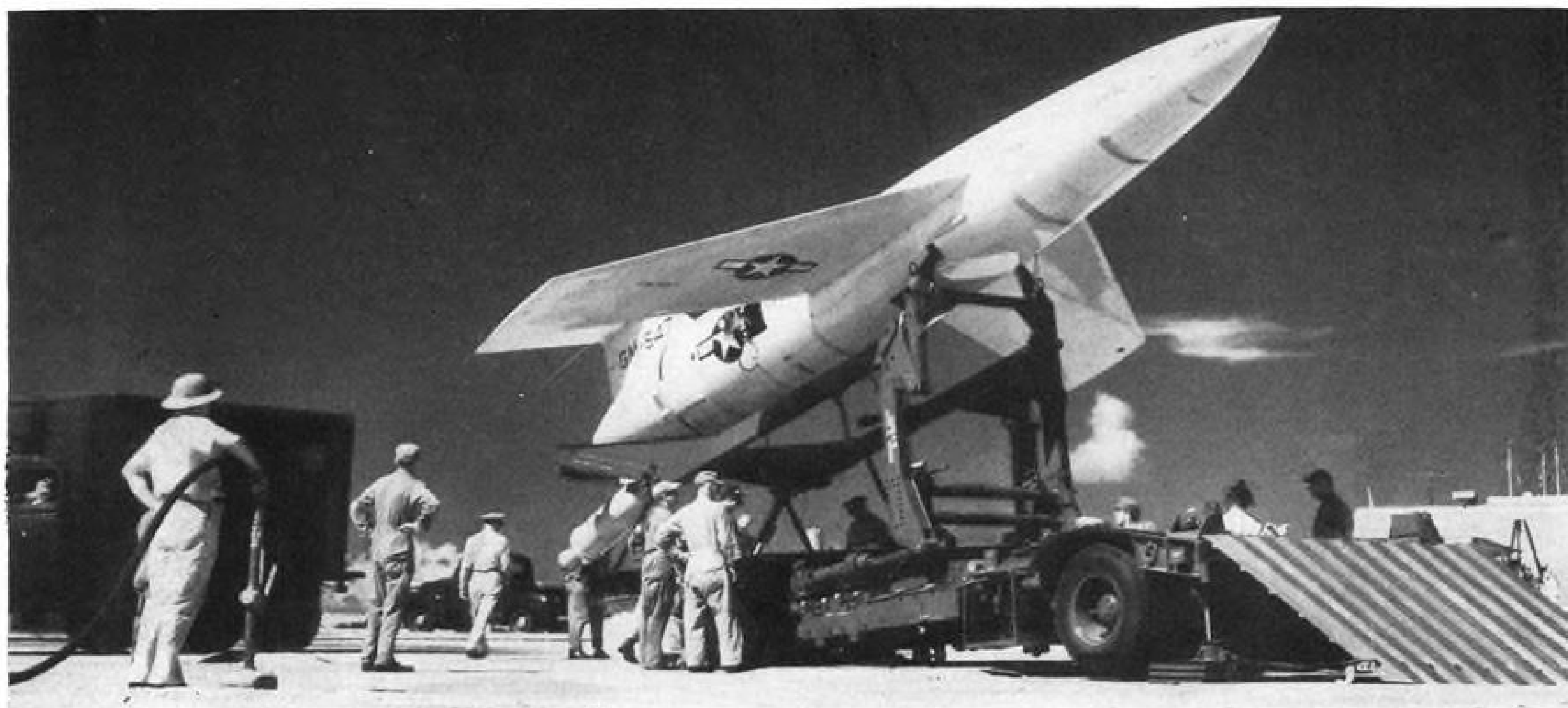
MATADOR uses zero-length launcher mounted on trailer for mobility, needs three other vehicles for firing-site support.
