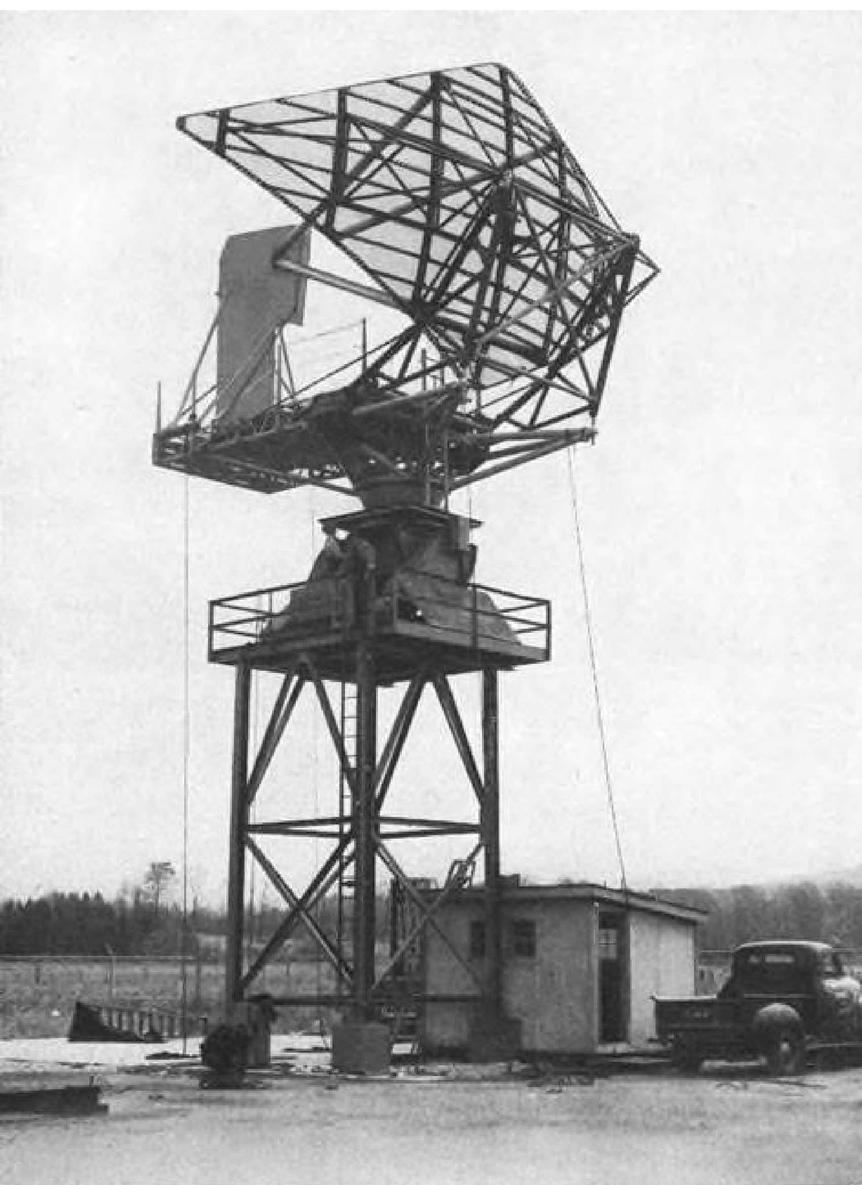
COMPLETE ELECTRICAL TESTING of giant FPS-7 radar search antenna being made on G.E.'s modern pattern test range. This range can test radiation patterns of all sizes in all standard radar frequencies and is the final step in making sure all radar antennas meet operational performance requirements.
