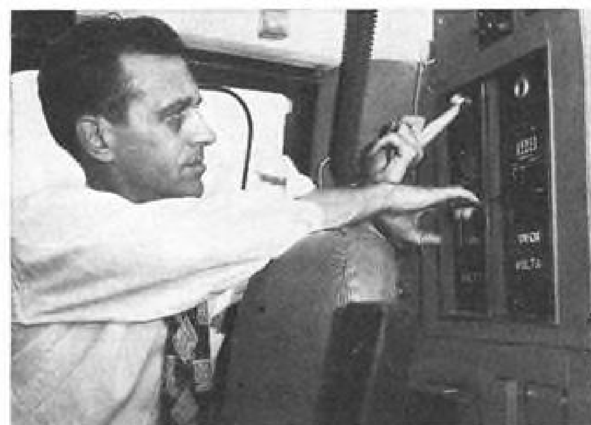
Sitting in co-pilot's seat, American project engineer removes generator control panel in Convair. Maintenance is facilitated by easy removal of generator protective devices which are grouped in G-E load-center units.
