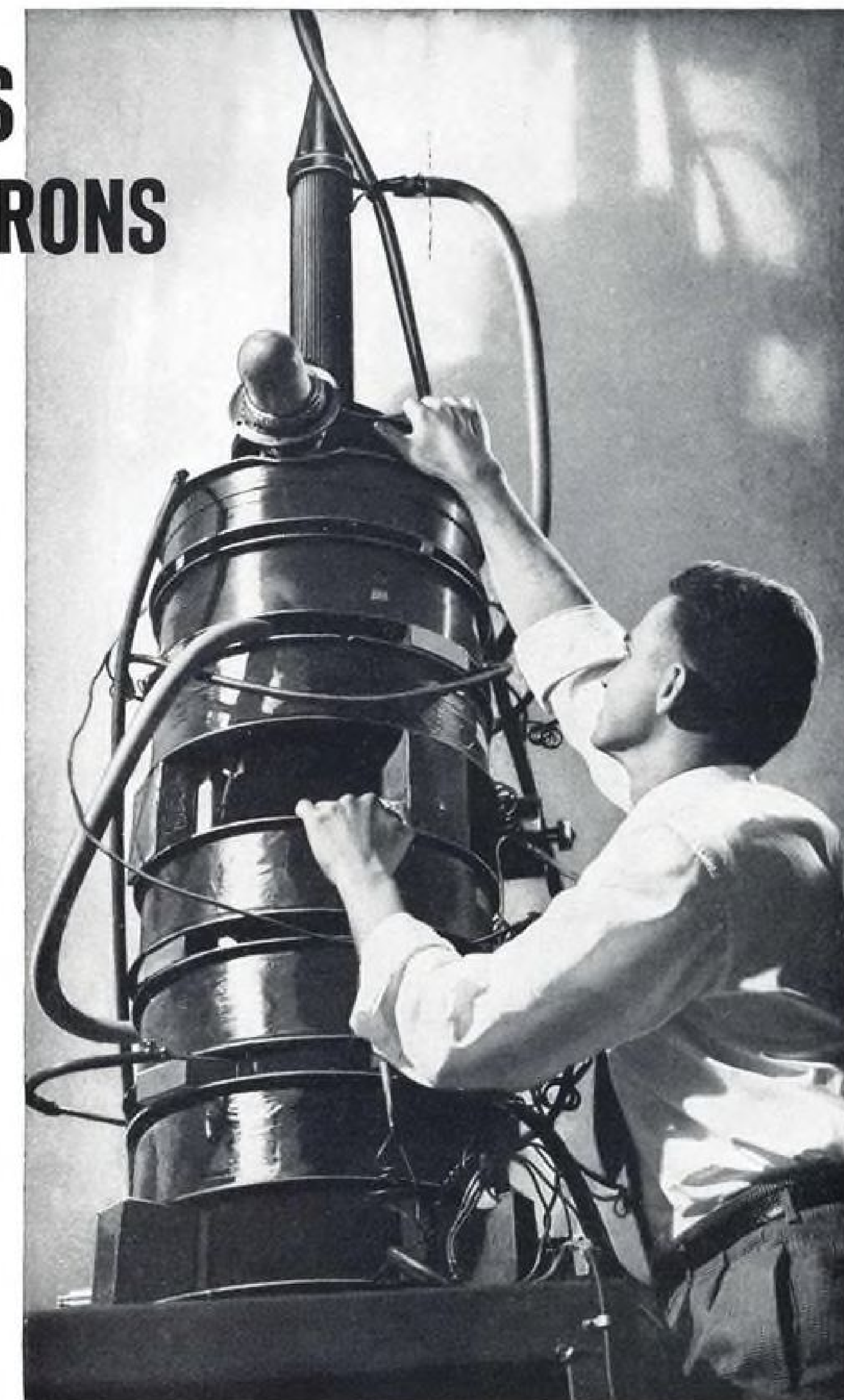
Eight feet tall, the first Megawatt Klystron Amplifier developed for military purposes by Sperry, develops 4,000,000 watts of power with up to 43% efficiency and 38 db. gain. Other Megawatt Klystrons are now in production.
