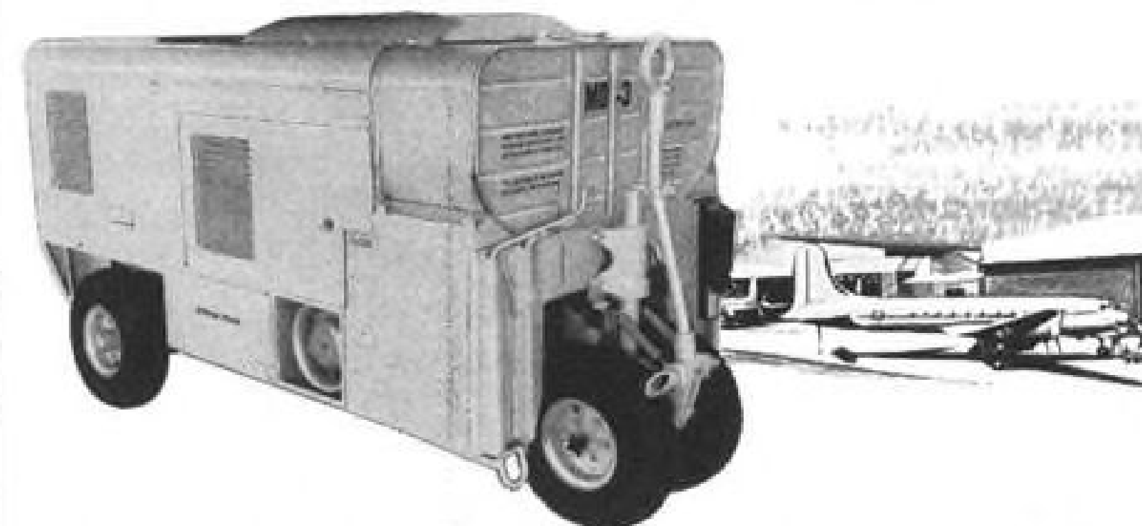
The MD-3 Ground Power Equipment designed and manufactured by Beech Aircraft Corp. is used by the Air Force to check out aircraft in pre-flight test. The VARO Frequency Meter is utilized as part of the system to provide accurate and reliable measurement of 400 cycle electrical systems.
