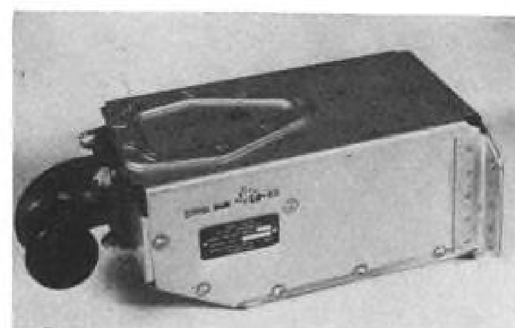
VALVE ends fuel tank vent-line splash.
