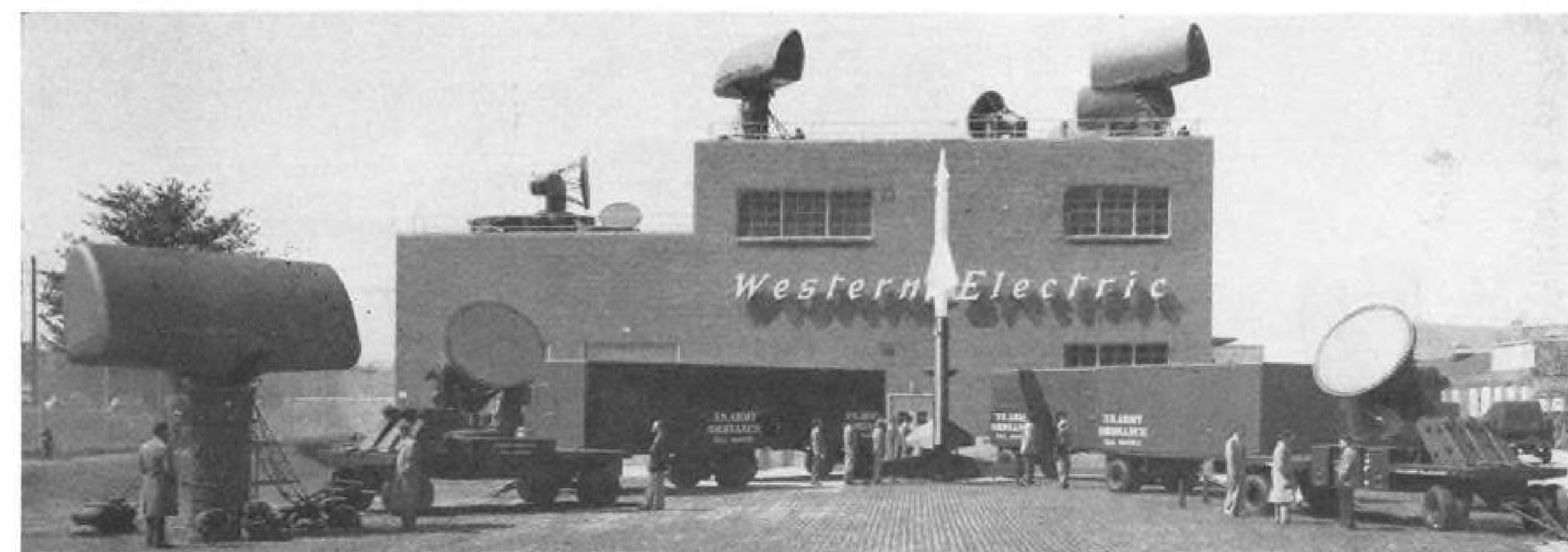
NIKE NEEDS are served by acquisition and guidance radars, vans for control and command centers and mobile launchers.
