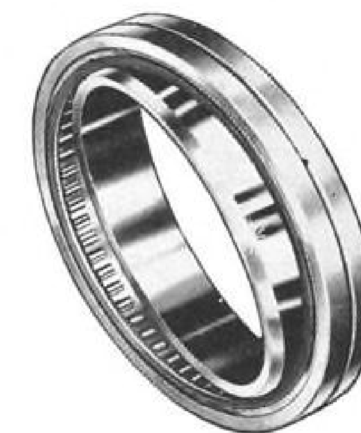
Double-Row Torque Tube Bearing ...Instant self-alignment always available....Easy relubrication without disassembly....High radial and thrust load capacity....Exceptional shock-load reserve strength.
