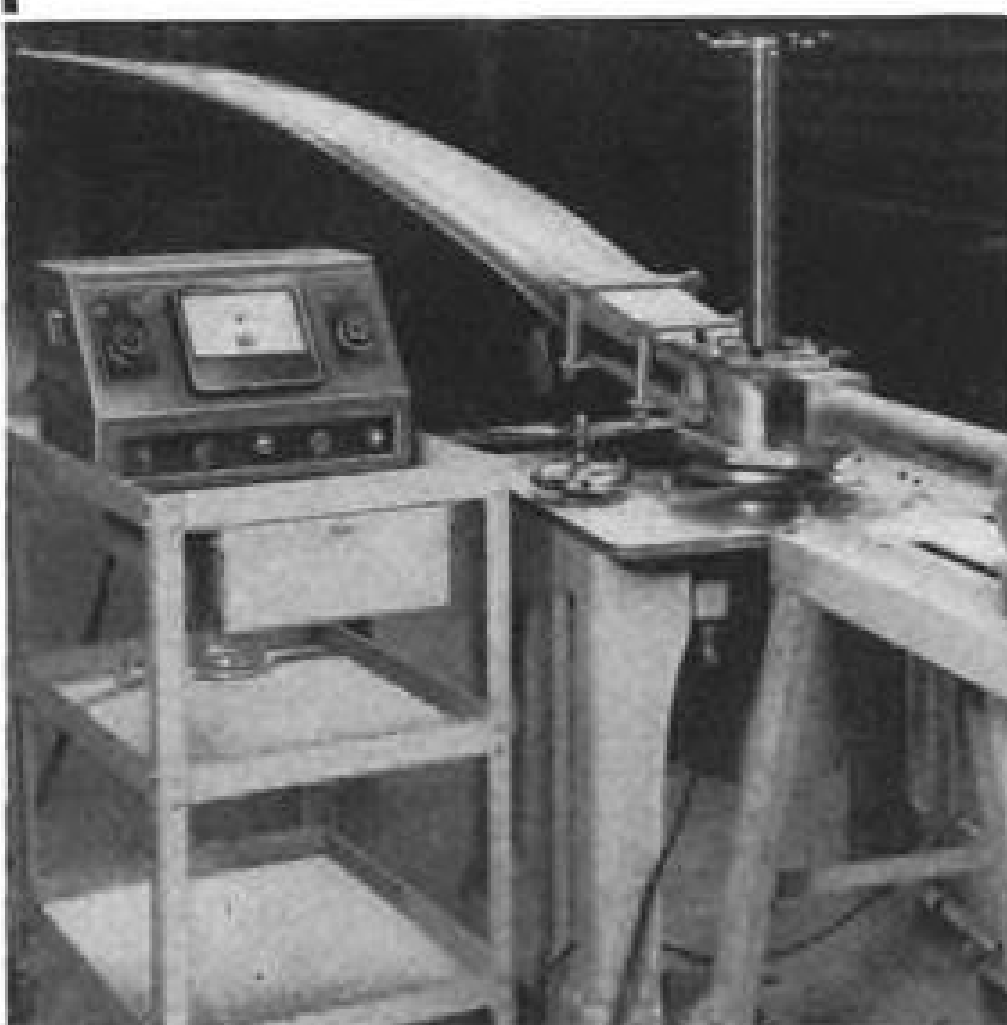
Kaman Aircraft Corp. Now Balances Their Helicopter Rotor Blades And Assemblies On a Dean And Benson Machine
