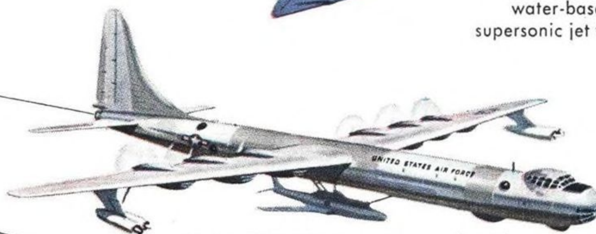
GRB-36 "AIRCRAFT CARRIER" — launches and retrieves fighters in flight
