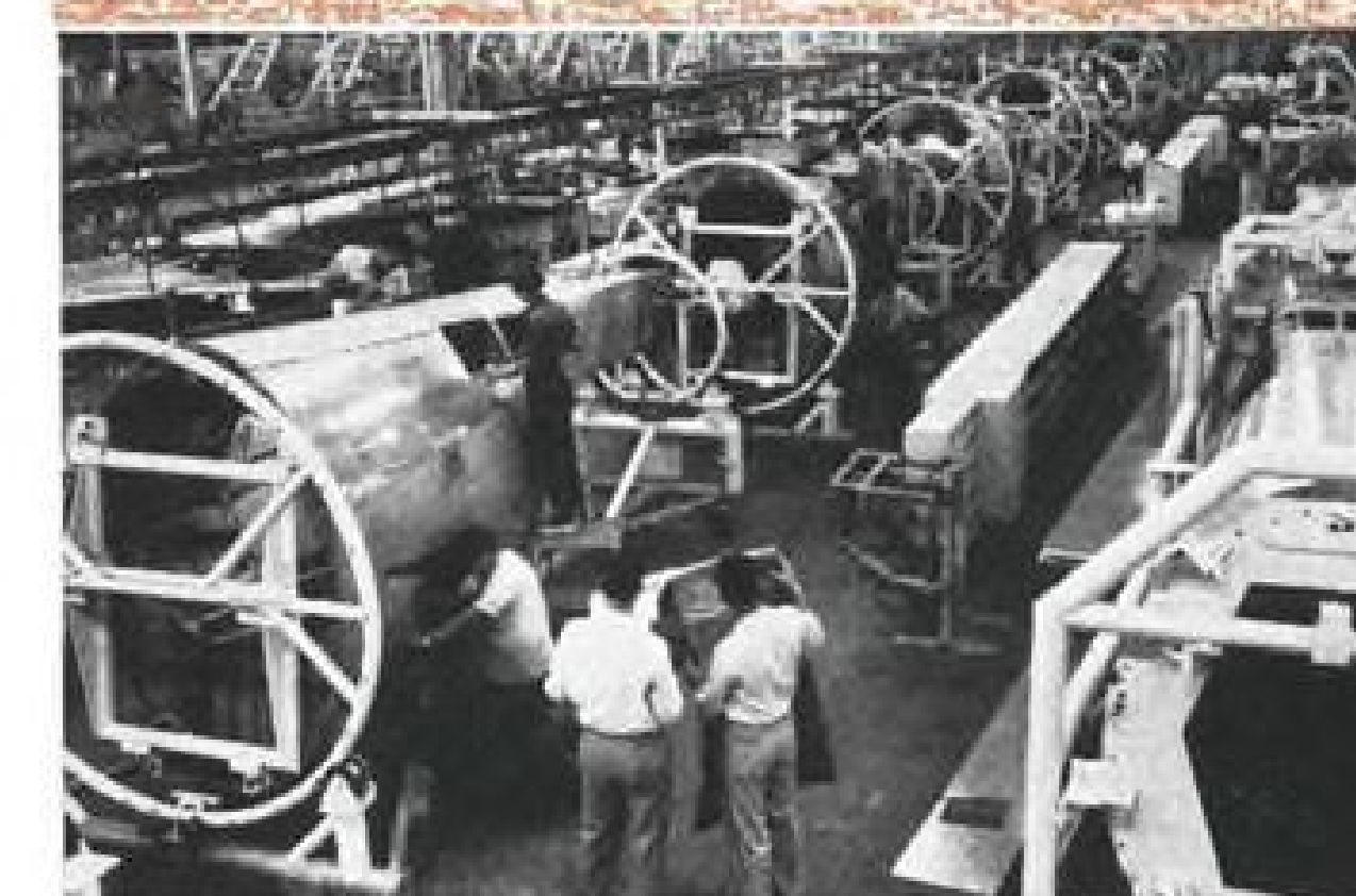
F3H aft fuselage sections on rotating circular jigs move down TEMCO-Dallas assembly lines. Elsewhere in the Dallas plant, a twin line is devoted to inner wings, while outer wings take shape at TEMCO's Garland plant.
