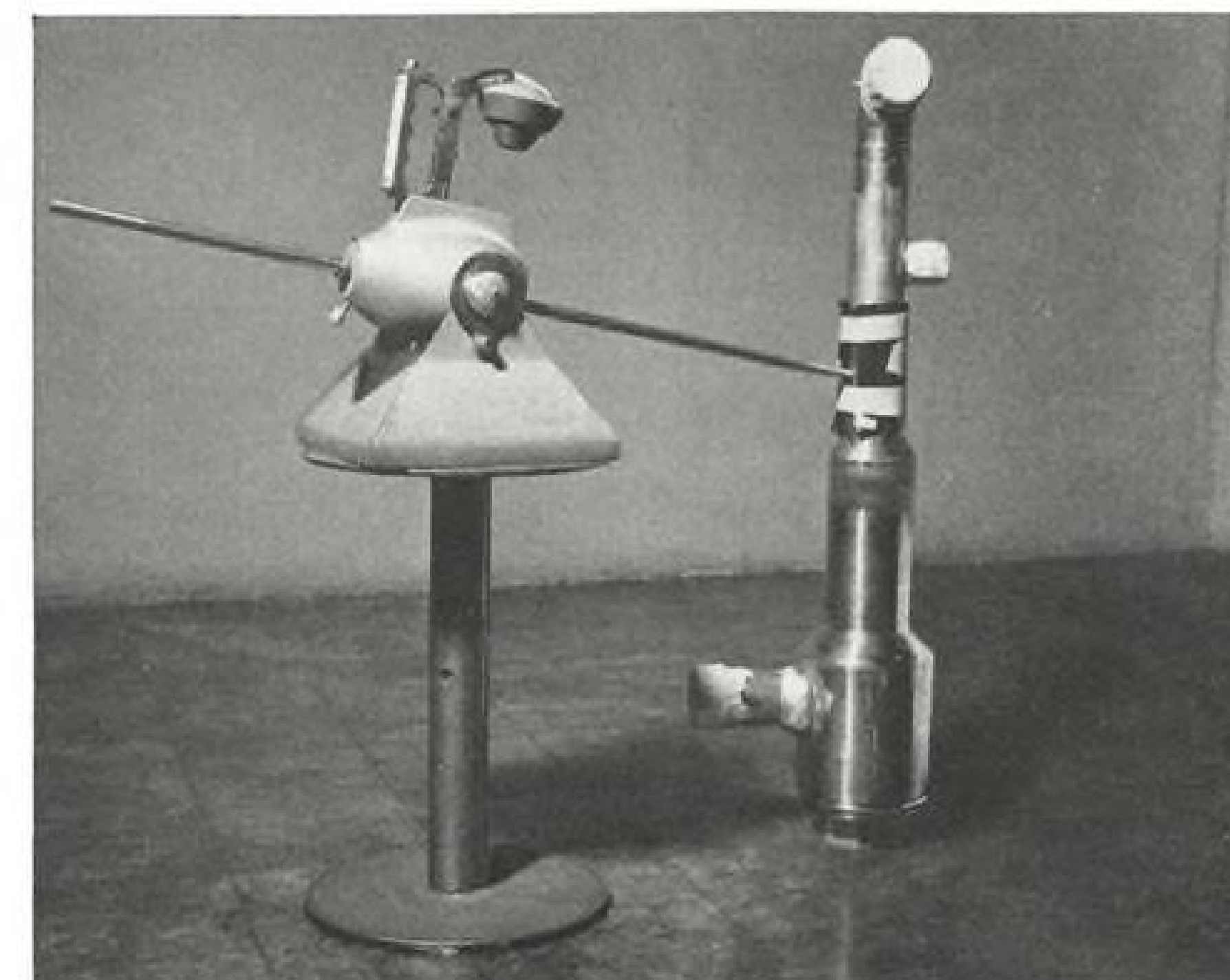
Welded pipe joint being radiographed with isotope camera using iridium 192.
