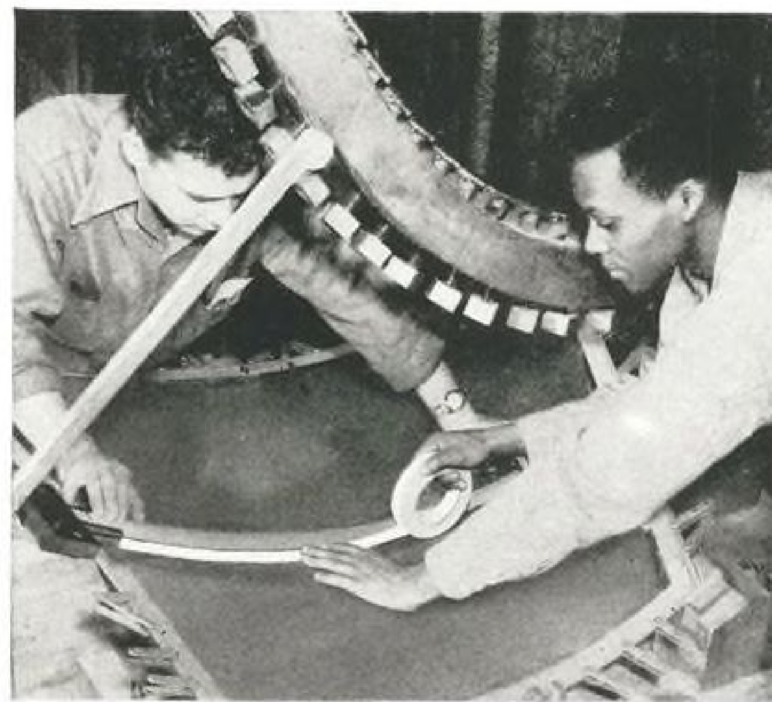
PERMACEL 76 masking tape is used to mask plastic helicopter nose assembly in Piasecki cementing operation. Specially treated to be highly resistant to solvents—does not pit or scar the plastic.
