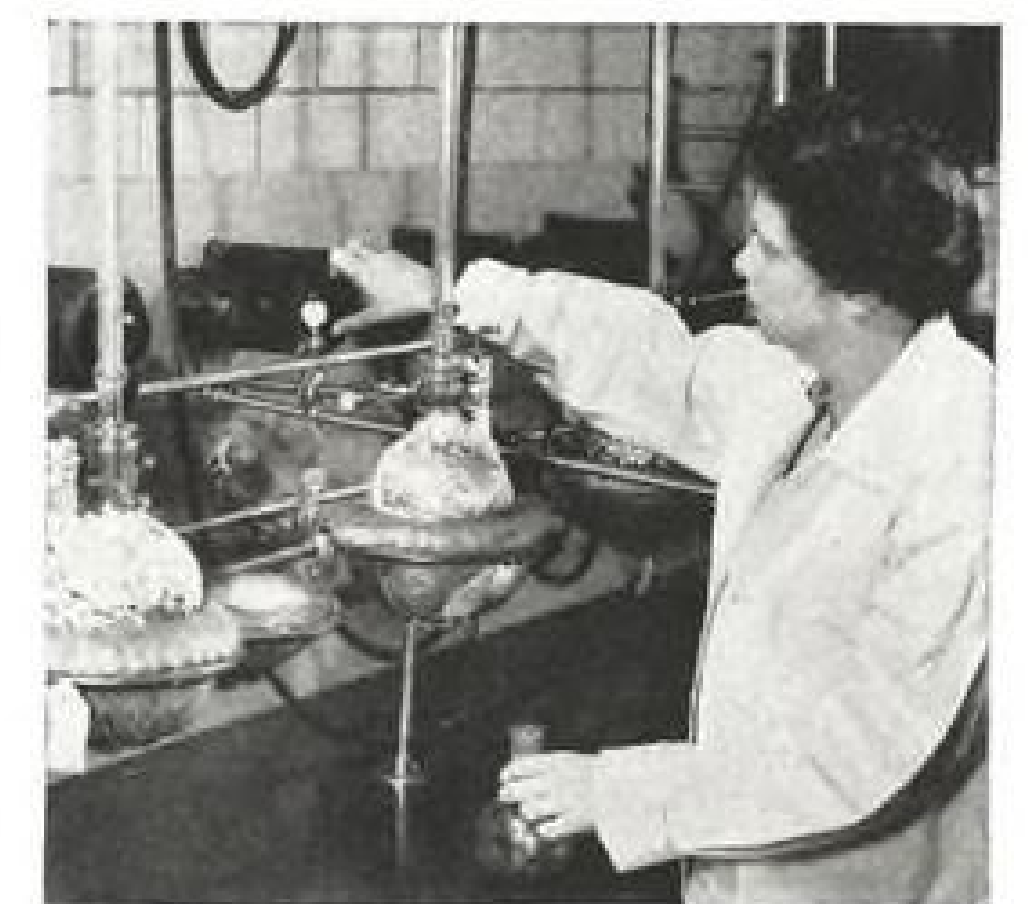
Laboratory and service tests check compound resistance to oils, fuels and chemicals at high and low temperatures ... assuring the long life of Parker O-rings.
