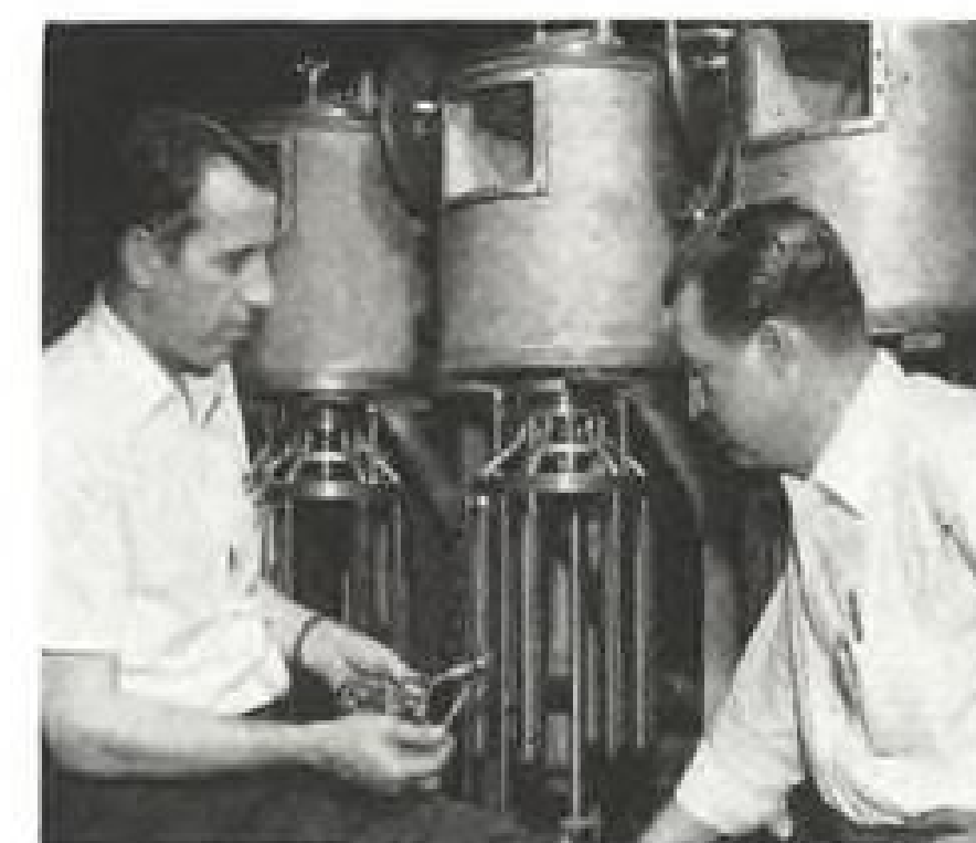
These two development engineers are evaluating a new fuel nozzle. The equipment in the background is designed to test the performance of fuel systems.
