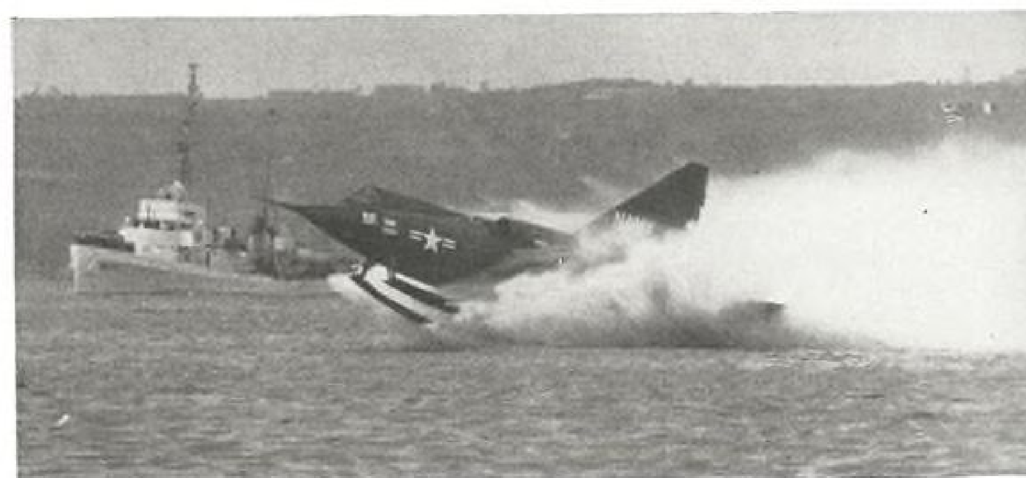
CONVAIRE XFV-1 SEA DART out of the water and on its twin hydro-skis during a run in a continuation of the experimental turbojet, water-based fighter's Navy evaluation program.
