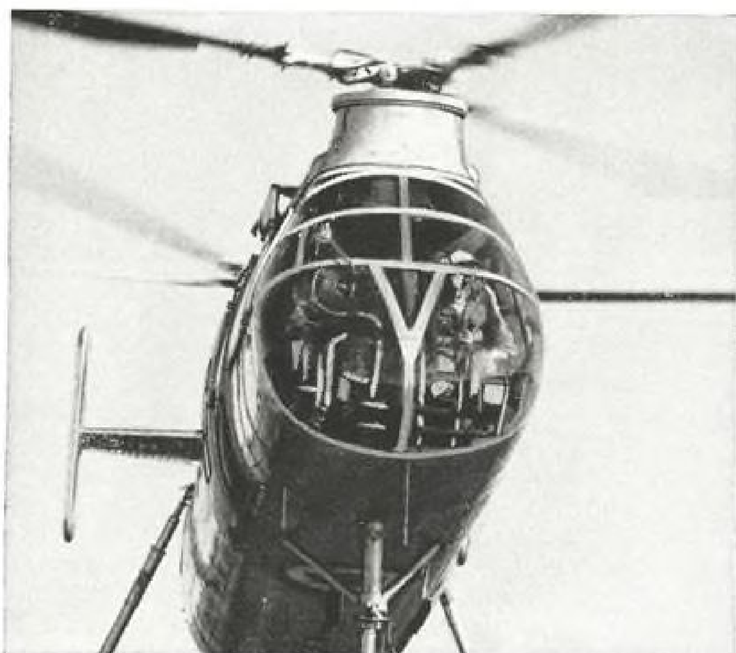
NOSE ON view of a Piasecki-built Royal Canadian Air Force helicopter showing complex plastic sections, the transparency of which was protected by Permacel 76 during cementing.
