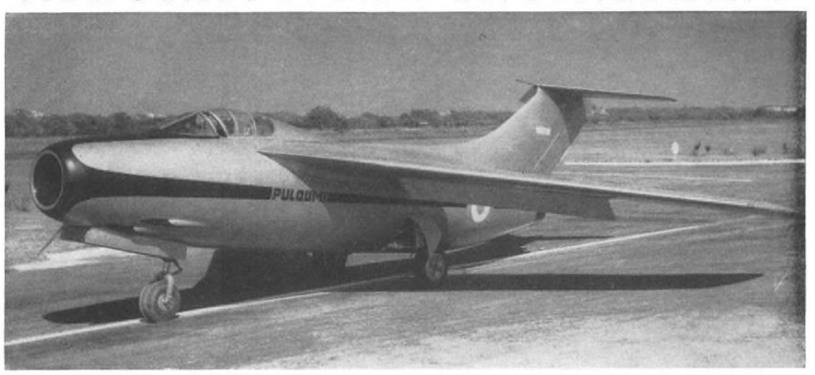
PULQUI II FIGHTER INTERCEPTOR with top speed of 625 mph. was second jet plane built in Argentina. First was the Pulqui I.
