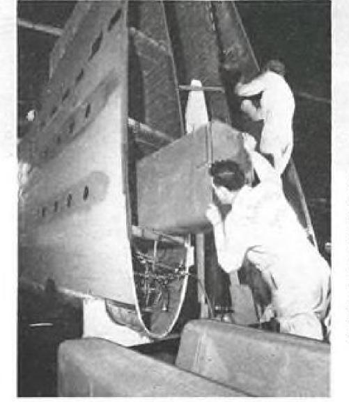
800 MILES MORE RANGE for DC-3s is achieved through the exchange of wings containing auxiliary fuel tanks with 400 gallons added capacity. By exchanging wings, installation time is cut in half.
