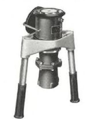
A self-sealing coupling valve, No. 4092 is quickly and easily connected for refueling or defueling. Unusually low pressure drop. Self-adjusting; fits any qualified adapter. Couples, locks and controls flow in one motion. No auxiliary controls. Seals automatically when disconnected.
