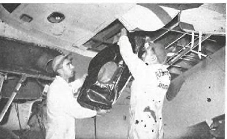
SAFETY FACTOR FOR LODESTARS INCREASED by replacing present integral tanks with Goodyear nylon fuel cells. Experienced, licensed mechanics at AiResearch Aviation Service have made this installation for many Lodestar owners.
