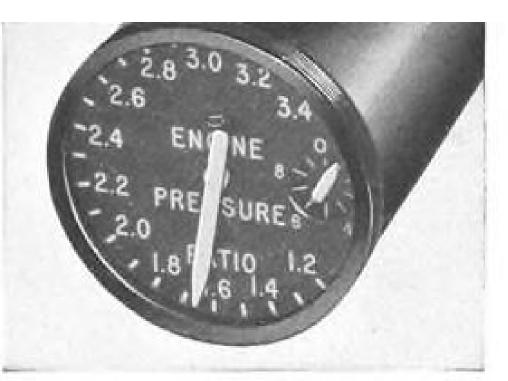
Pressure Ratio Indicator. Today's jet pilot is assured an easy, accurate take-off power check, and more economical cruise performance with the new Honeywell Pressure Ratio Indicator. It accurately measures the ratio of jet inlet pressure to exhaust pressure. Another model is available which measures the difference in pressures.
