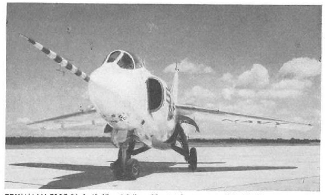
GRUMMAN F11F-1's knife-like airfoil could not take any part of the landing gear assembly.
