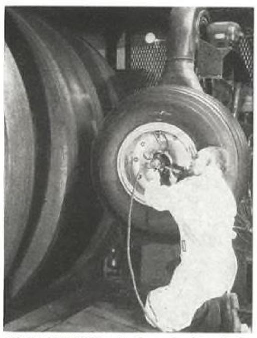
DYNAMOMETER simulates landing loads.
