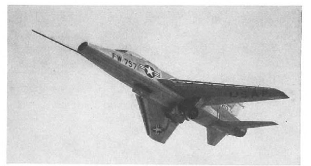
NORTH AMERICAN F-100's thin wing forced designers to tuck landing gear in fuselage.
