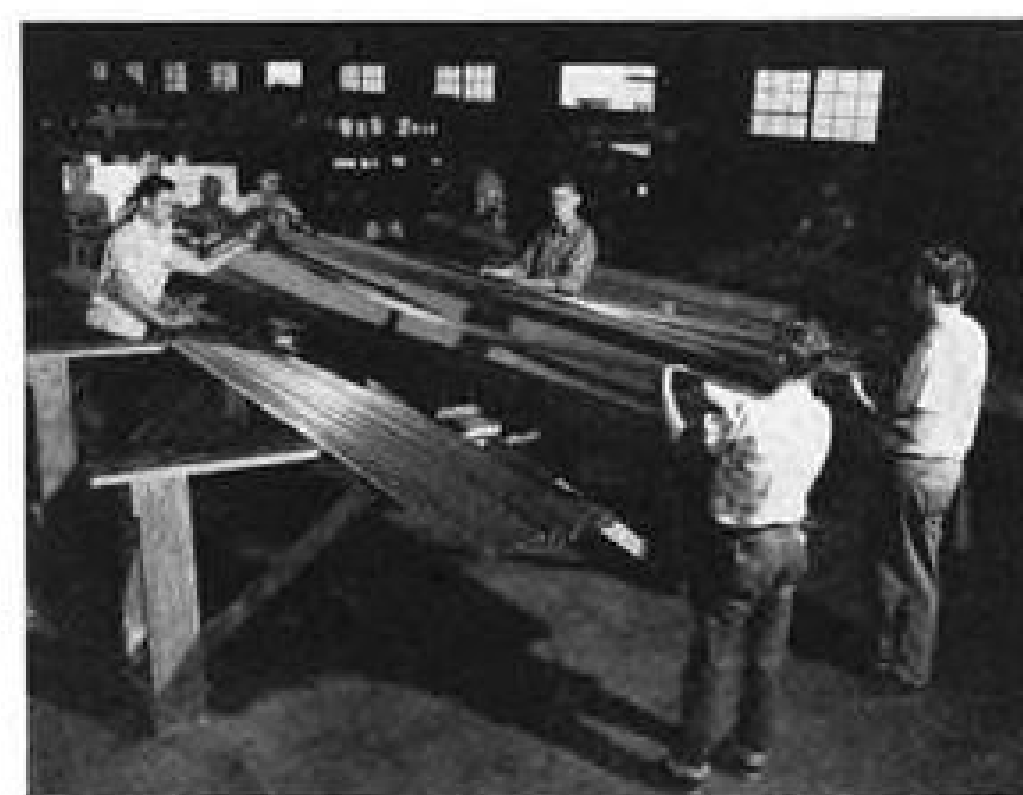
All extrusions are maintained in stock in an oiled condition to prevent corrosion and carefully packaged for safe, sure delivery.
