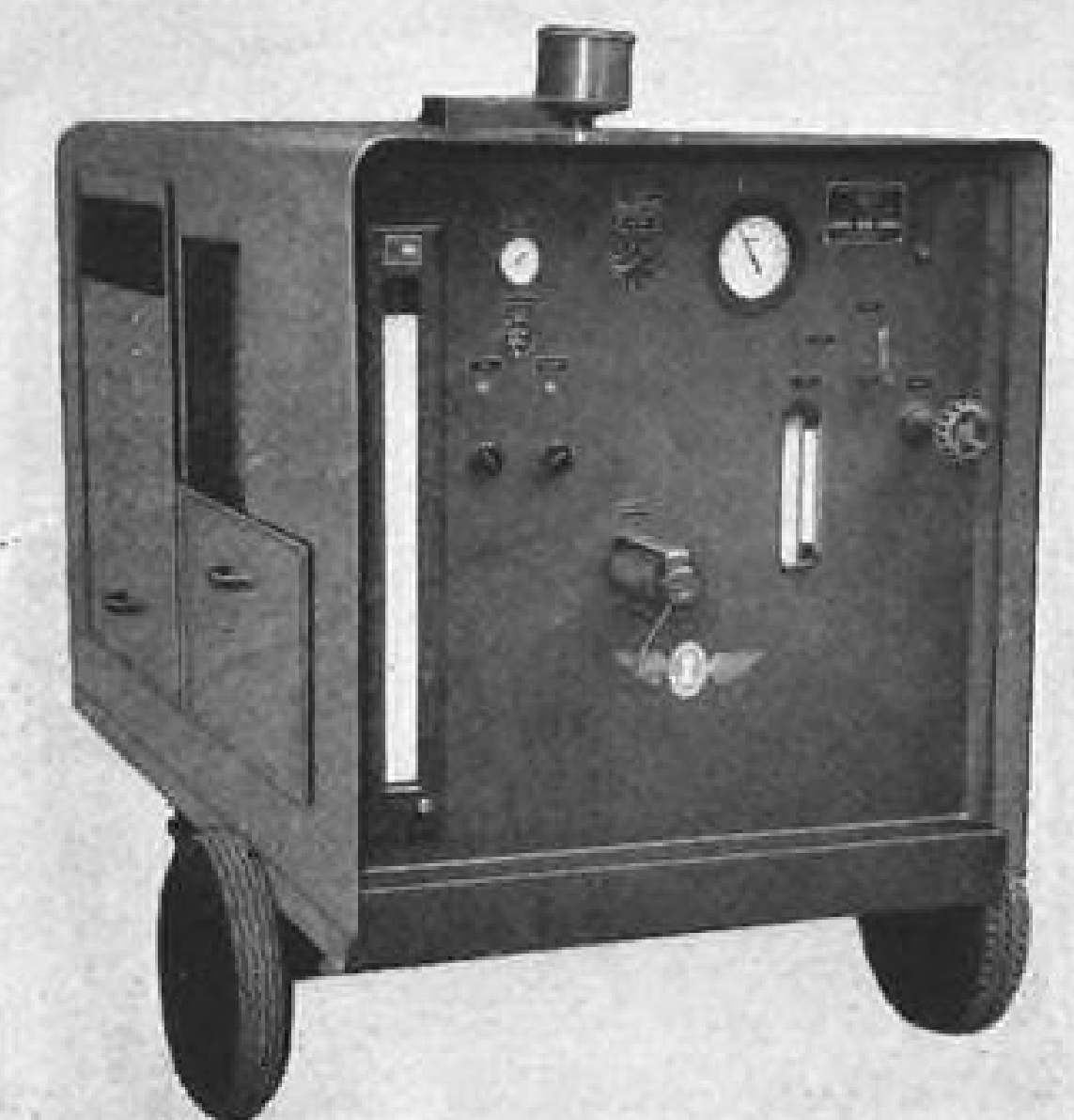
Greer aircraft cabin leakage test stands use Miehle-Dexter Positive Displacement Blowers for pressure testing cockpit and fuselage. Single blower integrated into original design provides 400 c.f.m. at 10 psig.
