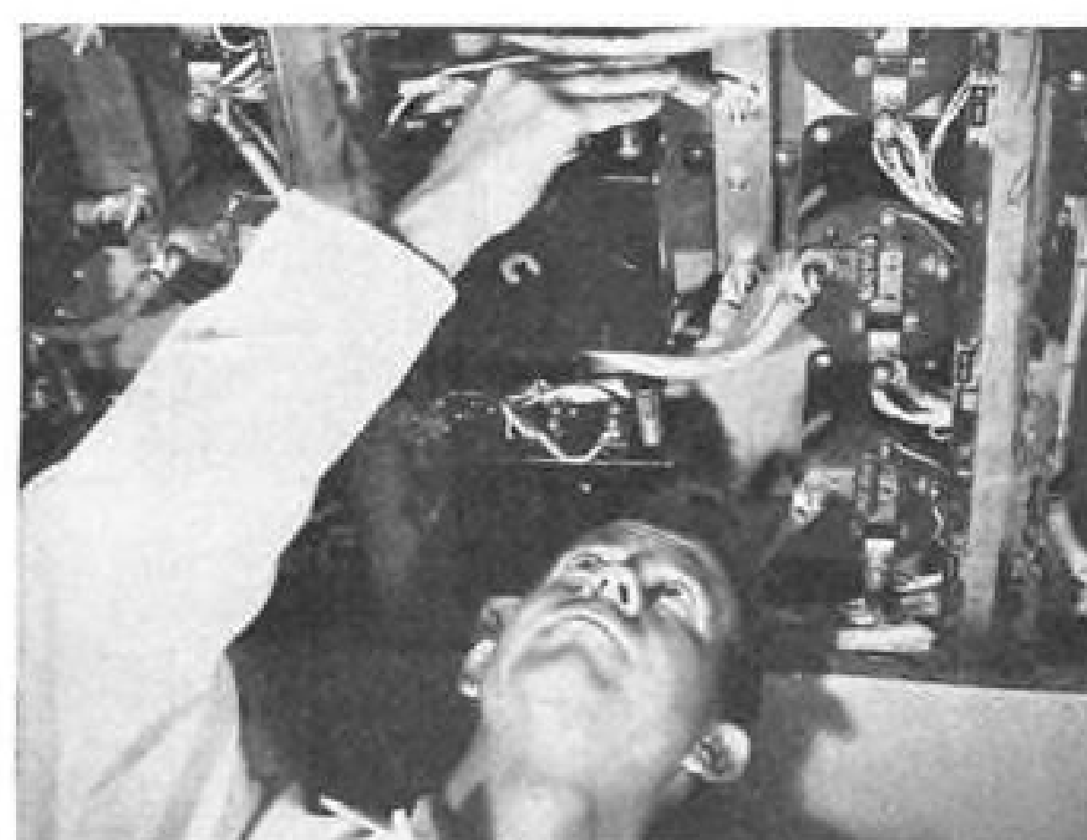
Arrangement of G-E circuit breakers shows high accessibility—an important part of Pan American's program for easier maintenance of electric systems.
