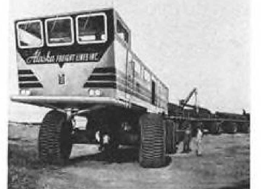
LeTOURNEAU SNO-FREIGHTER. 24 electric wheels of this six-section vehicle drive and brake to carry large tonnages of cargo into arctic wastelands.
