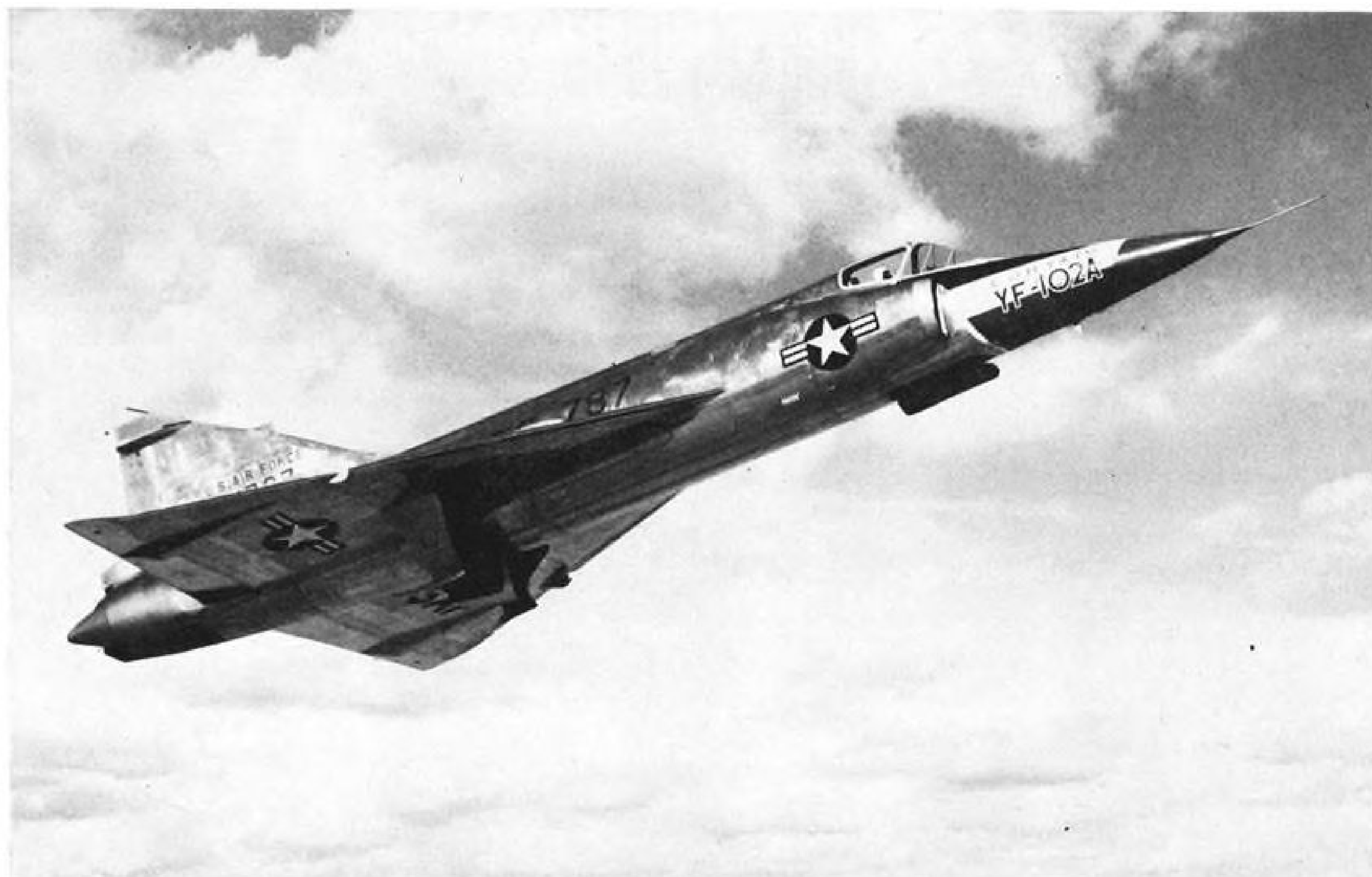
Landing gear of the new delta-wing Convair F-102A is almost retracted in this test flight takeoff. The new Air Force interceptor, designed to fly day or night—in any kind of weather, exceeded the speed of sound in level flight its second time in the air.
