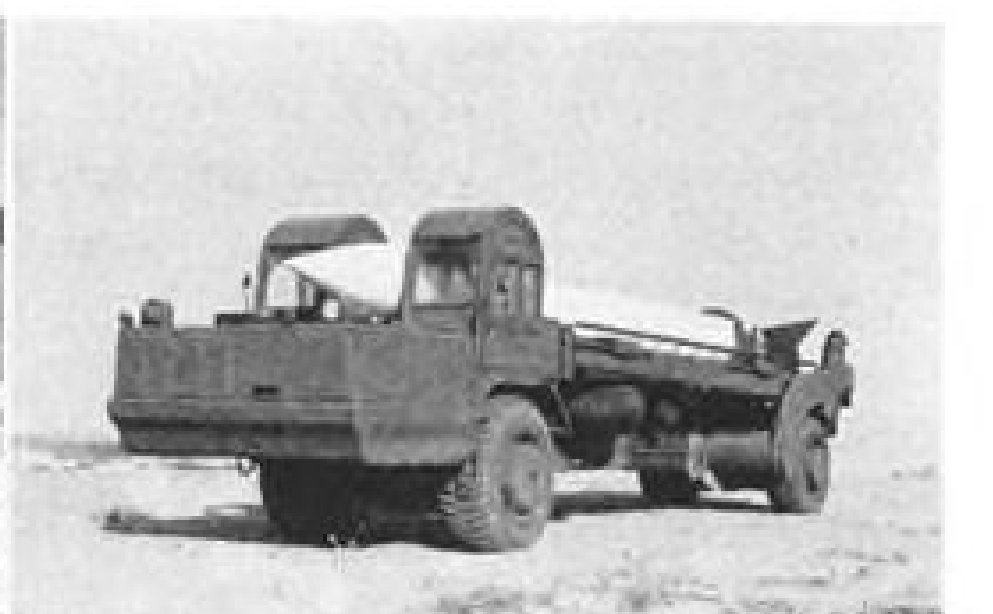
LeTOURNEAU CORPORAL LOADER for ground handling the Corporal Guided Missile. This electric wheel vehicle picks up, transports, and erects the missile.
