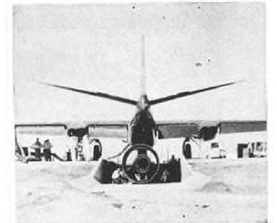
Flying test beds like this B-45 airplane are used to test new designs in the air . Flight testing is the ultimate proof of the value of a new design.
