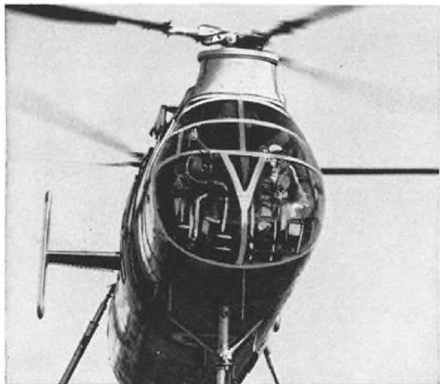
NOSE ON view of a Piasecki-built Royal Canadian Air Force helicopter showing complex plastic sections, the transparency of which was protected by Permacel 76 during cementing.
