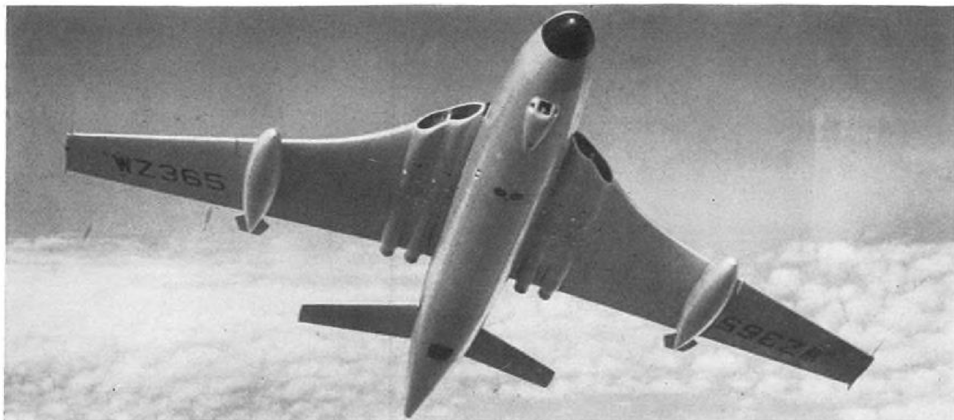
BELLY DETAILS OF THE VICKERS VALIANT , medium bomber now in service with the Royal Air Force, show nose radome containing advanced model of wartime H2S bombing system; visual bombing is done from housing just below and aft the radome. Bombardier is behind optically-flat window at front of housing. Behind housing are nose-wheel doors. Circular windows may be camera ports. Large bomb-bay has additional radar equipment mounted above the dielectric panel. Chutes for dropping anti-radar "window" can be seen either side of the camera ports; additional chutes are aft of the rear radar position. This production Mk. 1A Valiant features underwing, pylon-mounted fuel tanks with tail fins. Fences are short and on upper wing surface only and just outboard of the auxiliary fuel tanks.
