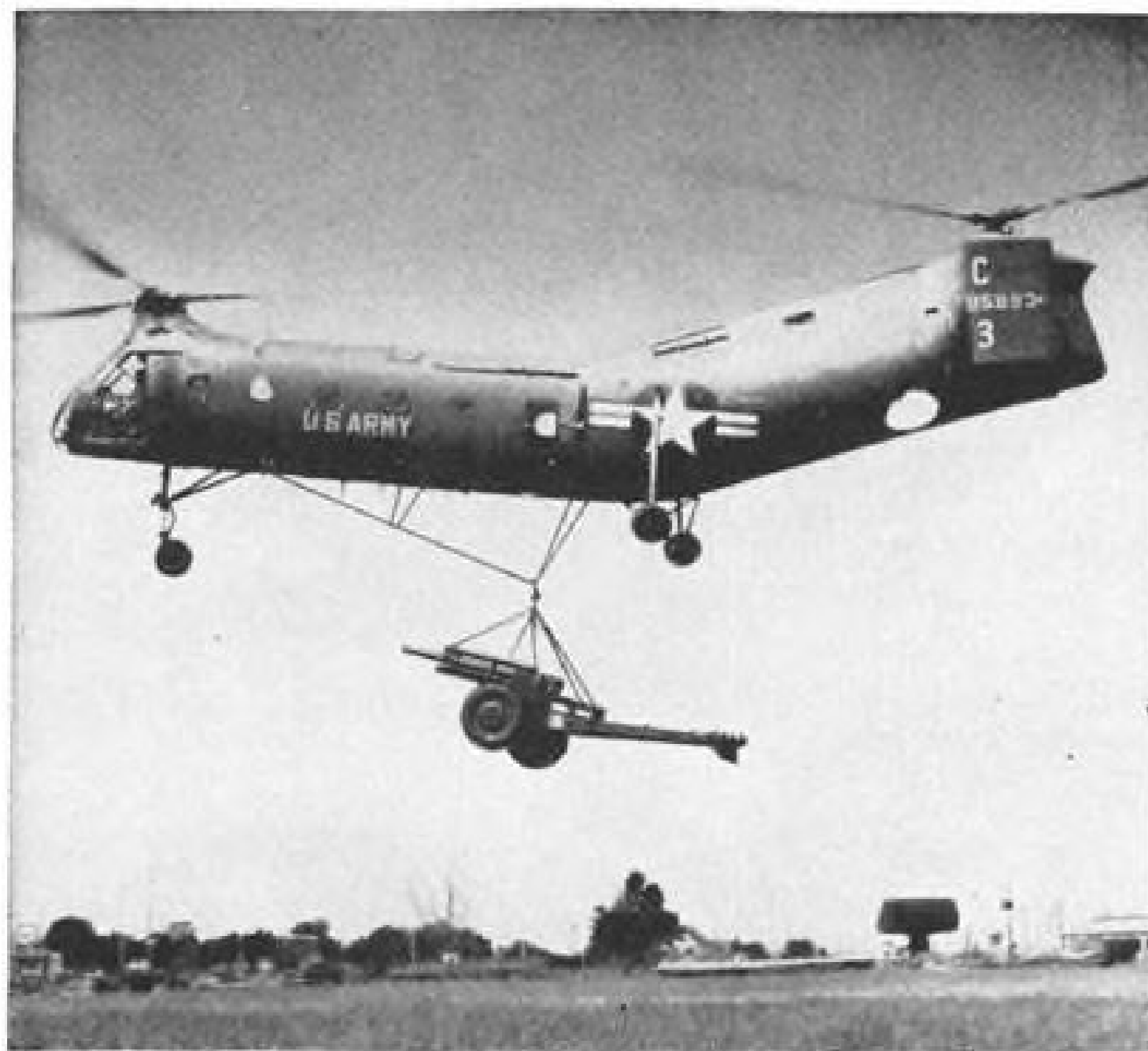
105 HOWITZER goes aloft by Piasecki-built Army H-21 C Work Horse helicopter—the heaviest load ever carried by a Service helicopter. Same ship carries 20 troops or 2 tons of cargo.
