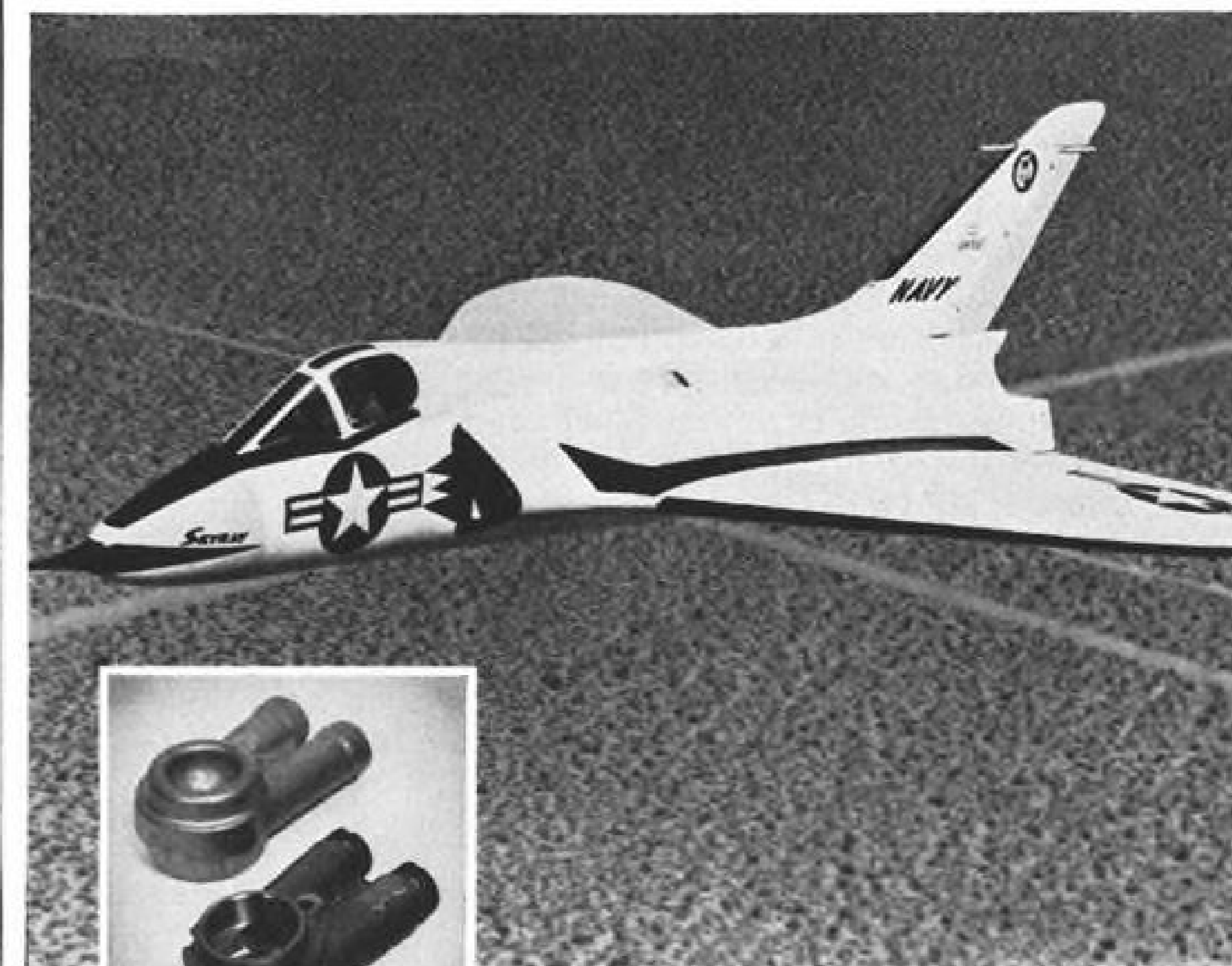
Forgings of MST titanium alloy before and after finish machining.
