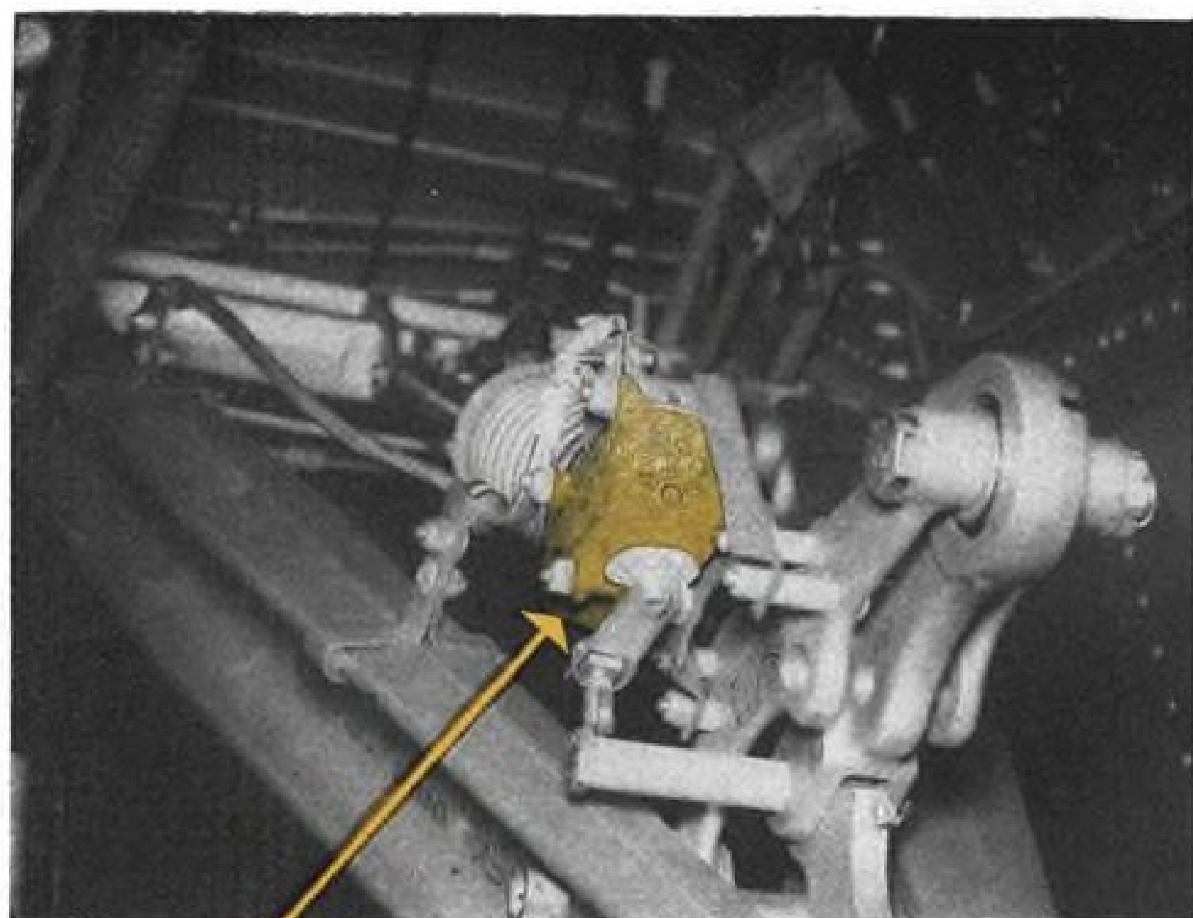
DOUGLAS GETS DEPENDABLE SWITCHING ON THE RB-66 Air Force-Douglas Bomber with Electro-Snap Hermetically-Sealed Limit Switches. Close-up of RB-66 nose gear assembly shows how Electro-Snap Switch is mounted to indicate when gear is locked down.
