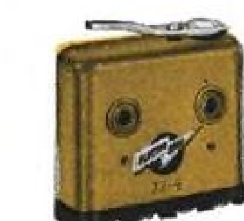
Flap Switch When flap closes and depresses actuator, switch simultaneously operates four 10 amp, 30v DC circuits.
