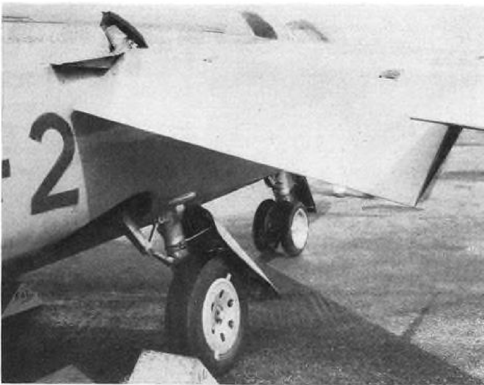
POWER-OPERATED inboard ailerons droop when undercarriage legs are fully down and serve as flaps to steepen angle and reduce Gnat's landing-approach speed.
