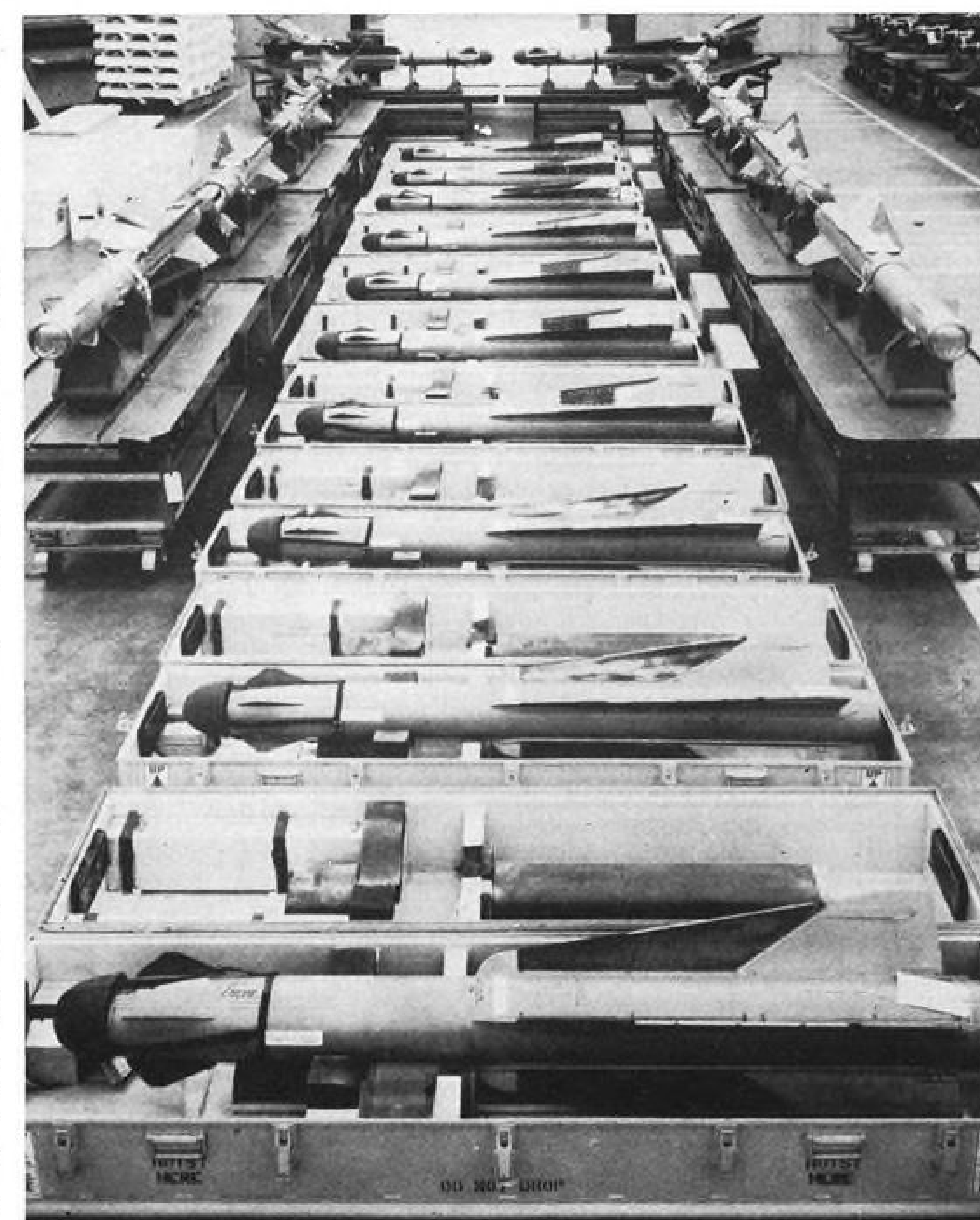
LEAVING THE NEST, a group of Falcons shown in shipping cases will be used for flight test purposes, as evidenced by telemetering antennas (silver strips) mounted on insulated portions of the wing. Reliable sources report that the Falcon missile is capable of operating well into the supersonic speed range.
