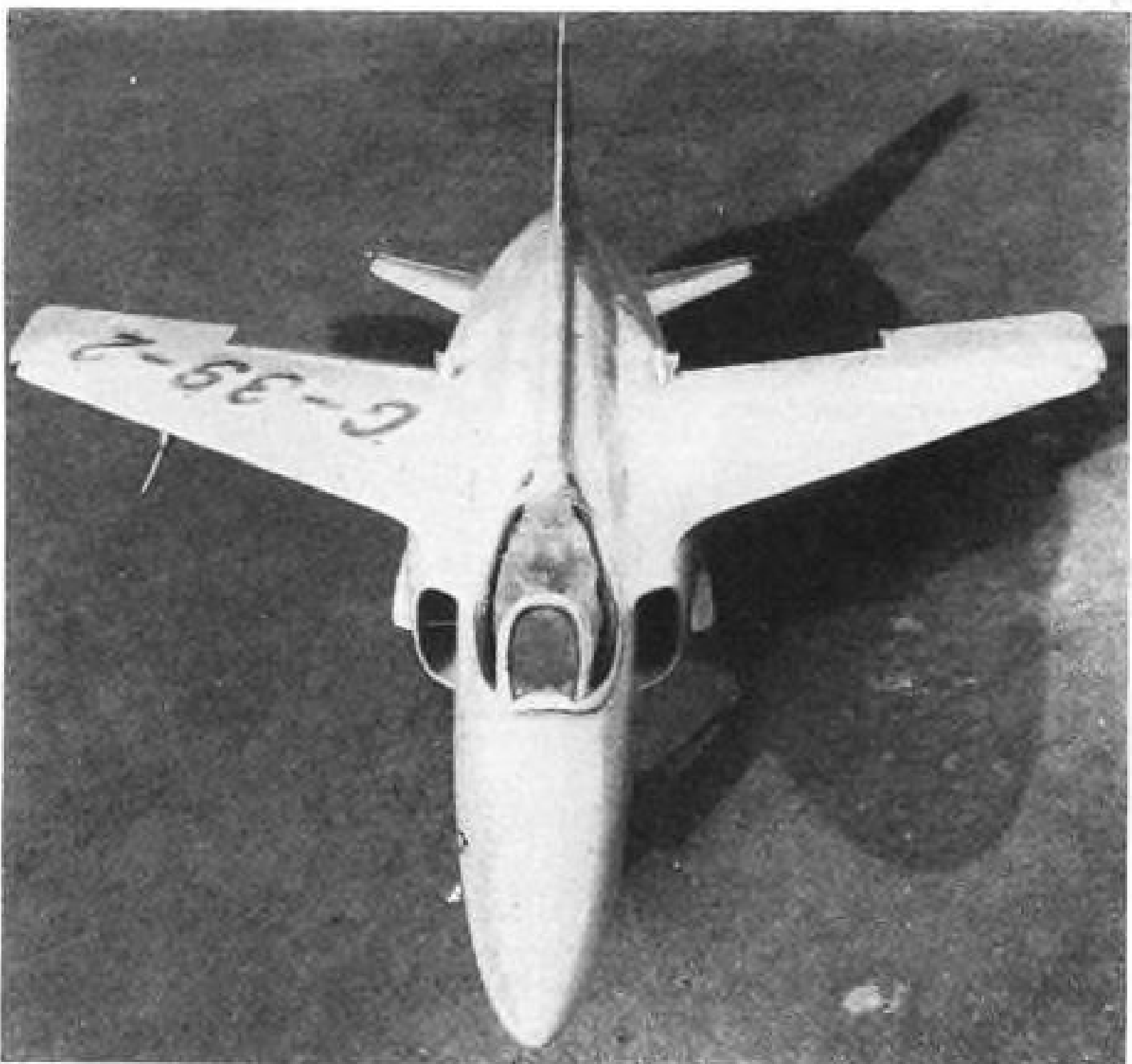
POWERED BY ORPHEUS jet engine, Gnat has been heralded by Folland as "the world's first successful light jet fighter." Plane is easily controllable right up to high-subsonic performance limit.
