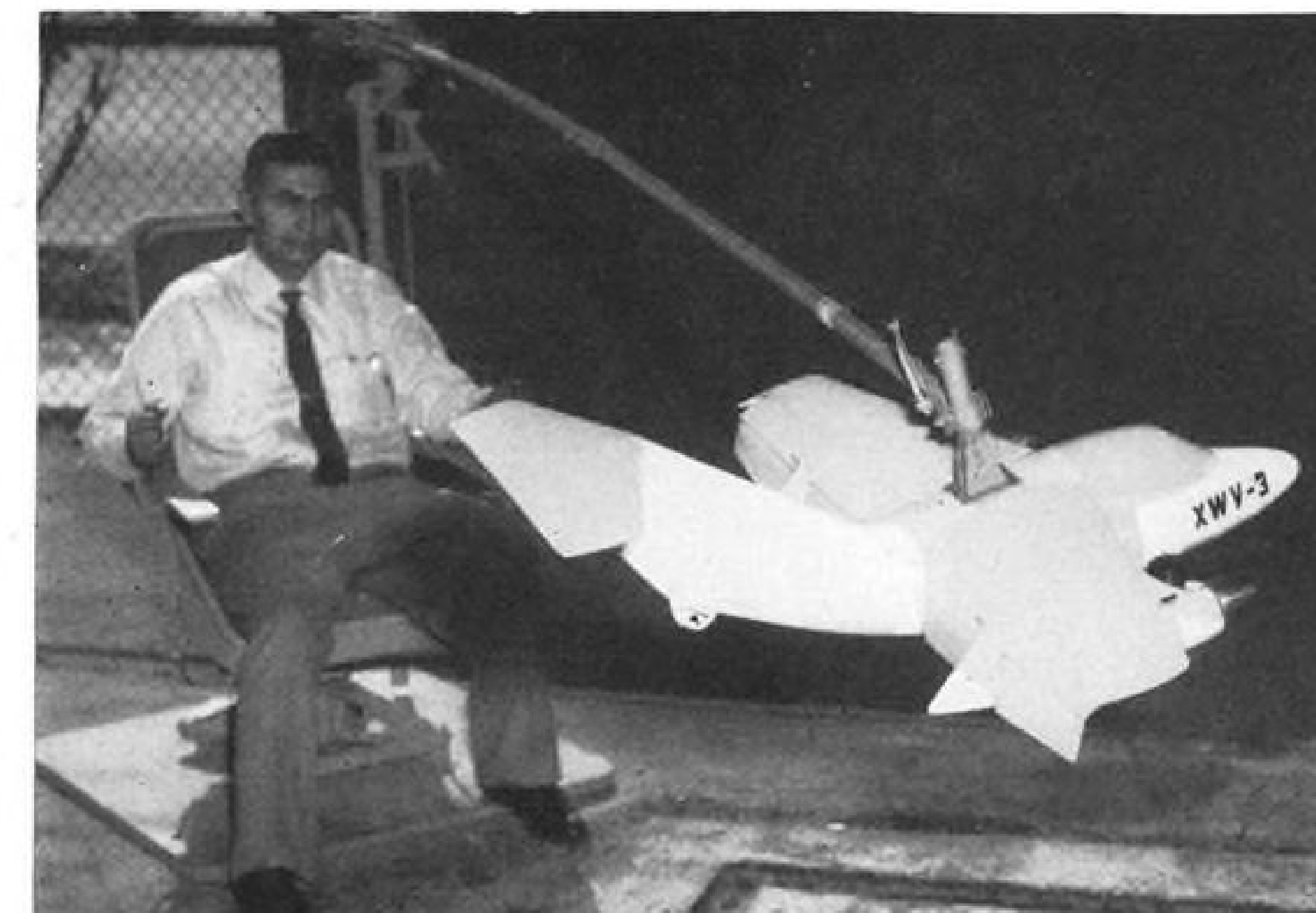
Puts his vertiplane model through paces. Note extended flaps for hovering.
