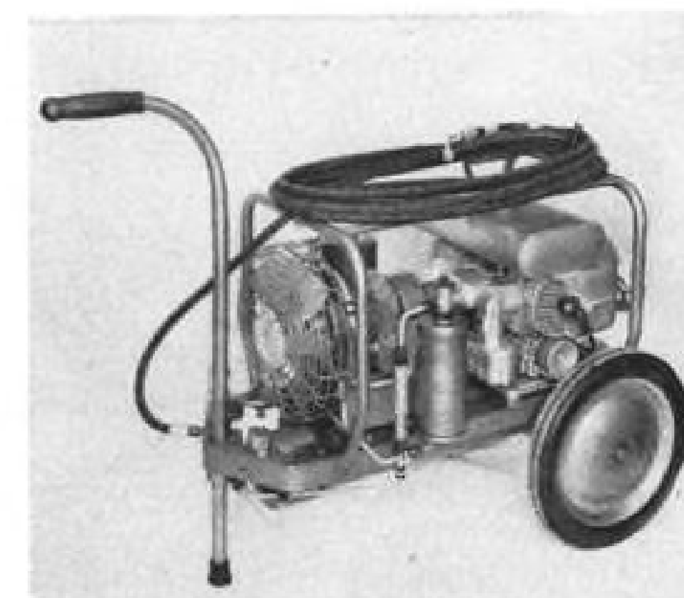
SPECIAL portable compressor designed for R.C.A.F. to service landing-gear struts.
