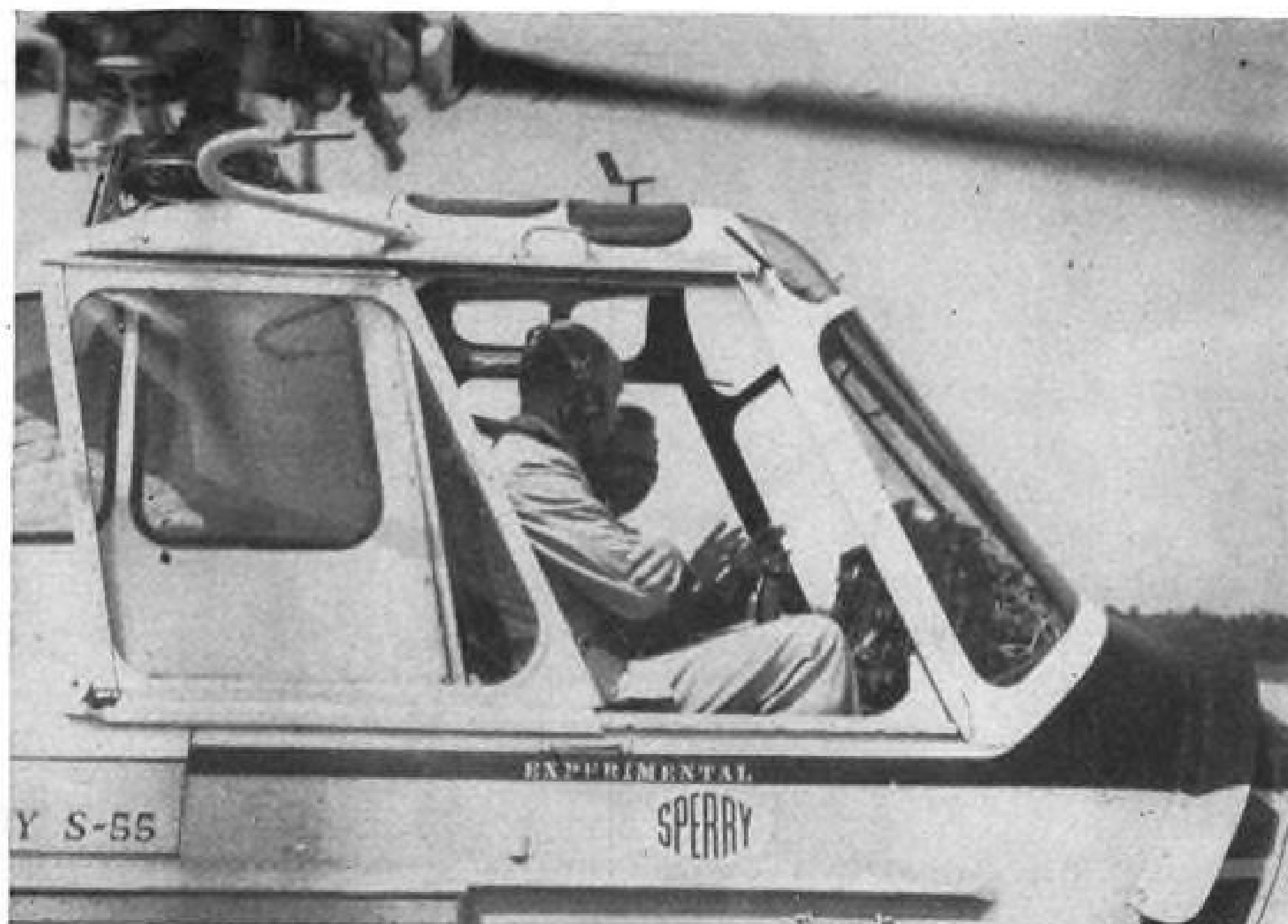
SPERRY flight-control unit hovers helicopter off ground. No hands are on controls.
