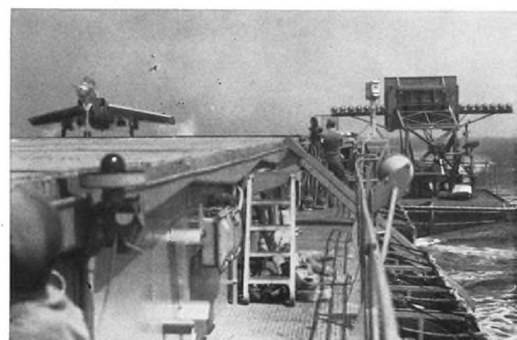
Gets first test as F7U-3 lands. Unit indicates glide path, altitude.
