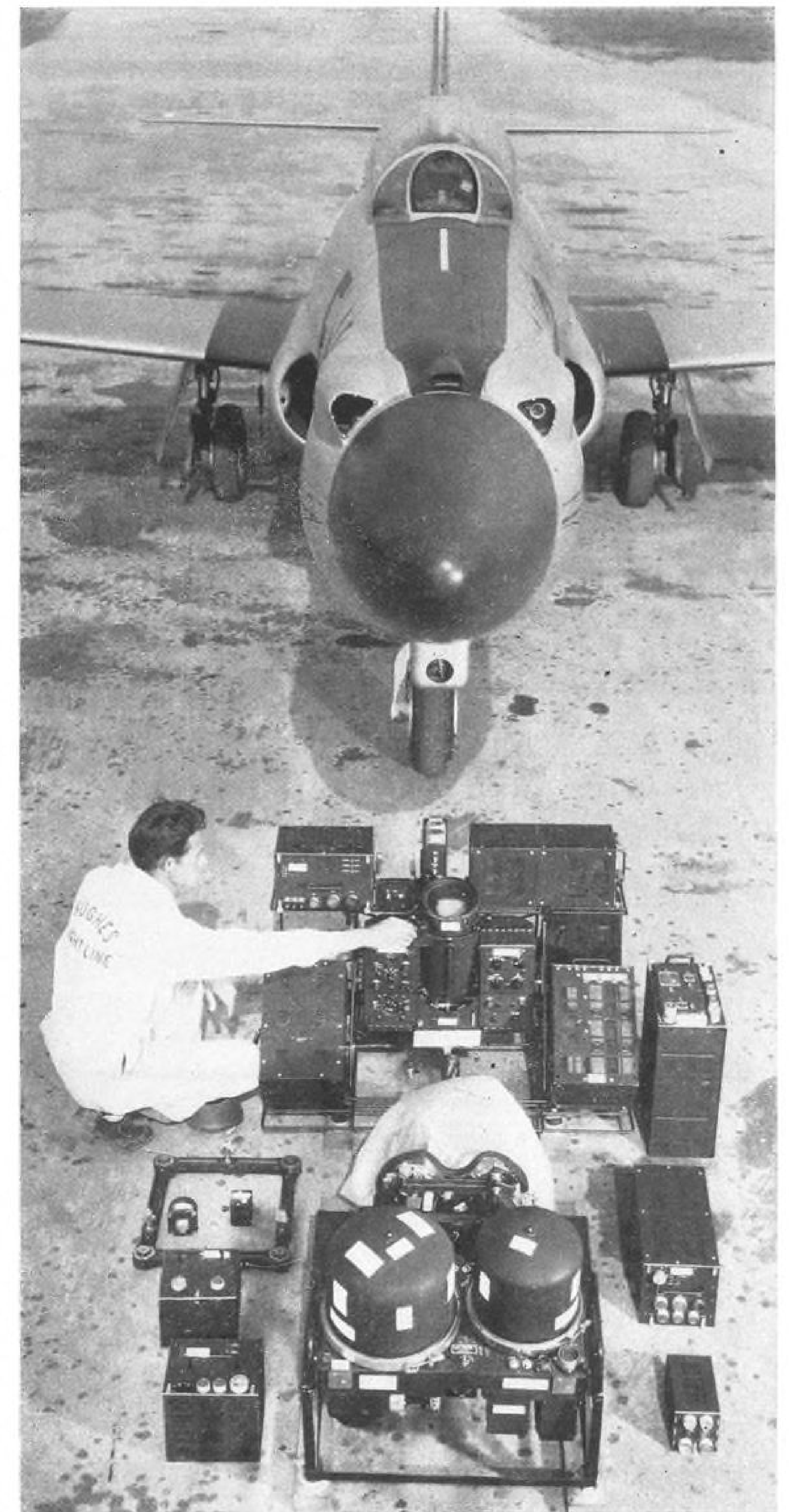
HUGHES FIRE CONTROL SYSTEM , enabling the F-86D to automatically locate and track down an enemy target by day or night, illustrates growing amount of avionics equipment aboard a modern interceptor. More advanced system is under development for F-102A.
