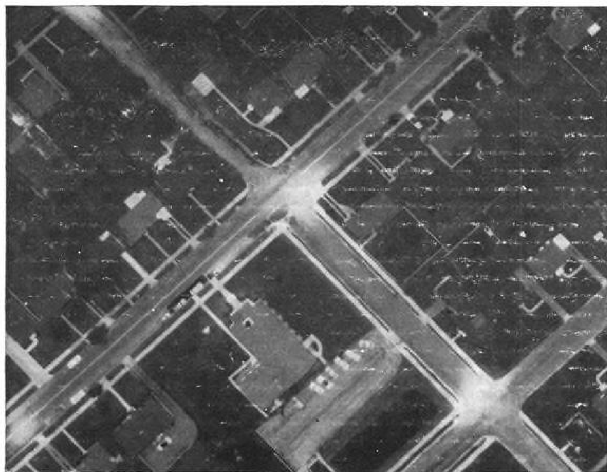
LOW-ALTITUDE night photograph of Dayton, Ohio, residential section. Only illumination used in the experiment was three mercury arc lamps mounted in nose of a C-47.
