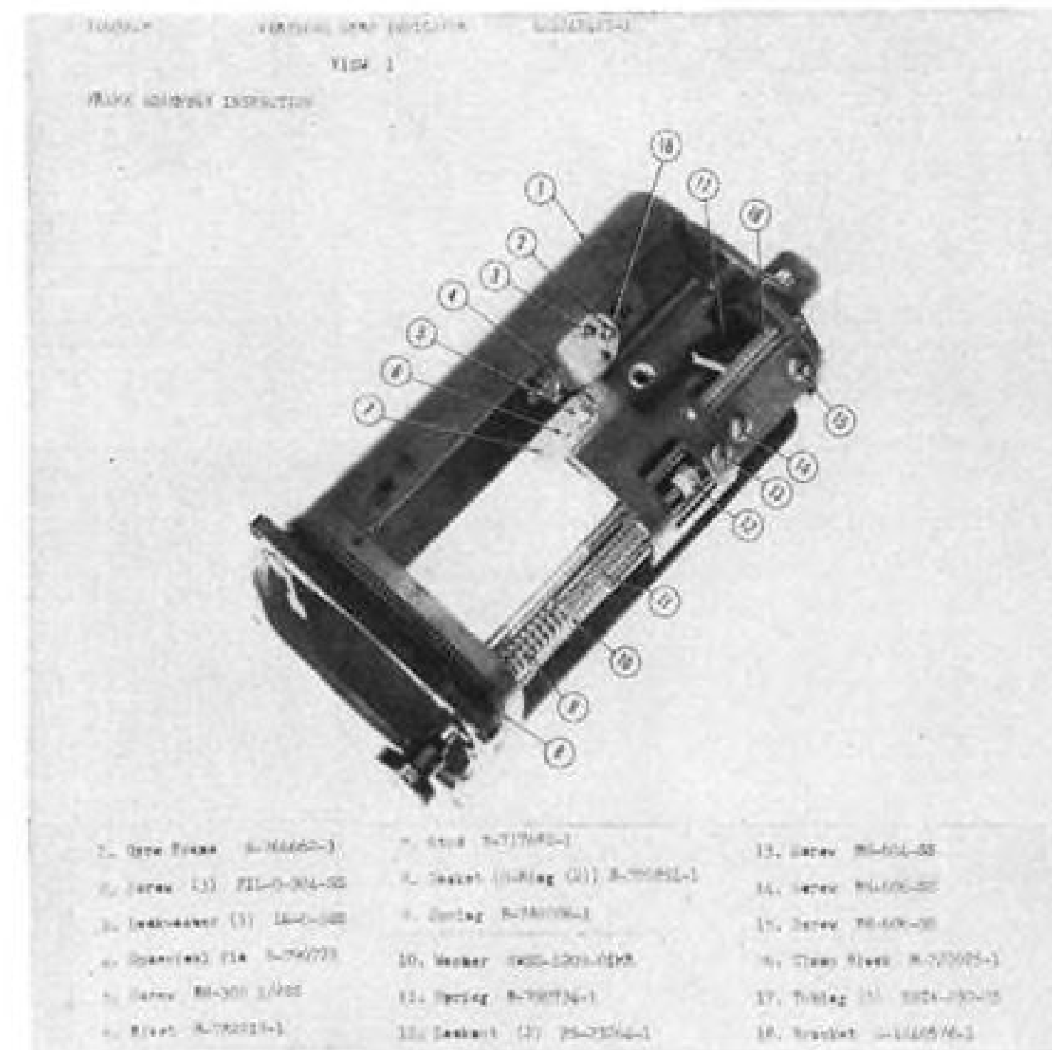
PICTORIAL INSPECTION —Assembly is checked against labeled picture and instruction sheet; typical picture sheet shown at right.
