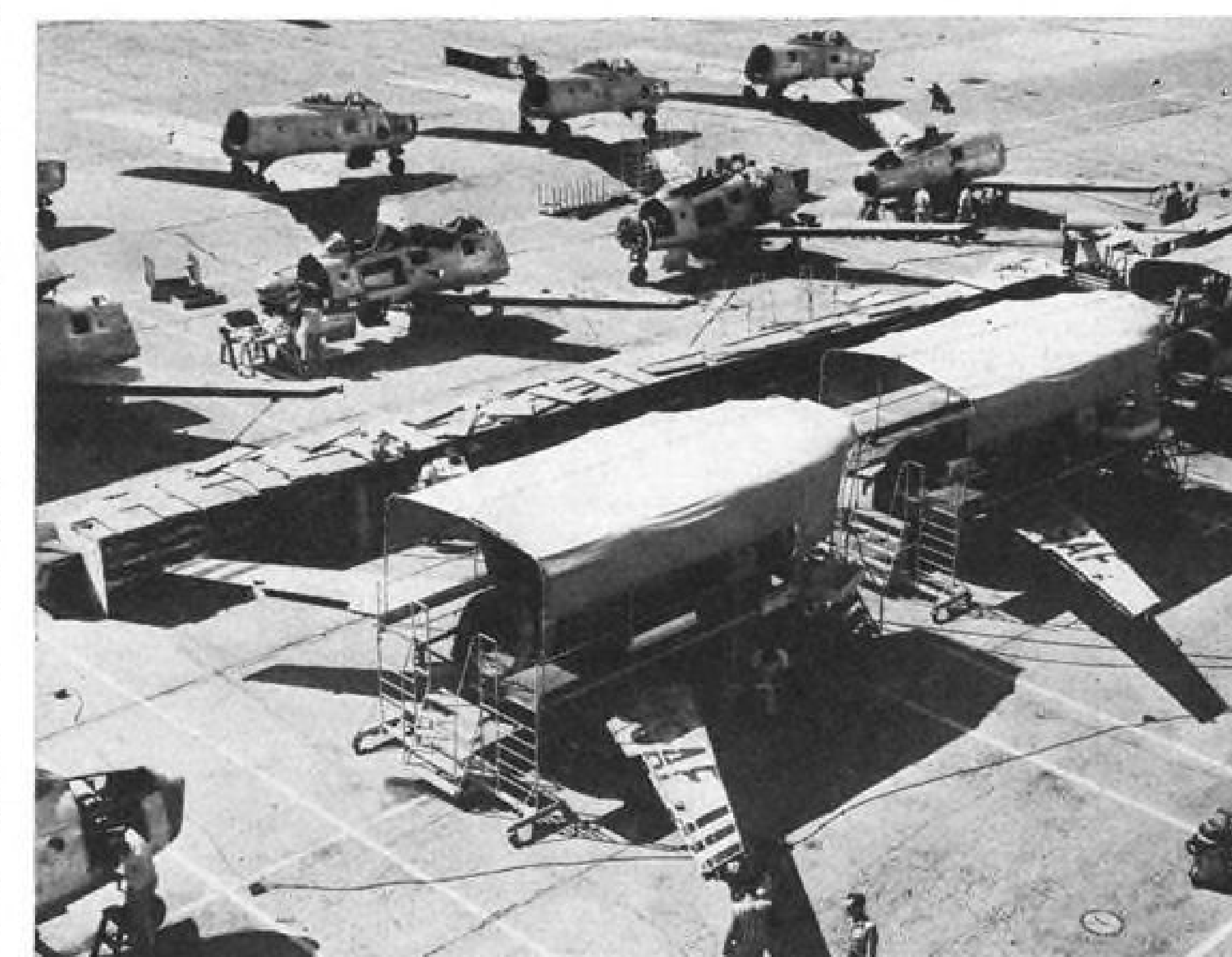
SERVICE-WORN F-86's are modified and modernized at North American Aviation's Fresno, Calif., Division. Following complete teardown, the plane's are brought up to latest service standards. Shelters in foreground protect workers from hot sun during the work.
