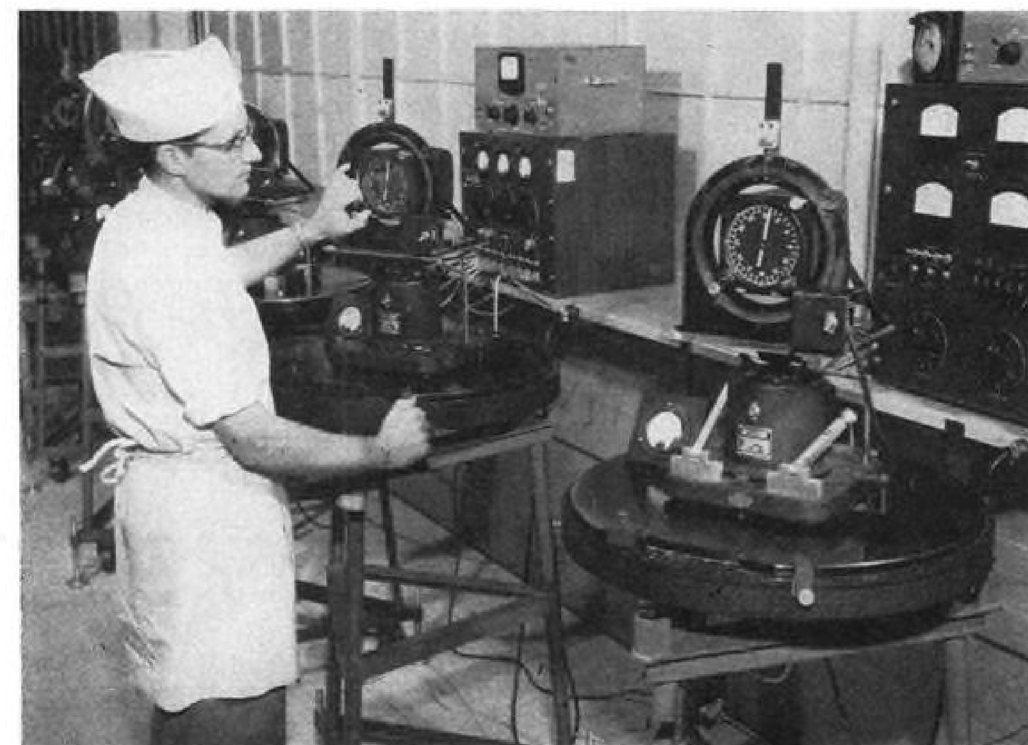
GYROSCOPE is adjusted during routine run-in on Scorsby stand before shipment.
