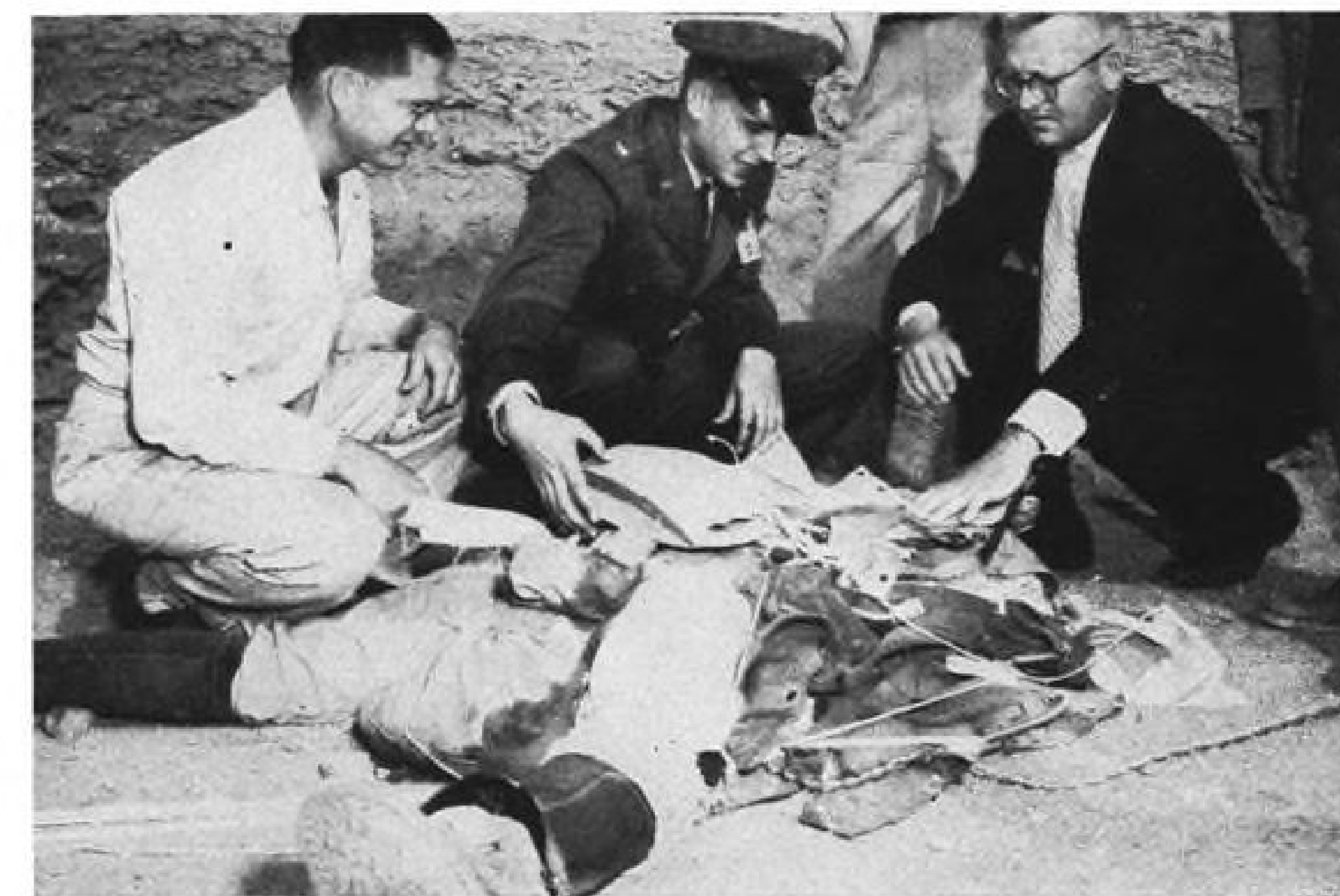
DEAD DUMMY is examined after ejection test simulating supersonic bailout.
