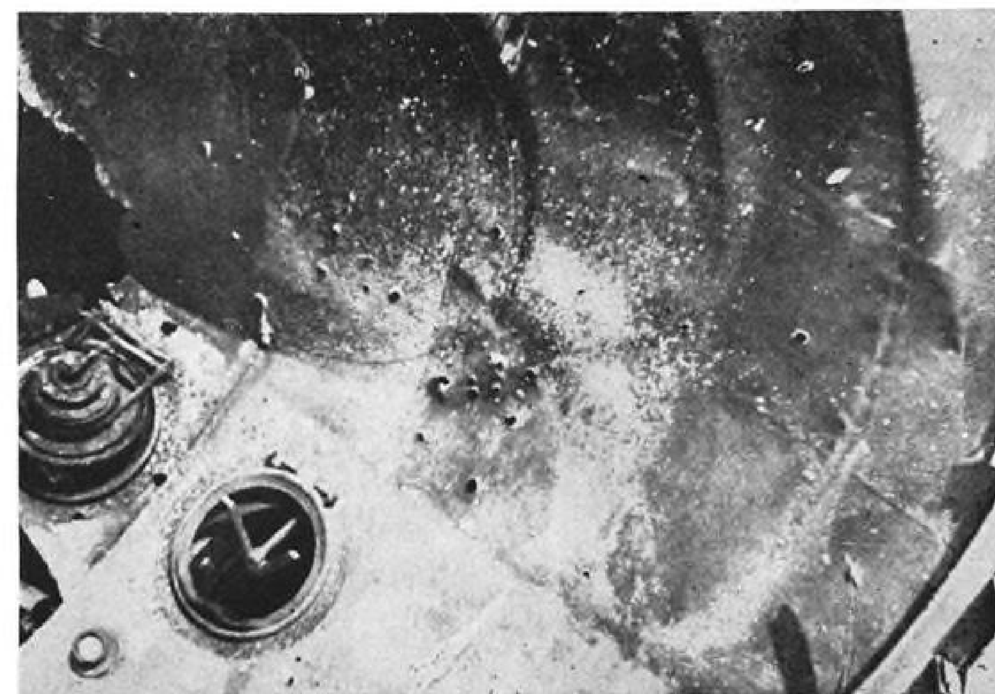
REAR PRESSURE BULKHEAD of El Al Israel Constellation had been sprayed by bullets.
