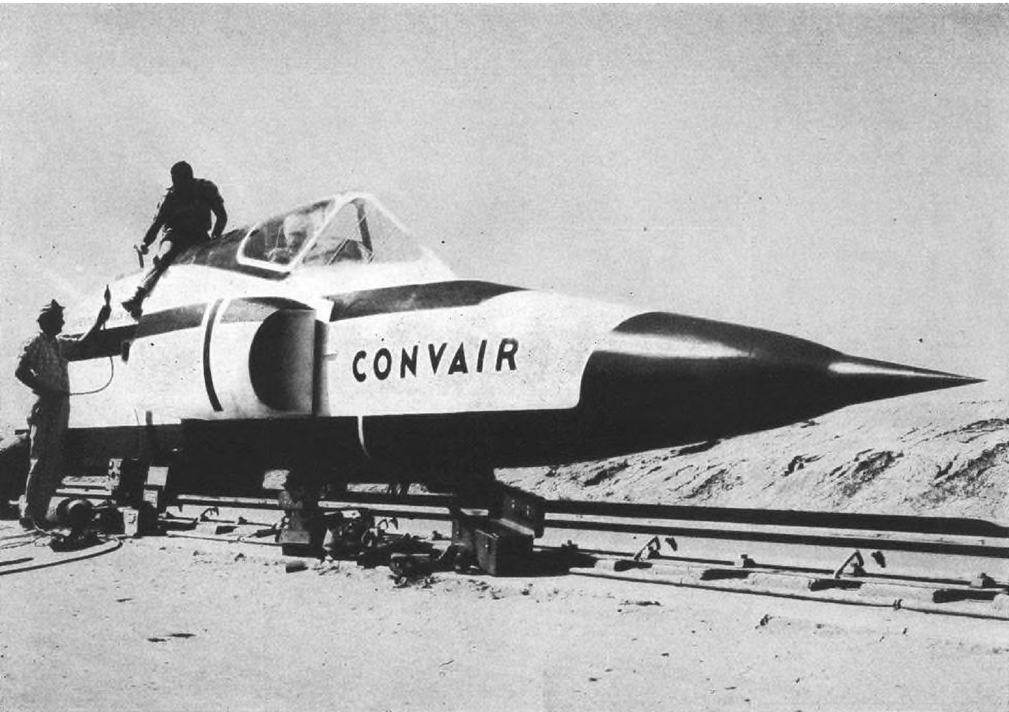
CONVAIR F-102A escape system is checked out before highspeed test of dummy pilot ejection and seat separation.
