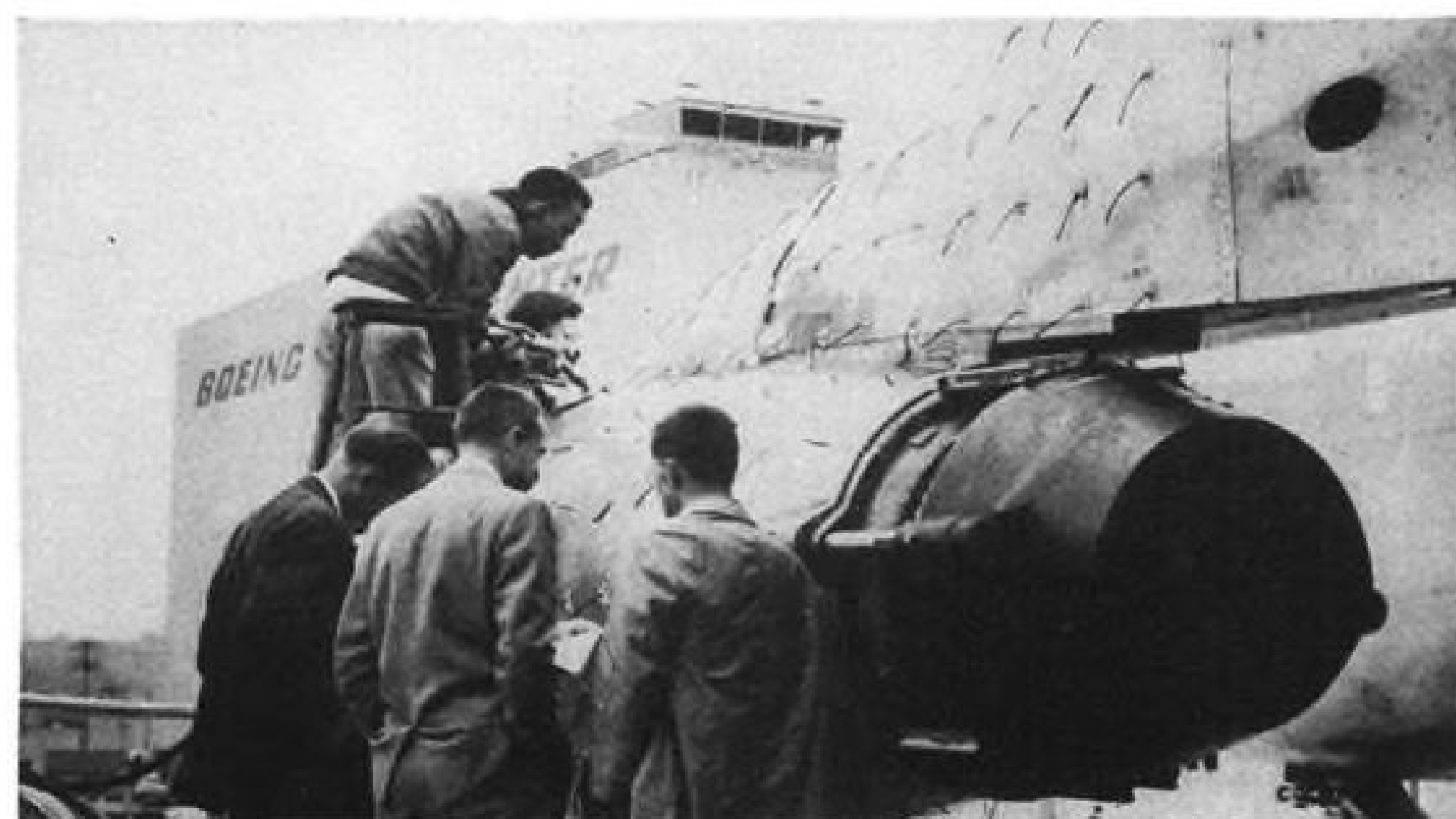
THRUST REVERSER-NOISE SUPPRESSOR produced by Boeing is, the Port of New York Authority believes, the first step in the right direction. Pictured above is an experimental reverser which has been taxi-tested on the 707 prototype at 98 mph.
