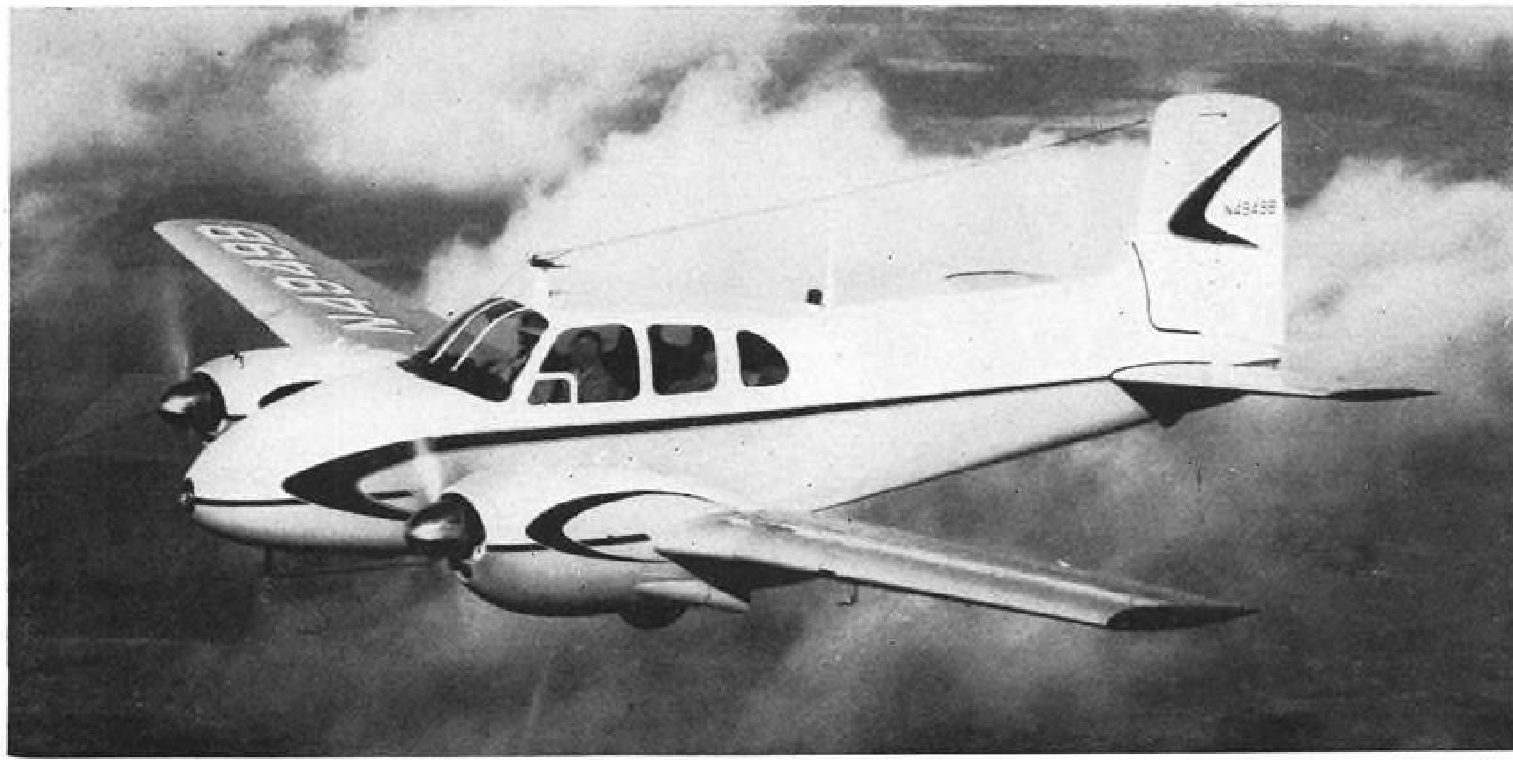
TWO TWIN-BONANZA MODELS will be available in 1956. The newest, the D50, has 295-hp. Lycomings turning three-blade propellers.
