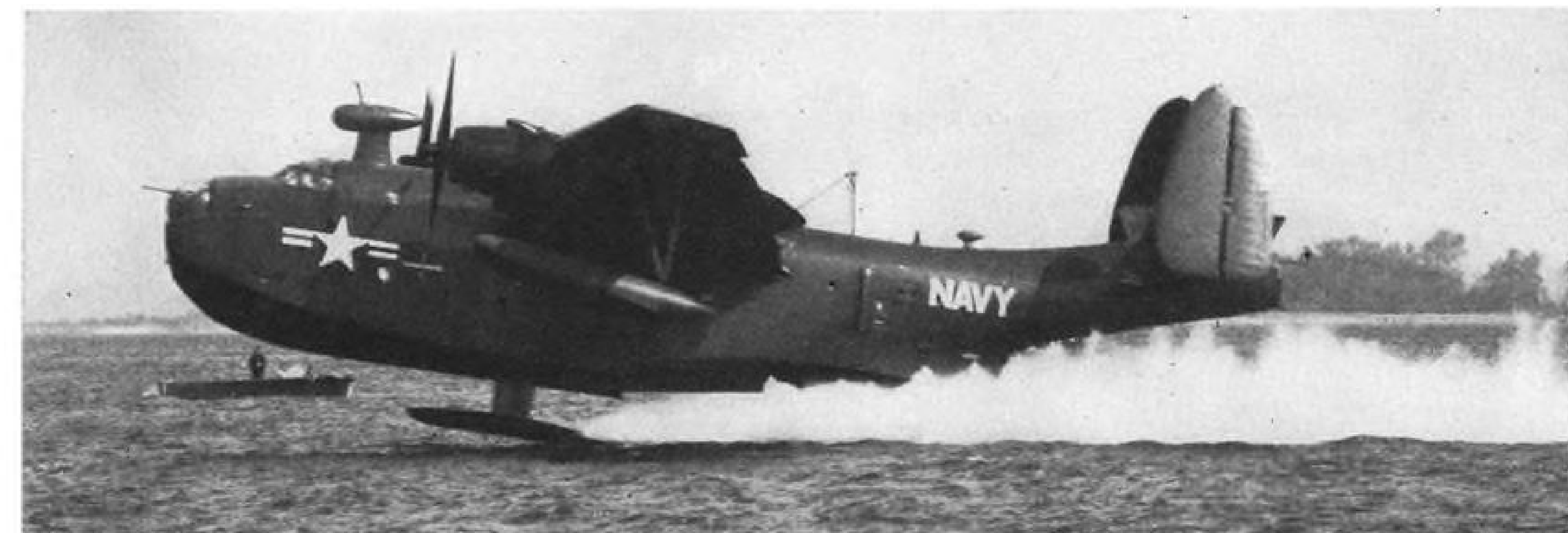
MARTIN PBM MARINER (above) goes through tests to determine whether hydro-skis will be installed on future production models.
