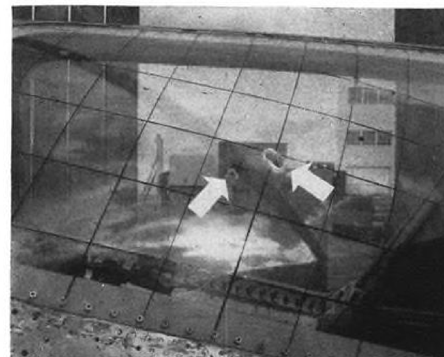
GUNFIRE TESTS produced small bullet holes in stretched plastic F-102 panel (arrows, left) but shattered "as cast" canopy (right).
