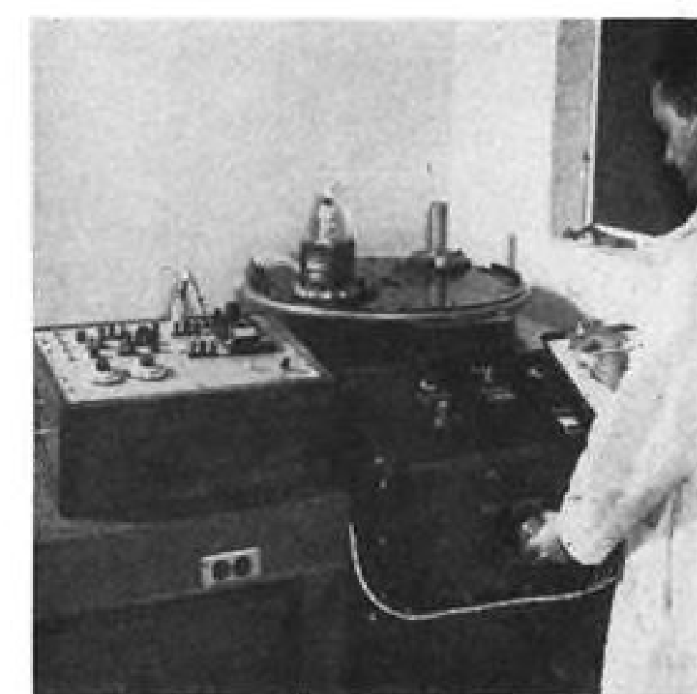
RATE-OF-TURN table used for precision calibration of accelerometers and gyros.
