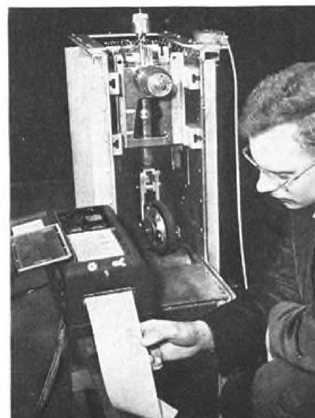
MODEL for nose-wheel shimmy tests.
