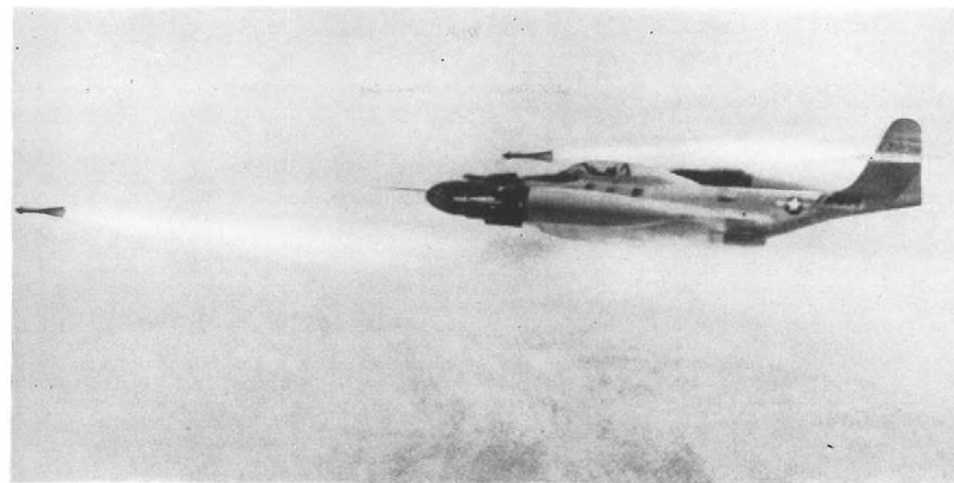
Northrop Aircraft, Inc., last week unveiled its new F-89H Scorpion (above and at left below), first operational aircraft to carry Hughes Falcon air-to-air guided missiles as part of its standard equipment. In each of its wingtip pods, the F-89H carries three Falcons plus a packet of folding-fin, non-guided rockets. When ready for firing, below left, the Falcon missiles are extended from the sides of the pods for launching. The test program included Falcon firings from both wing pods and pylons (below and left above).
