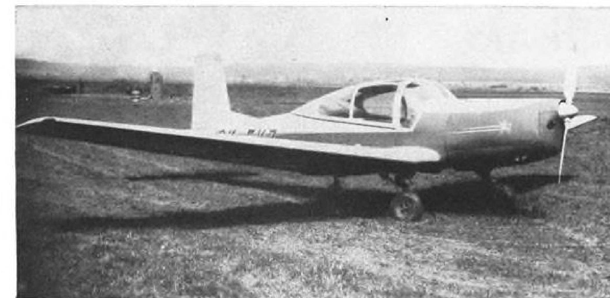
LD-40 three-seater has unusual "reverse tricycle" landing gear with tailwheel under cabin.
