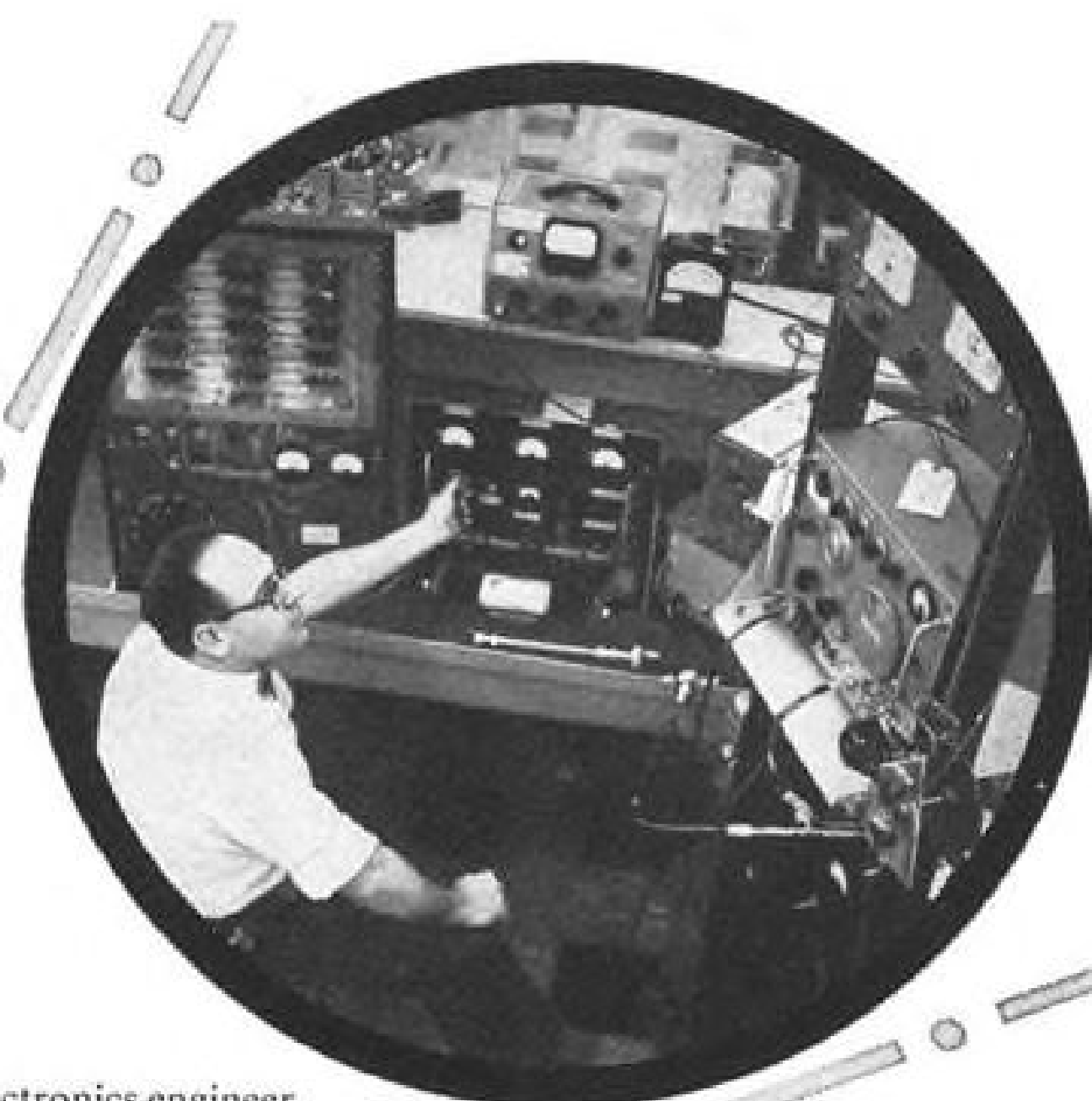
Carl Cutler, electronics engineer, testing a traveling wave tube at the Waltham Laboratories.
