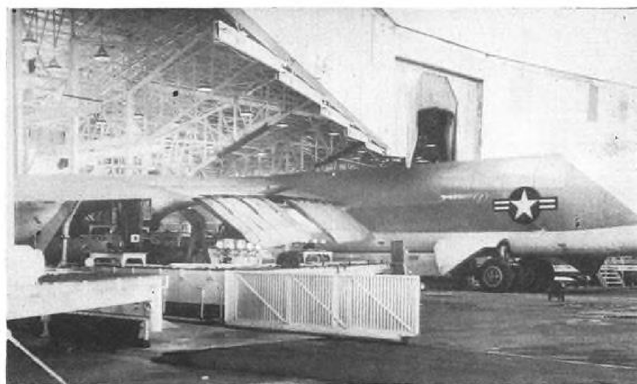
B-52, note wing-flap size, undergoes flight-line maintenance in Castle AFB nose dock.
