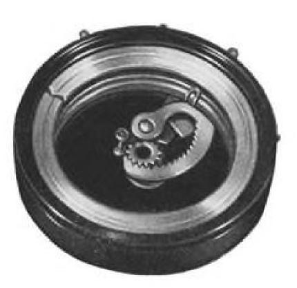
This is a cam characterized potentiometer, one of several in Honeywell's advanced MB-3 Autopilot. By scheduling circuit gains as functions of the basic flight control parameters, these Honeywell-made precision potentiometers help make the aircraft behave at supersonic speeds. The pilot gets the aeronautical equivalent of power steering: he applies the same stick force for a given maneuver, regardless of the aircraft's speed or altitude.
