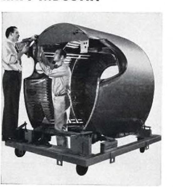
TITANIUM can save hundreds of pounds per plane. Its lightweight and high strength factors plus an outstanding resistance to corrosion make it an extremely attractive metal for use in nacelle construction, firewalls, frames, etc. Republic produces titanium and titanium alloys in hot rolled and cold drawn bars, sheets, plates and billets.
