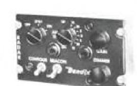
CON-1D CONTROL UNIT For remote control of RDR-1 AIR-BORNE RADAR SYSTEM (except for controls located on indicator face). Incorporates Bendix DA-
