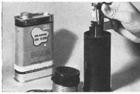
By retaining a practically consistent viscosity from room temperature to bottomhole temperatures ranging up to 400 F. 200 Fluid helps to keep Halliburton's drift-angle and direction-survey tool accurate within half a degree at angles up to 13°.
