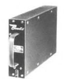
MKA-7A MARKER RECEIVER New ¼ ATR, 75 mc. marker receiver weighs only 8.5 pounds with power supply. Improved circuitry greatly reduces possibility of FM or TV interference. Designed for reception of airways and ILS approach markers.
