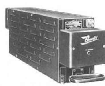
MN-85F VHF NAVIGATION RECEIVER Provides visual and aural reception of all VHF navigation aids including localizer. 280 crystal controlled channels, spaced 100 kilocycles apart from 108.0 to 135.95 mc.
