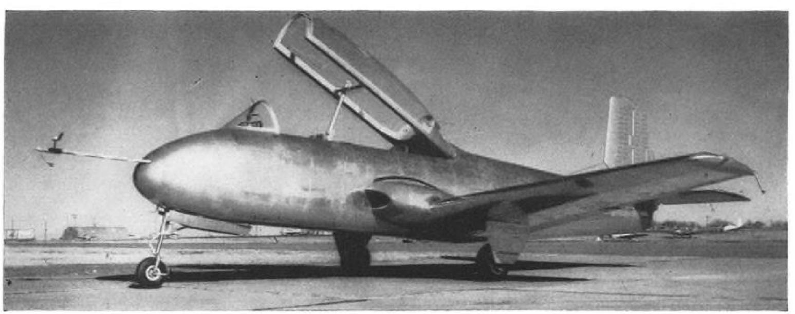
CLAM-SHELL CANOPY covering both cockpits is power-actuated. Beech has tested lightweight ejection seats should customer want them.
