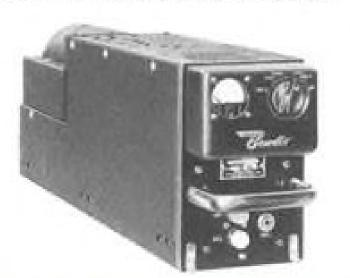
TA-20A VHF COMMUNICATIONS TRANS-MITTER 360 crystal controlled channels from 118.0 to 135.95 mc. 50-kilocycle channel spacing. Provides 30 watts of r-f output power. Built-in meter and switch permits checking currents in six major circuits.
