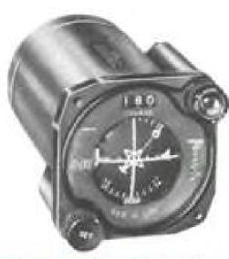
MN-97H OMNI-MAG Visual reception of VOR, ILS and relative magnetic heading information in a single instrument. Optional features include standard or expanded range movement (vertical bar), matte white or radium lettering.
