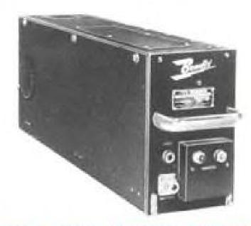
RA-18C-1 VHF COMMUNICATIONS RE-CEIVER Provides 360 crystal controlled channels from 118.0 to 135.95 mc. 50-kilocycle channel spacing. 3-microvolt sensitivity. Carrier operated squelch control.
