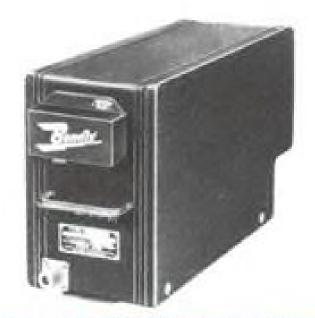
MN-100A GLIDE SLOPE RECEIVER 20 crystal controlled channels from 329.3 to 335.0 mc. for reception of tone-modulated 90/150 cps. glide slope information. Control panel may be wired for simultaneous frequency selection of localizer and Glide Slope.
