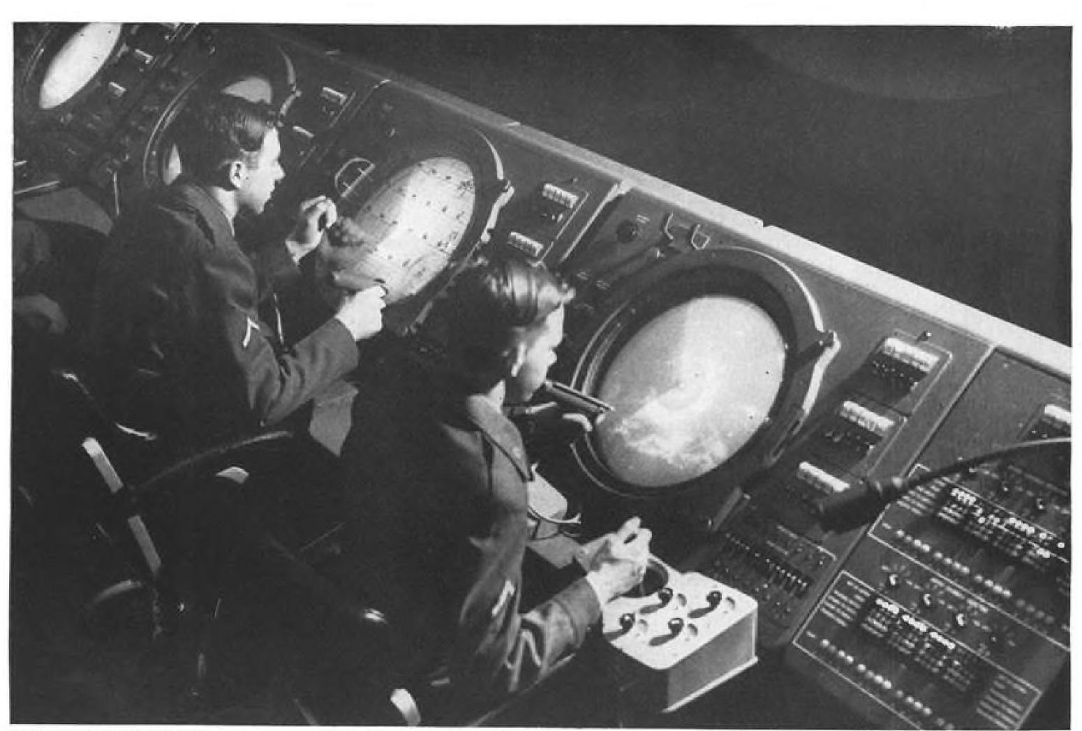
ELECTRONIC CONSOLES are heart of Missile Master System. Operators enter targets on tracking screens with photo-electric guns.
