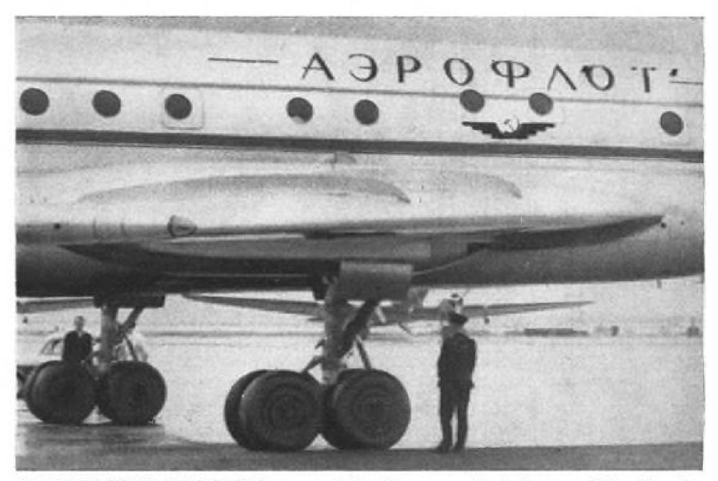
SEPARATE WING NACELLES house main landing gear; wheels have a 42-in. diameter.
