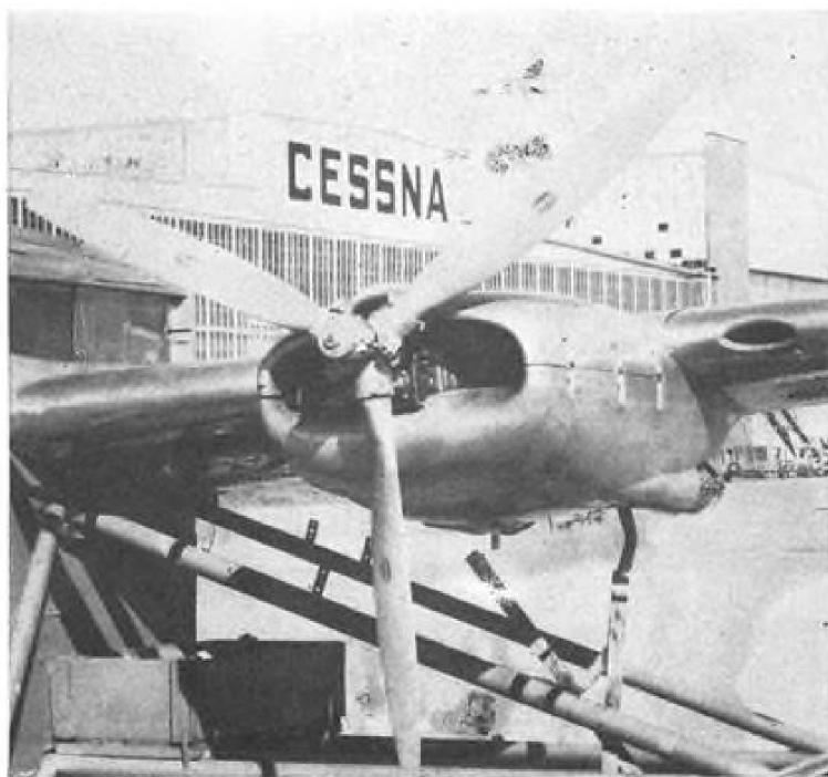
WING (left) fitted with tip tanks and engine nacelles, nears end of tests. Engine and cowl mockup (right) is tested outdoors.
