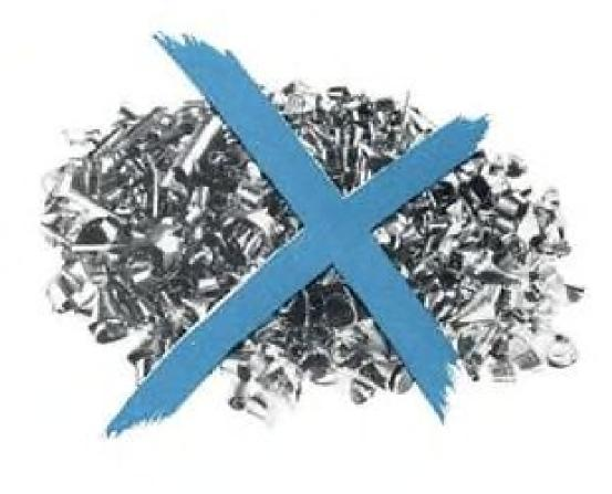
This is the old way of making an aileron actuator attach fitting . . . machining it from aluminum billet stock. It has three drawbacks. First, it adds many hours to plane construction time . . . second, it requires specialized, expensive machinery ... third, it can waste up to 90% of the metal.
