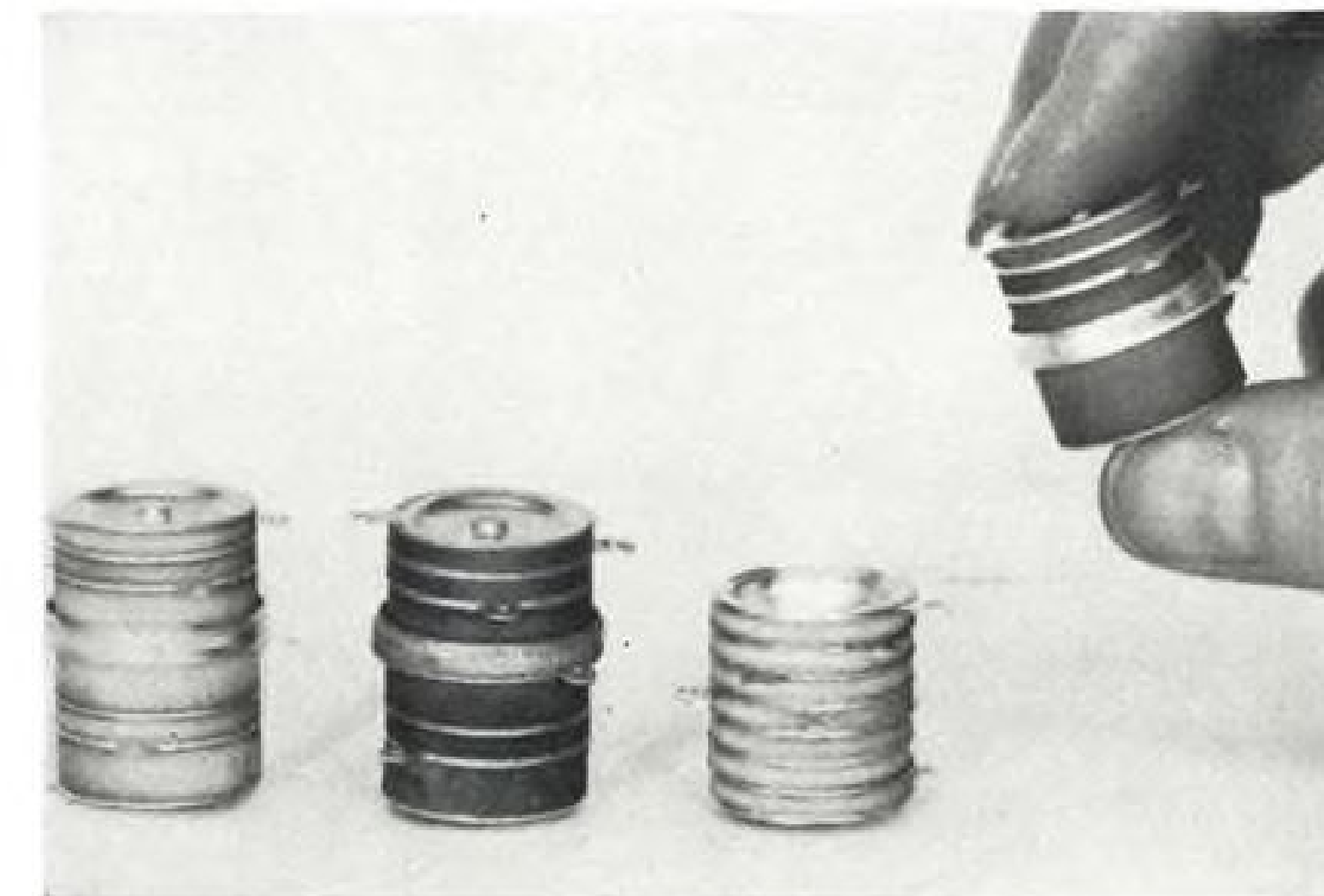
FOUR TYPES of Eimac stacked ceramic tubes which were developed especially for new aircraft and missiles.
