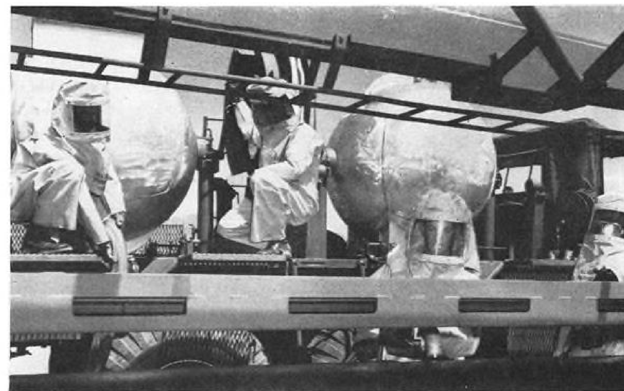
MEN OF THE 601ST Missile Battalion, Ft. Bliss, Tex., dressed in special acid resistant suits made of Polyethylene, during fueling of Corporal.
