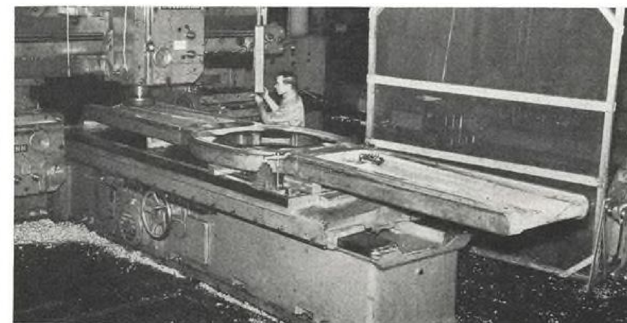
PLANING IS FIRST machining operation on this 2,500-lb. 75 S aluminum forging for the wing spar of a modified Martin B-57 bomber. Excess material is removed in this step.
