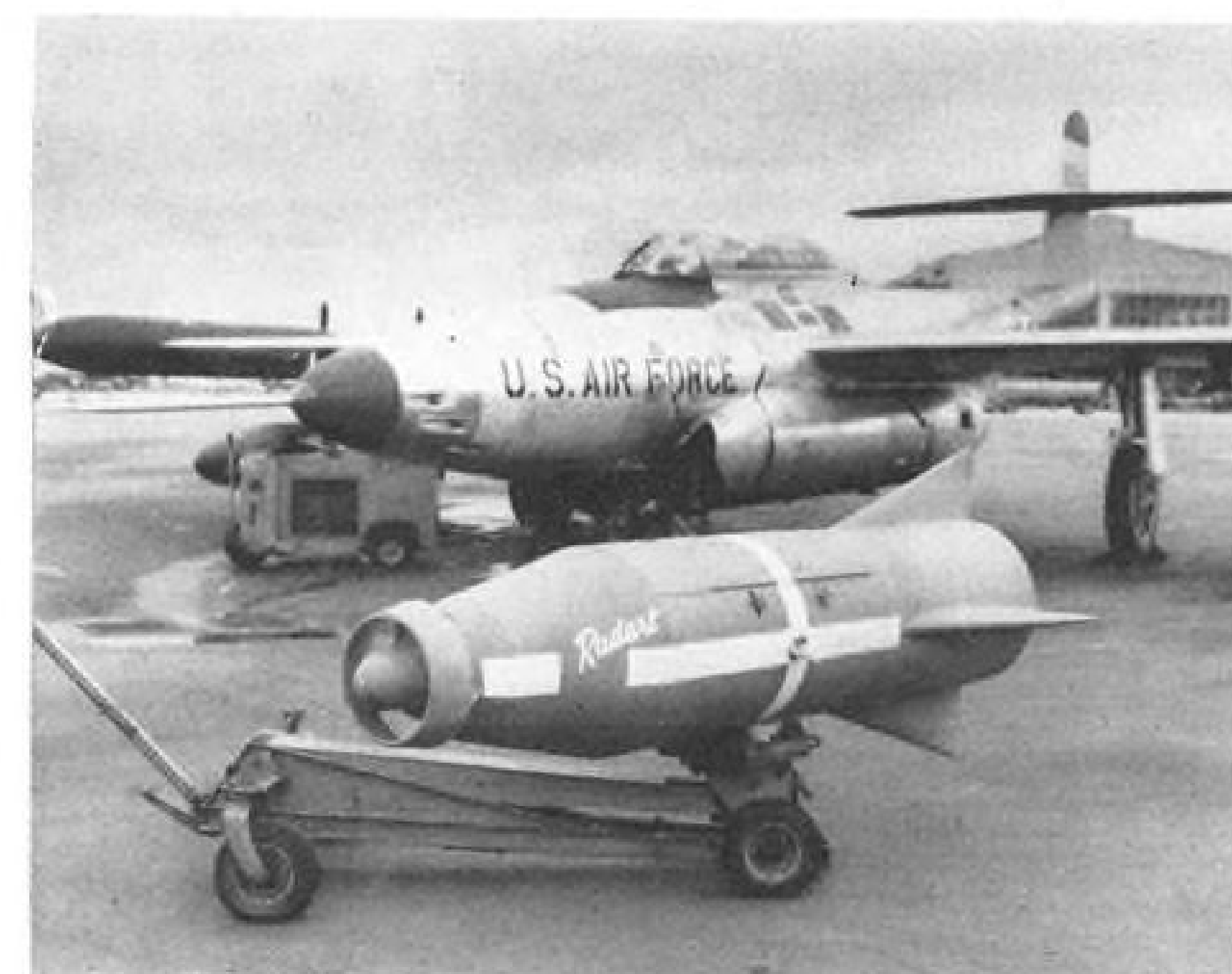
TOW TARGETS: FLUIDYNE RADART (LEFT) AND DEL MAR'S FRANGIBLE RADOP.
