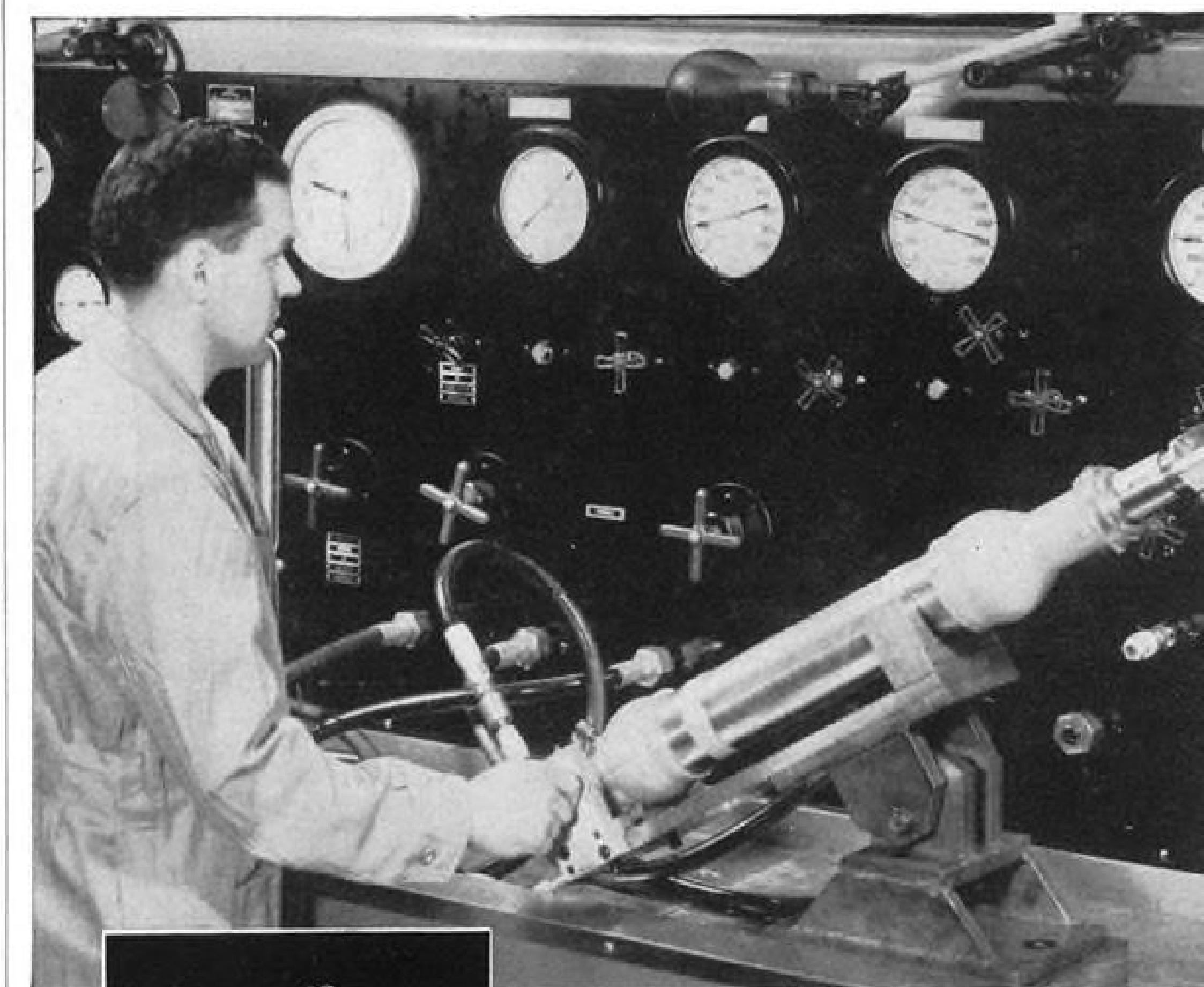
This test stand checks actuating assemblies under simulated operating conditions.
