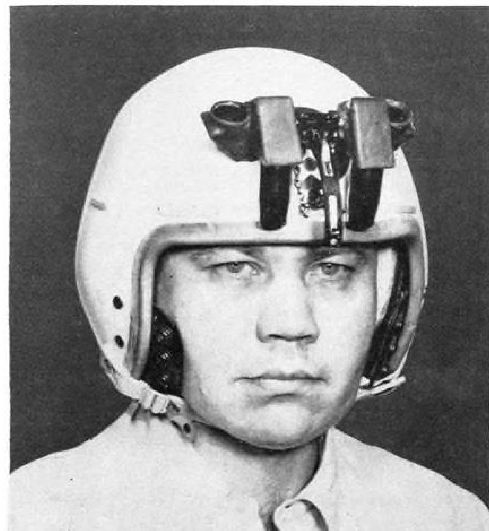
HELMET binoculars compensate for fast jet closing rates.
