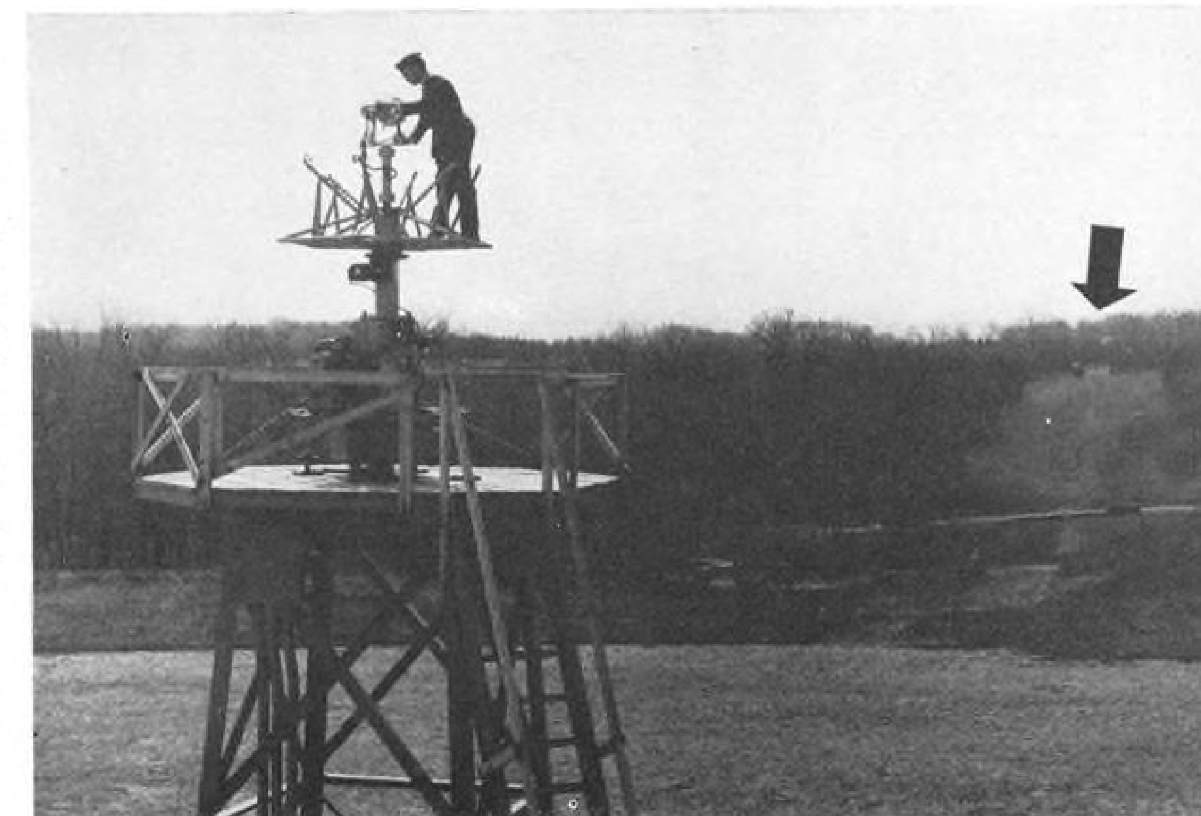
ELECTRONIC COMPONENTS LAB'S RANGE WILL TEST NEW RADOME MATERIALS.
