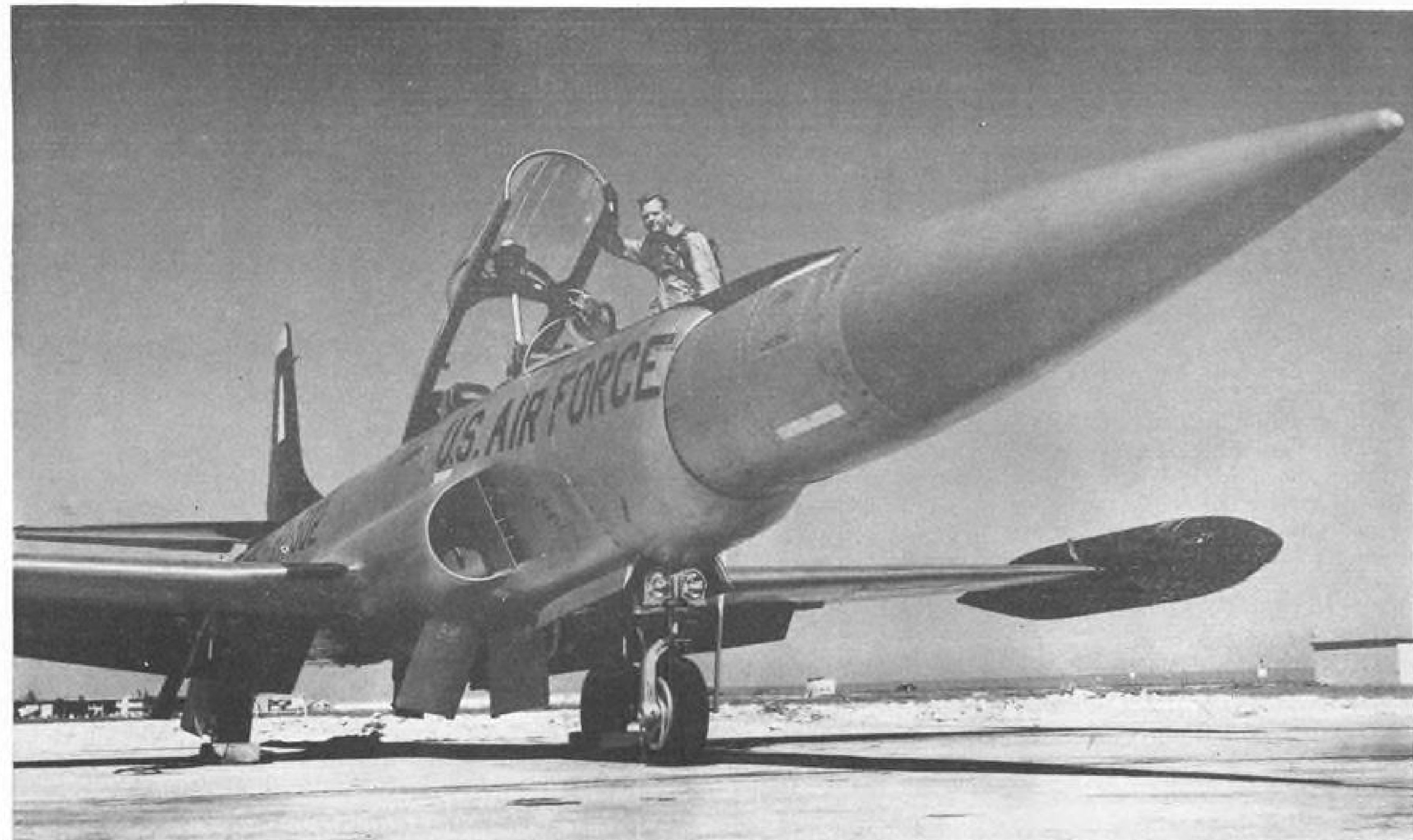
SPECIAL RADOME ON F-94C TESTS AND EVALUATES MISSILE COMPONENTS
