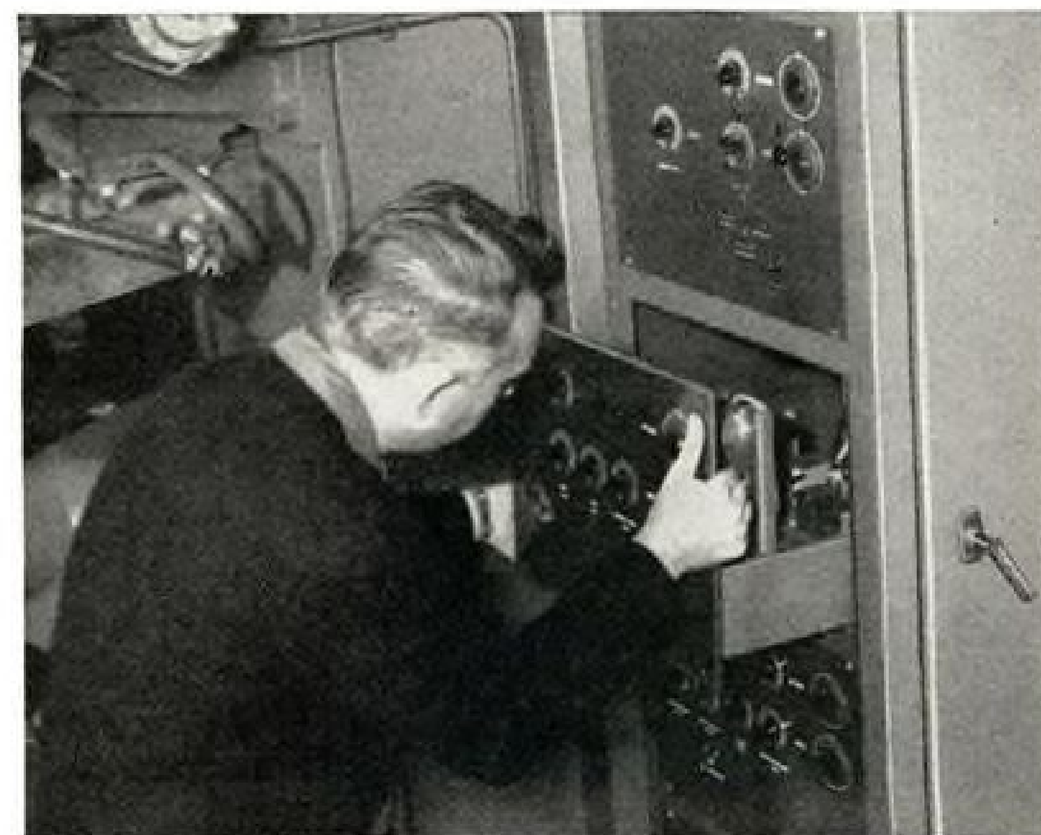
Note the ease with which a plug-in new function unit can be added.
