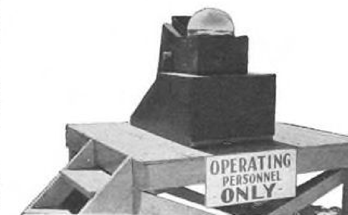
FULL SKY recording camera takes picture every 15 min. of complete sky as reflected in a 12-in. glass sphere.
