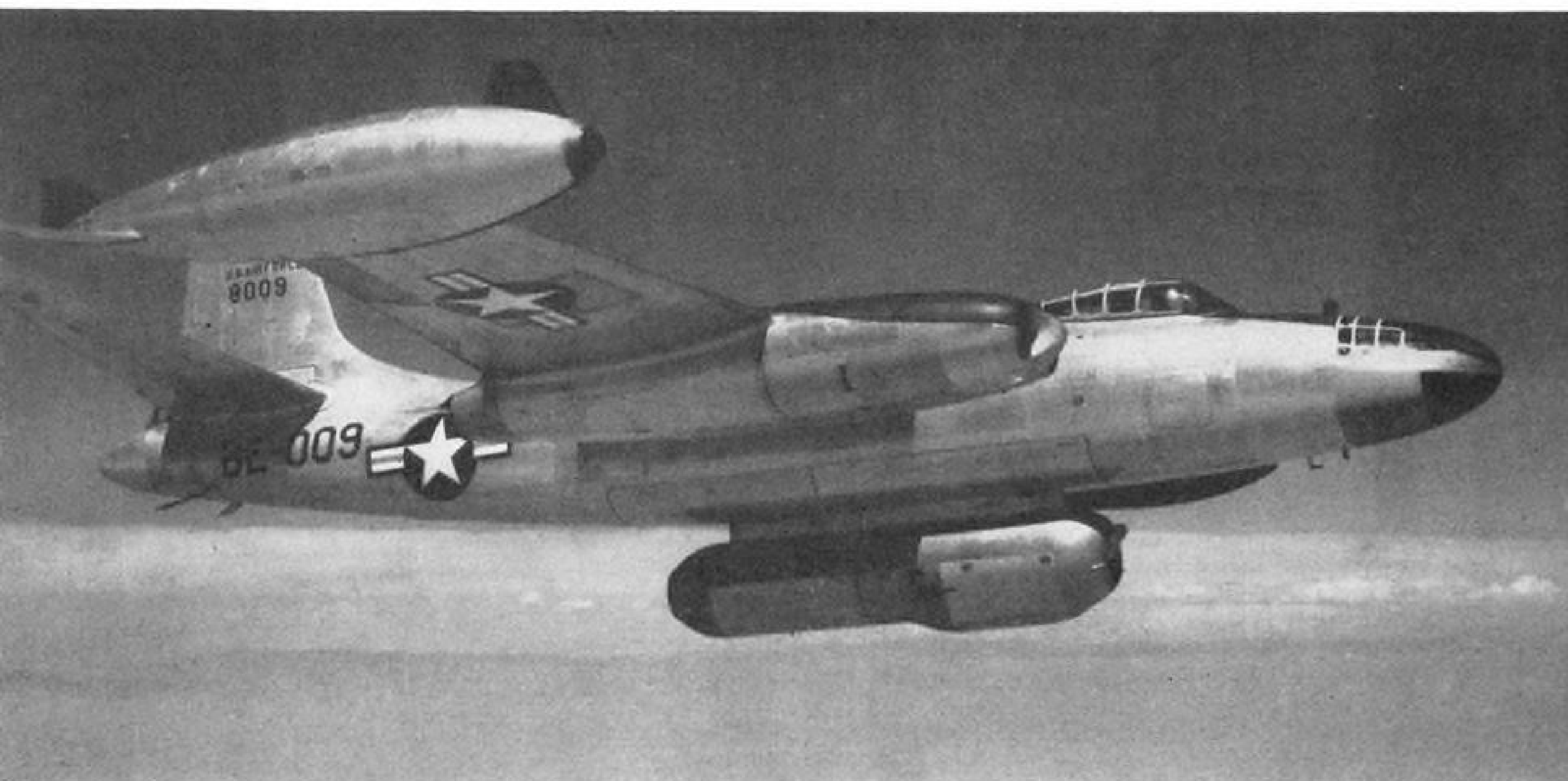
B-45A TORNADO IS TESTBED FOR JET ENGINES
