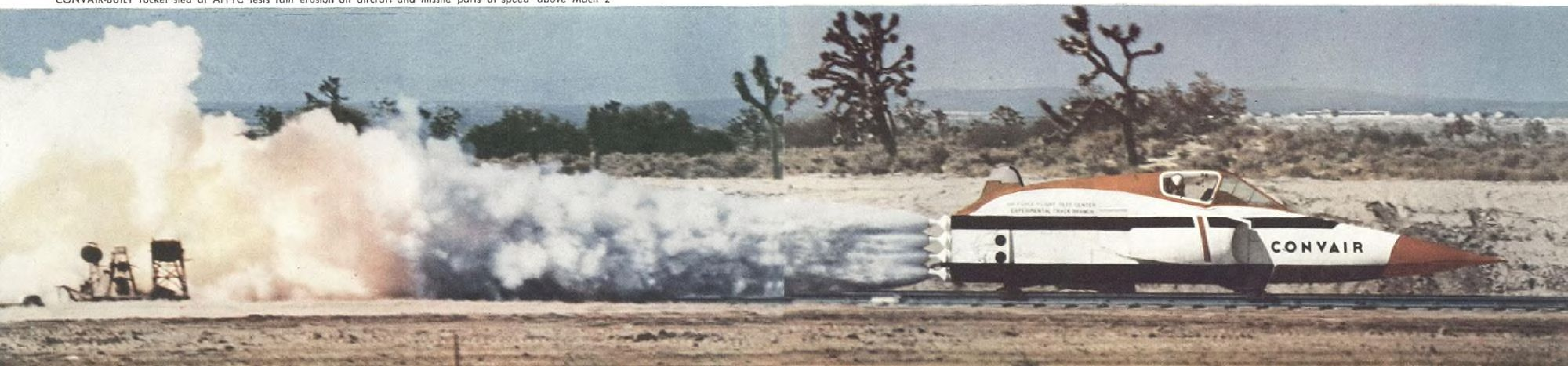
CONVAIR-BUILT rocket sled at AFFTC tests rain erosion on aircraft and missile parts at speed above Mach 2
