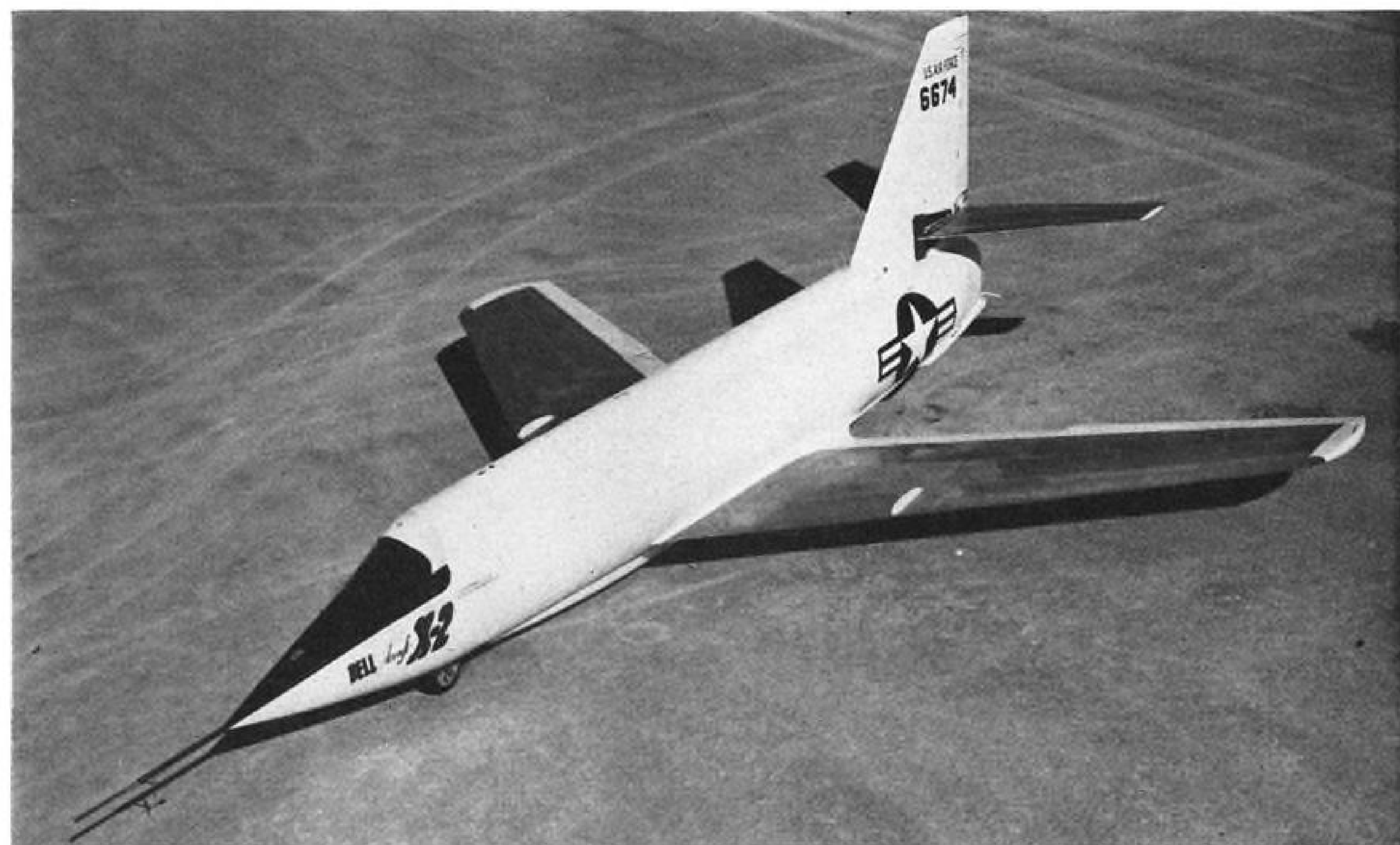
STAINLESS STEEL is the material from which Bell X-2 wing and tail are fabricated. Other X-2 pictures are on pages 72-73.
