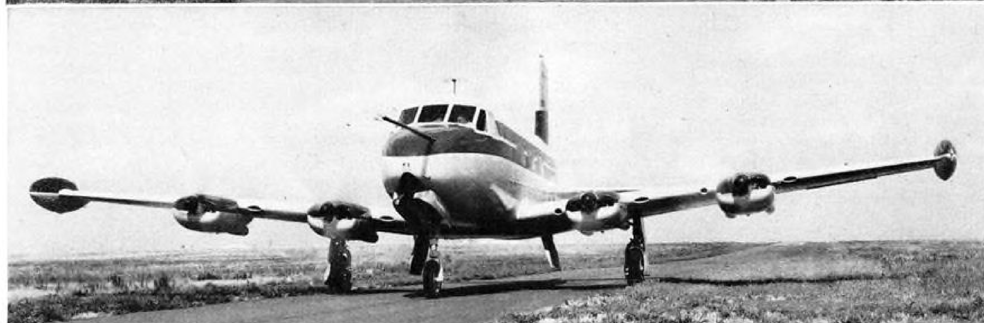
PROTOTYPE of Cessna Model 620 with the four Continental GSO526-A engines running. Powerplants, rated at 320 hp. takeoff, are mounted in underslung nacelles for maintenance accessibility. The airplane is on a taxi strip at Cessna's Pawnee plant, which is adjacent to McConnell Air Force Base, Wichita, Kans. First flight of the pressurized executive transport will be made at the Air Force base.
