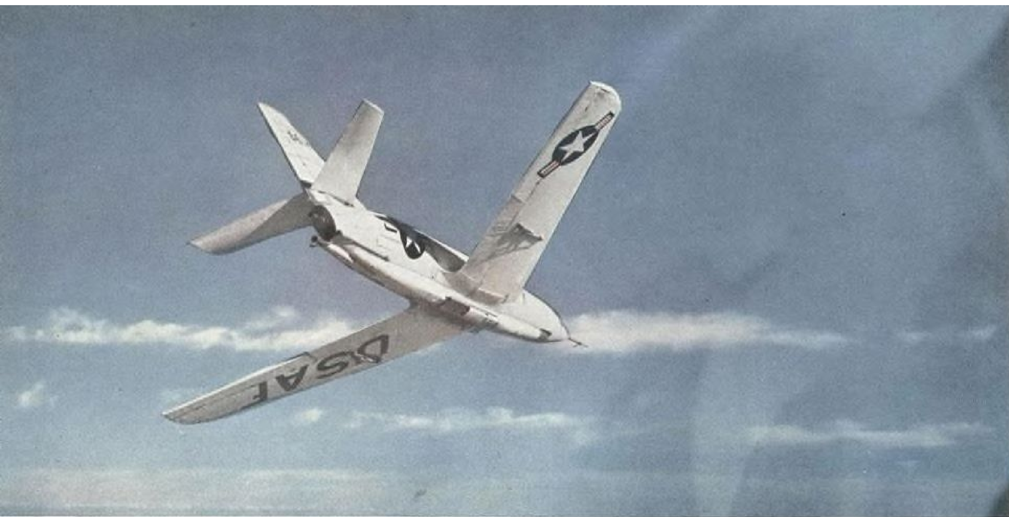
BELL X-2 rocket aircraft explores heating problems at Edwards AFB. Note blunt trailing edges of ailerons. Its pilot is . . .
