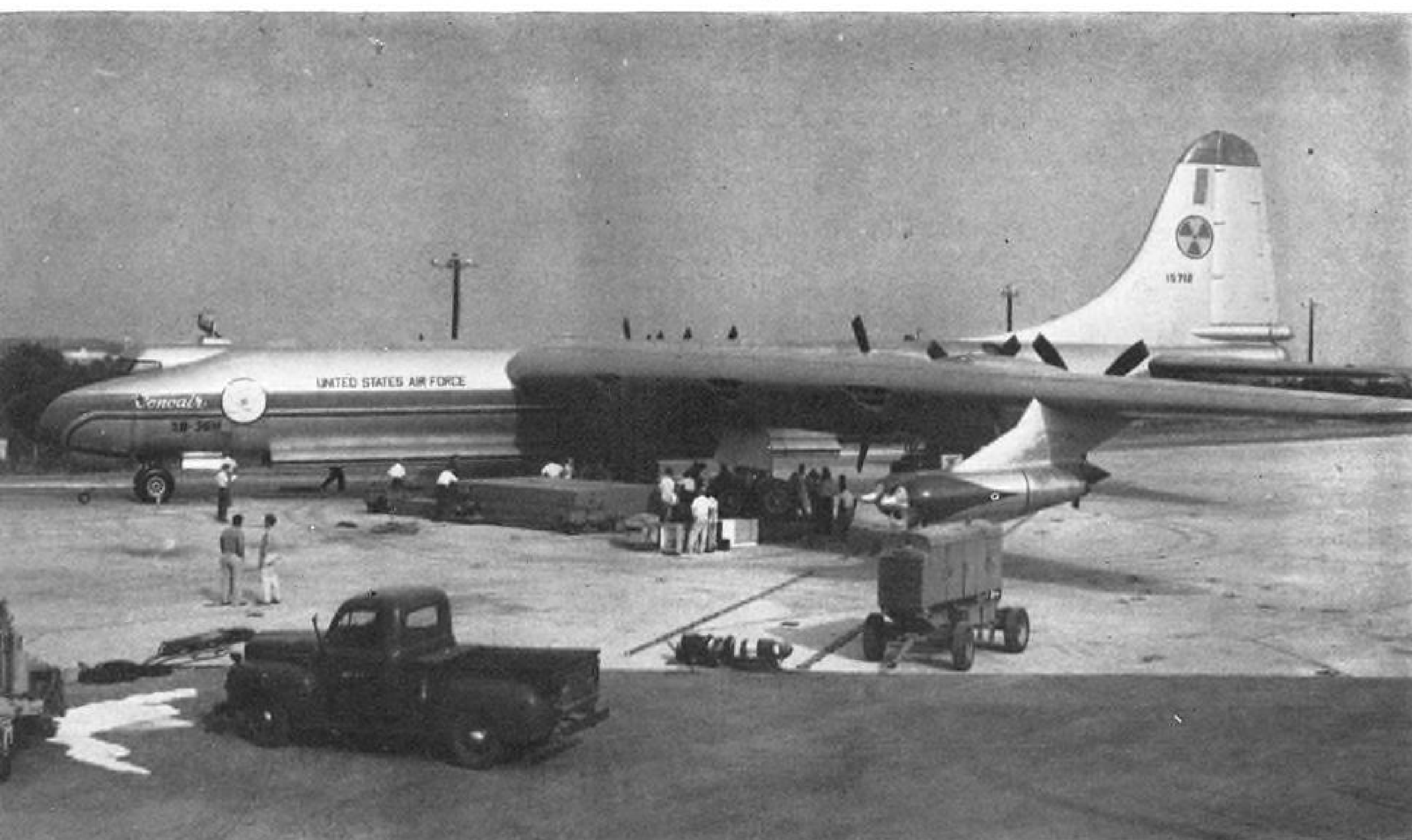
ENLARGED nose of modified B-36 contains shielding. Official radiation symbol decorates tail.
