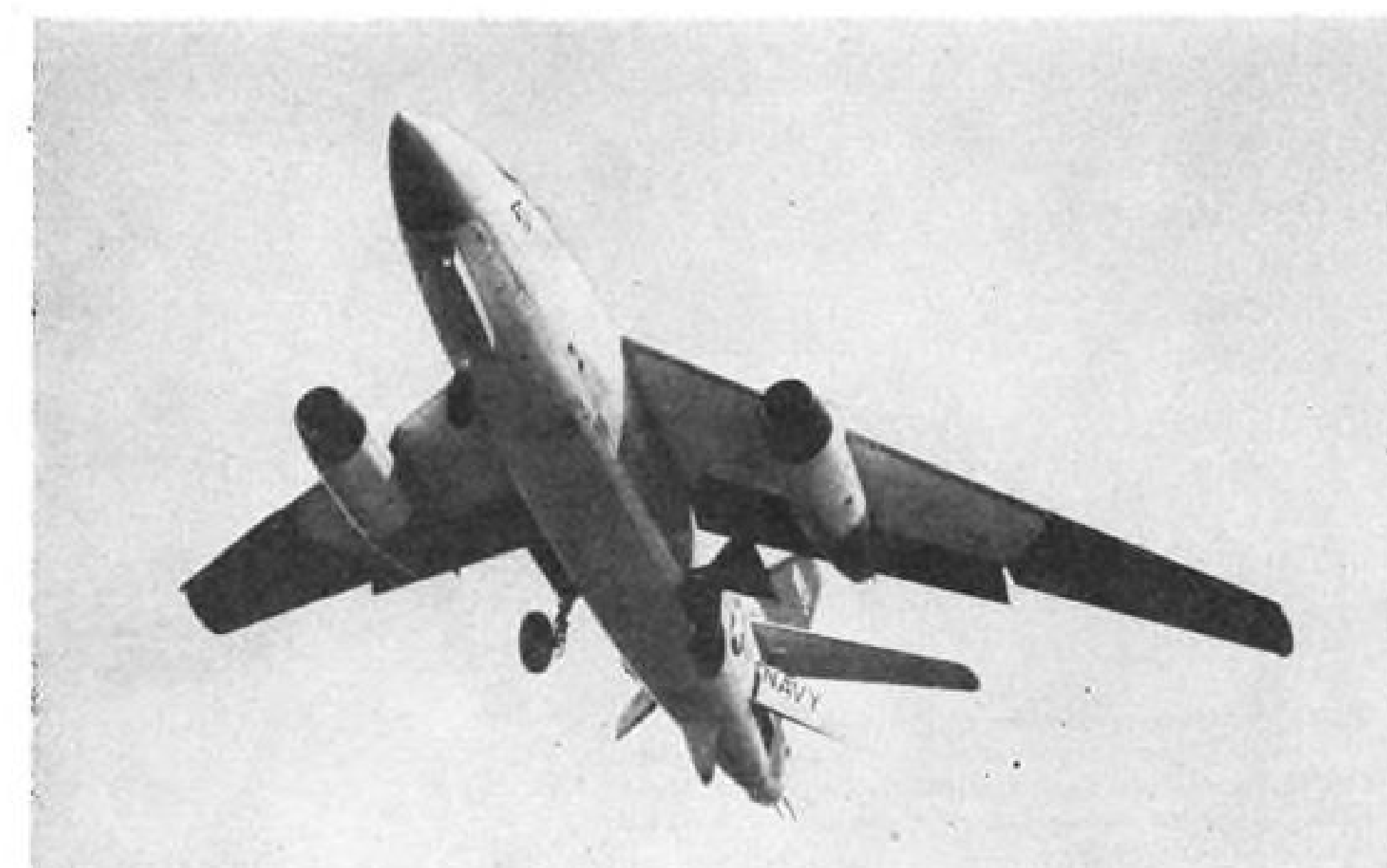
NAVY VERSION, A3D, coming in for landing on USS Forrestal. Wing sweepback of 36 deg. is same for both A3D, B-66, but B-66 has extended center section trailing edge.
