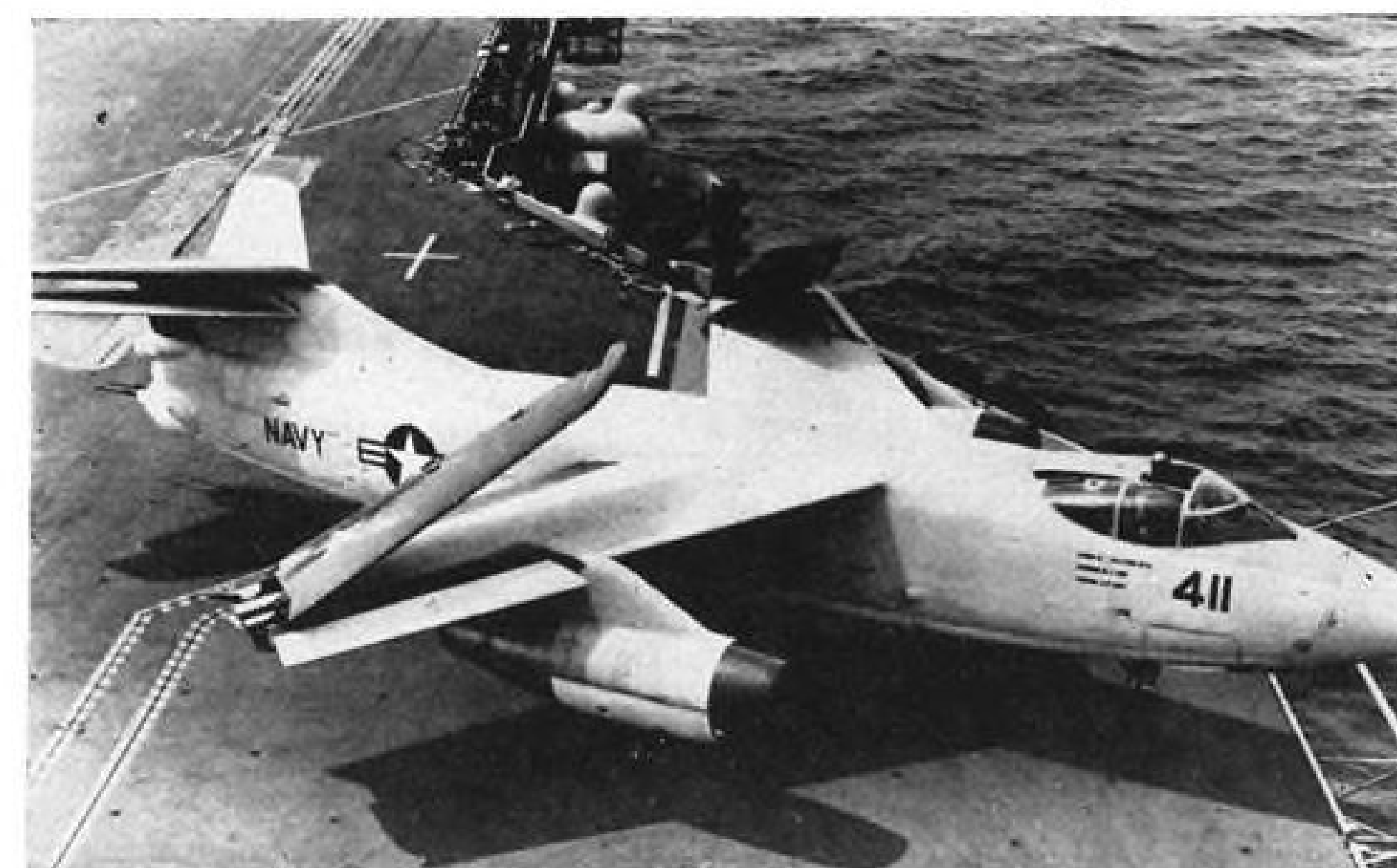
A3D ON DECK edge of Forrestal. Primary difference in two planes is in mission: Navy's is for high altitude, USAF's for low-altitude. A3D-1 uses J57-P-6 engine; B-66 uses J71.
