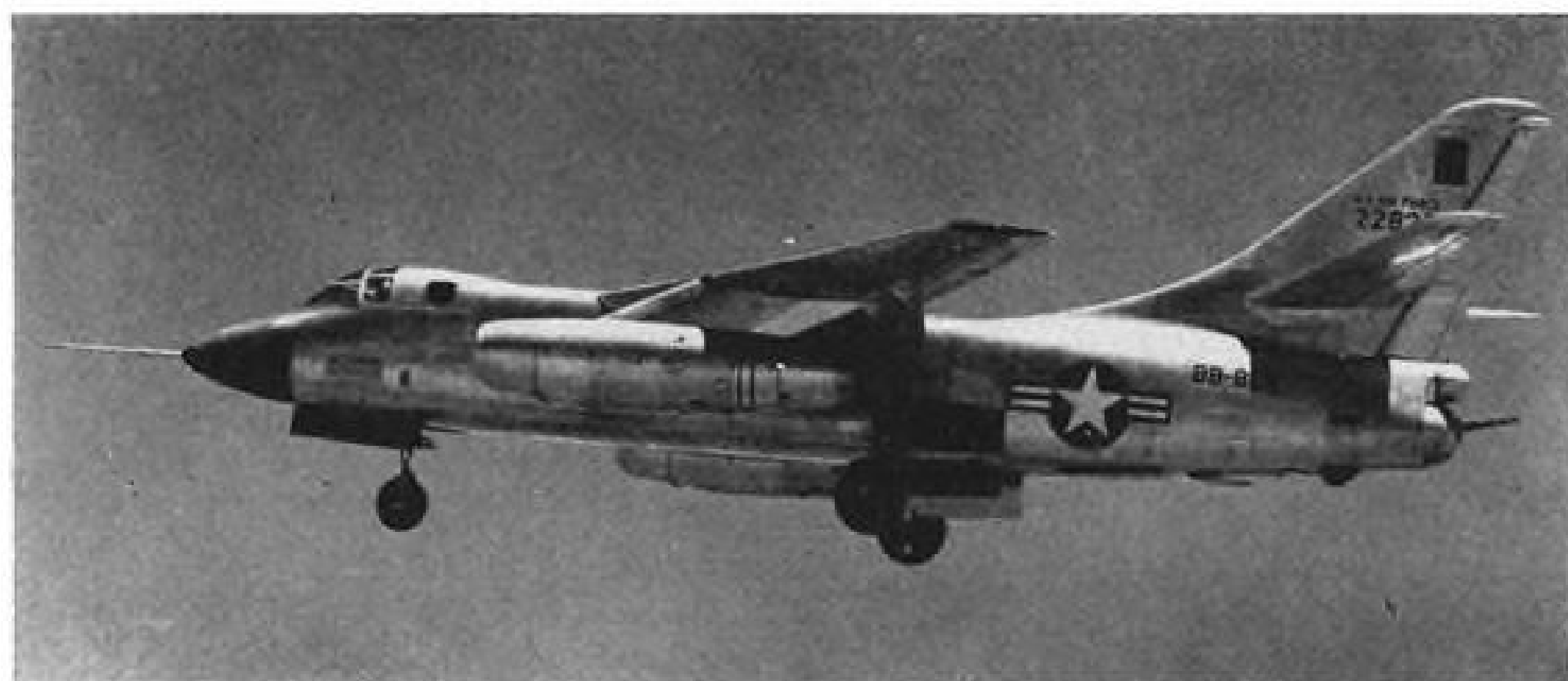
RB-66A MADE its first flight in June, 1954. Total changes from original A3D concept exceeded 400, including new control system, ailerons, spoilers and engine.
