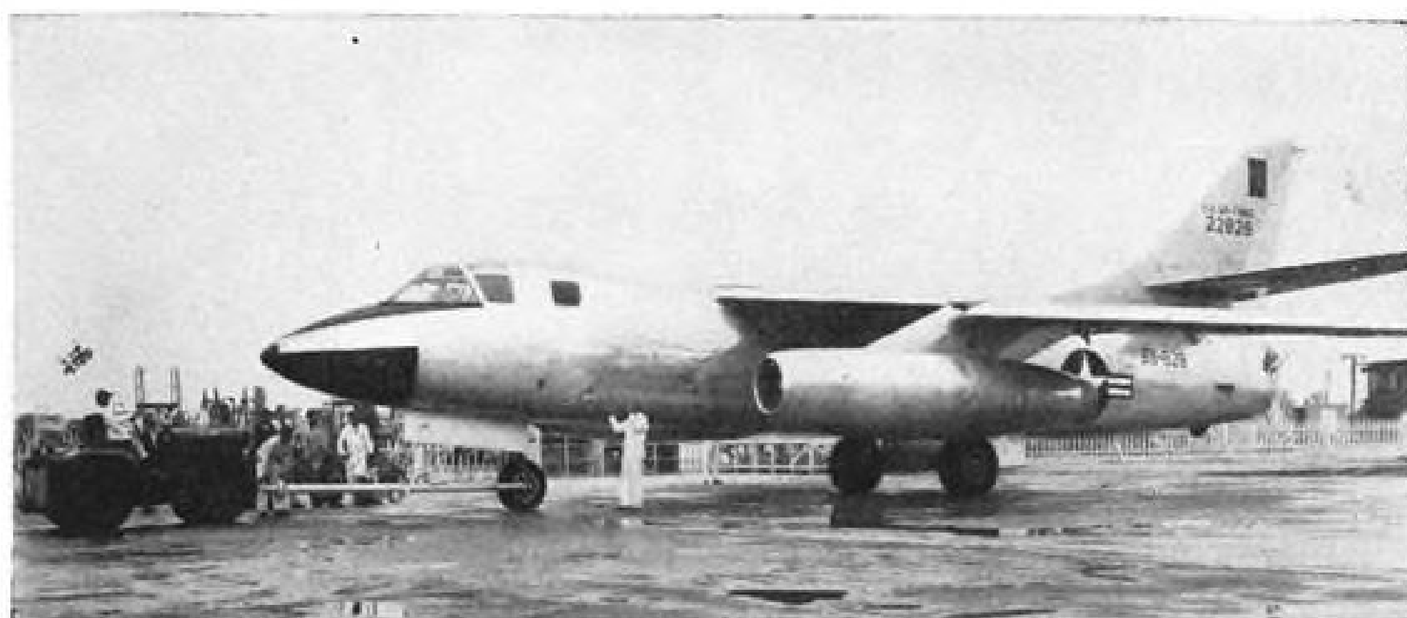
ENGINE MOUNTING pylons of RB-66A were changed to cleaner configuration, straight leading edge, elimination of overlap on top of wing. Note A3D picture page 61.
