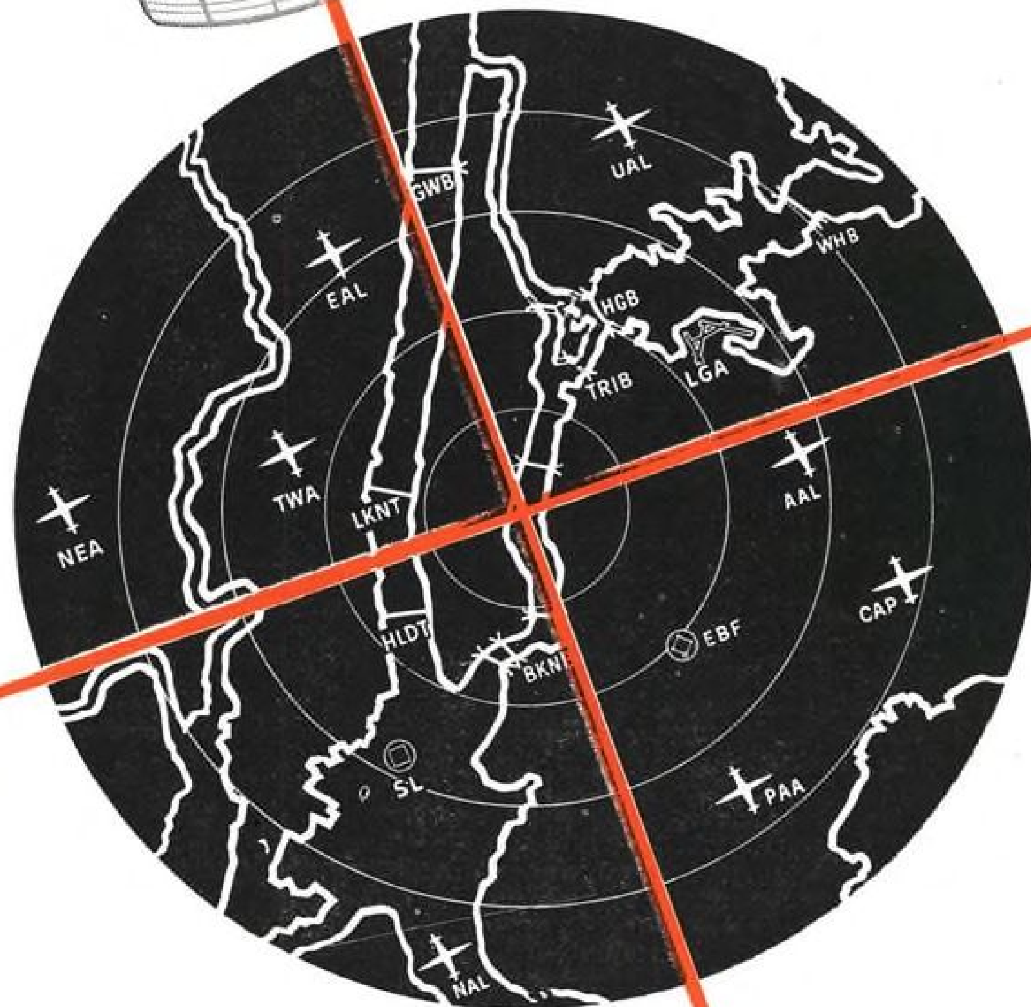
DESTINY ON DISPLAY IBM computer generated display presents moving "situation map" of the skies over New York City. Symbols represent commercial airliners and ground reference.
