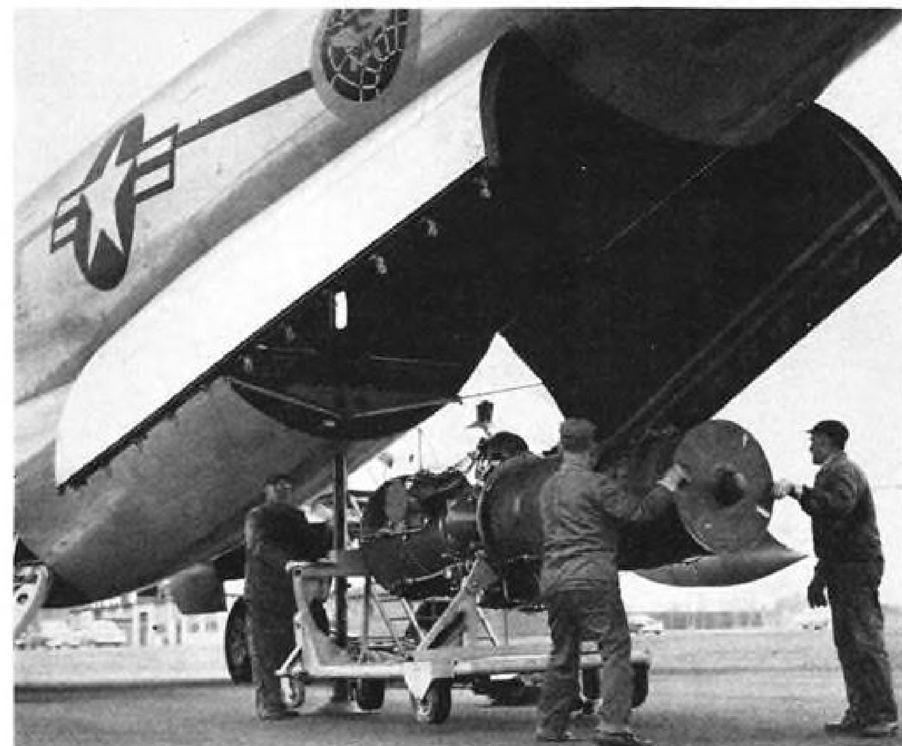
A PRATT & WHITNEY AIRCRAFT T-34 turboprop engine is loaded aboard a YC-97J Boeing Transport.
