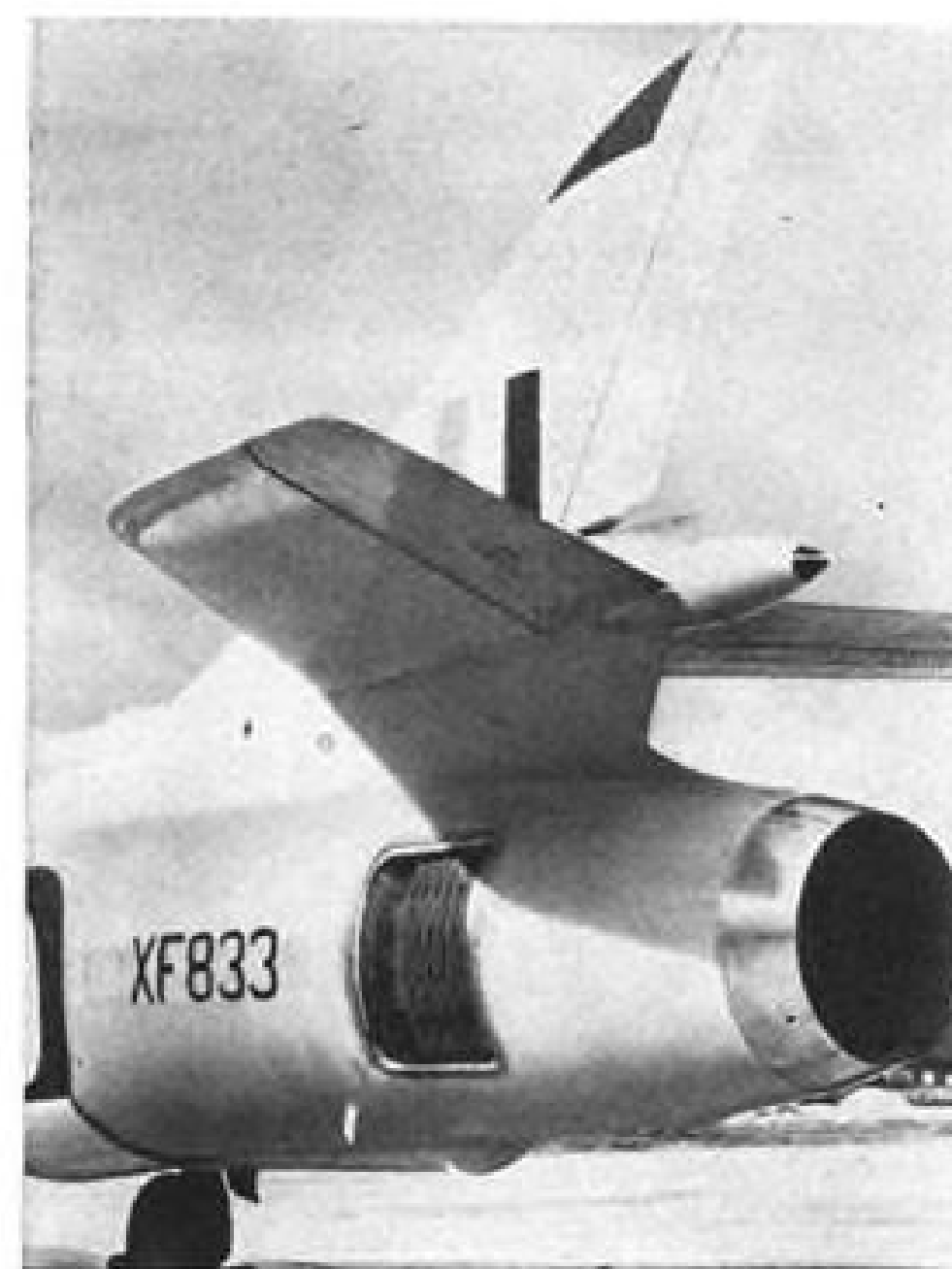
ROLLS-ROYCE reverse thrust unit is installed in the tailpipe of a Hawker Hunter F Mk. 6 fighter. Outlet grills are on each side of rear fuselage.
