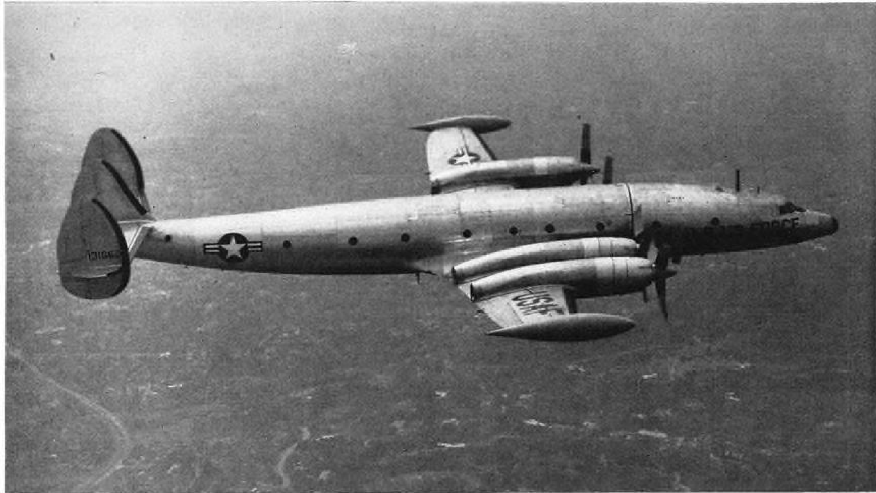
THE LOCKHEED YC-121F, powered by four Pratt & Whitney T-34 turboprop engines, is the world's fastest propeller-driven transport. The aircraft cruises at 420 mph.
