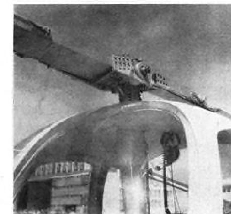
FORWARD position of Continental FSO-470A engine (top right) eliminates special induction, lubrication systems in Cessna YH-41 helicopter. Rotor has simple pylon mount (bottom).
