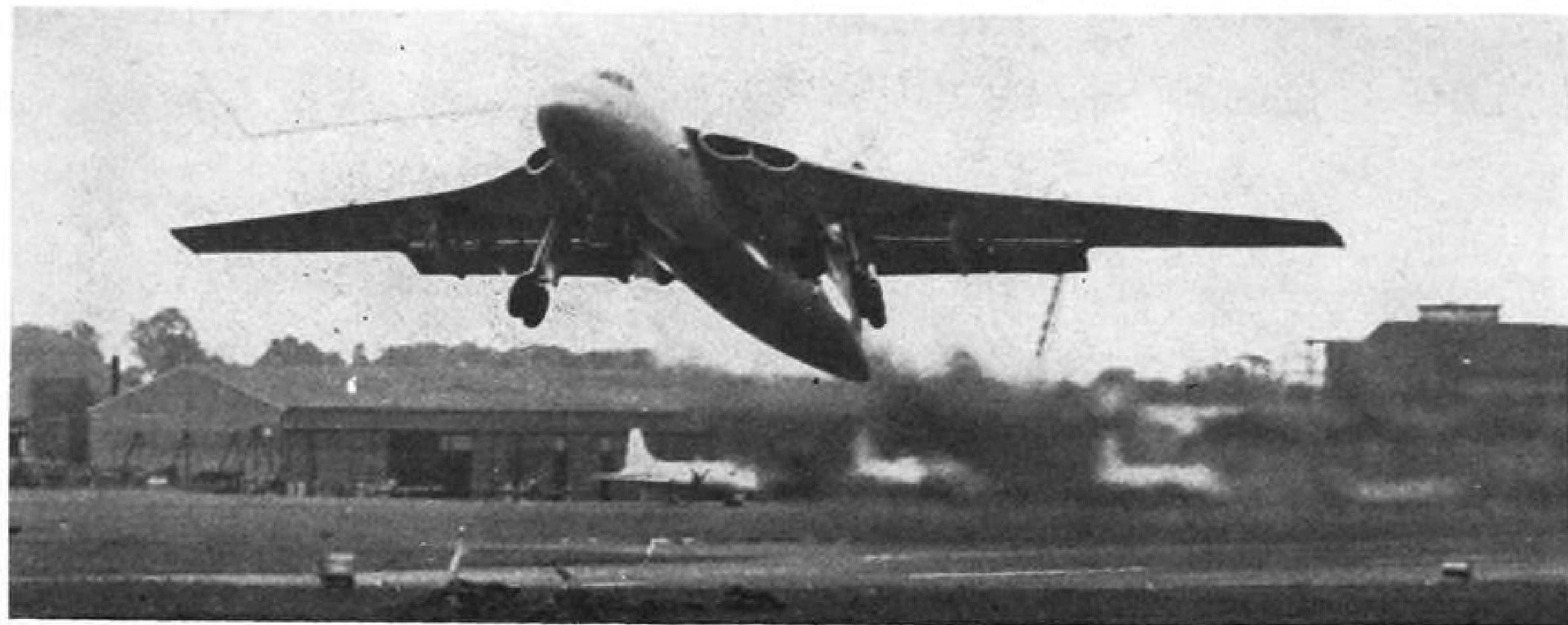
VICKERS VALIANT bomber takeoff run is cut with the aid of two de Havilland Super Sprite rocket engines (AW Aug. 20, p. 34).
