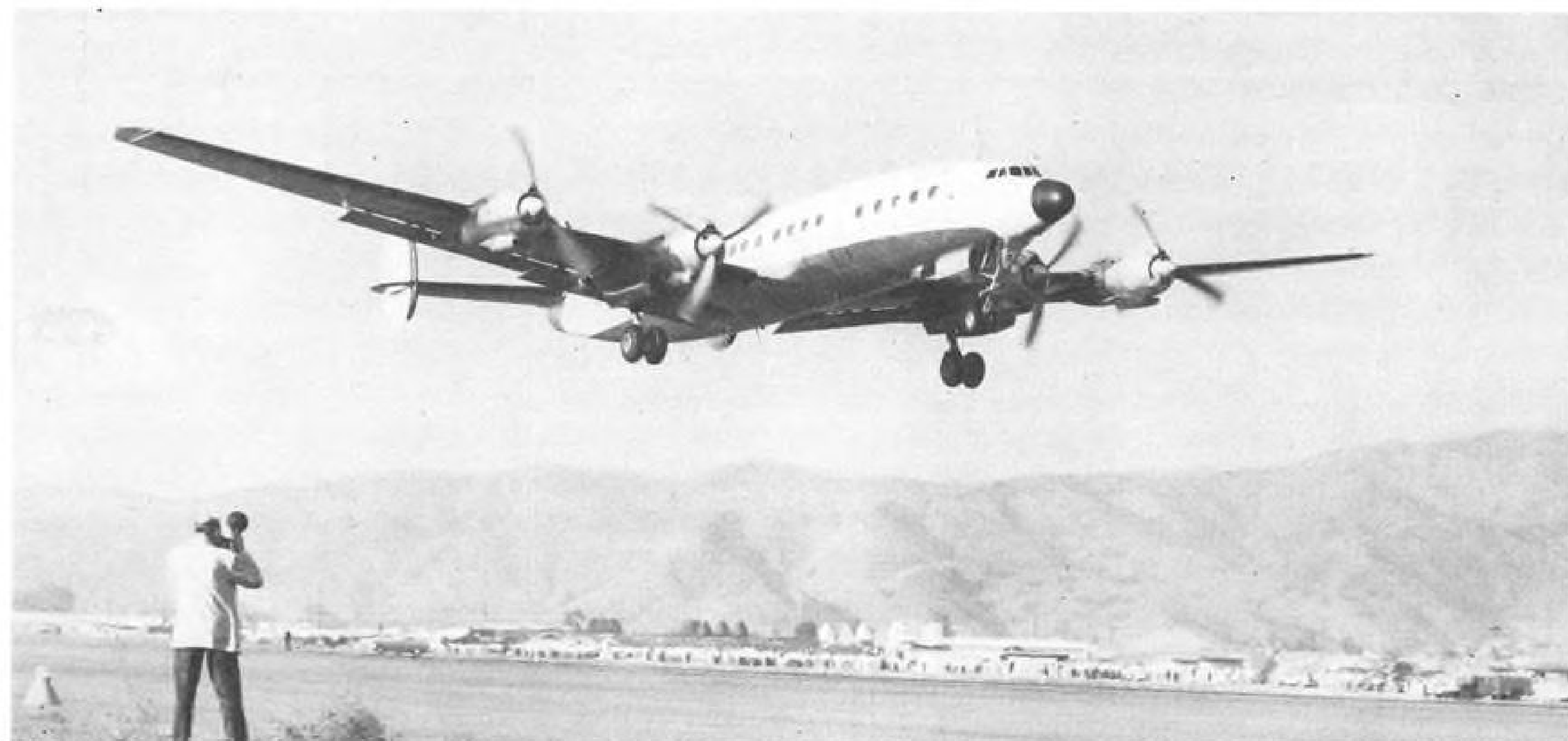
FIRST 1649A Constellation taking off from Lockheed Air Terminal and in flight on maiden hop. Flight was first test of new 150-ft. wing, 27 ft. greater than previous Super Constellations. Aircraft is in production at Lockheed for Trans World Airlines and will go into service next spring and summer on the transatlantic as well as domestic flights.
