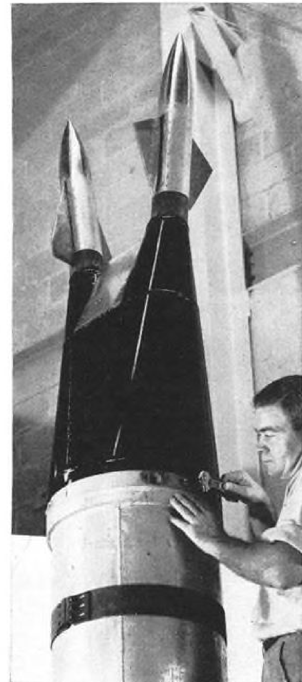
TWO-HEADED test vehicle measures heat transfer on two body-wing combinations simultaneously at an angle of attack.
