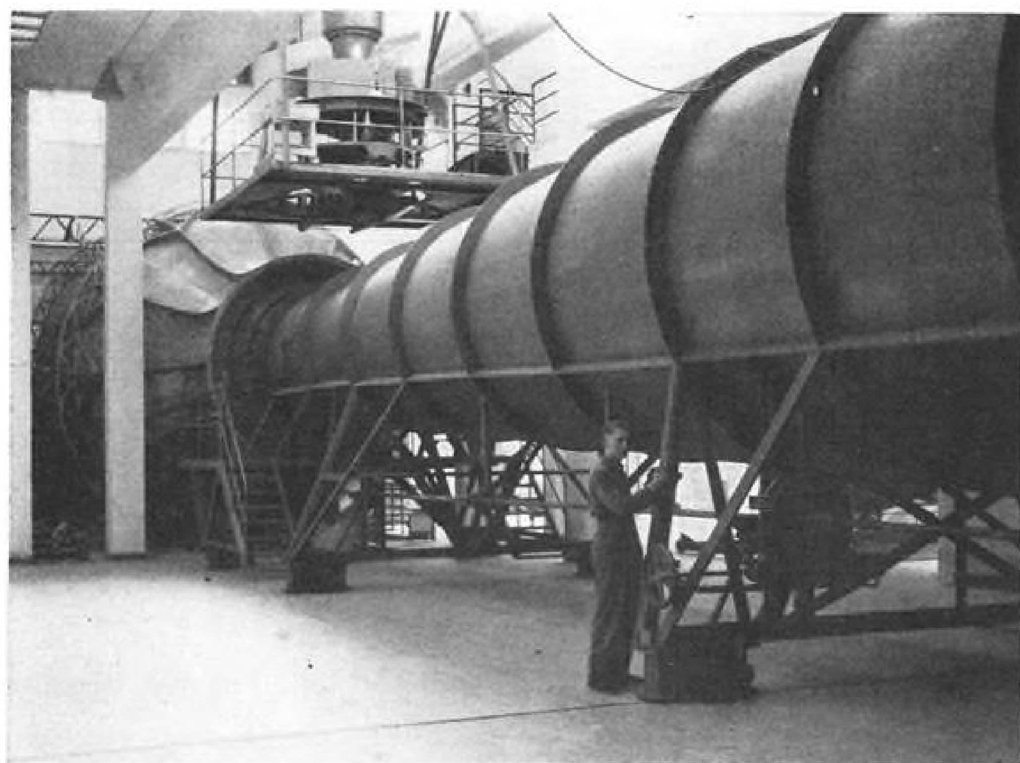
FACILITIES OF NATO'S new Training Center for Experimental Aerodynamics include supersonic wind tunnel capable of speeds to Mach 2.3; composite low speed wind tunnel.
