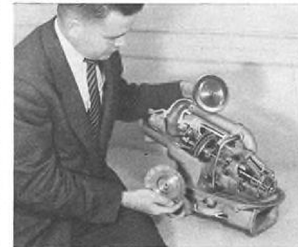
G-E Afterburner Turbopump Gives North American F-86D Instant Power Reserve
