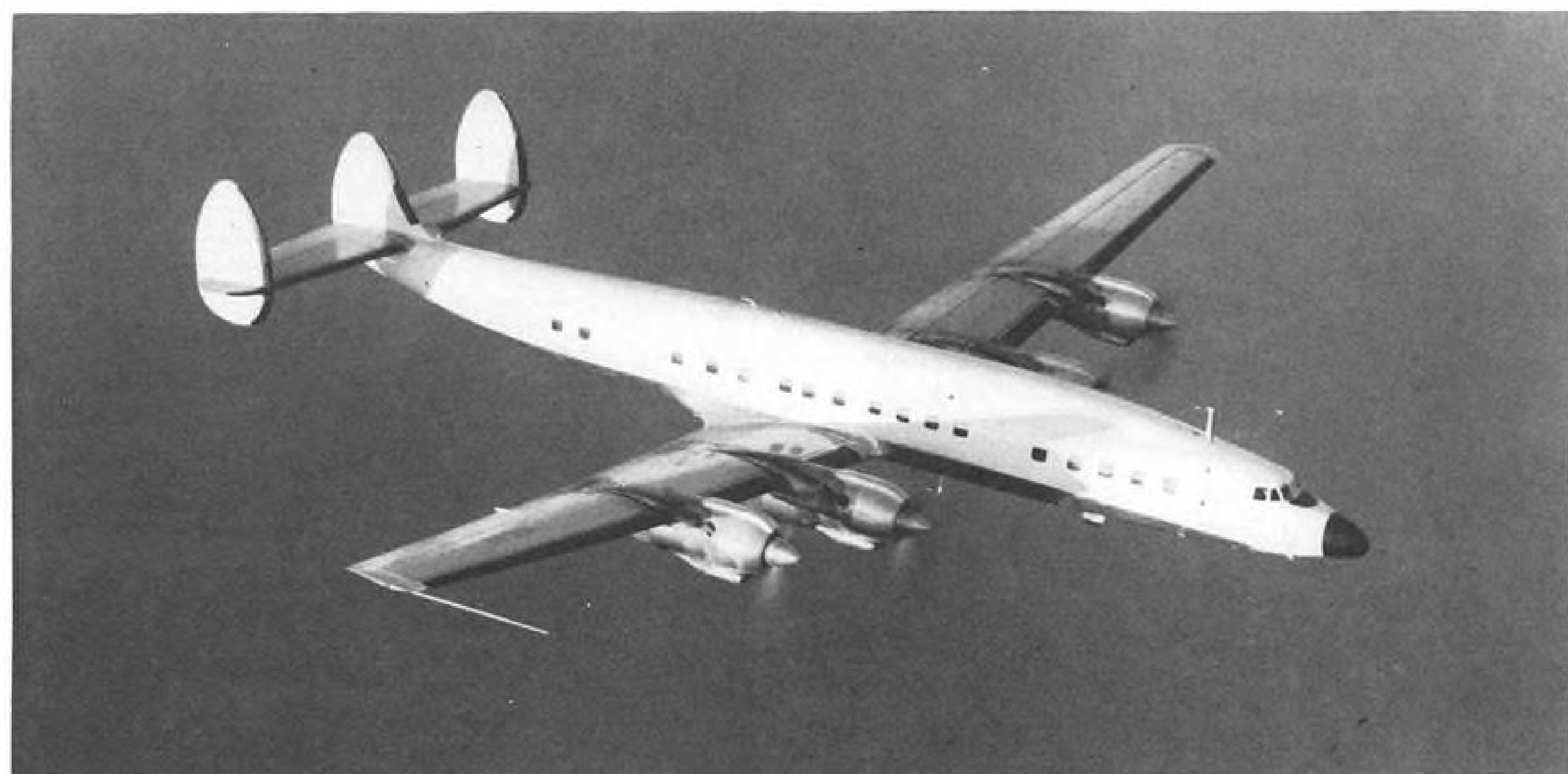
FIRST 1649A Constellation taking off from Lockheed Air Terminal and in flight on maiden hop. Flight was first test of new 150-ft. wing, 27 ft. greater than previous Super Constellations. Aircraft is in production at Lockheed for Trans World Airlines and will go into service next spring and summer on the transatlantic as well as domestic flights.
