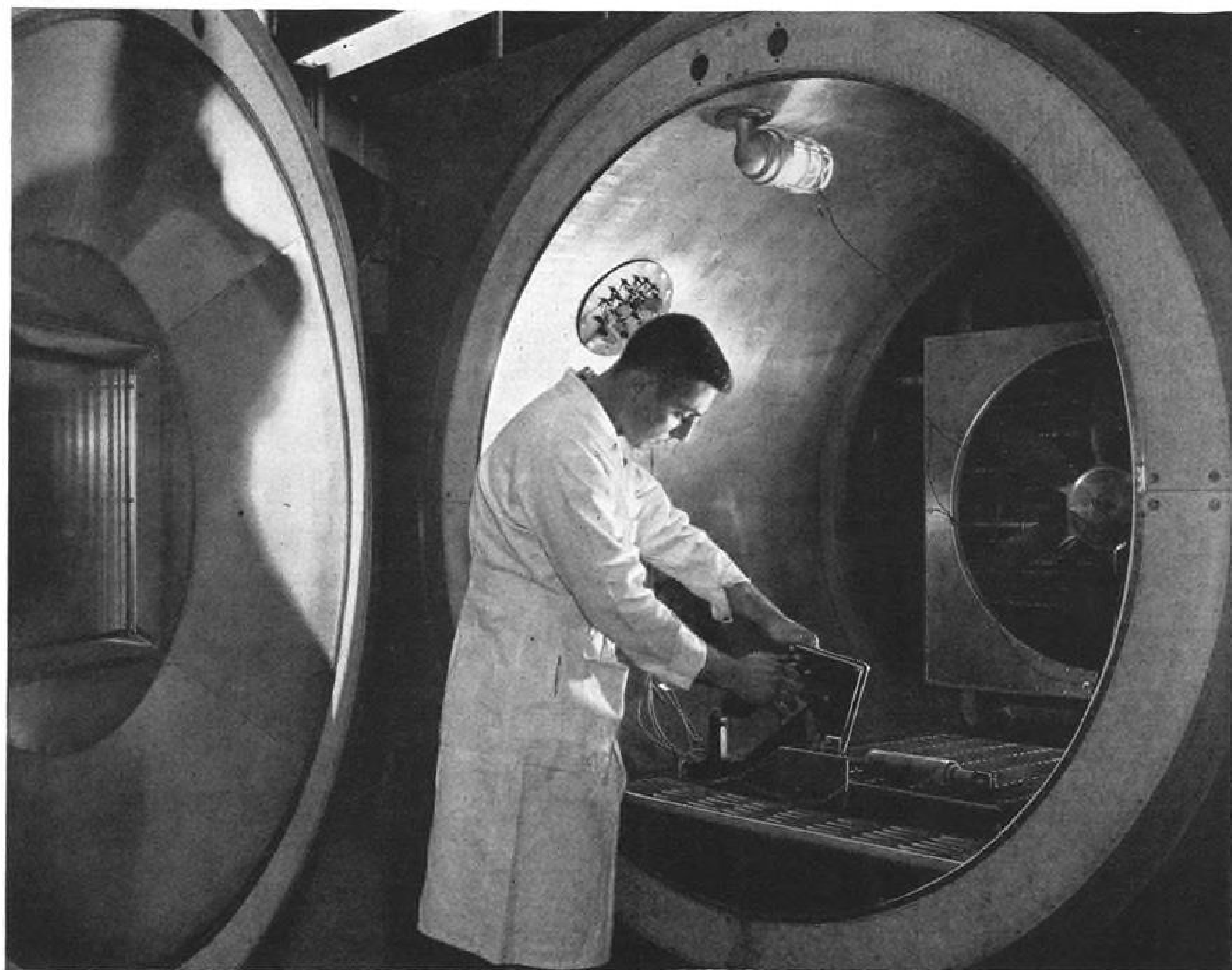
Altitudes high above ceilings for today's aircraft are simulated in this chamber.
