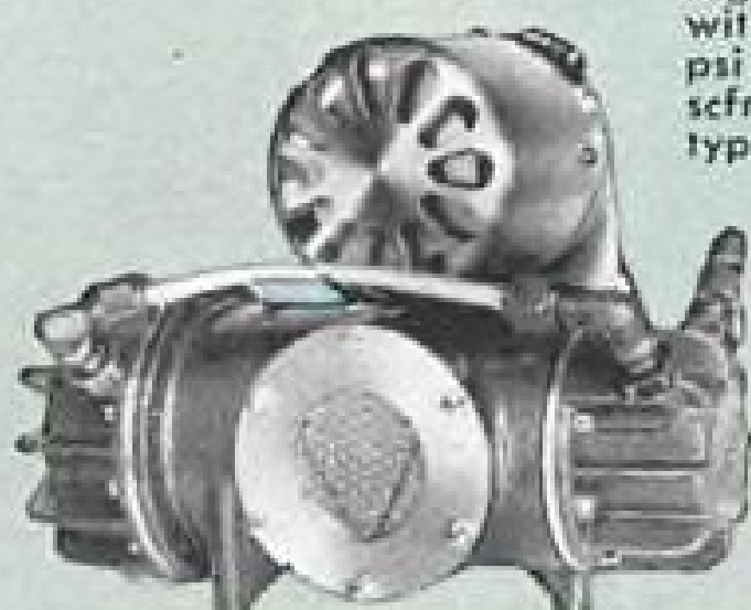
Low Pressure Air Compressors —For pressurization of electronic equipment, hydraulic and fuel reservoirs. Rated at 1 cfm of free air at 25 psig and altitudes up to 50,000 ft. Available with explosion-proof AC or DC motors, relief valve, pressure switch, and dehydrator.
