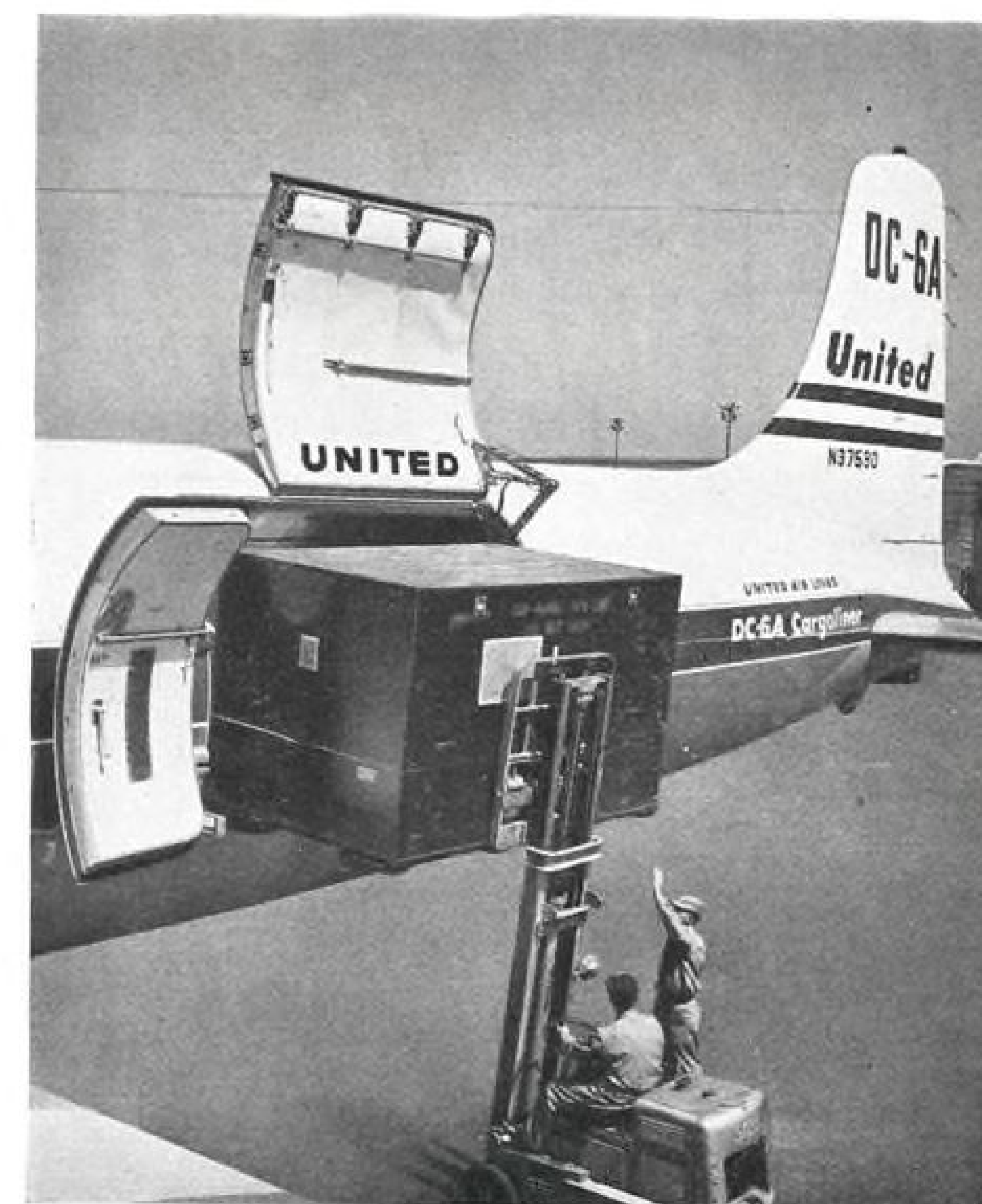
LARGE-SIZE OBJECTS , hitherto restricted from air shipment, fit easily into the spacious cabin of United's DC-6A. Cargo capacity is 30,000 pounds.
