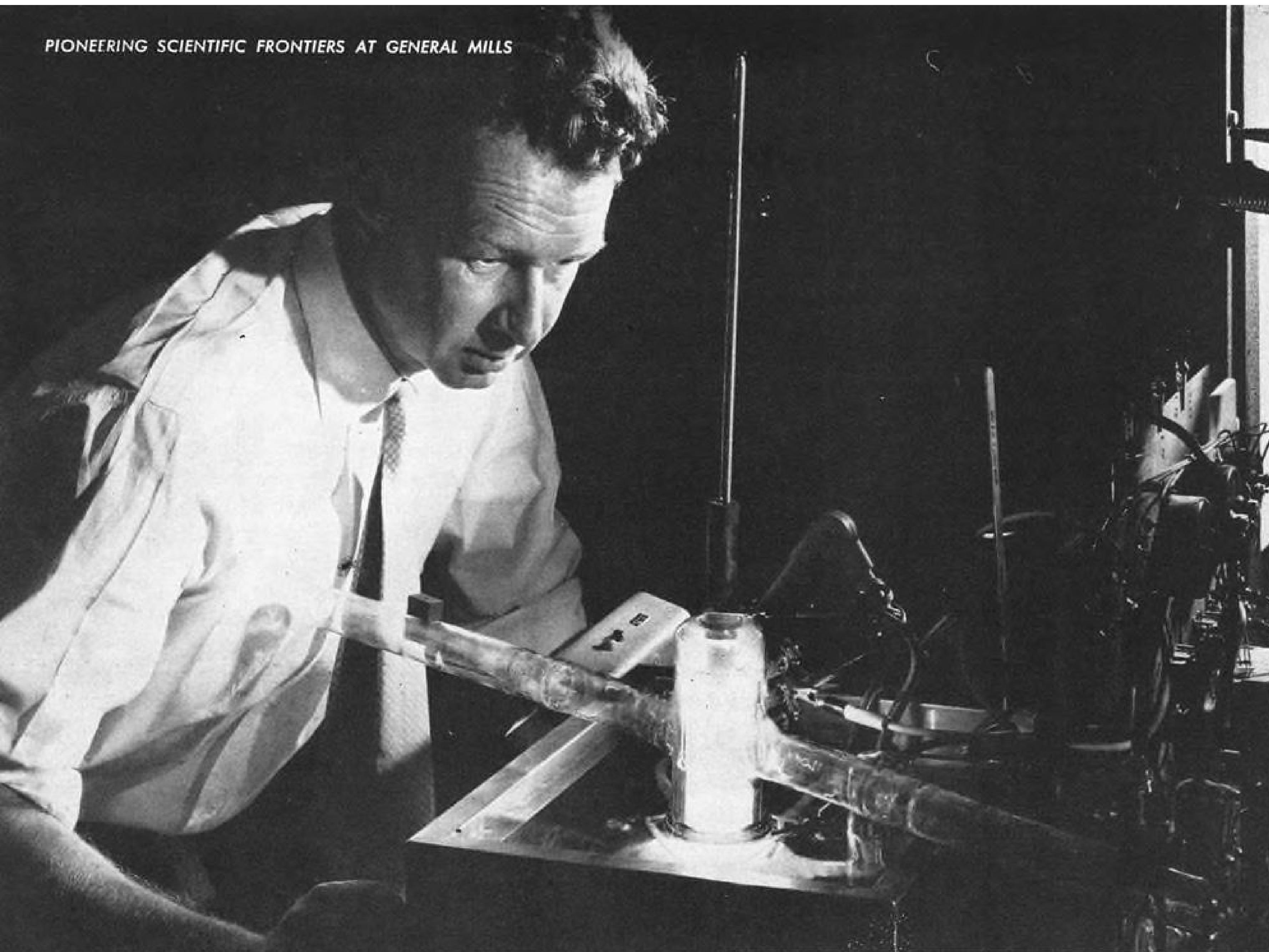
This scientific pioneer is Dr. G. K. Wehner, designer of the space chamber which he uses here to determine the "sputtering" or disintegration rate of molybdenum under bombardment from atoms moving at 25,000 m.p.h., 200 miles above the earth.
