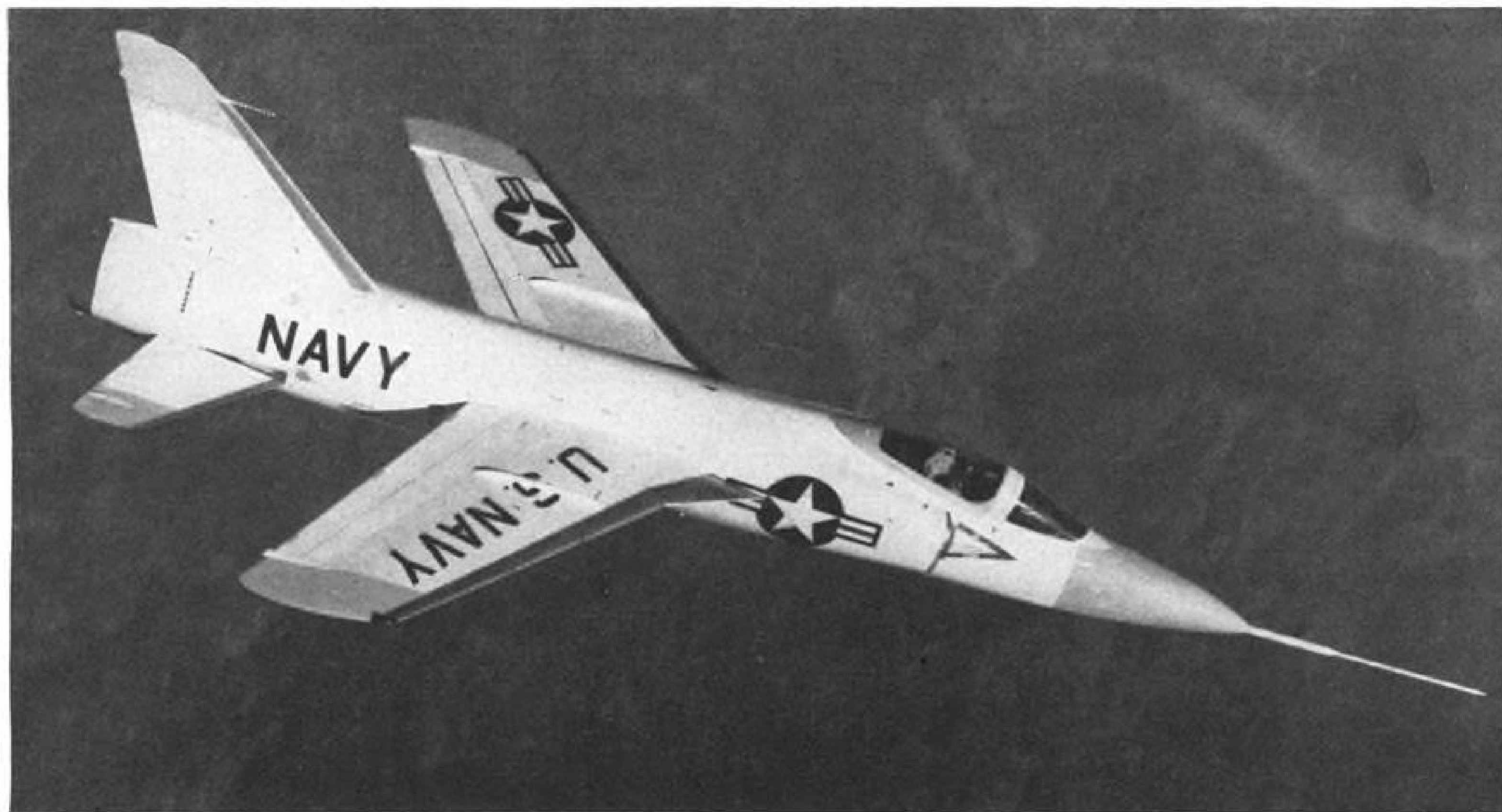
LATEST Tiger in flight shows wing root and tail extensions characteristic of this modification of the supersonic fighter.
