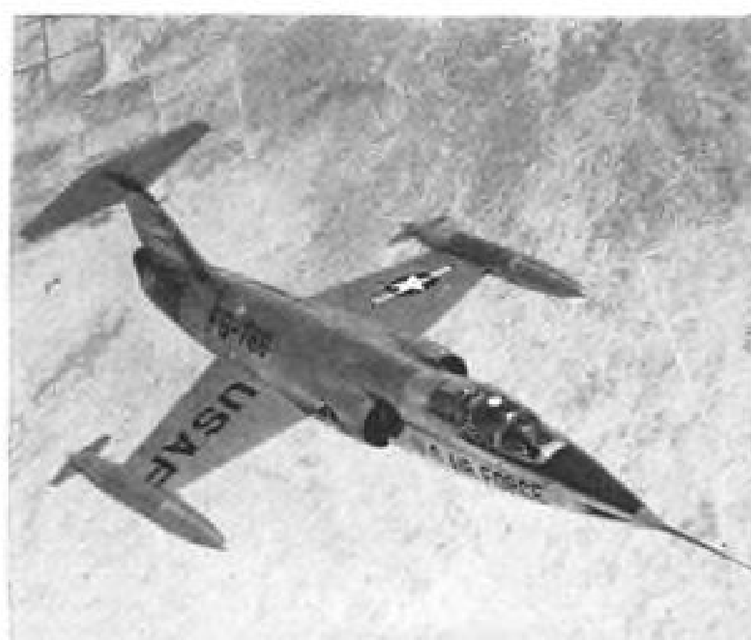
World's faster fighter, Lockheed's new, ultrasonic F-104A Starfighter is powered by the new General Electric J-79 jet engine. Wing measures only 7½ feet from fuselage to tip. Unique features include: The most powerful jet engine, thrust per pound, ever developed; a T-shaped "flying tail."
