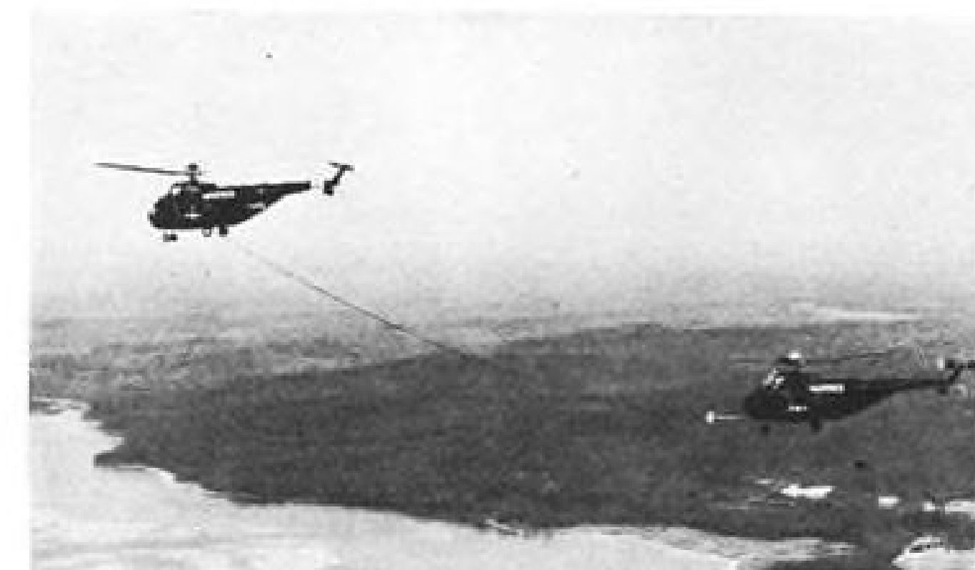
How Probe and Drogue system, pioneered by Flight Refueling, Inc., can be successfully used for helicopter to helicopter refueling is shown in preliminary Marine Corps trials.
