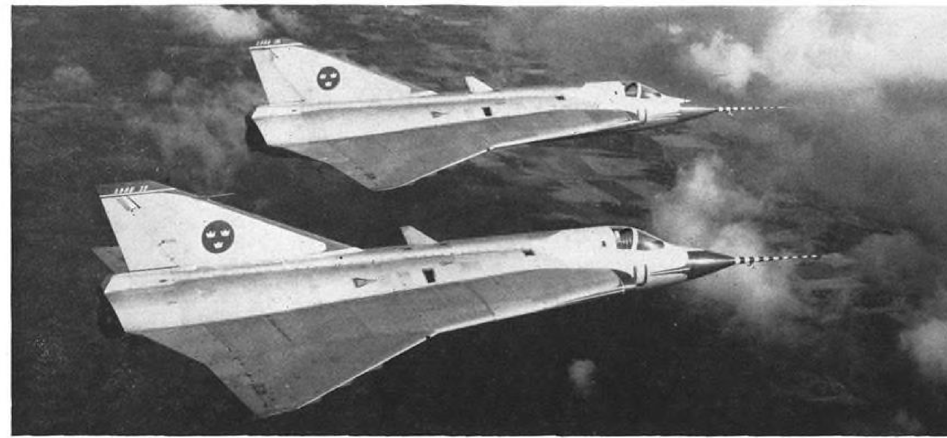
FLYING DRAGONS show sleek aerodynamic layout; small separate dorsal fin on fuselage spine has been added since prototype.
