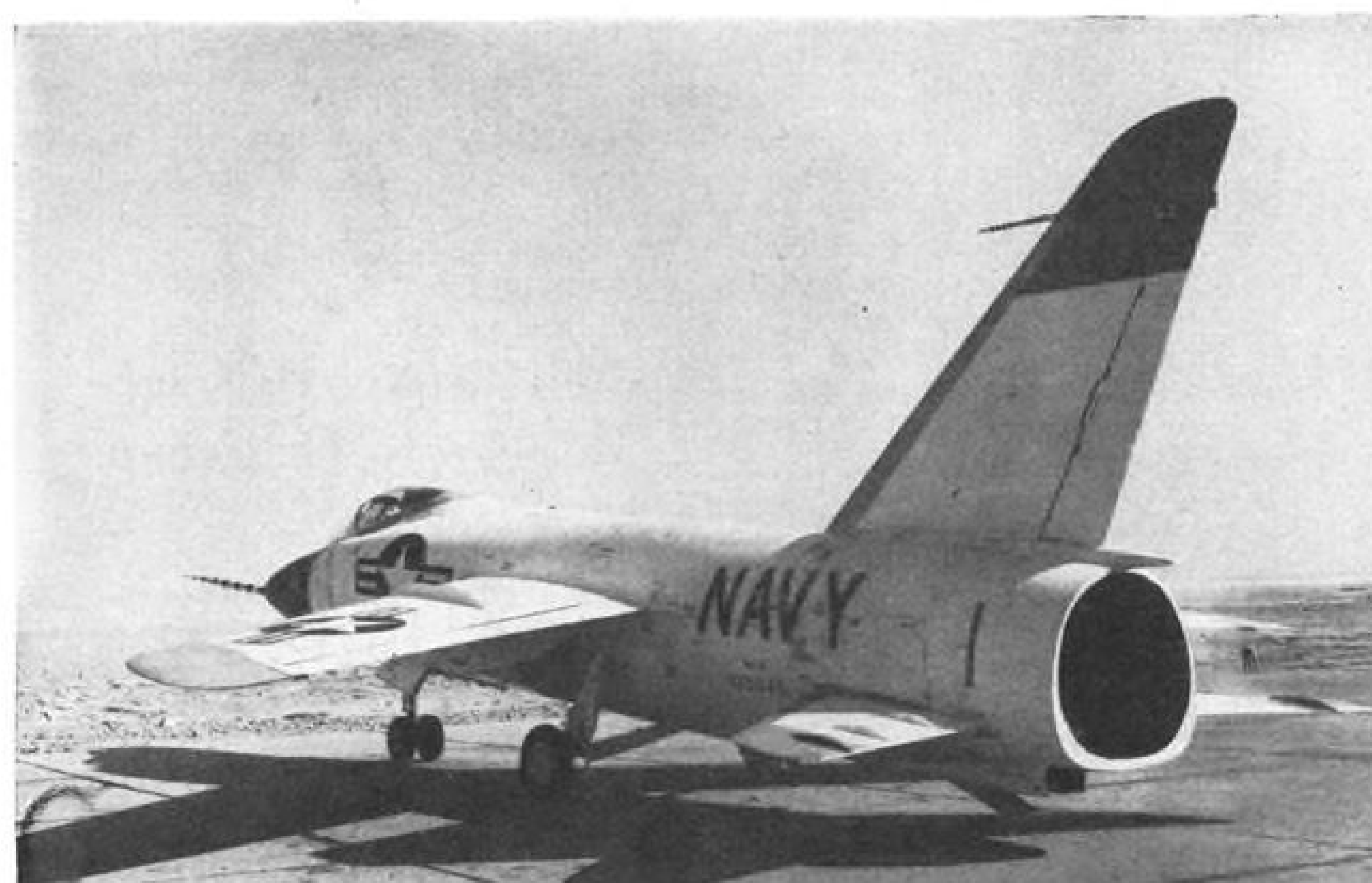
BELLY plan of F11F-1F shows external changes: extended wing leading edge, swelled rear fuselage and new engine inlet ducts.
