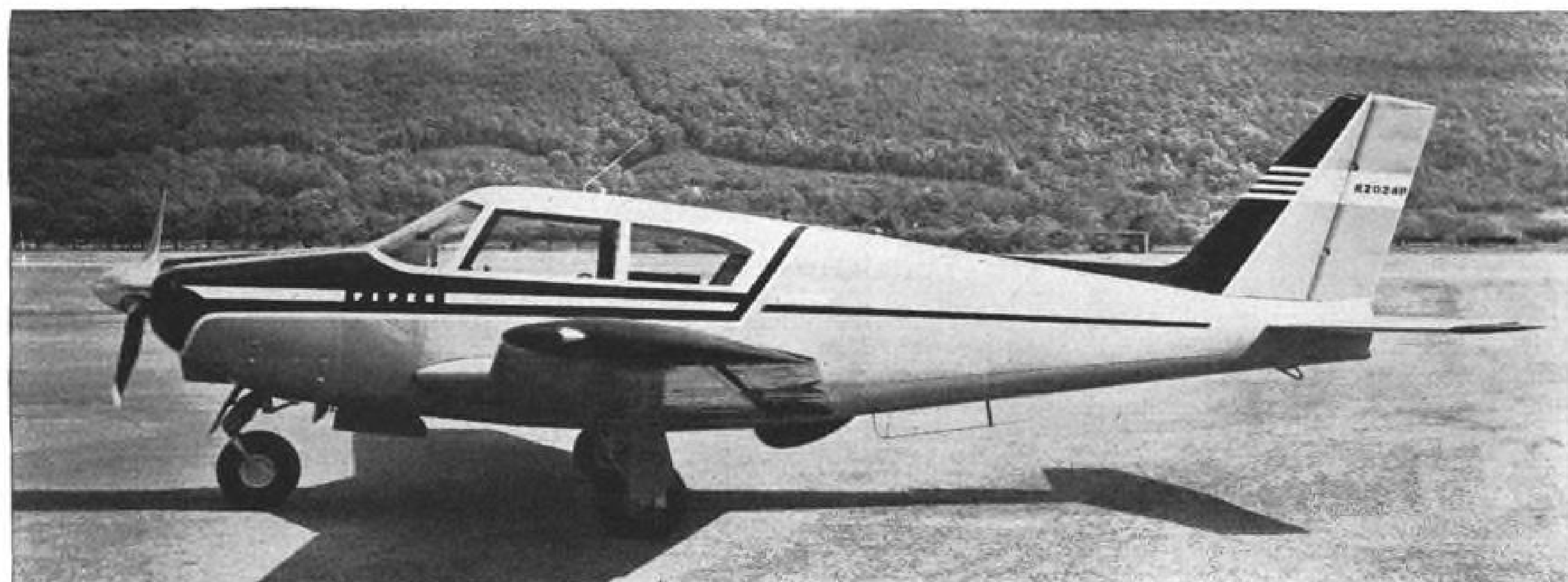
PIPER COMANCHE will be produced in two models, one with 180 hp. engine as in prototype, the other with 250 hp. engine.
