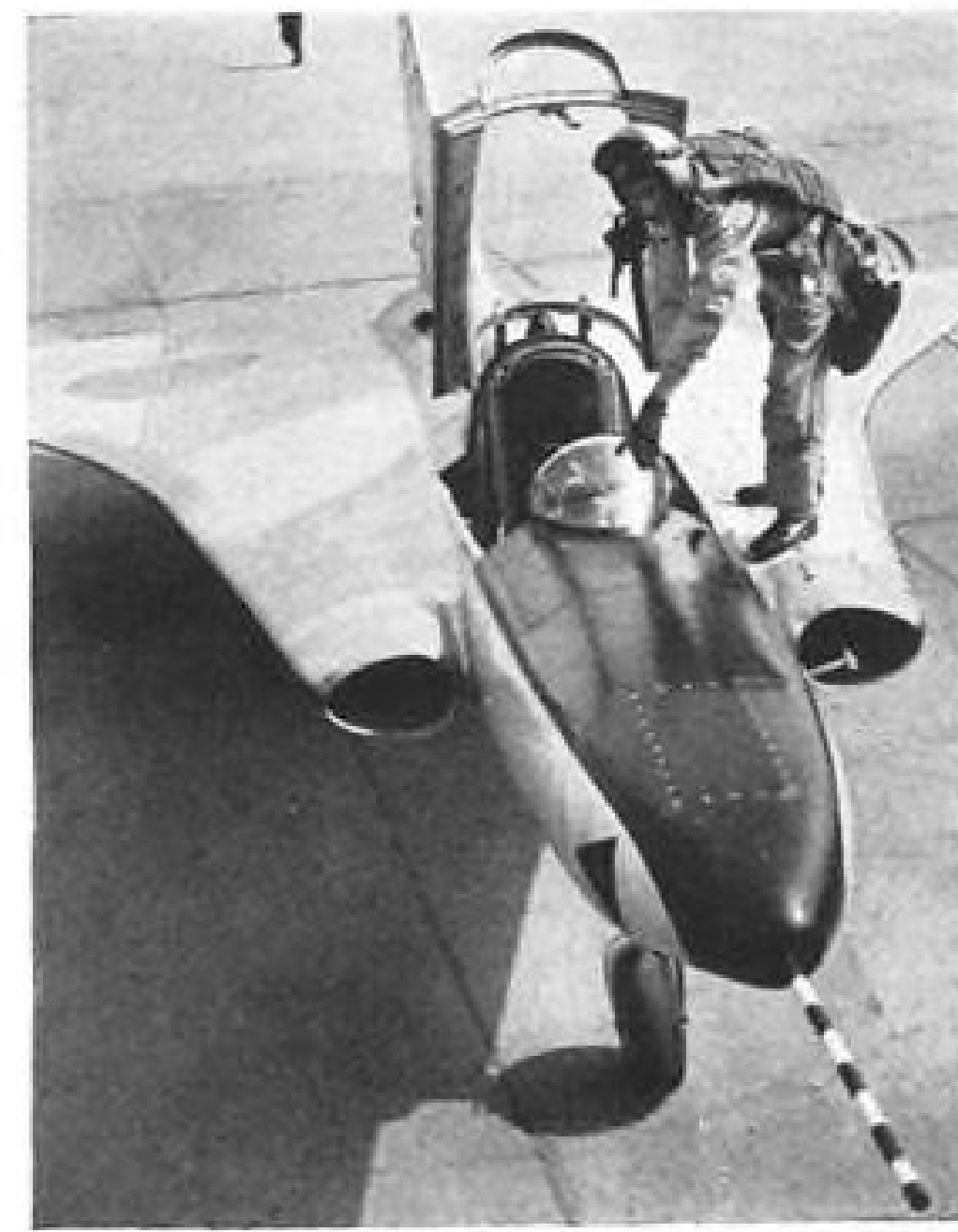
SAAB 210 research plane was developed as aerodynamic test vehicle. Pilot (right) indicates size of later, longer-nosed vehicle.
