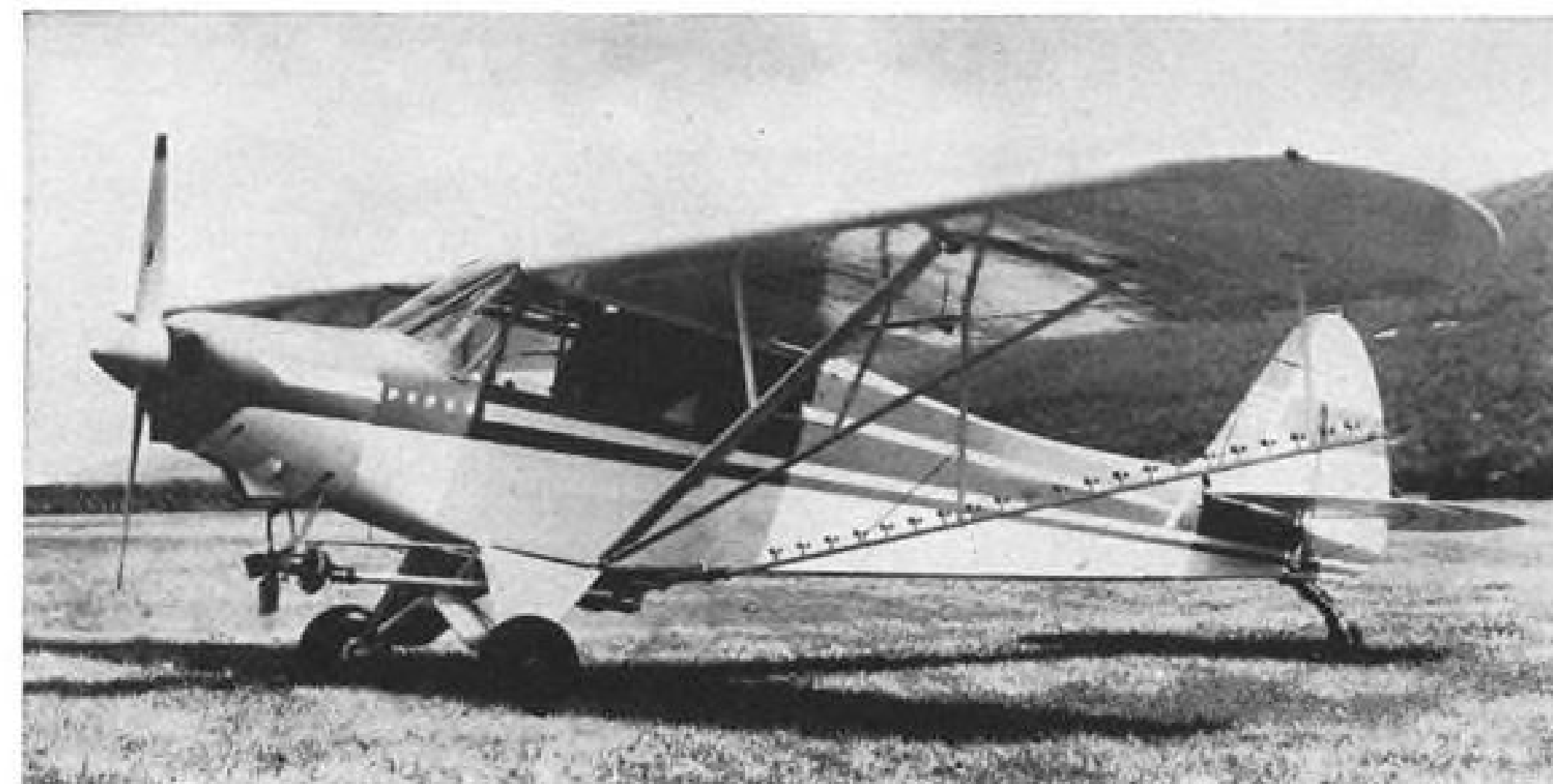
PIPER SPRAYER is fitted with floating booms that swing back if they strike object.
