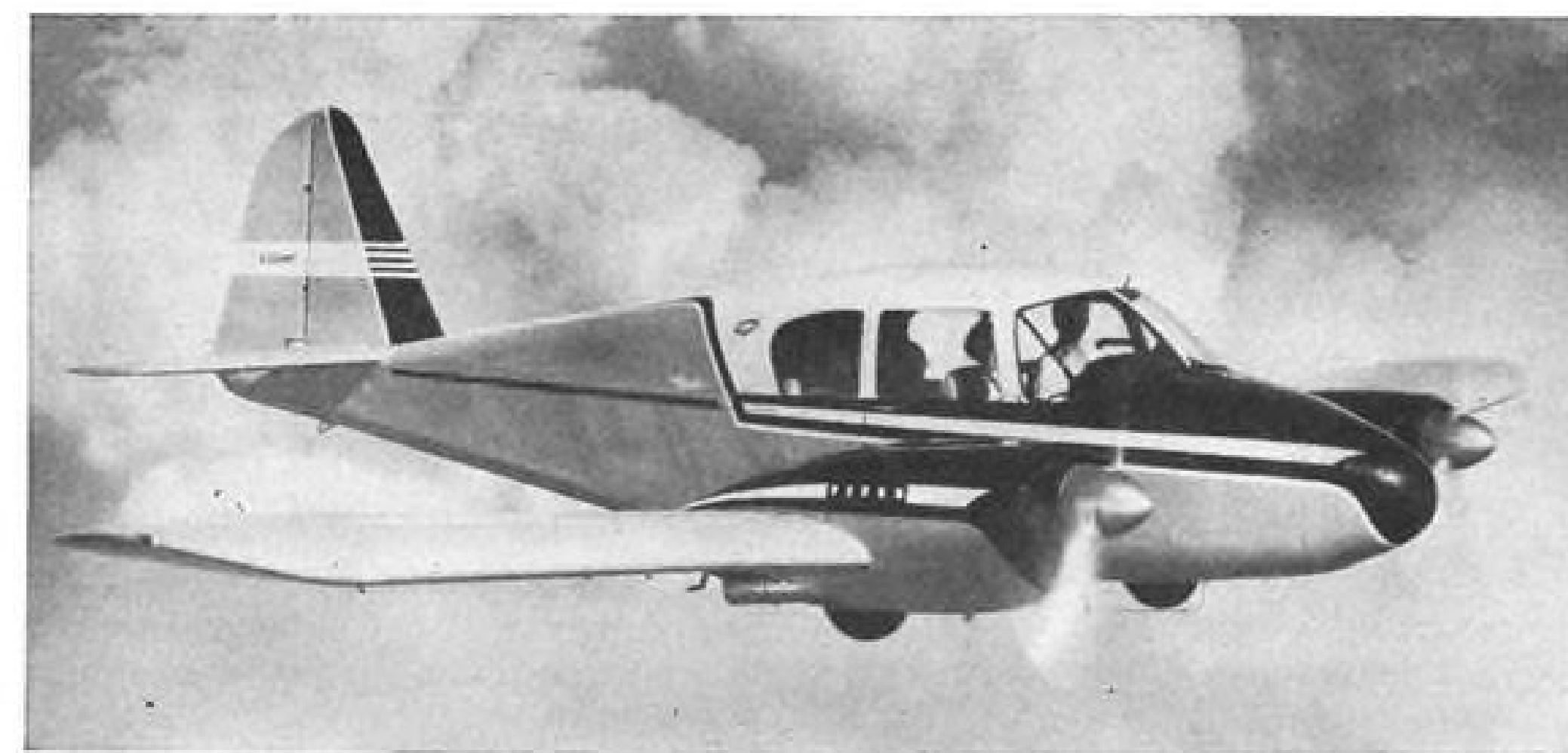
NEW COLOR scheme is used on 1957 Apache. Black nose, nacelles reduce glare.
