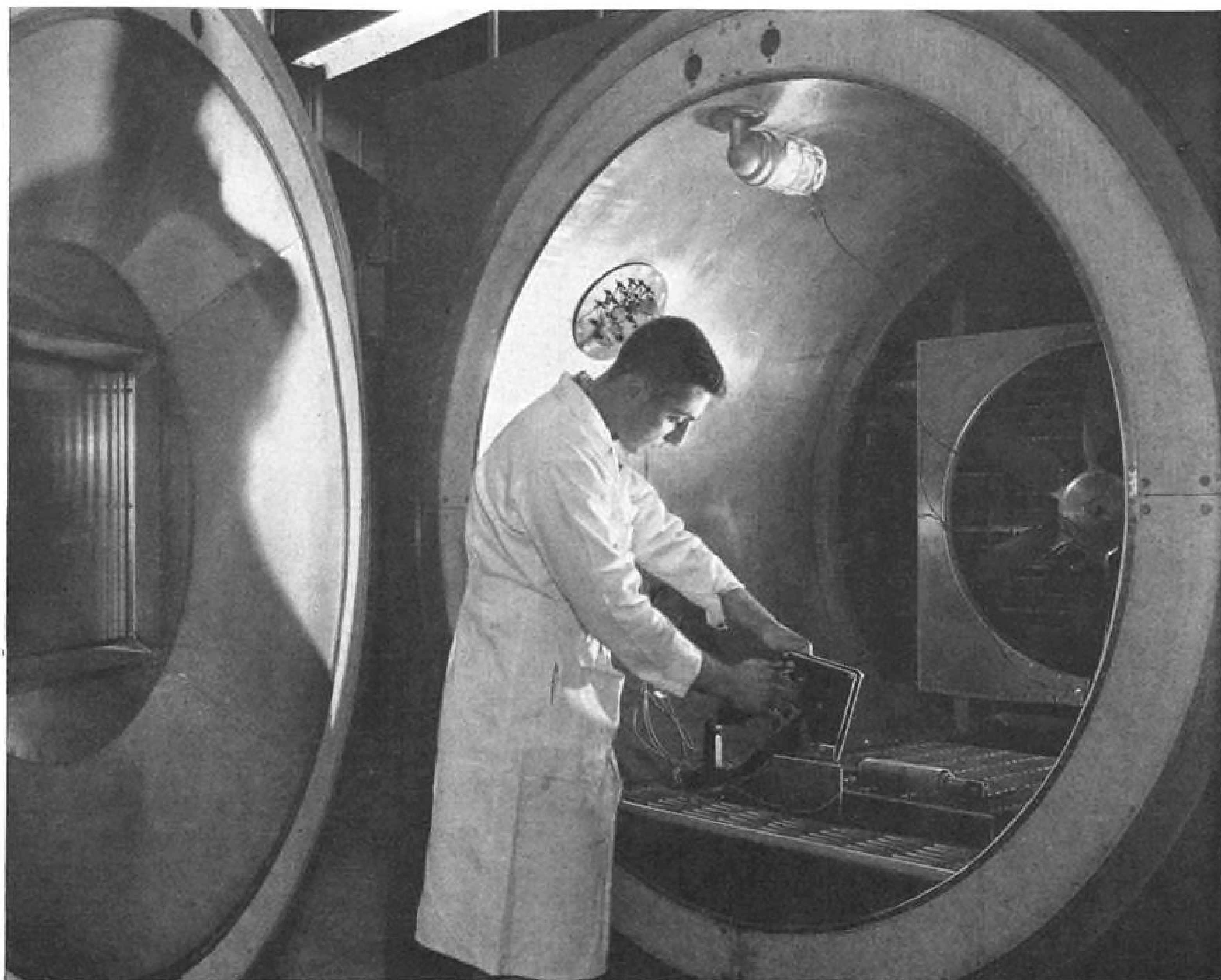
Altitudes high above ceilings for today's aircraft are simulated in this chamber.
