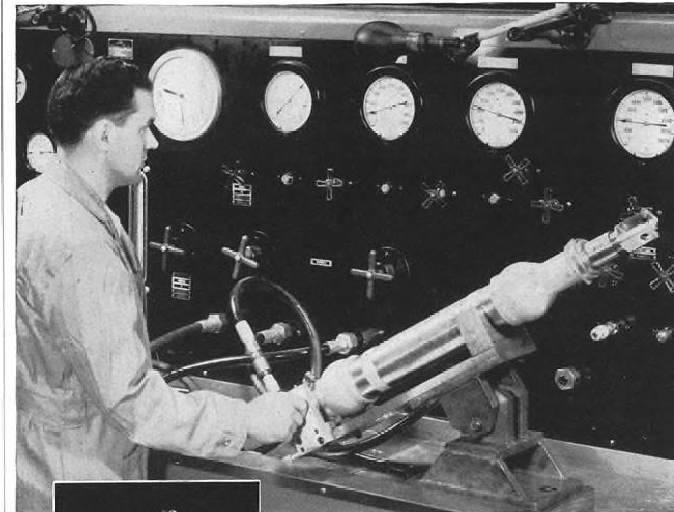
This test stand checks actuating assemblies under simulated operating conditions.
