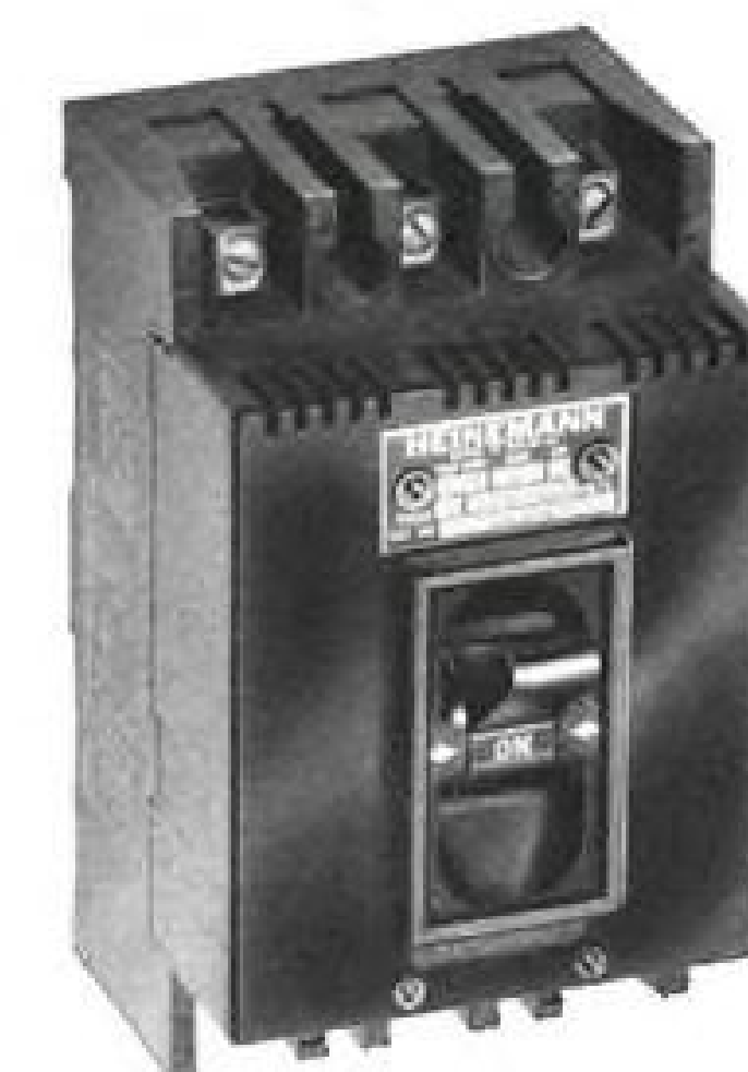
Heinemann General Purpose Three-Pole Circuit Breaker. Available in odd or fractional ratings from 0.010 to 70 amperes. (Other models to 100 amperes.) Ratings are not affected by ambient temperature.
