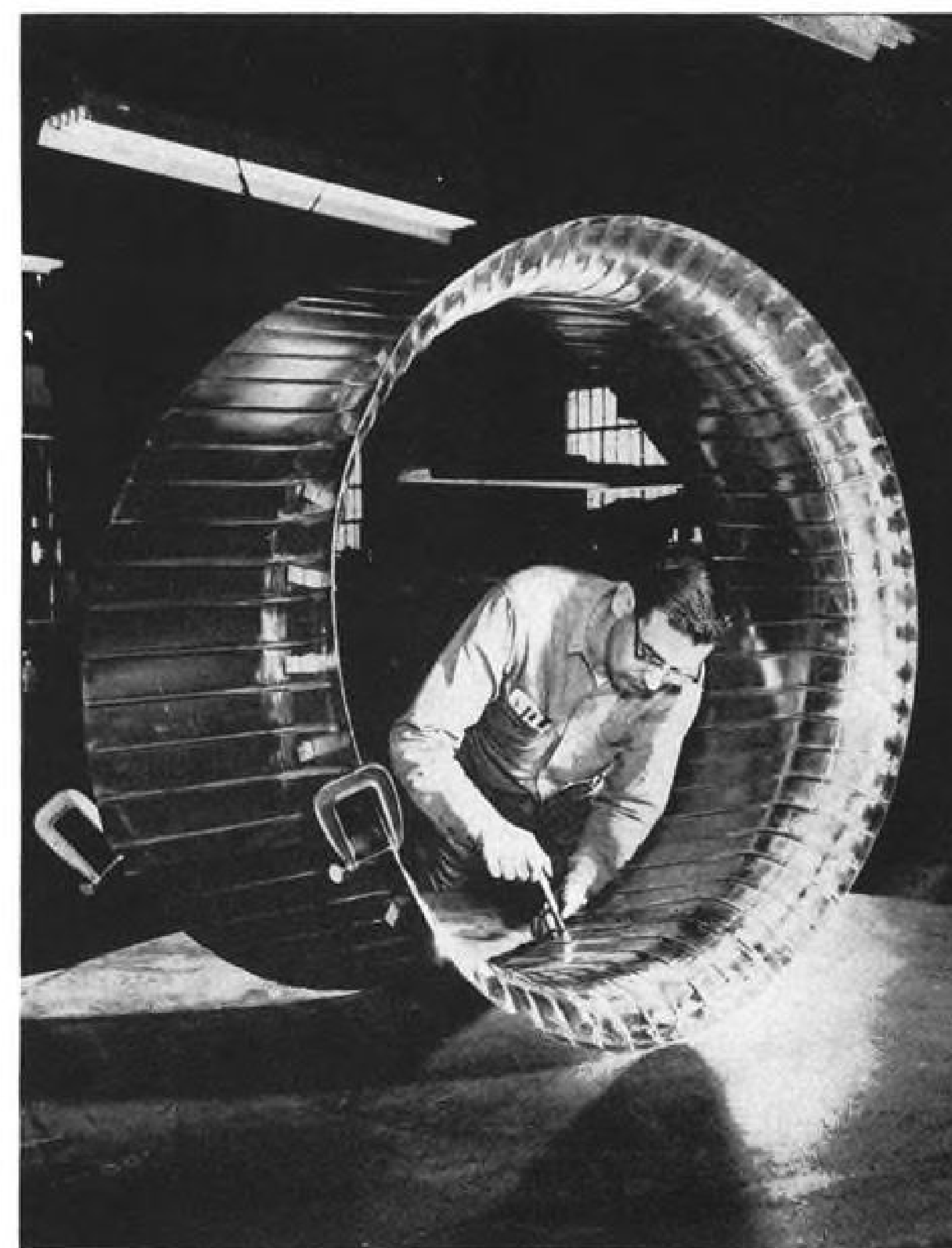
RAMJET NOZZLE LINER (left) and ramjet nozzle housing (upper and lower right) are two Curtiss-Wright subcontractor-made parts which match in size and placement of attachment fittings. They probably are for the North American Navaho missile. The 48-in. diameter ramjet on which these would be used would have a thrust of 30,000-40,000 lb.
