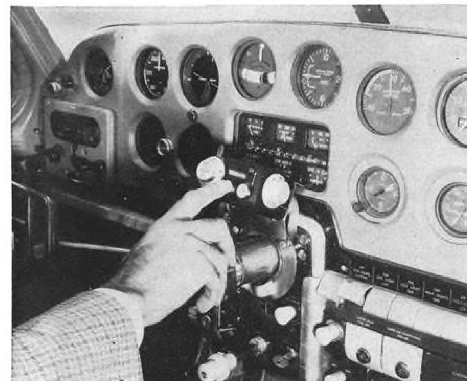
TACTAIR T-3 CONTROL HEAD has two pairs of aneroid capsules (right) which transmit commands from control knobs to control servos.
