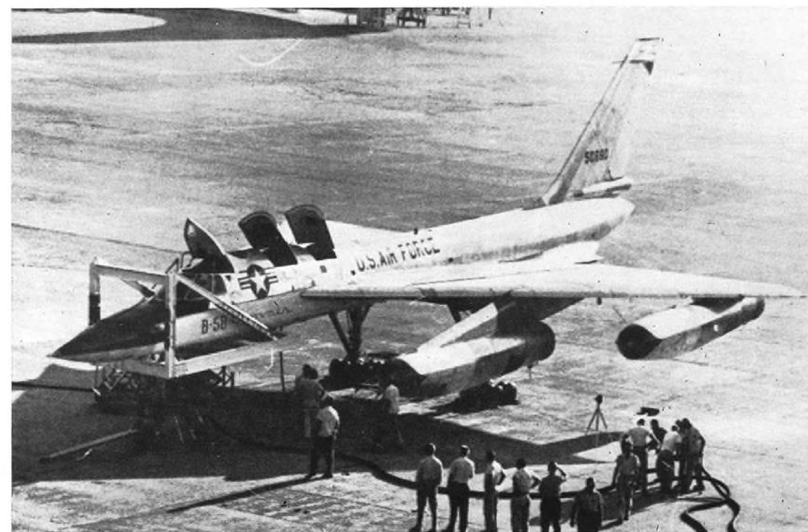
CONVAIR XB-58 shows use of conical camber to solve high subsonic cruise condition, permit supersonic dash speeds.
