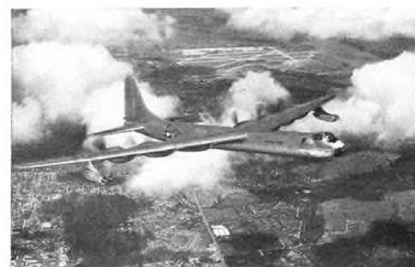
1949 Convair B-36 is armed with a complete G-E defense system including turrets, sighting stations, radar control and a G-E electronic computer.
