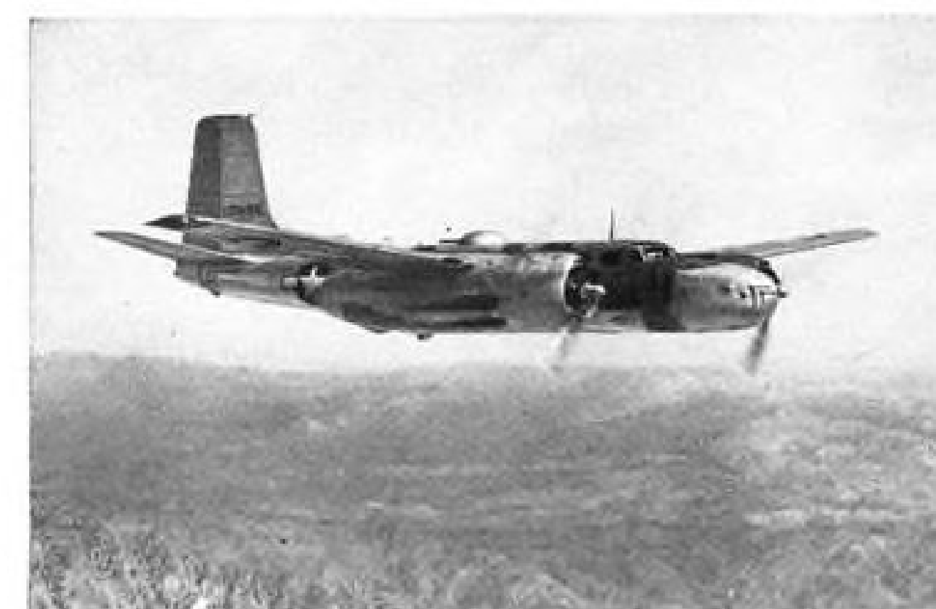
1944 G-E control and turrets linked with a periscopic sight allowed Douglas B-26 gunner to aim and fire both upper and lower turrets by remote control.
