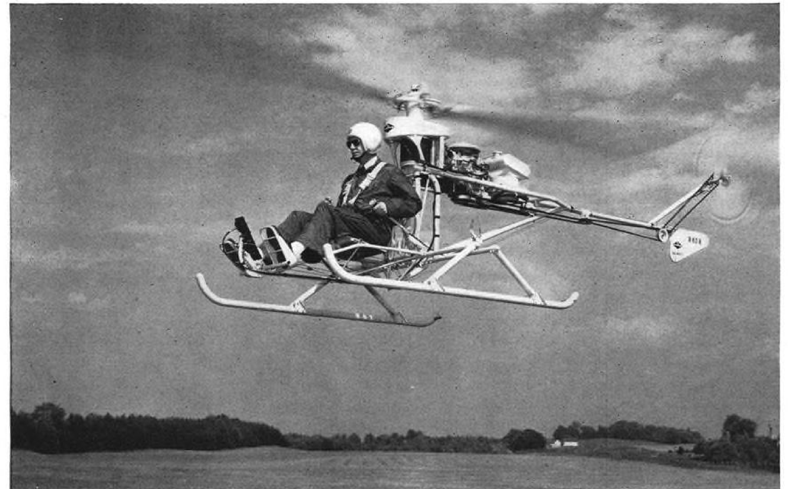
LIFTING characteristics of Airmat fabric rotor blade will be studied by Goodyear Aircraft Corp. engineers after mounting on GA400-R Gizmo one man helicopter. Tests are scheduled to begin early next year.
