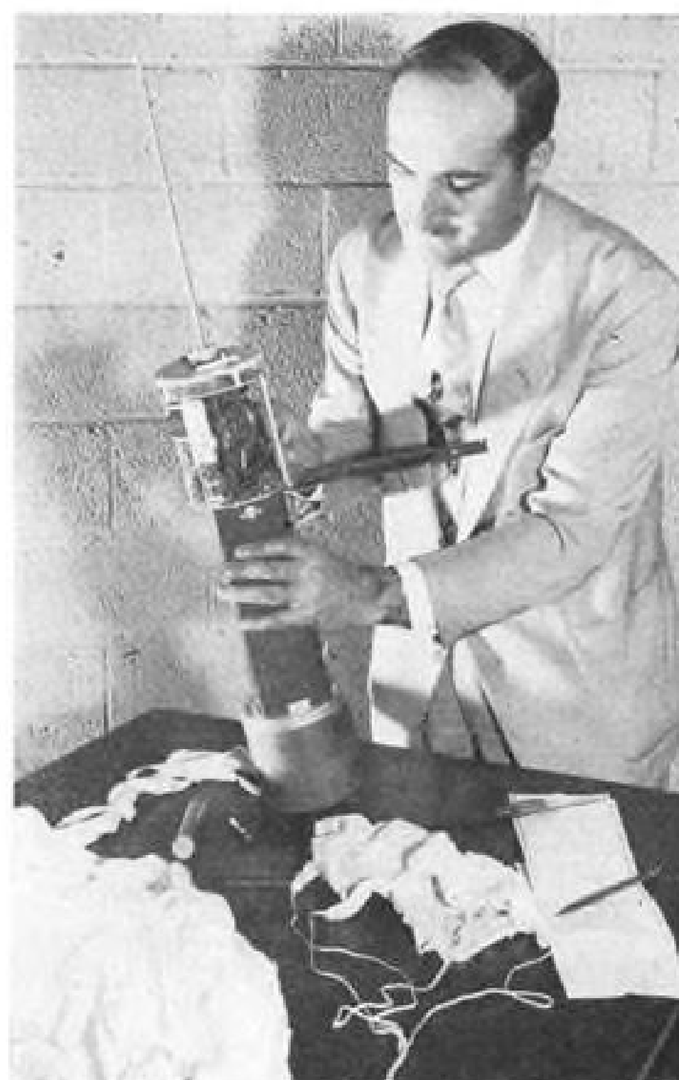
NEW RADIOSONDE developed by ARDC is adjusted for pressure setting by Wilson A. Maxim of Wright Air Development Center Aerial Reconnaissance Laboratory.
