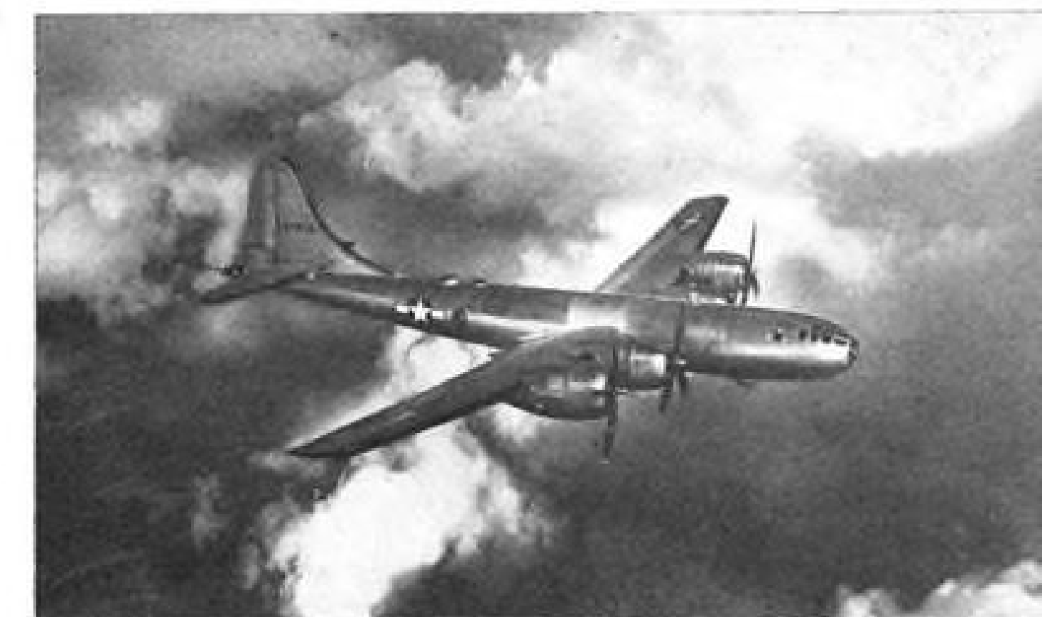
1942 Boeing B-29 Superfortress was defended by the first remote-control armament system including General Electric controls and turrets.
