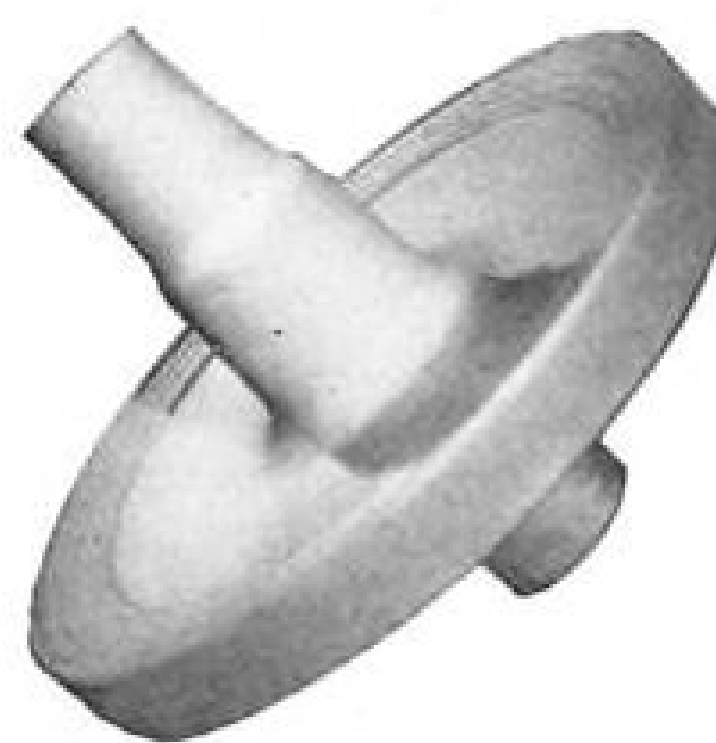
At the bottom left is a turbine disc forging made from high density heat resisting alloy, and next to it is a titanium compressor wheel forging for two of the most powerful jet engines yet produced.
