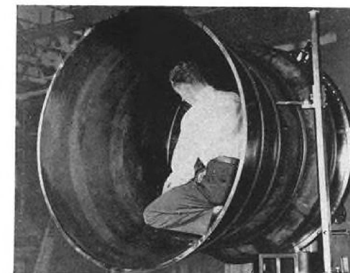
RAMJET NOZZLE LINER (left) and ramjet nozzle housing (upper and lower right) are two Curtiss-Wright subcontractor-made parts which match in size and placement of attachment fittings. They probably are for the North American Navaho missile. The 48-in. diameter ramjet on which these would be used would have a thrust of 30,000-40,000 lb.
