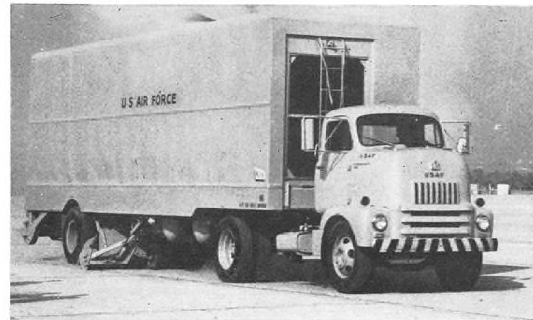
RUNWAY vacuum cleaner made by Coleman Engineering Co. has nozzles in low front unit. Hoppers for debris are mounted under separator drums in center.
