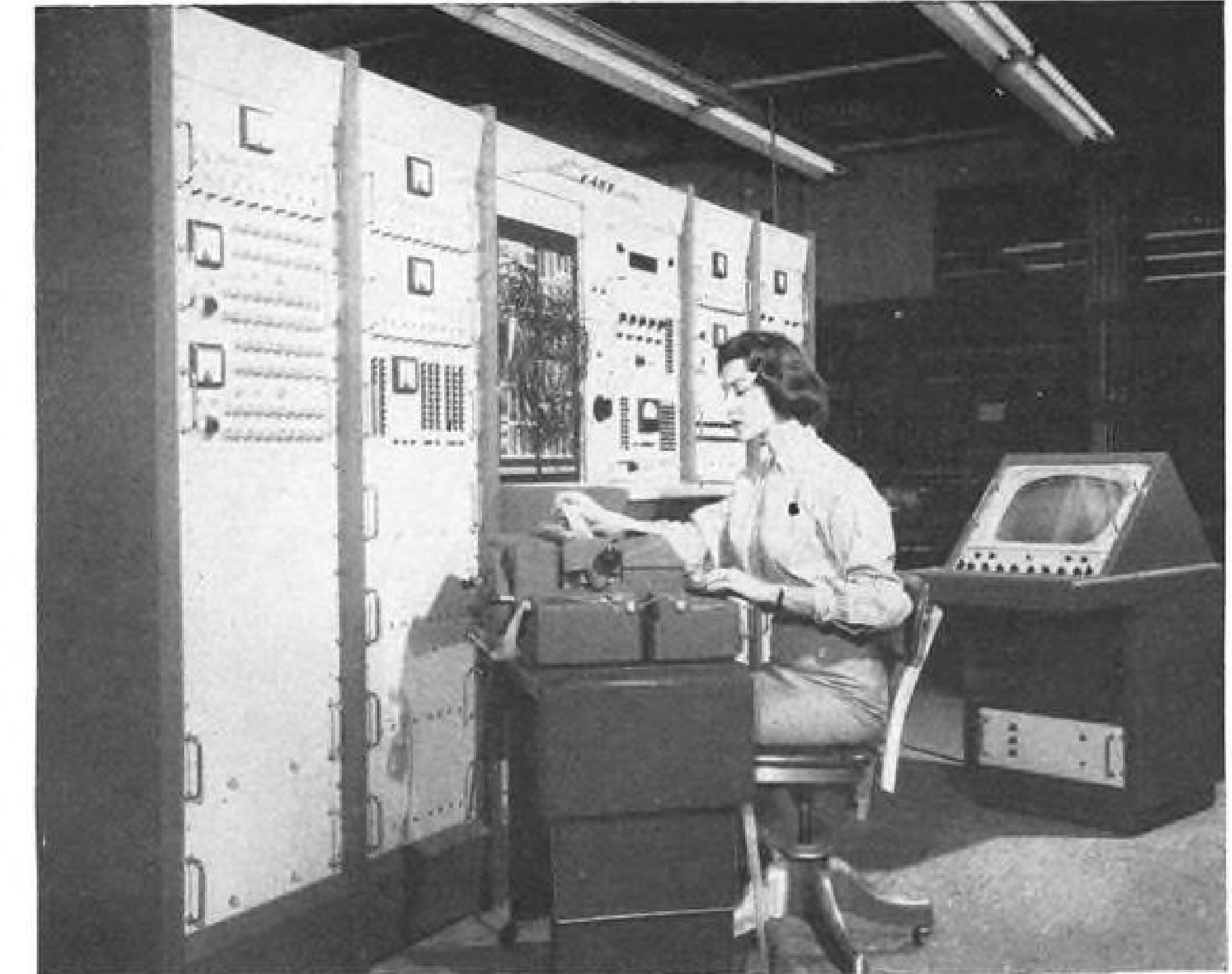
NEW analog-digital computer uses punch tape programming to set up problem automatically and record its solution on tape, increasing flexibility, utilization.
