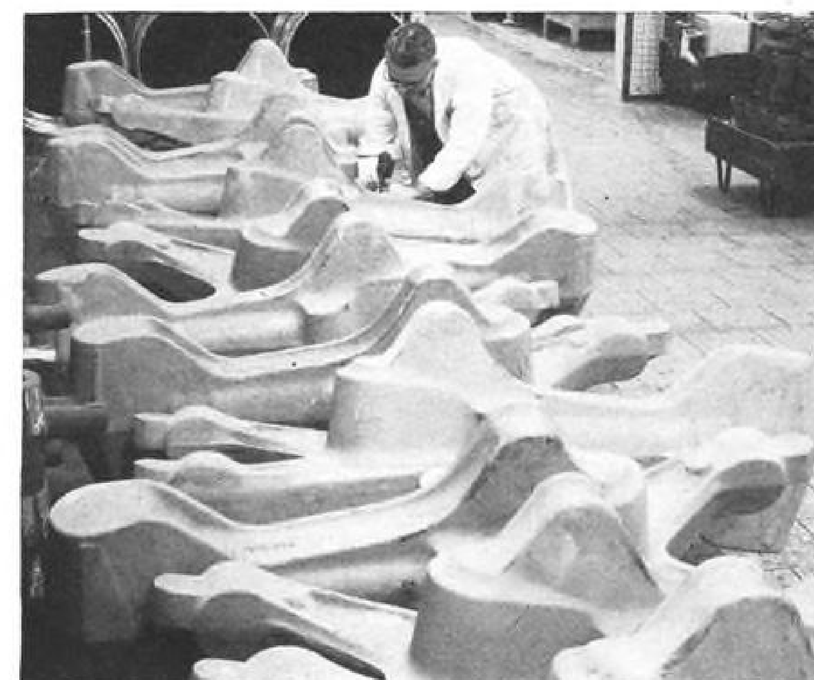
FORGINGS of upper part of main landing gear legs are inspected.
