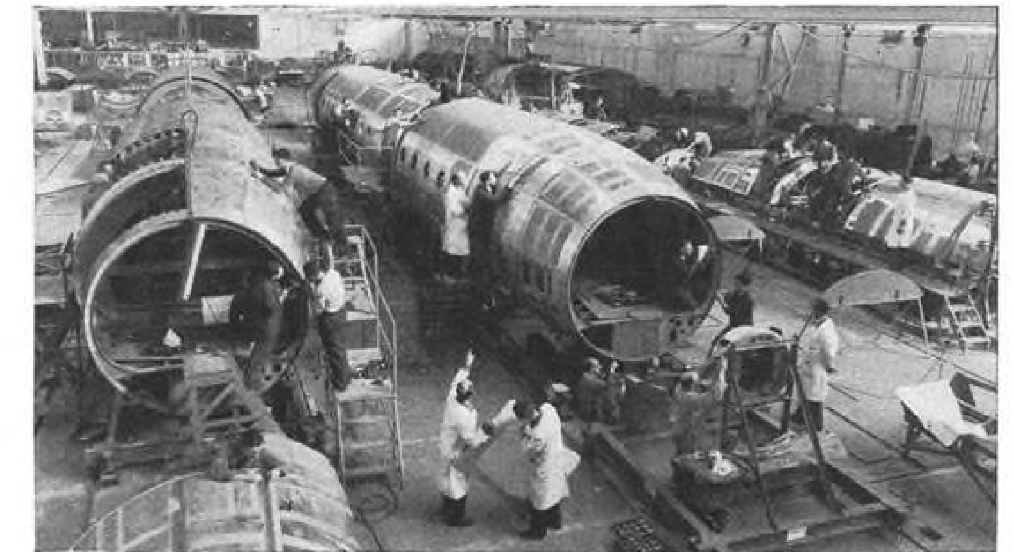
DOUBLER is installed around hatch in Comet 4 fuselage.
