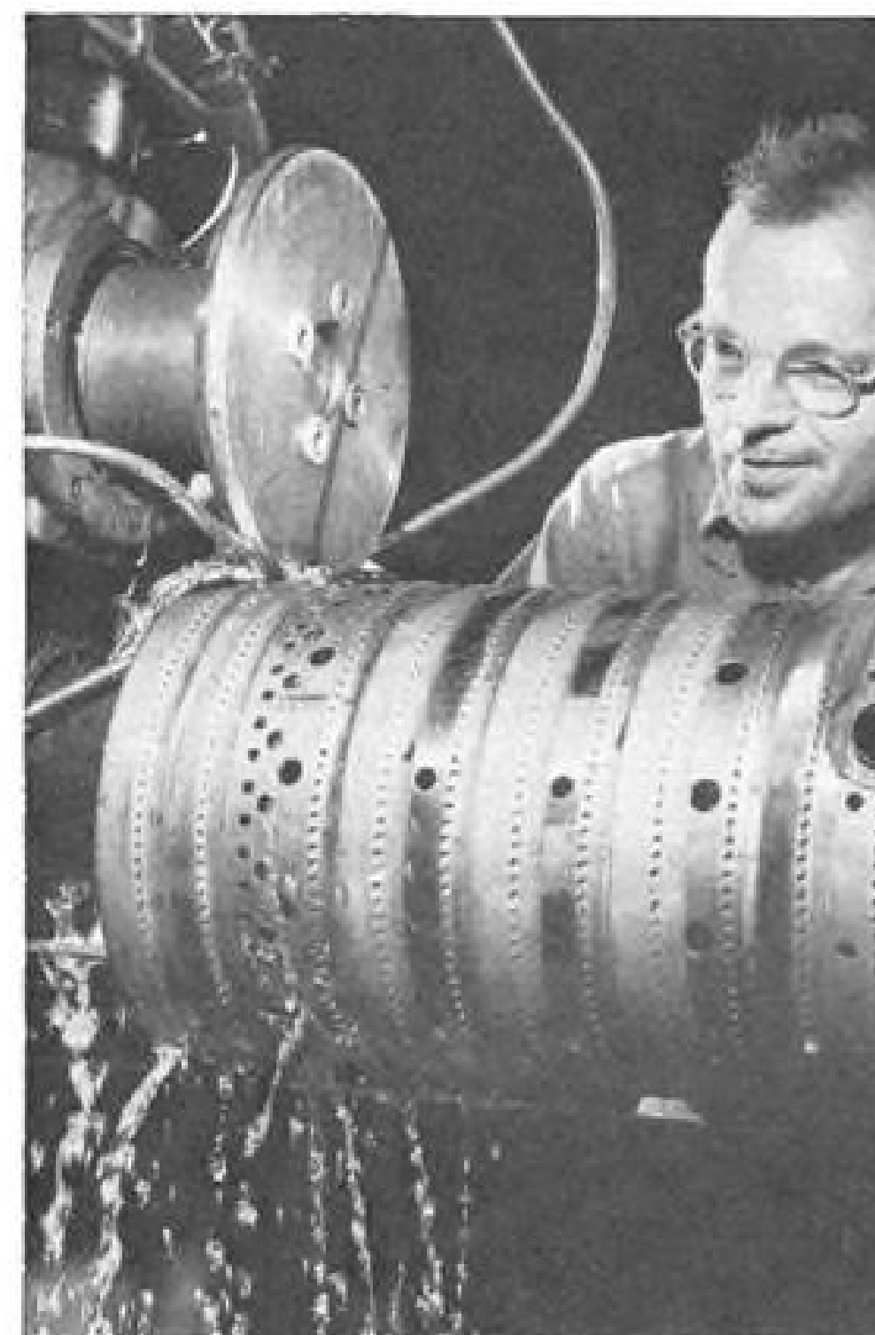
COMBUSTION chambers are resistance welded by water-cooled welding wheels. Welding is used on 76 major J57 parts.
