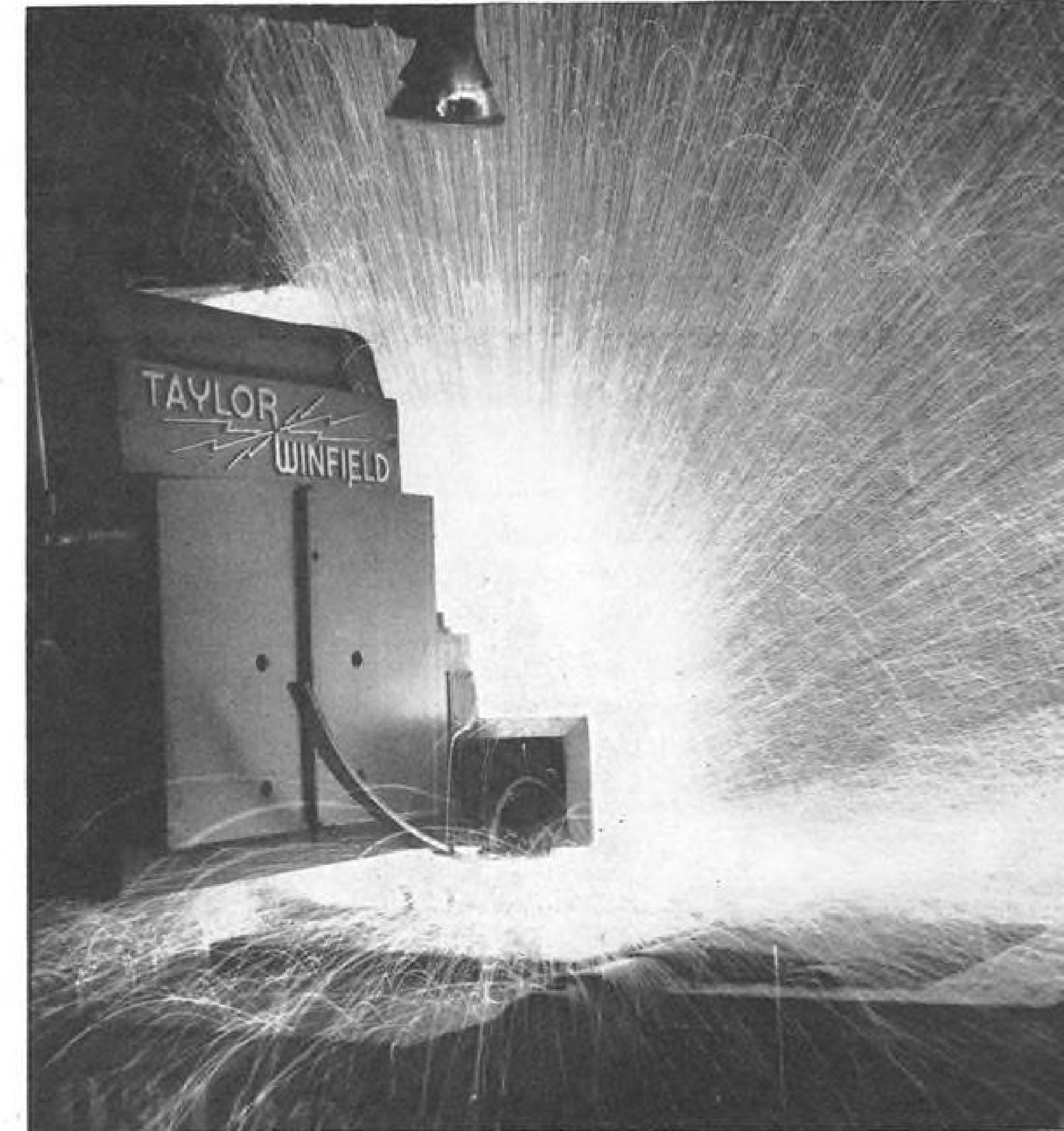
FLASH butt welding machine welds titanium at 3,200F. Electricity is used to erode portions of the titanium parts while they are being forged together.
