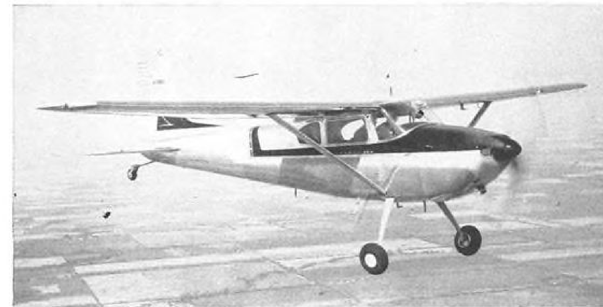
NEW INTERIOR and castoring landing gear are standard equipment in 1957 Model 180.
