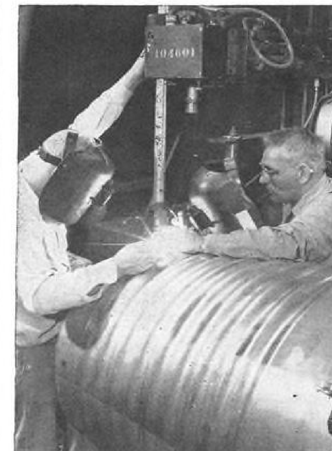
IN THIS fusion welding operation, inert gas is used to prevent contamination of nickel alloy component.
