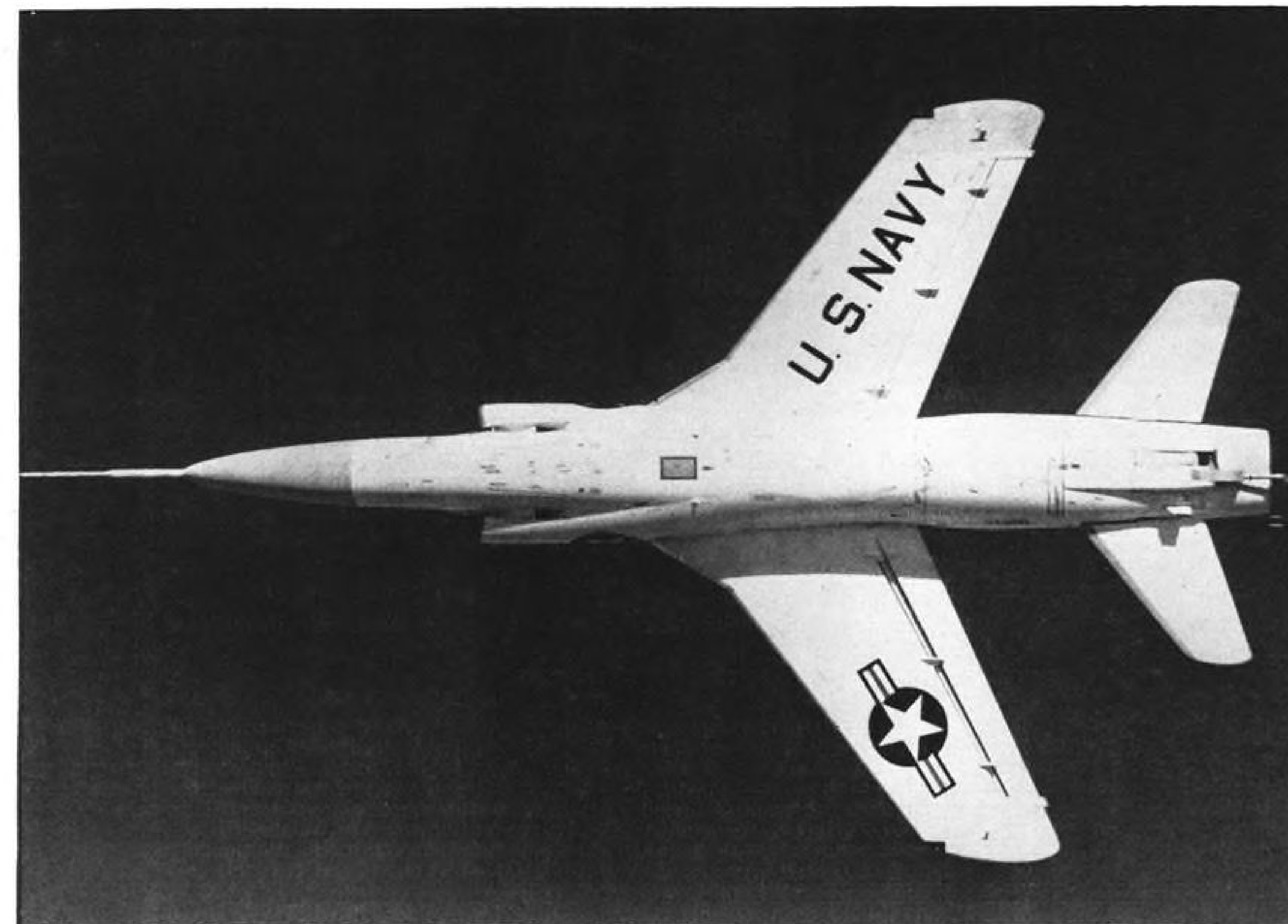
LARGER aft fuselage section was necessary to house J79 afterburner. Leading edge extensions improve supersonic speed stability.
