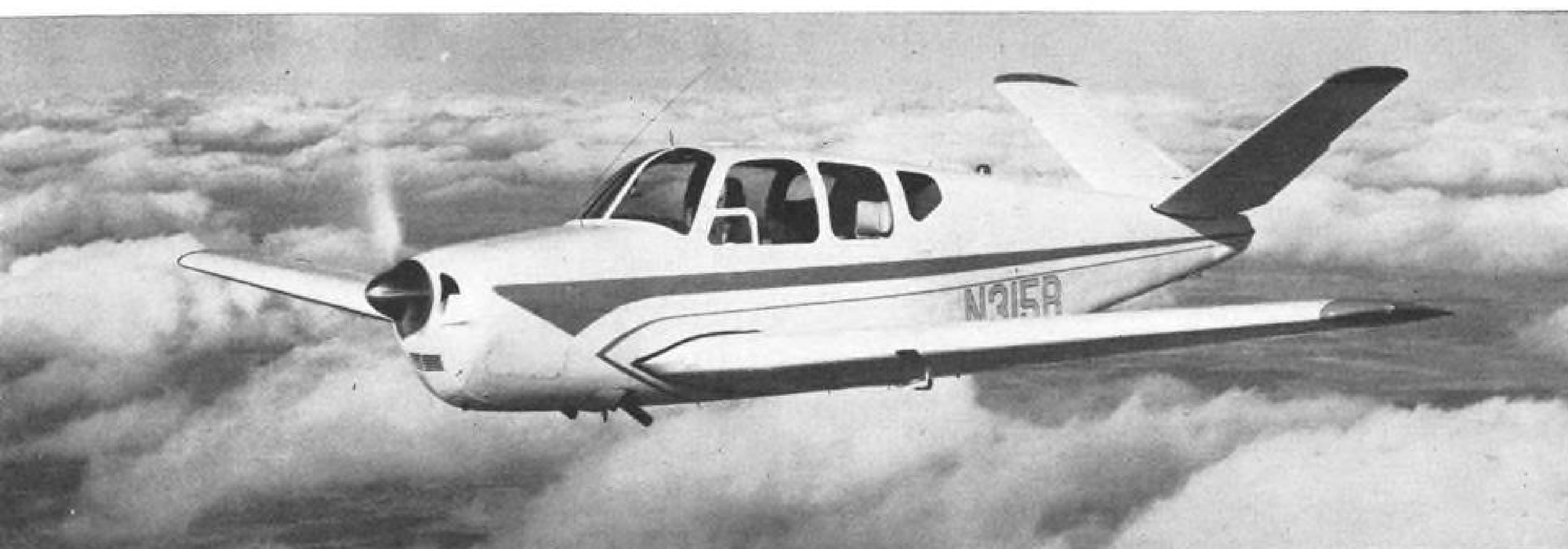
BONANZA H35 has more powerful engine delivering 240 hp.; eight-place E18S (below) has range increased to 1,626 mi. with reserve.
