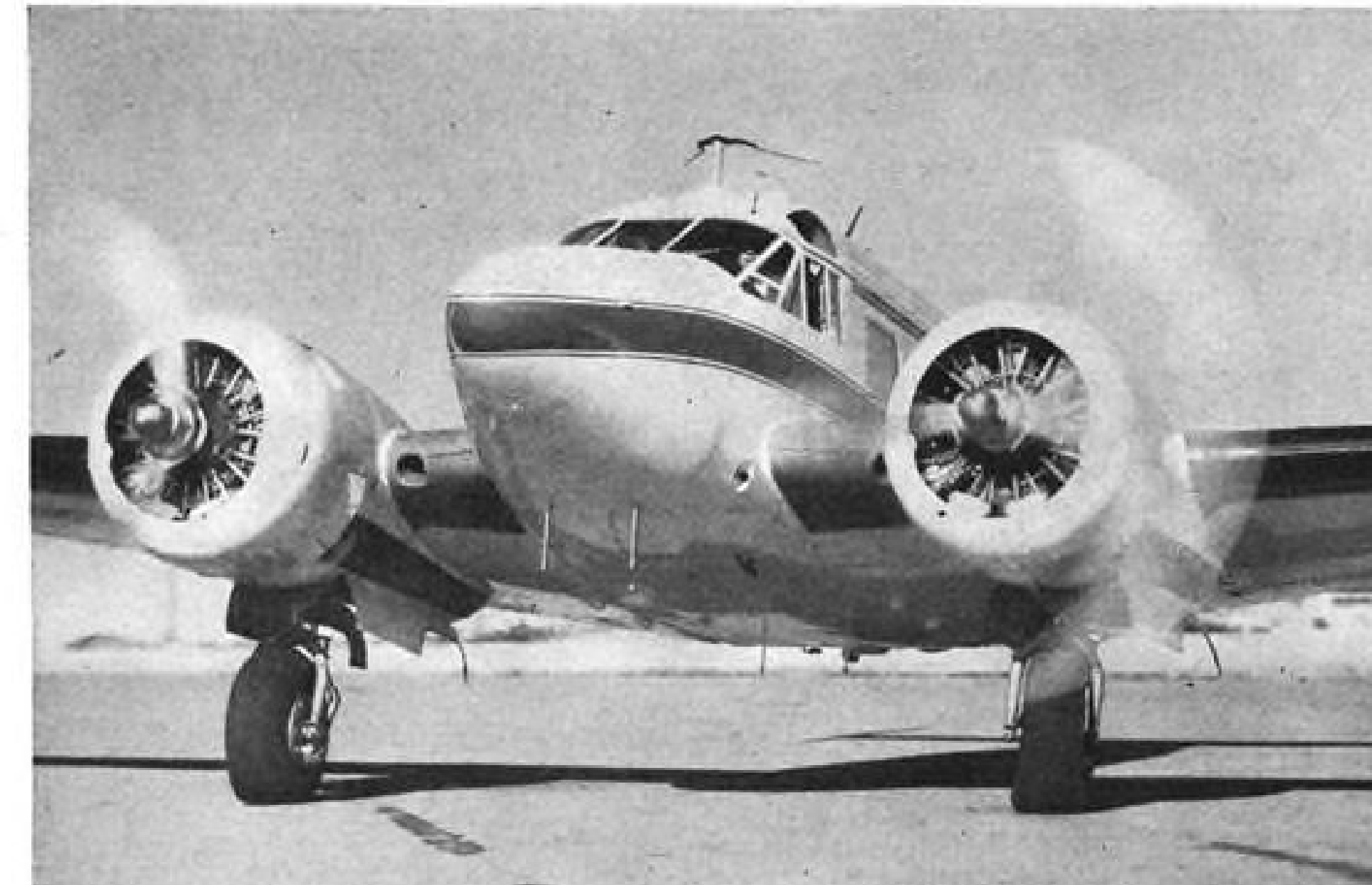
GEISSE CROSSWIND landing gear is being installed on majority of new E18S transports.
