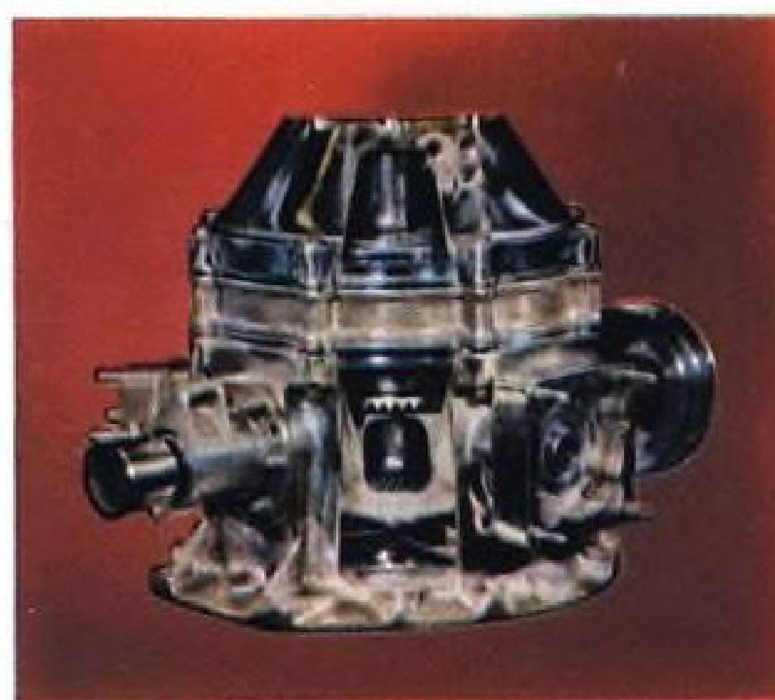
Bell 47-G transmission is one of over 100 parts produced by Kelsey-Hayes for the 47-G helicopter. Other products for the aviation field include accessory gear assemblies, actuators, computers, controls, bomb hoists, gun turrets, radar tracking and scanning assemblies, power recovery units, compressor rotors and turbine sections, blades, buckets, vanes.
