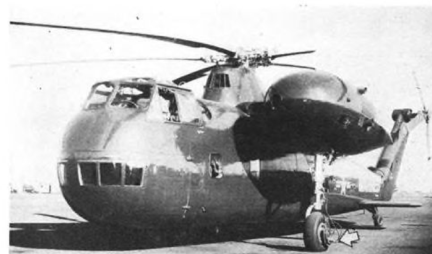
FIRST PICTURES of a hydraulically-powered taxi motor mounted on the main wheels of a Sikorsky HR2S-1 helicopter. Device is used to taxi the machine when its rotor blades are folded. Forward speed and turns are controlled through main engines which drive pumps powering individual motors. Units may be quickly removed from wheels when not needed.
