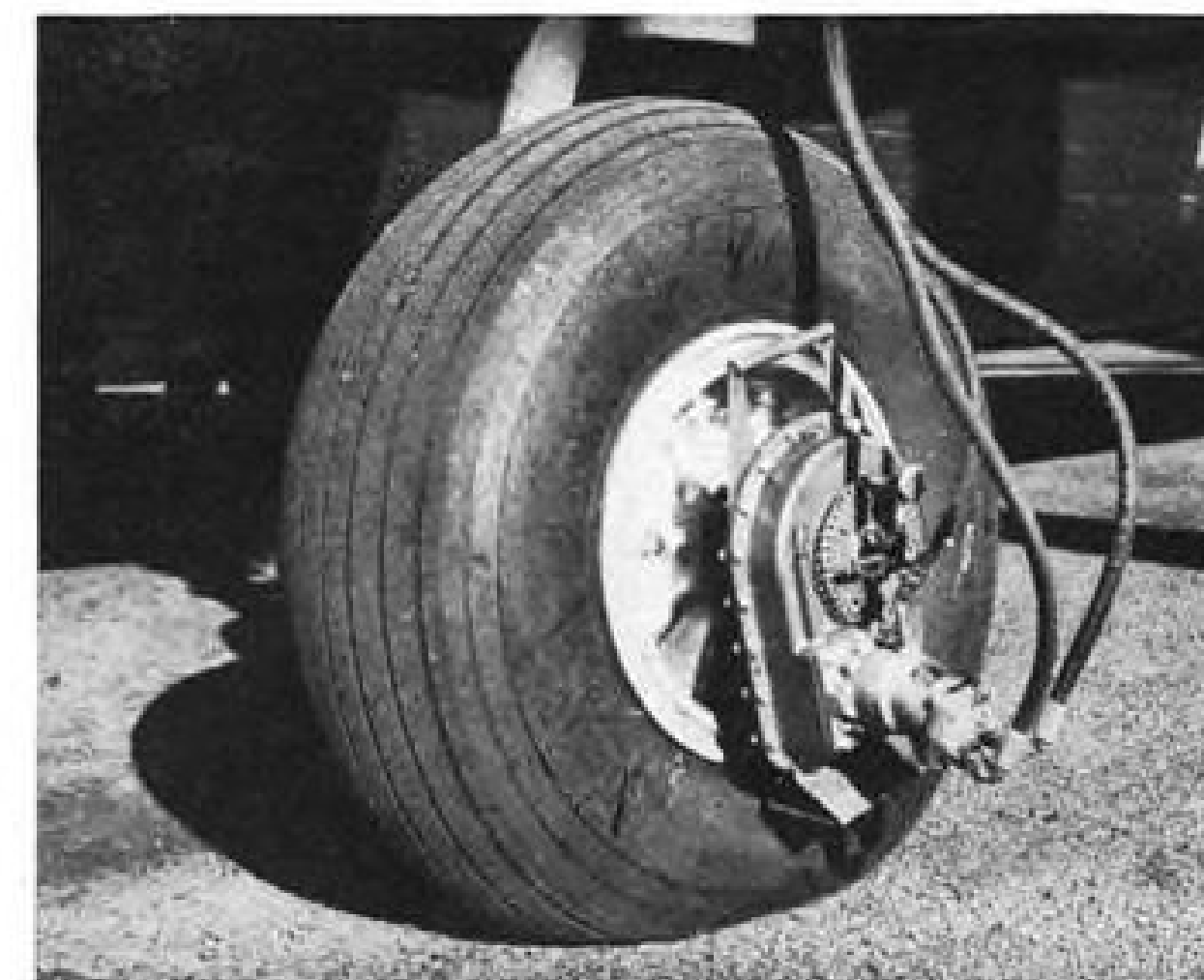
FIRST PICTURES of a hydraulically-powered taxi motor mounted on the main wheels of a Sikorsky HR2S-1 helicopter. Device is used to taxi the machine when its rotor blades are folded. Forward speed and turns are controlled through main engines which drive pumps powering individual motors. Units may be quickly removed from wheels when not needed.
