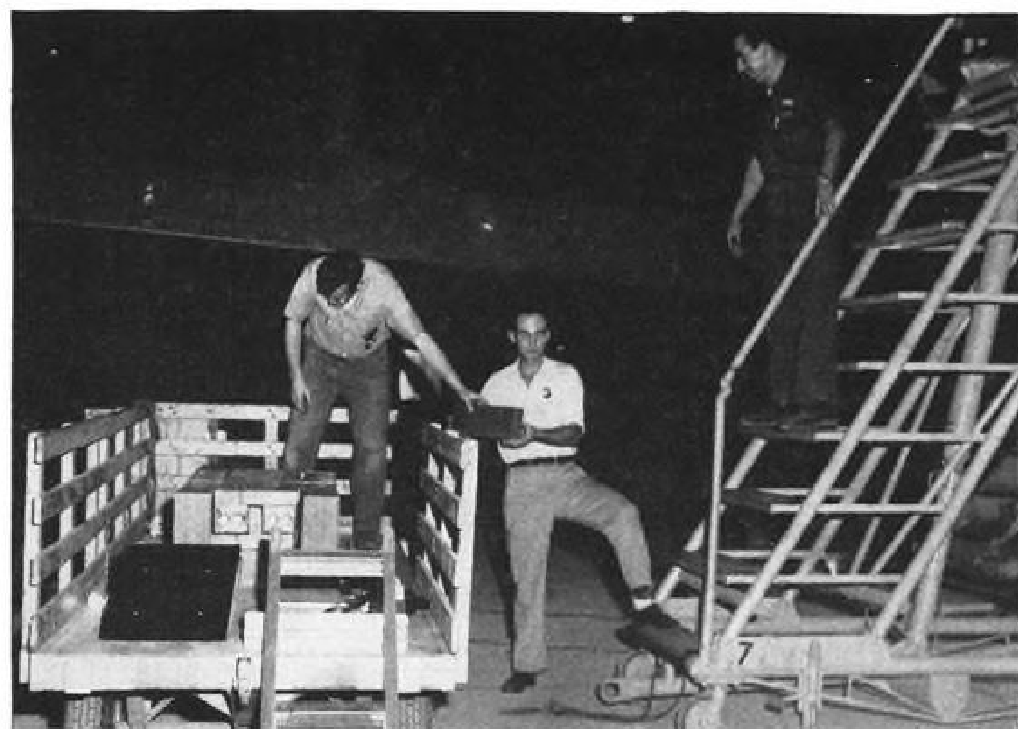
NEUTRON PILE is taken apart and lead and paraffin blocks are restacked in the KC-97. Ends of neutron counting ion tubes are visible in part of the pile in truck.
