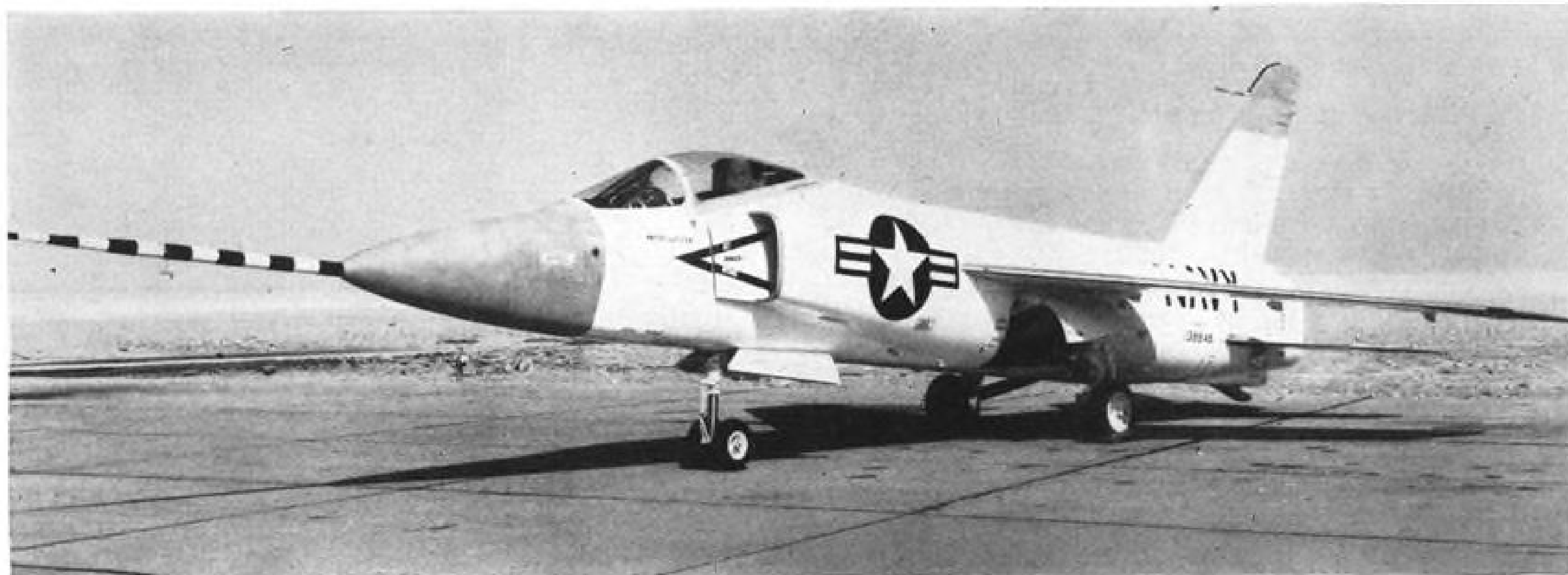
MODIFICATIONS of F11F with J79 installation include larger engine inlet ducts. Single-pane clear windshield was added.
