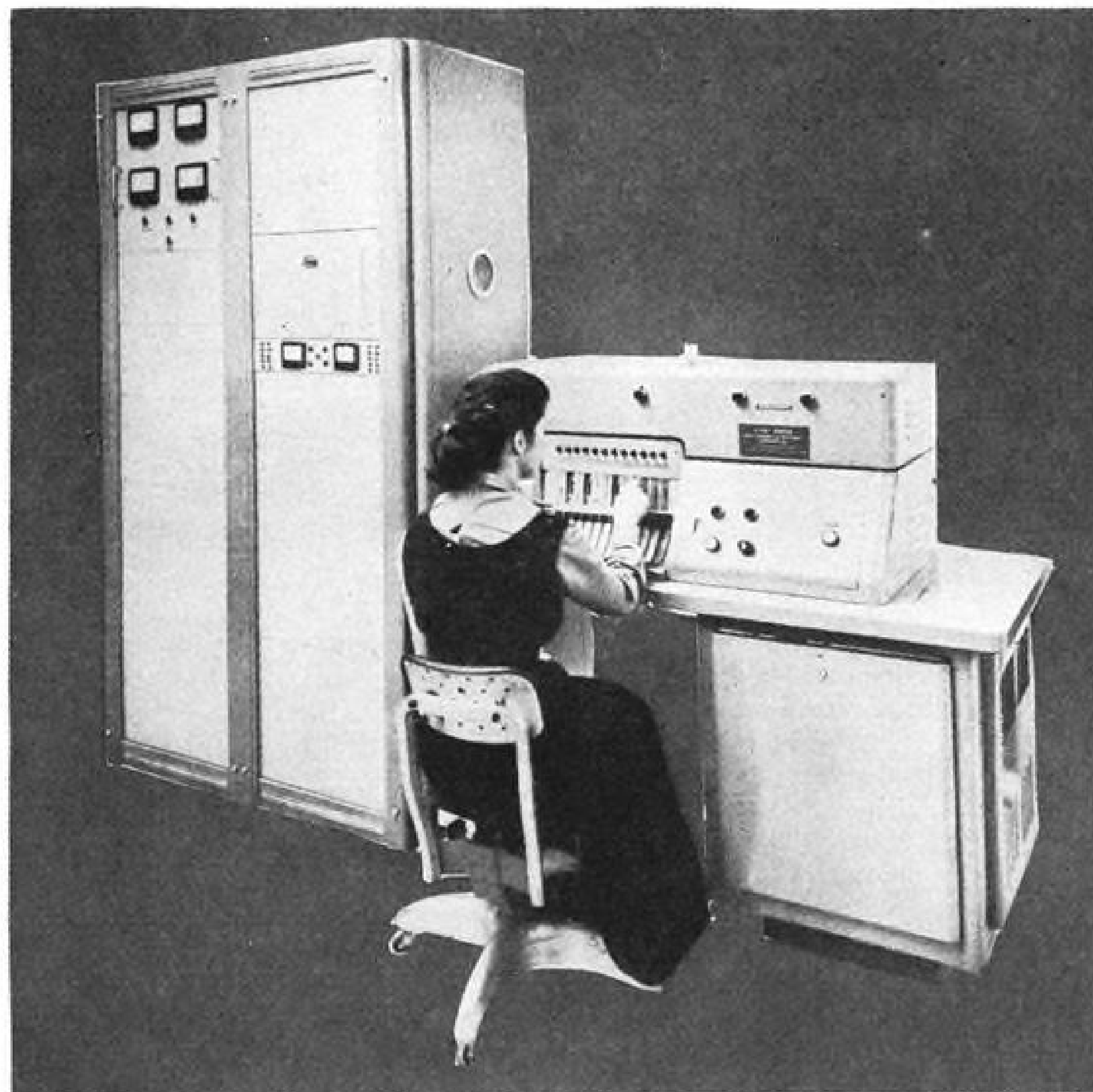
CRYSTAL blank X-ray sorter checks 43 pieces per minute, can be operated by unskilled worker. Blanks arrive in plastic cartridges and are sorted into similar marked cartridges.
