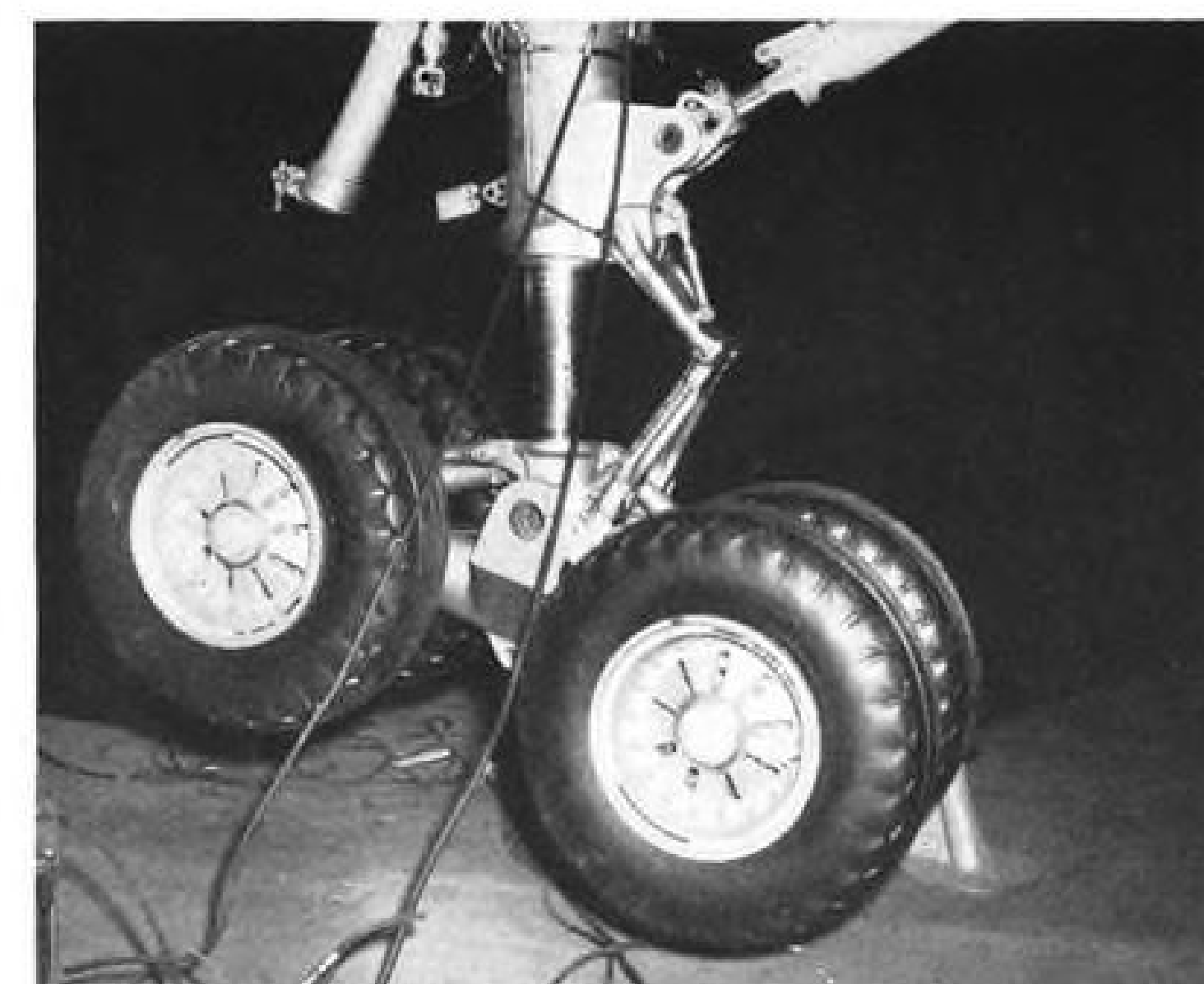
1. CL-28's MAIN, bogie landing gear starts retracting. For storage-clearance considerations, four-wheel bogie is folded through 60 deg.
