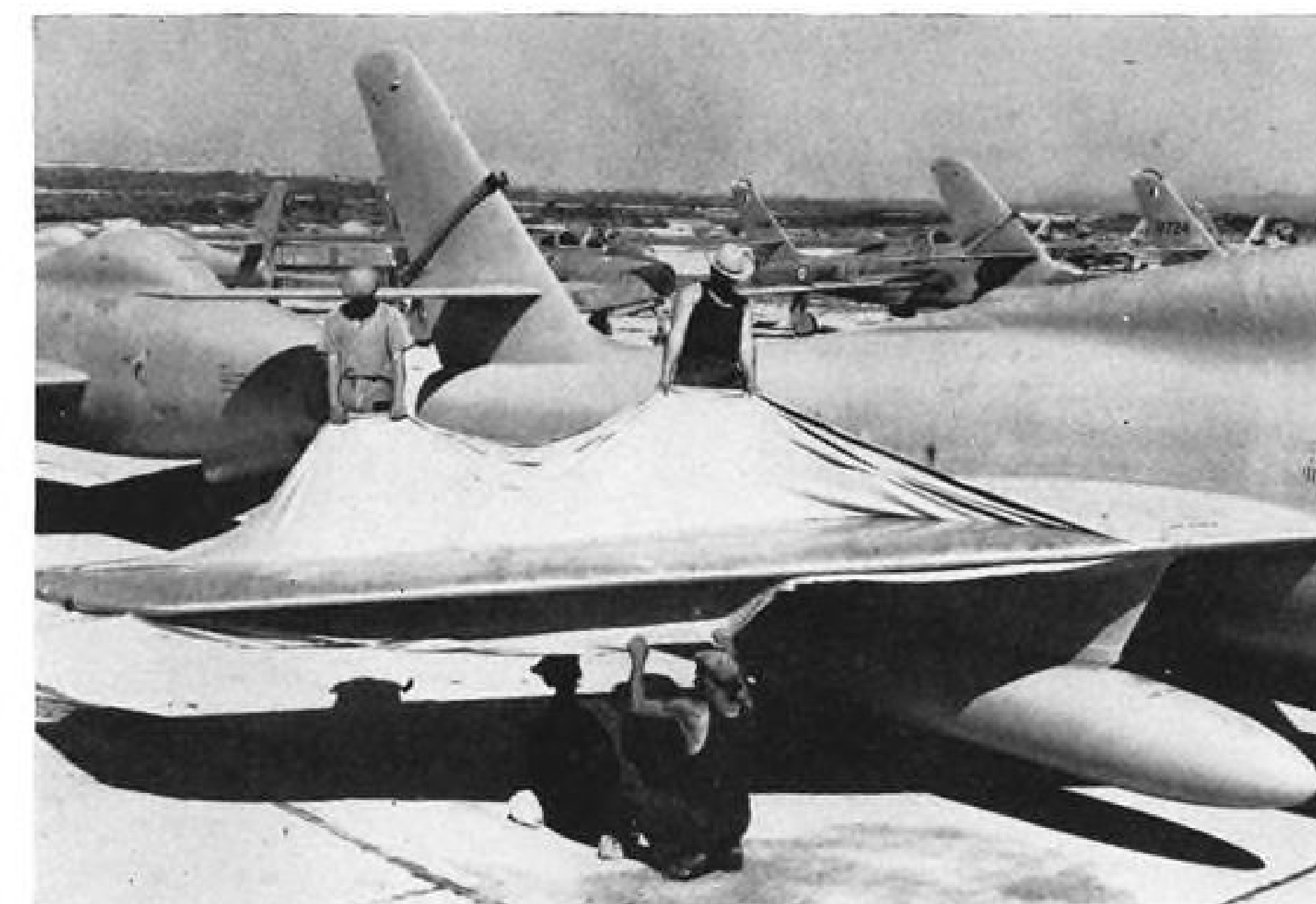
DE-COCOONING (removal of heavy plastic coating), washing down of aircraft to arrest corrosive effects of sea spray, are done before modification work starts.
