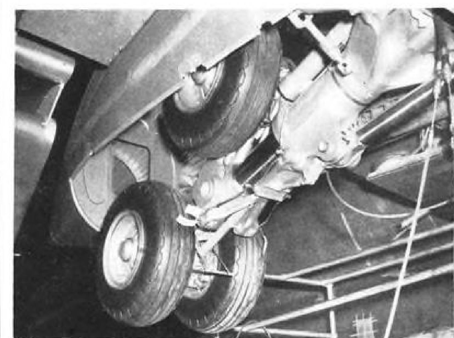
3. AS LANDING gear nears fully retracted position, bogie folding is almost complete. Main and nose gear on CL-28 fold rearward. 4. HERE MAIN LANDING gear is almost completely retracted with four-wheel bogie tucking into aft part of inboard engine nacelles.
