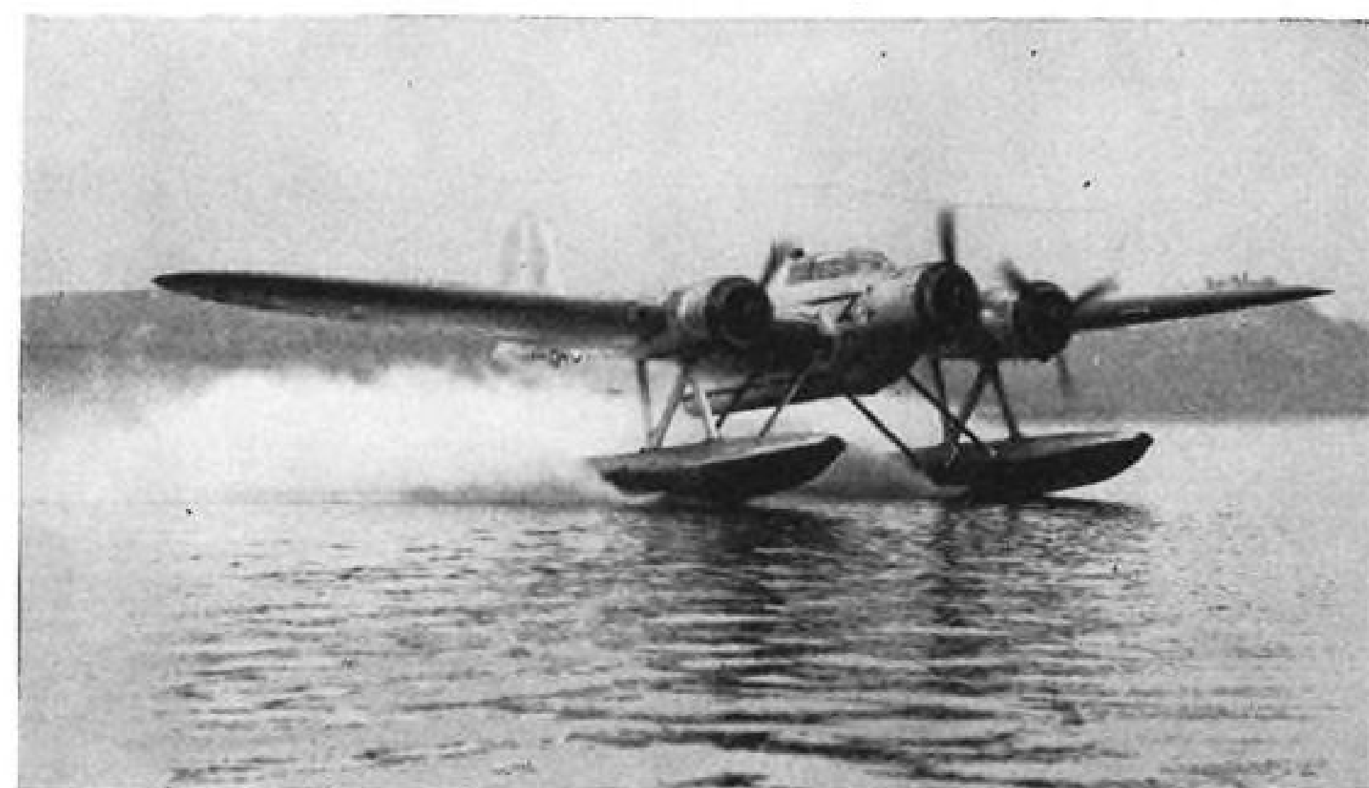
Cant Z.506 tri-motored seaplane, on the step, is one of major members of Italian air aid squadrons. Plane is used for long-range rescue missions, such as flying to pick up injured or sick crewmen on a tanker in the Mediterranean. Designed in 1936, the Cant is all-wood, and grosses about 27,000 lb. Wingspan is 87 ft.; powerplants are Alfa Romeo 126 R.C.34 engines rated at 750 hp. each. Cruise speed is about 200 mph.
