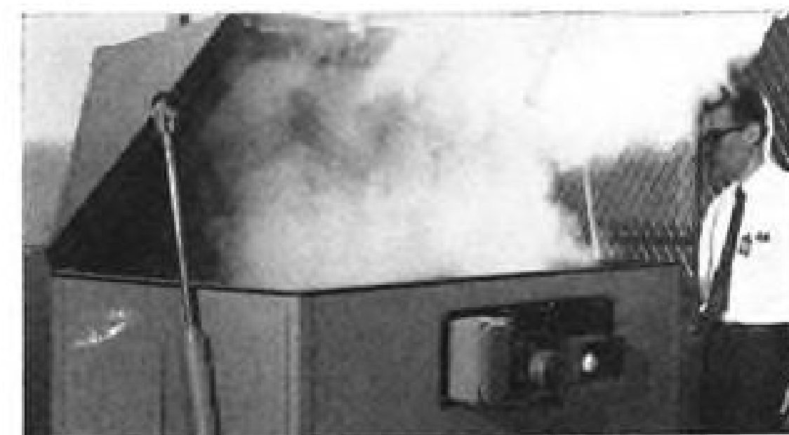
▲ Engineer at Ford Instrument Company opening salt spray chamber in which equipment for BuAer is being subjected to environmental test.
