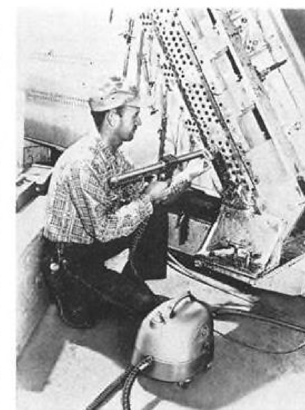
Chicago Pneumatic Tool Co., N.Y., makes this one-pass close-tolerance Broach Puller which operates off shop air. The Company claims that this tool will permit tolerances of plus-or-minus .0005 in. in one pass, even through sandwiches of dissimilar materials such as aluminum and steel.
