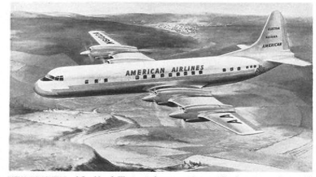
NEW DRAWING of Lockheed Electra turboprop revises nacelle shape to conform with Allison engine-Aeroproducts propeller combination, now flying on Super Constellation.
