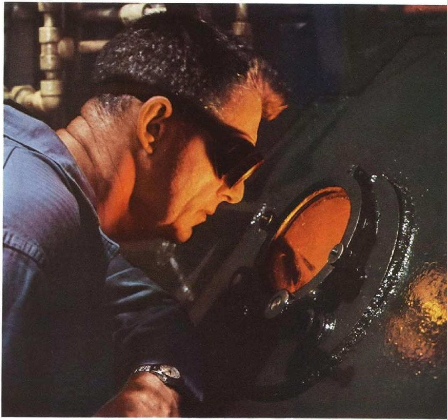
Utica technician viewing melt under a vacuum of approximately one-millionth of atmospheric pressure.
