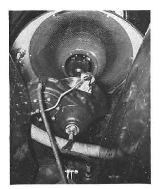
TURBINE inlet screen and firewall (background), drive shaft, rotor disk brake, turbine/transmission speed reduction unit and generator blast tube.
