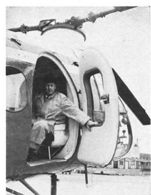
FORWARD CARGO DOOR is feature of Model 44. Cabin accommodates 600 cu. ft. of cargo; 2½ tons can be handled by an external cargo sling. Delivery of new civil copter could start next year. Airliner price will be about \$290,000.
