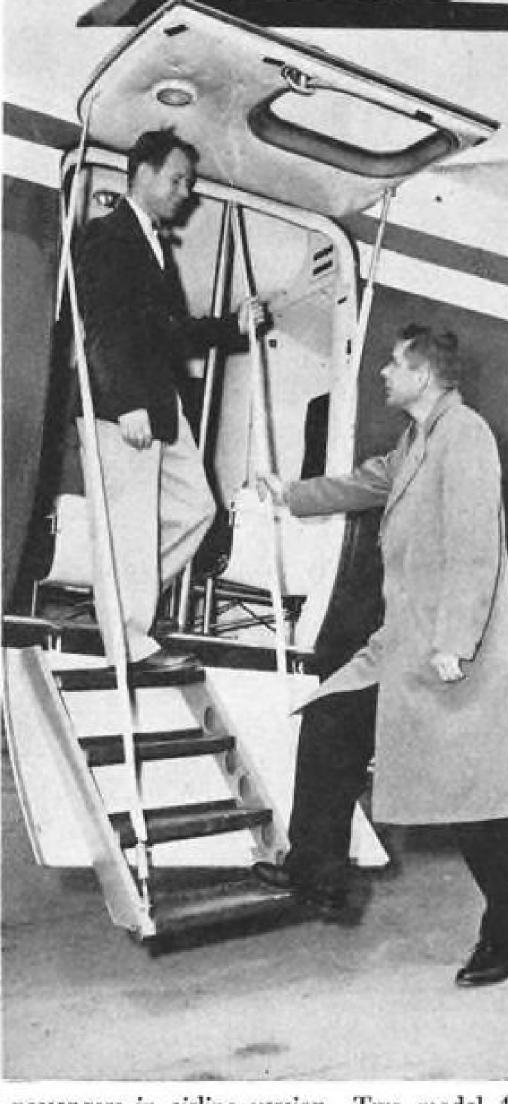
VERTOL COMMERCIAL HELICOPTER demonstrated last week at Philadelphia seats 15 passengers in airline version. Two model 44 aircraft displayed bear French markings (top left above). Cabin features soundproofing, carry-on baggage rack, clam-shell loading door.
