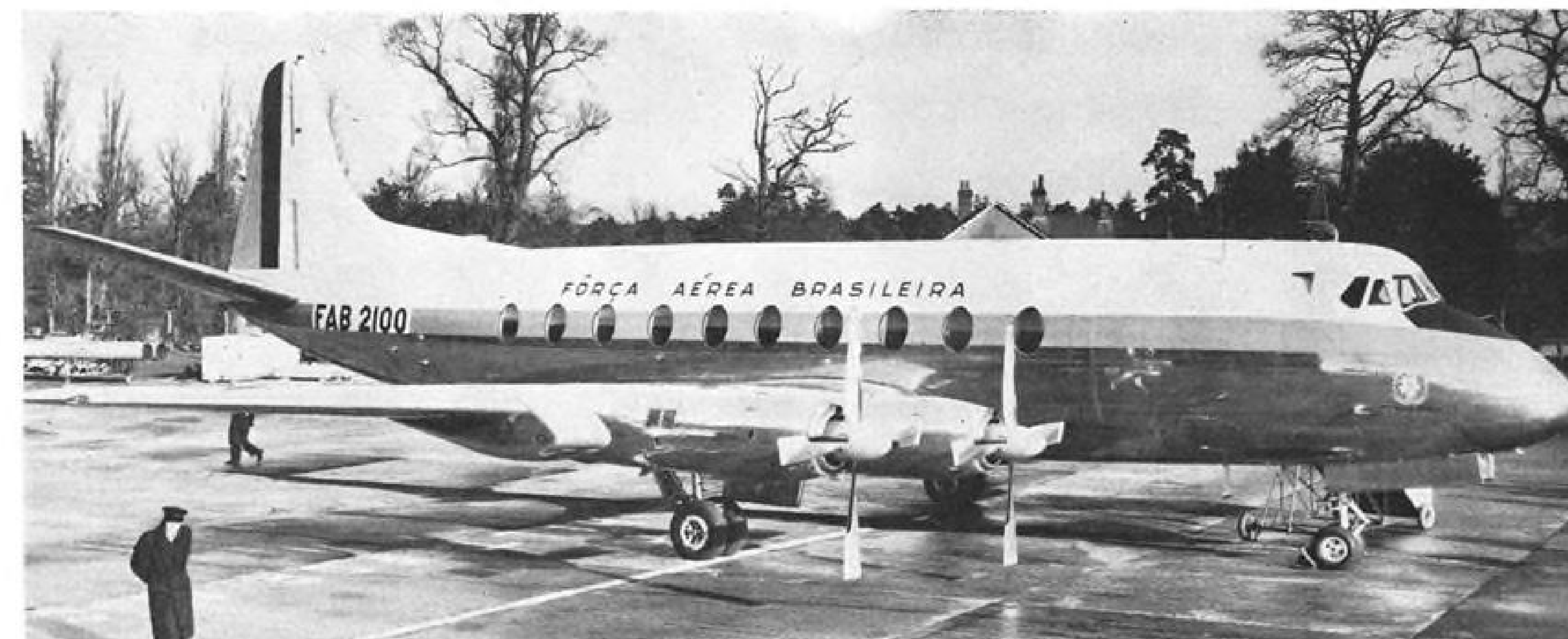
VISCOUNT used by Brazilian president carries auxiliary fuel tanks on undersides of wings outboard of Rolls-Royce Dart engines.
