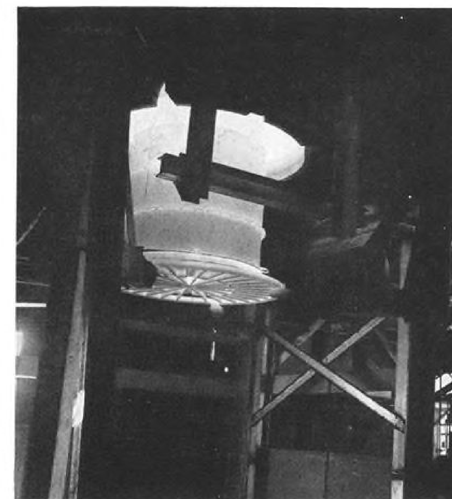
SOLAR OVEN is installed in its high-bay area (left). Work in muffle-box is being lowered out of white-hot oven (right).
