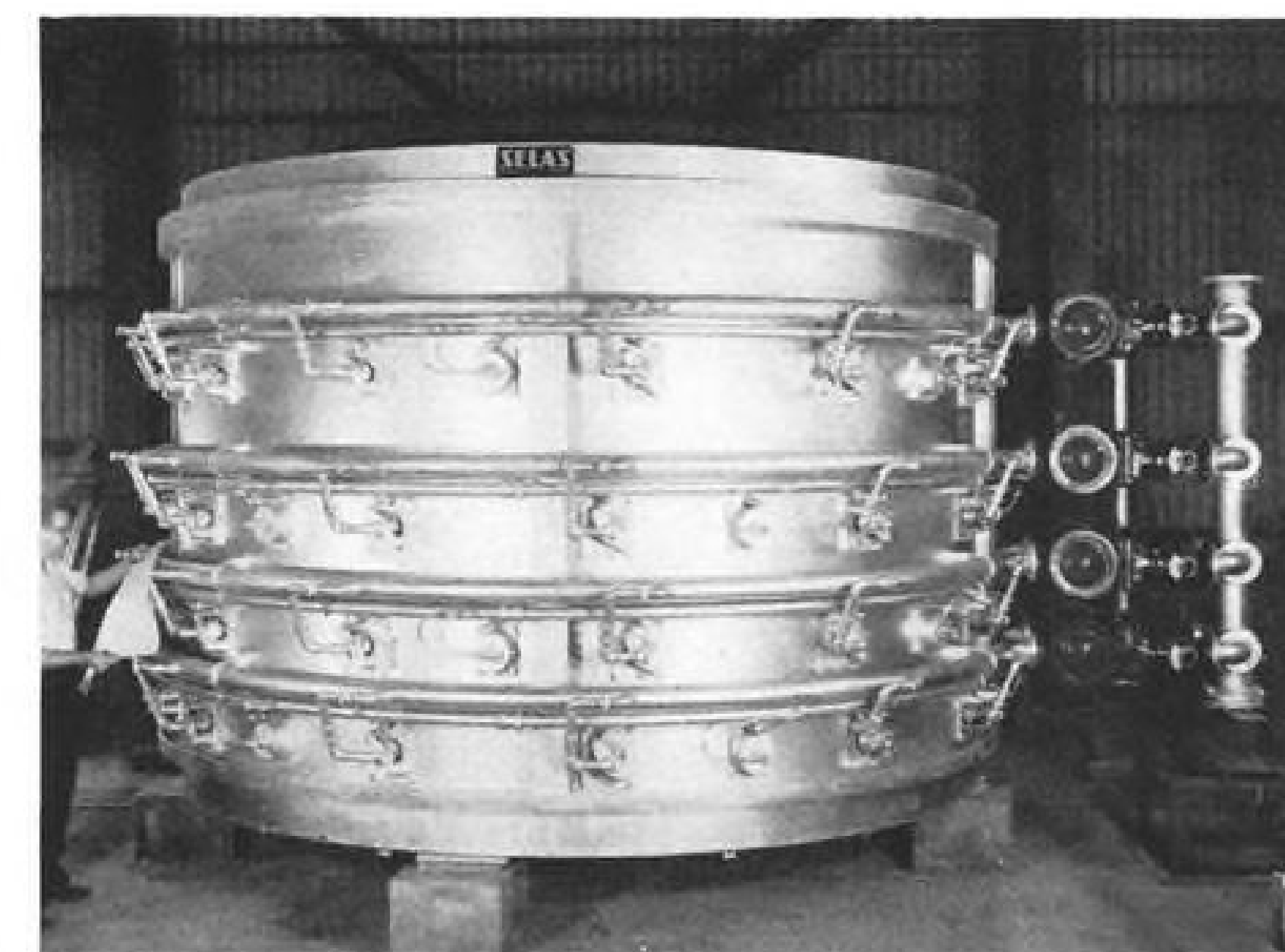
FAST AND SLOW gas burners inside the Twigg furnace (left). Outside view shows manifold system for burners (right).
