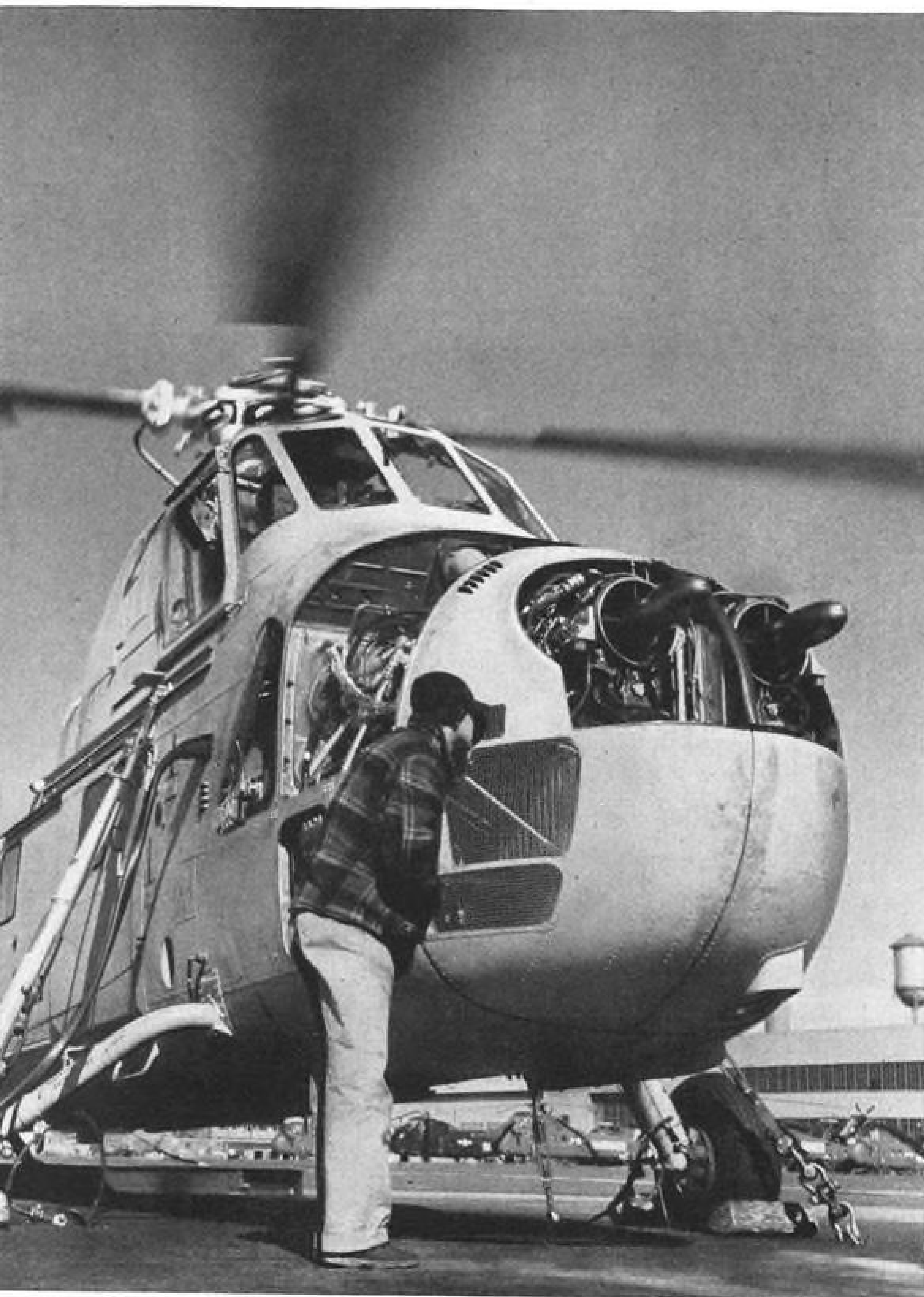
NOW BEING FLIGHT-TESTED in a modified Sikorsky S-58 helicopter, two T58 engines deliver more than 2000 horsepower, yet weigh only 650 pounds.
