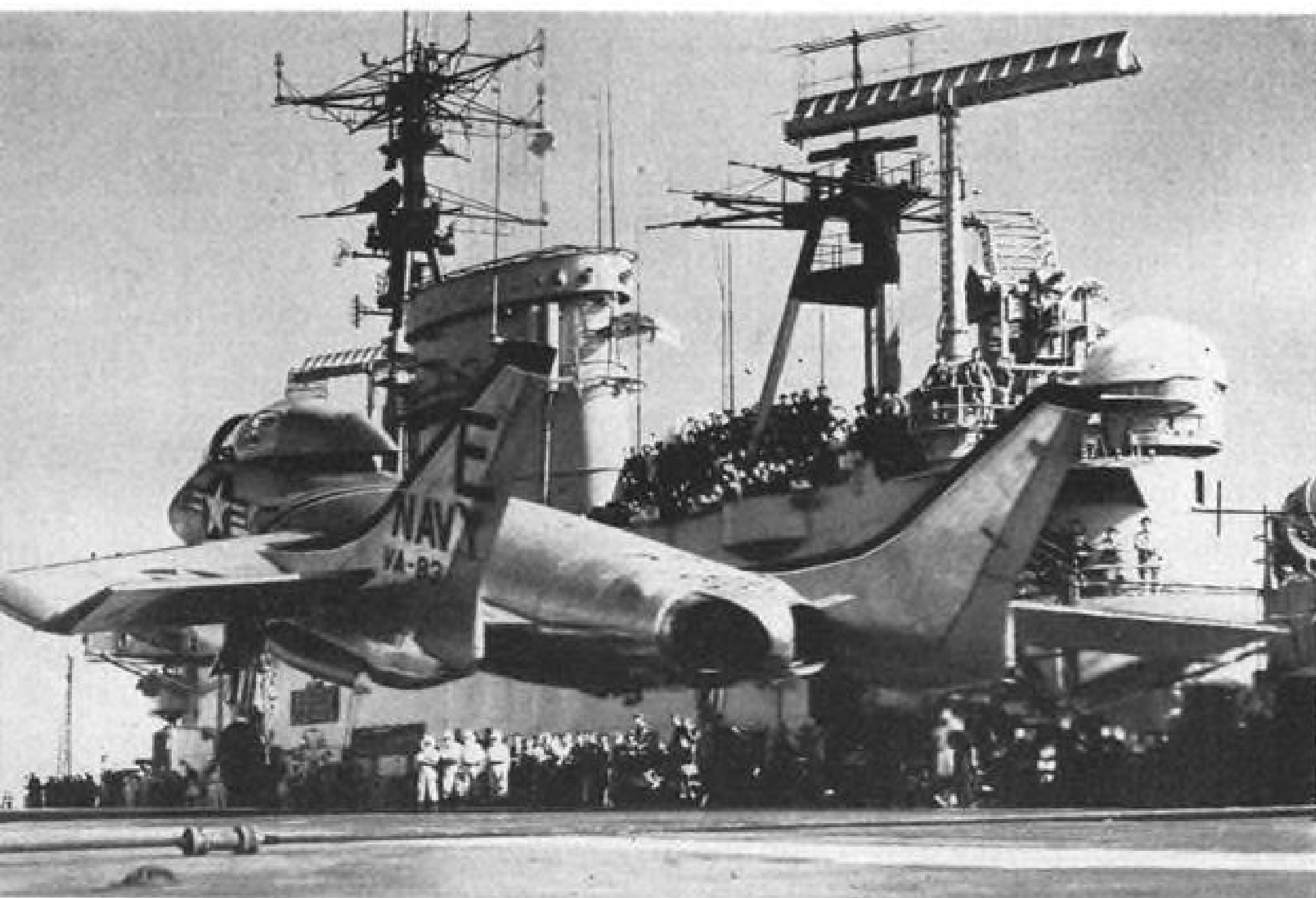
CHANCE VOUGHT F7U (above) has blunt ailerons to improve transonic stability. NACA used modified F-86 (below) to obtain transonic flight test data on the basic concept.
