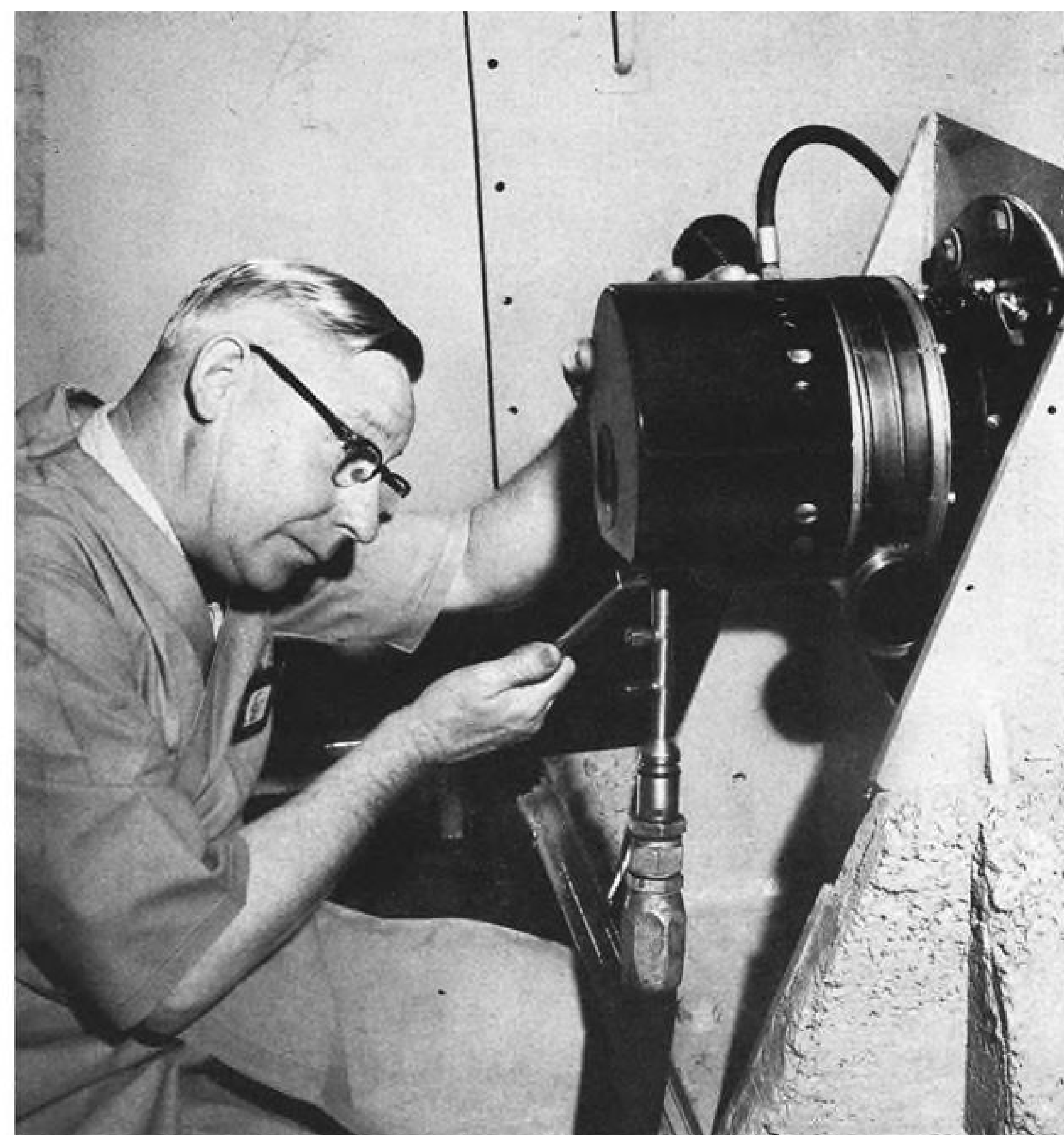
Production model of the General Electric fuel-air turbostarter for a current high thrust engine weighs only 46 pounds, has a 8 3/4 inch diameter and 12 3/8 inch length. Rated torque is 485 foot-pounds and a cut-out speed of 2500 rpm is reached in 10.8 seconds.
