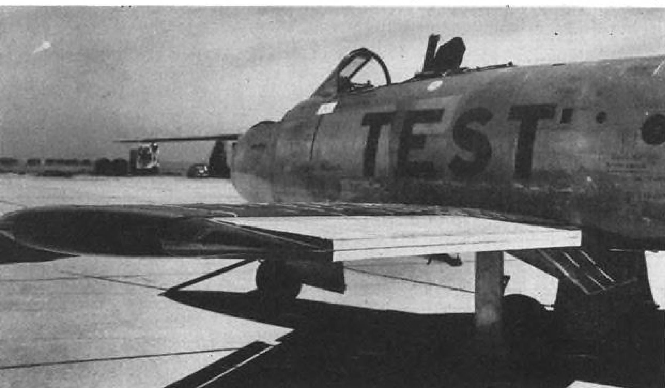
CHANCE VOUGHT F7U (above) has blunt ailerons to improve transonic stability. NACA used modified F-86 (below) to obtain transonic flight test data on the basic concept.
