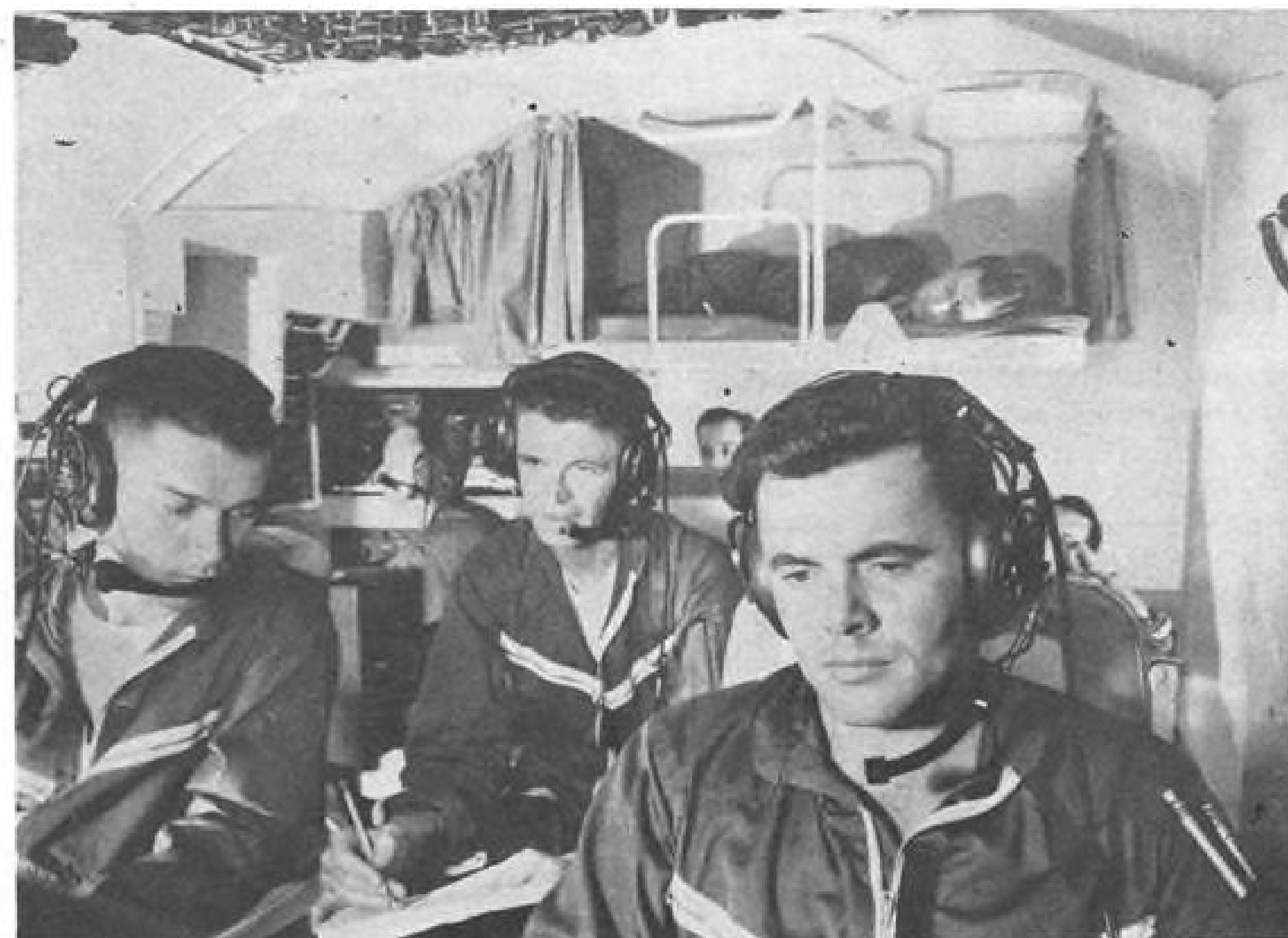
MOCKUP of flight deck of commercial version of Hercules is demonstrated at Lockheed Aircraft Corp.'s Marietta, Ga., plant. Compartment contains two bunks, hot meal galley, stowage space, toilet facilities, soundproofing and insulation.
