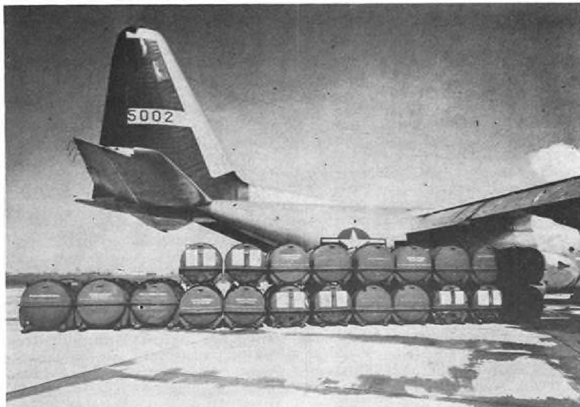
PAYLOAD of one Hercules flight included 21 turboprop engine gear box shipping containers (shown above), 2,100 lb. of T56 engine parts, 500 lb. of tiedown chains—total, 14½ tons. Load was lifted from Marietta, Ga. to Indianapolis, Ind.
