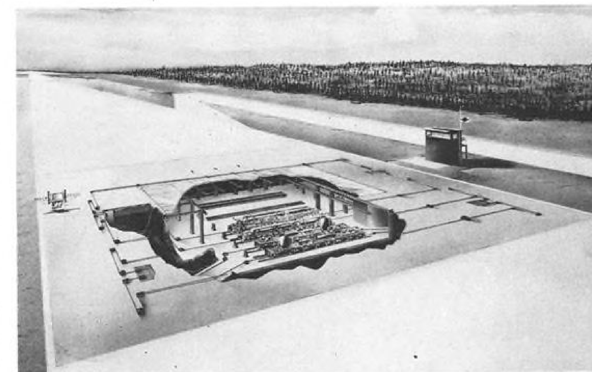
RUNWAY Arrested Landing Site drawing shows under-runway installation of four Mk. 7 Mod. 1 arresting engines with space for two more. At right is diversion strip for rapid-landing operation and RALS control station. Mirror landing system is shown at left.
