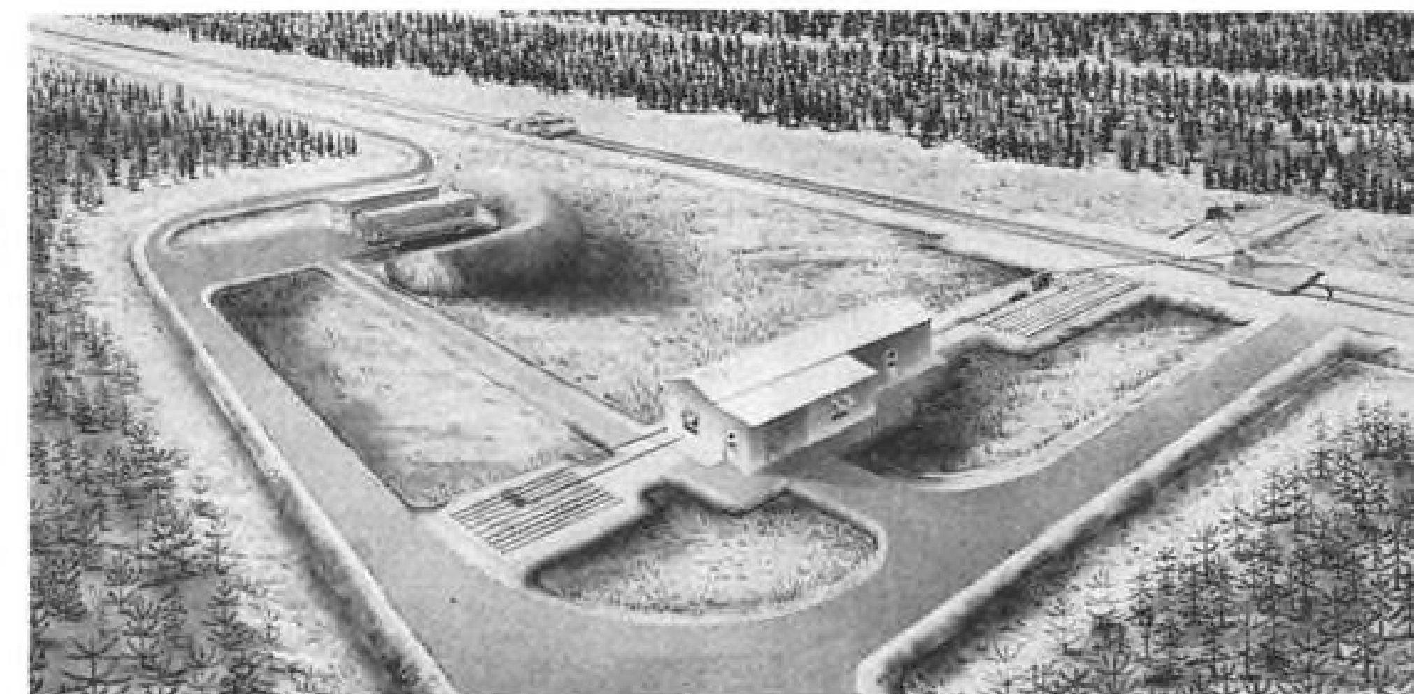
RECOVERY System Test Site. Artist's drawing shows jet car stopped (center) as deadload hurtles into arresting pendant (right). Arresting engine is in shack (foreground). Technicians in trailer are protected from whipping of broken cable by earth revetment.
