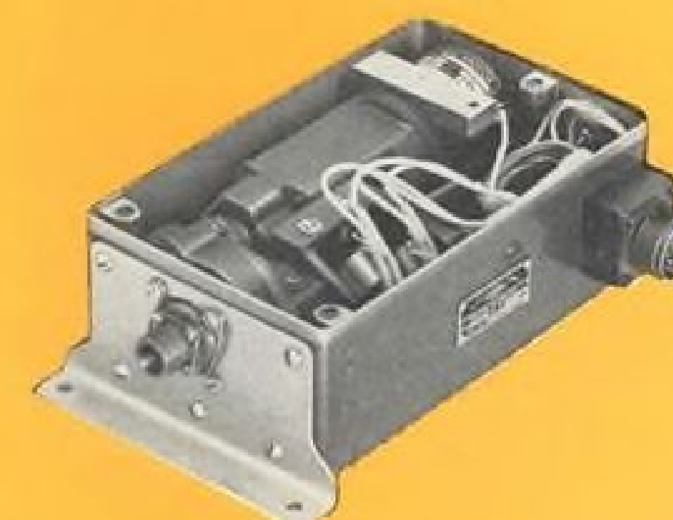
Type: D-892 Power Package; Size: 7 1/4" x 4 3/4" x 2 3/4". Output: 28 volts D.C., 1390 RPM at take-off shaft, 18 inch-oz. torque. Weight: 3 3/4 lbs.; Operative in ambient temperatures to 250° F. Meets Military Specifications: MIL-A-8064 for actuators, MIL-M-8609 for motors.
