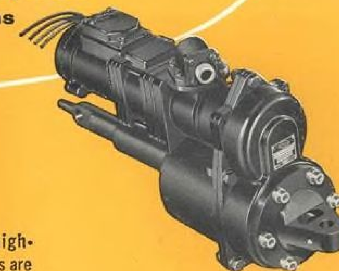
Type: D-818 Leading Edge Flap Actuator; Weight: 20.5 lbs. Normal Operating Load: 6,000 lbs.; Maximum Operating Load: 12,000 lbs. Ultimate Static Load: 24,000 lbs.; Stroke: 3.15"; Rate of Travel: .33" per second; Amperes: 3 amps at 480 cycles on 200 volts at the 6,000 lbs. load. Meets Mil. Specs.: MIL-A-8064 for actu- ators, MIL-M-7969A for motors.
