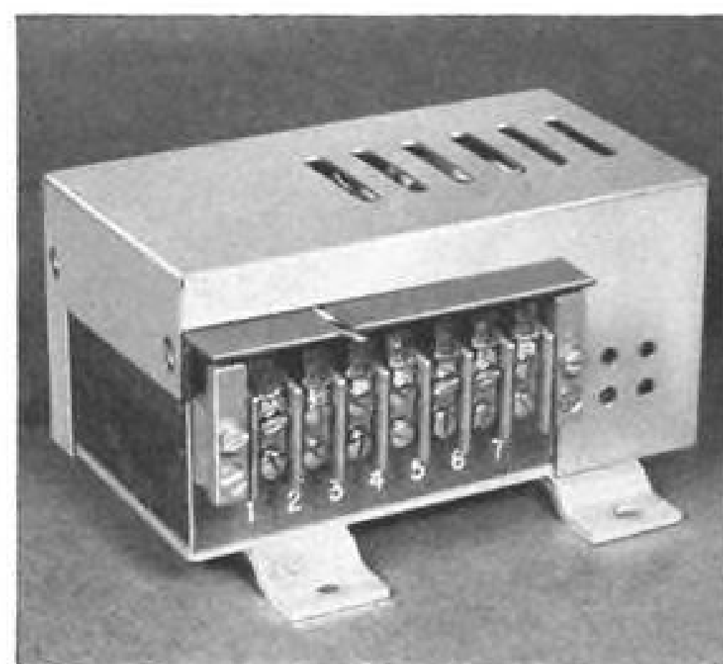
General Electric regulator (left) and alternator (right) combine to form a 30-pound power package rated at 10 KVA. The alternator is 9 1/4 inches in length and 6 inches in diameter. The voltage regulator is 5 inches long. Total RMS harmonic content of the alternator output is less than 1% of fundamental. The generator has an efficiency of 85% at rated load.
