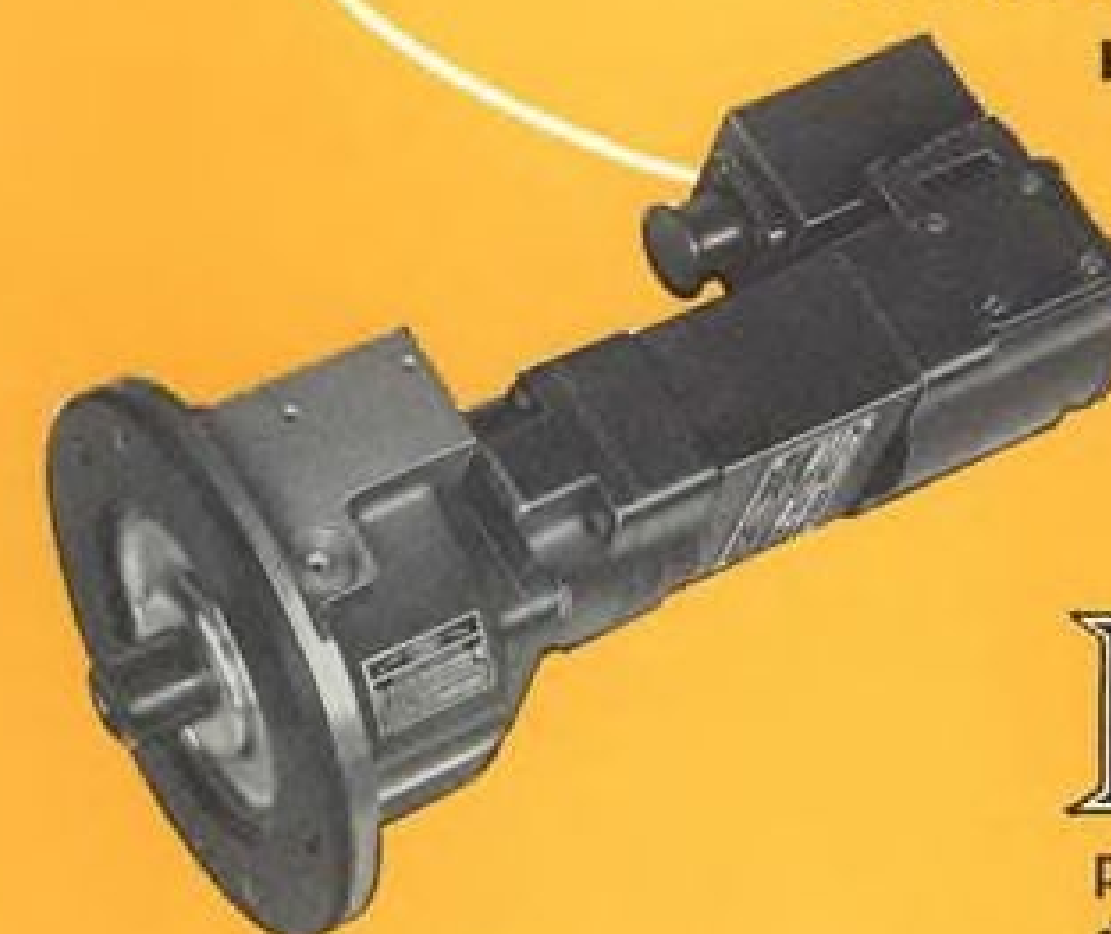
Type: D-925 Rotary Actuator for Missile Fin. Output: 400 inch-pounds @ 64 RPM, 24 volts, 27 amps. Duty Cycle: 1 minute on, 10 minutes off; Gear Reduction: 135 to 1 in 2.25" length; Weight: 6.75 lbs. Meets Mil. Specs.: MIL-A-8064 for actu- ators, MIL-M-8609 for motors.
