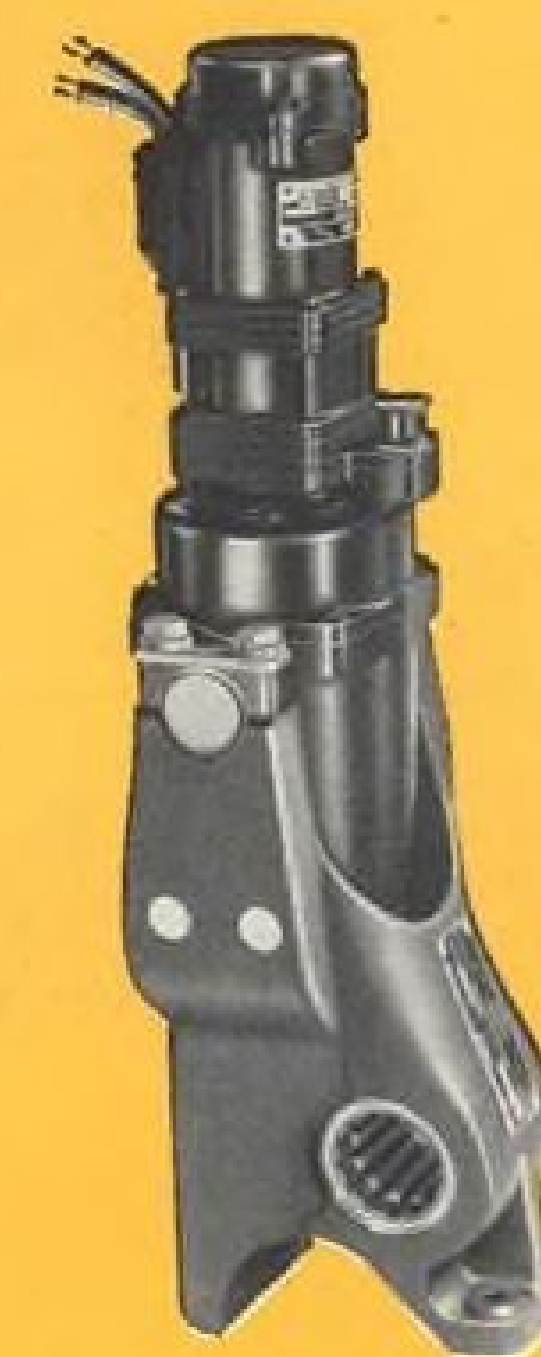
Type: D-868 Rotary Actuator; Weight: 9 1/4 lbs. Power: 200 volt, 400 cycle, 3- phase motor. Ambient Temperature Range: -65°F. to +400°F.; Shaft Torque Limit: Adjustable. Load: 1,650 inch-lbs. maximum to approx. 2 RPM on 1.5 amps. Meets Military Specifications: MIL-E-7894 and MIL-A-8064.
