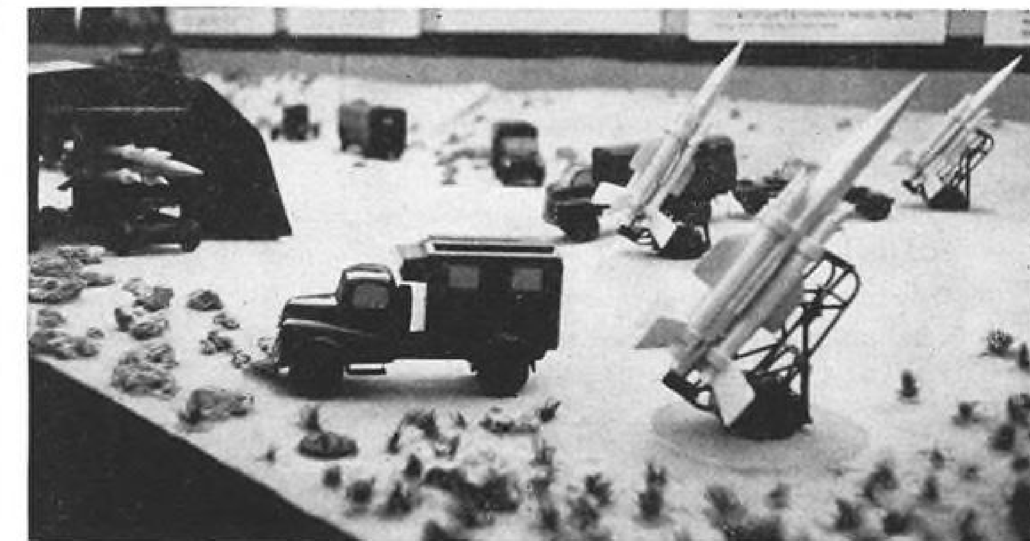
Missiles are delivered to assembly site in containers (above). After assembly and checkout, missiles are delivered by truck-drawn dolly to launchers (below). Model layout was shown at Farnborough. Thunderbird test missiles have been fired at Woomera, Australia testing area.
