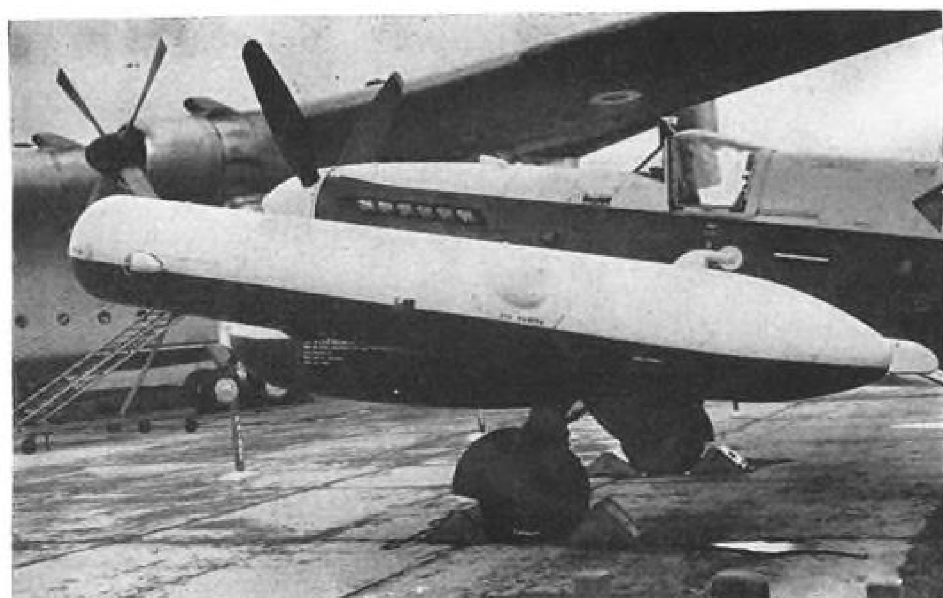
Hawker Hunter lineup (left) shows lipped tailpipe being tested as a possible configuration change on the near two. Wing-tip pod of Fairey Firefly target aircraft (right) carries five wide angle cameras to record hits and near misses of test rounds.
