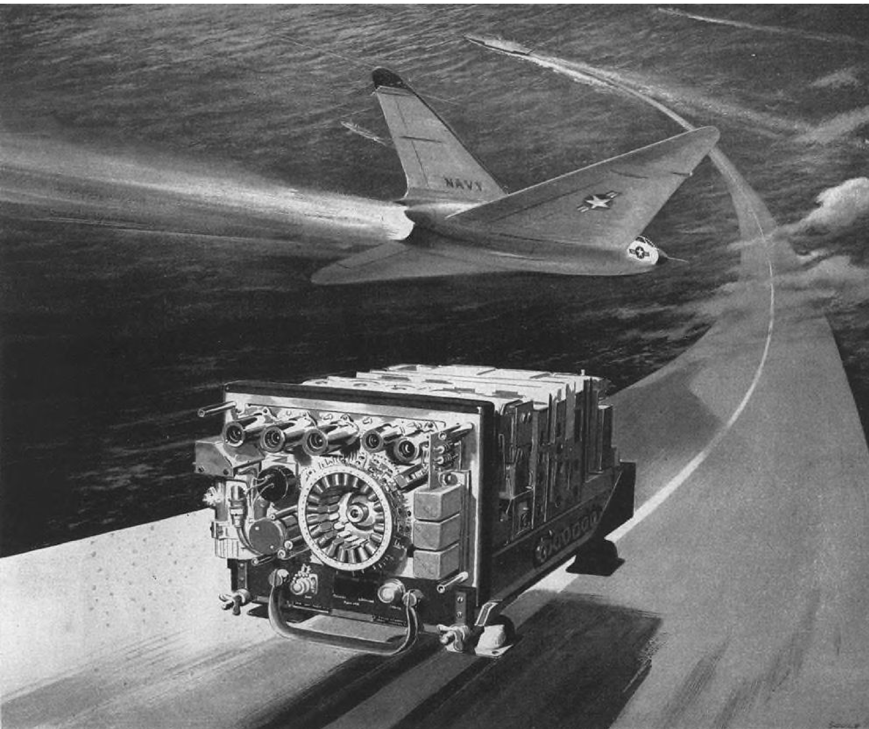
TACAN unit shown with covers removed; plane is a composite model.
