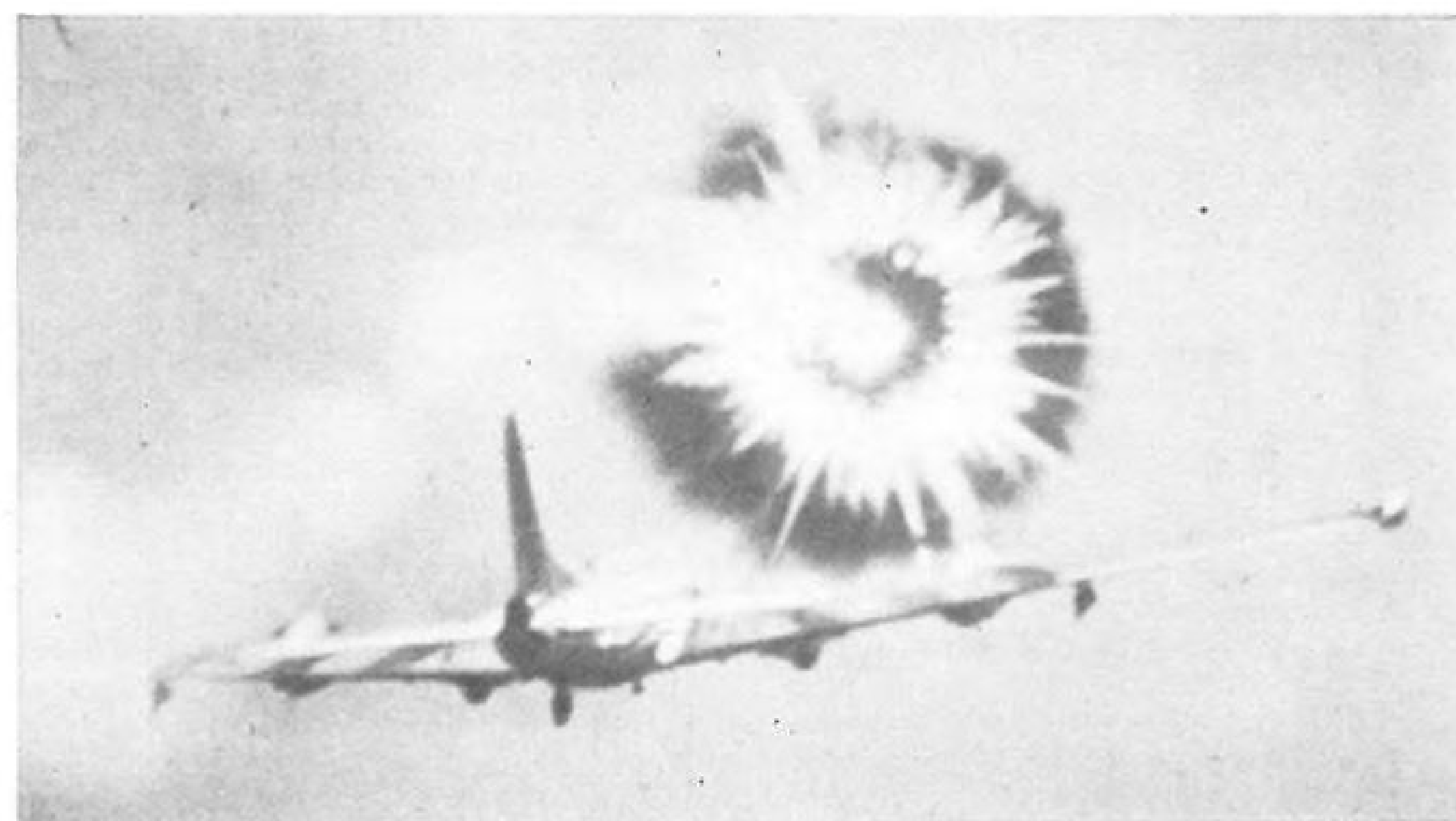
SPARROW I attacks radio-controlled B-17 drone with proximity fuzed warhead.
