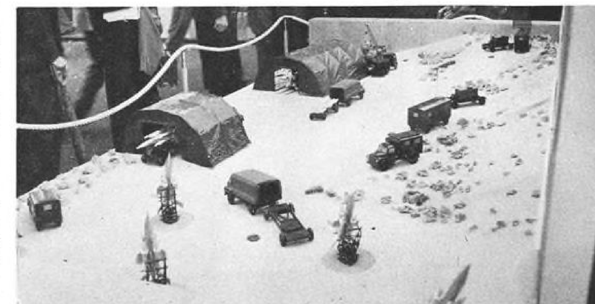
Model field installation shows English Electric Thunderbird ground-to-air missiles on launchers with assembly and test shelters at rear and radar and control trucks at right. System was designed to use standard British Army trucks and vehicles and require a minimum amount of special equipment.
