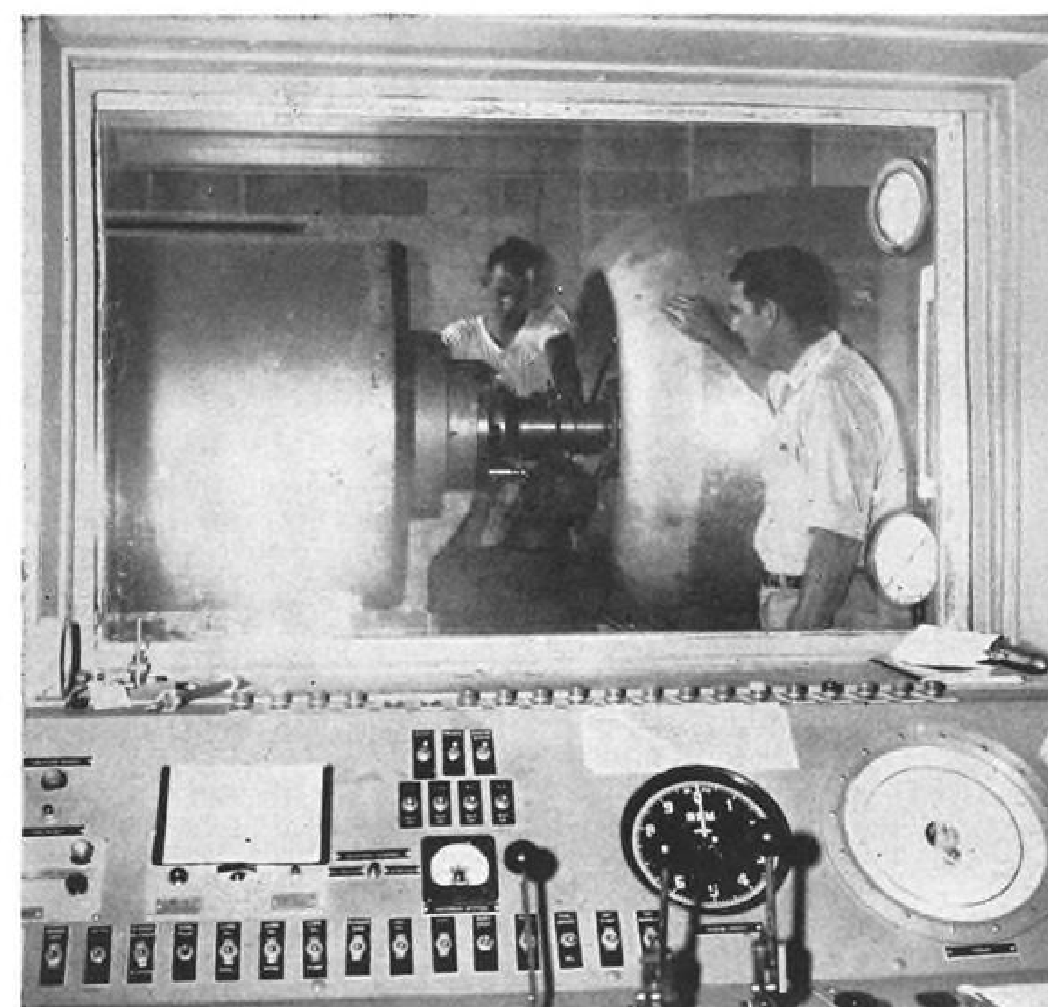
BRANIFF MECHANICS link propeller shaft with coupling flange to new dynamometer at airline's Dallas overhaul base. Photo taken from control room.
