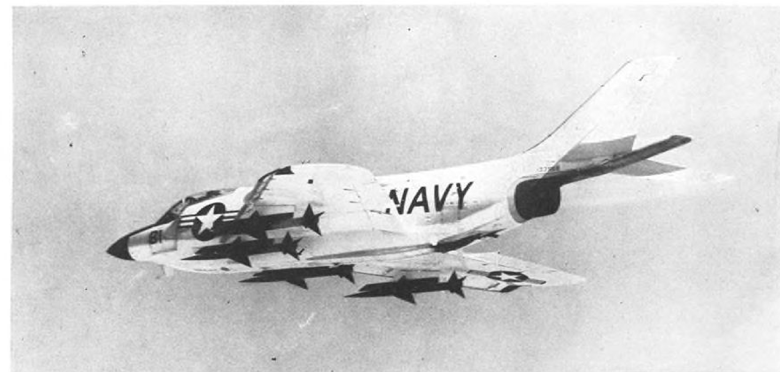
FOUR SPARROW I's roost under wings of McDonnell F3H-2M. Missile is in use with Sixth Fleet.
