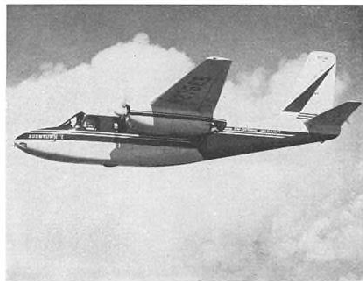
THE PLANE: A standard production model of the new Aero Commander 560-E, a 7-place twin-engine executive transport with a 1625-mile range, plus safety fuel reserve.
