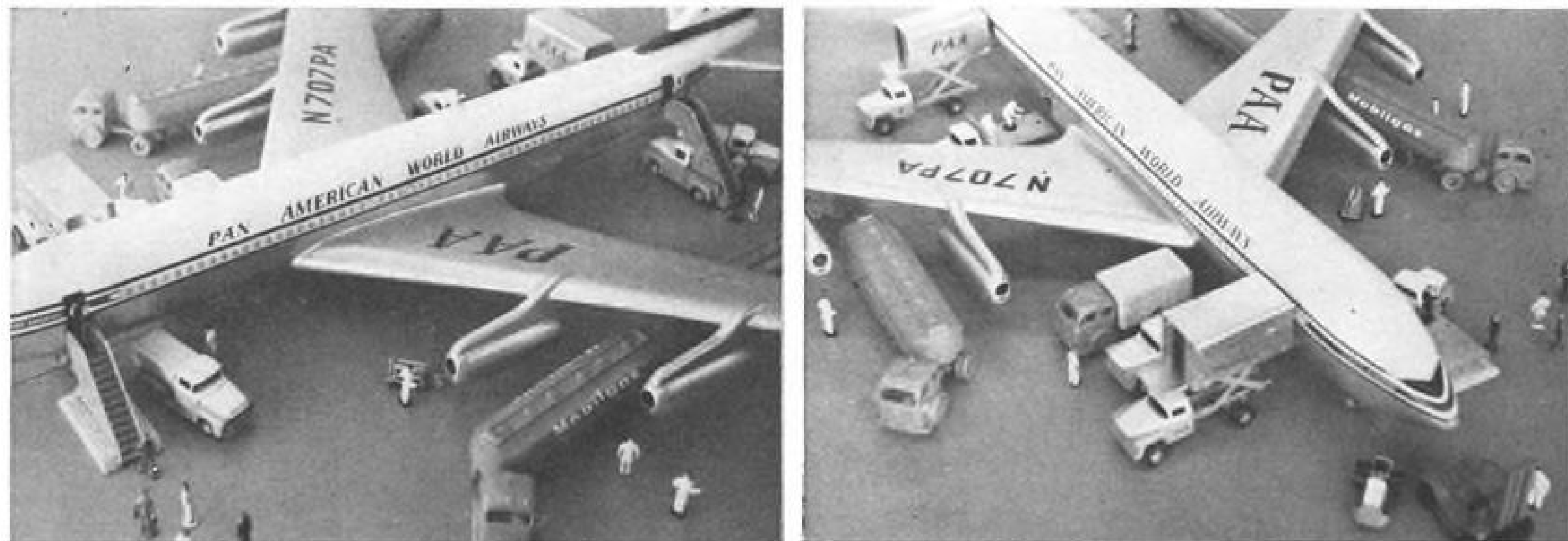
EQUIPMENT surrounding Pan American Boeing 707 model represents items needed on ramp during initial operations. Some differences will appear in actual hardware. In picture at right, items clockwise from nose to tail left side, are tow tug, power unit, galley truck, baggage truck, air conditioning truck, fuel truck, baggage truck, galley truck. In left picture, items clockwise from tail to nose right side, are toilet service truck, self-propelled loading stairs, fuel truck, start cart, water service truck, loading stairs.
