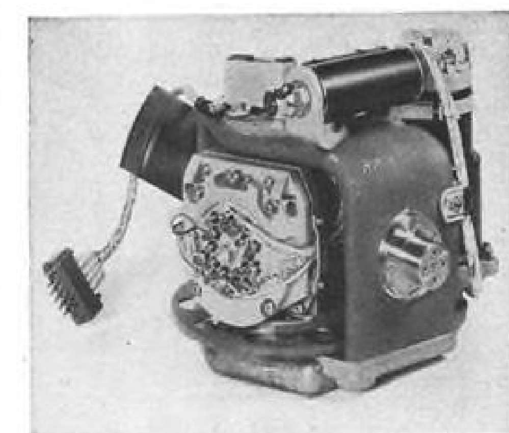
INTEGRATING accelerometer employs a pendulous liquid-floated integrating gyro.
