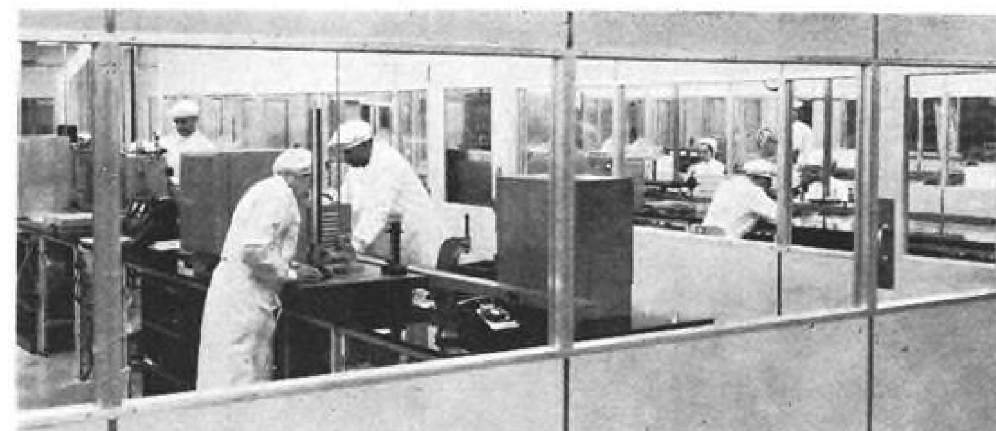
STERILE rooms used in assembly of gyros and accelerometers are air conditioned, pressurized with heavily filtered air, swabbed down twice a day to maintain required cleanliness.
