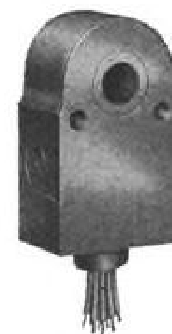
Cole Electric Co. Hermetically-sealed Rotary Sequencing and Indicating Switch. Two pole, double throw. 4 circuit. 10 amps, 30 volts D.C. Serrated actuating tube permits tandem mounting.
