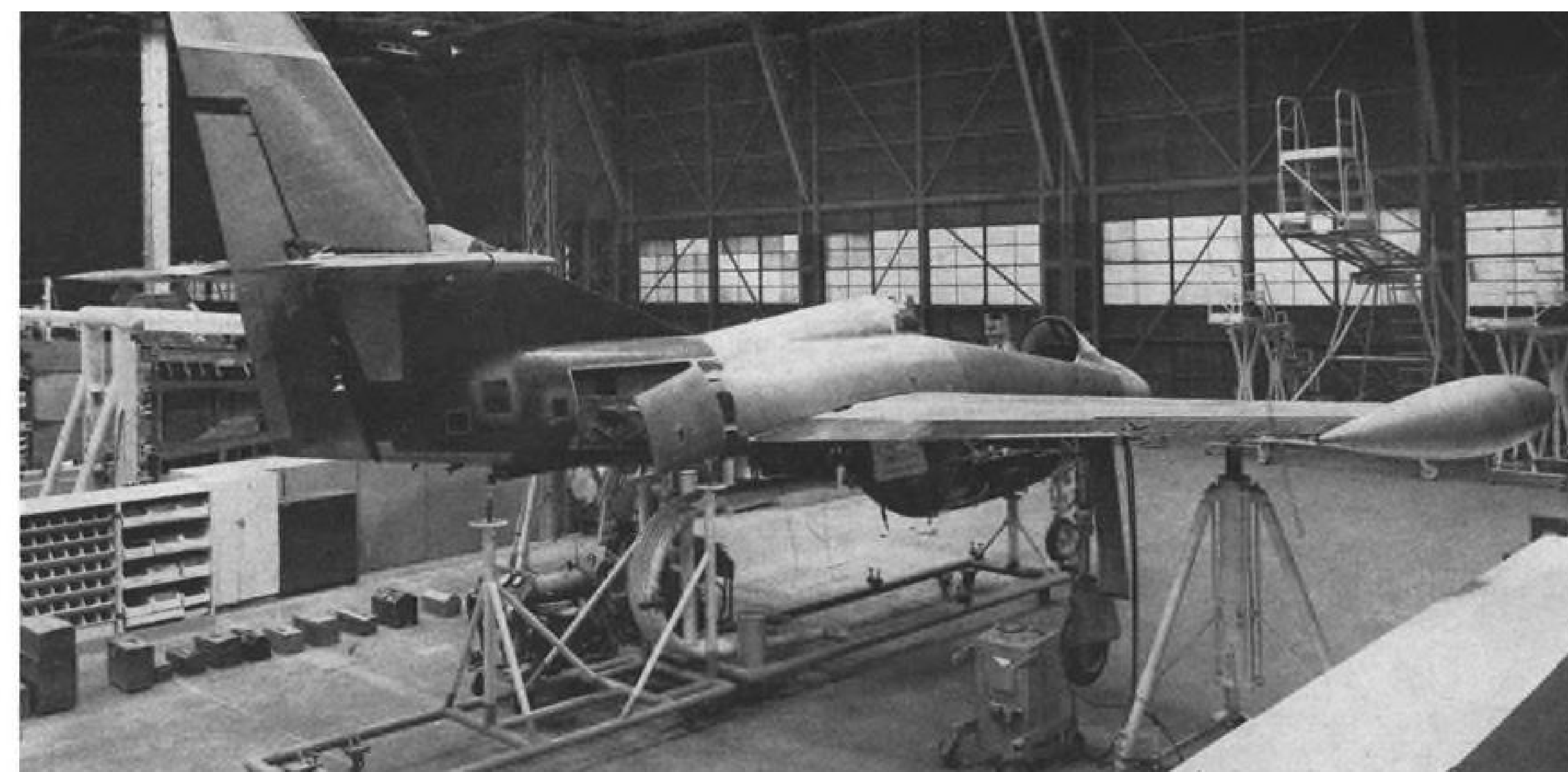
BIG TAIL is designed to provide positive control at low speeds; 45% of rudder is below horizontal tail to aid in spin recovery.
