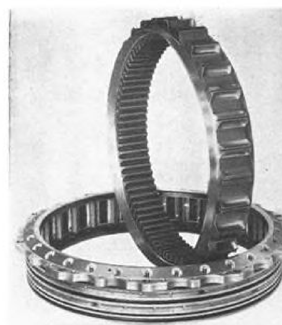
TORQUEMETER improves isolation of reduction gear from propeller vibration.
