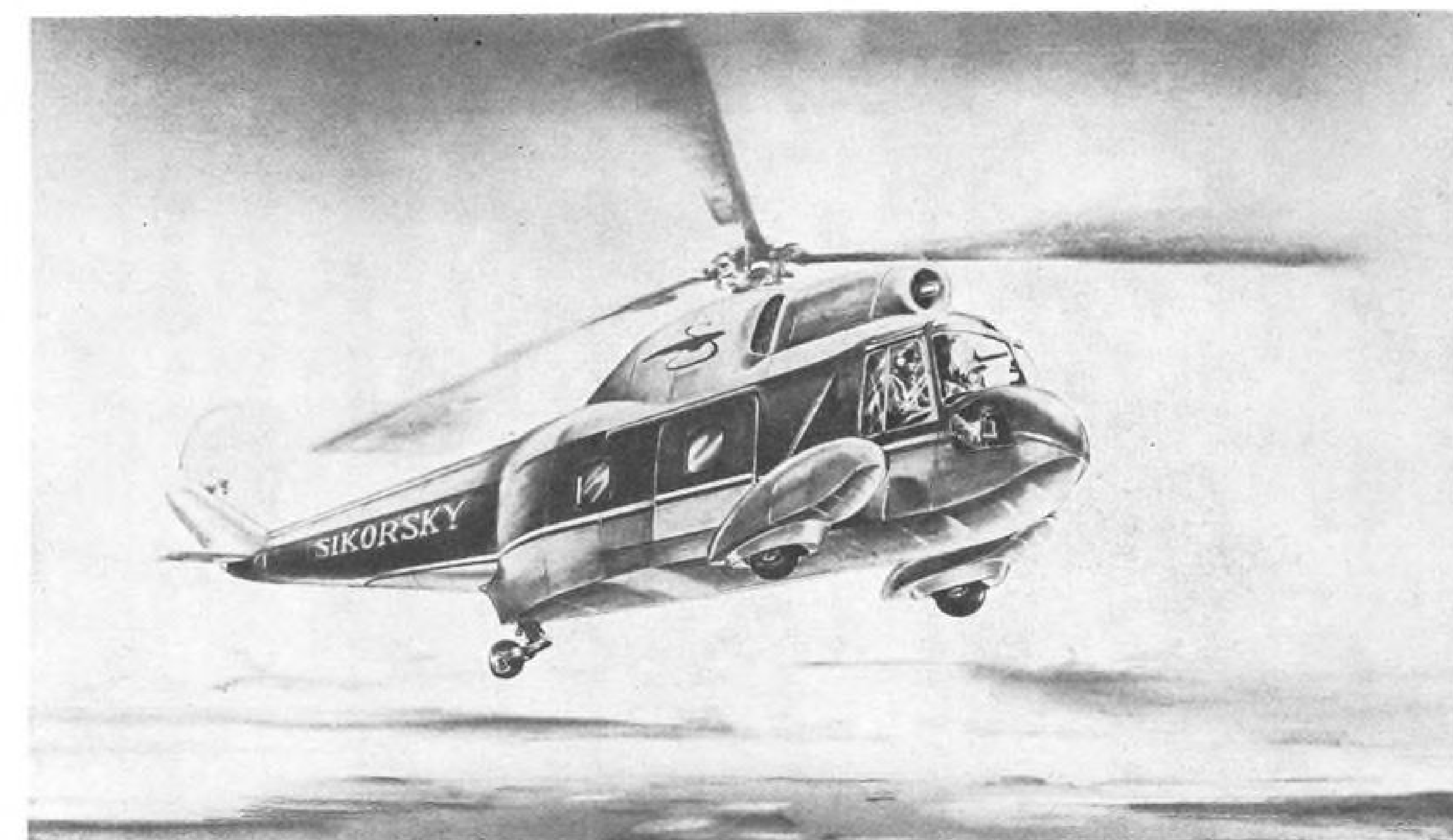
SIKORSKY S-62, shown here in artist's conception, has flying boat hull, turbine engine. It uses many S-55 components.
