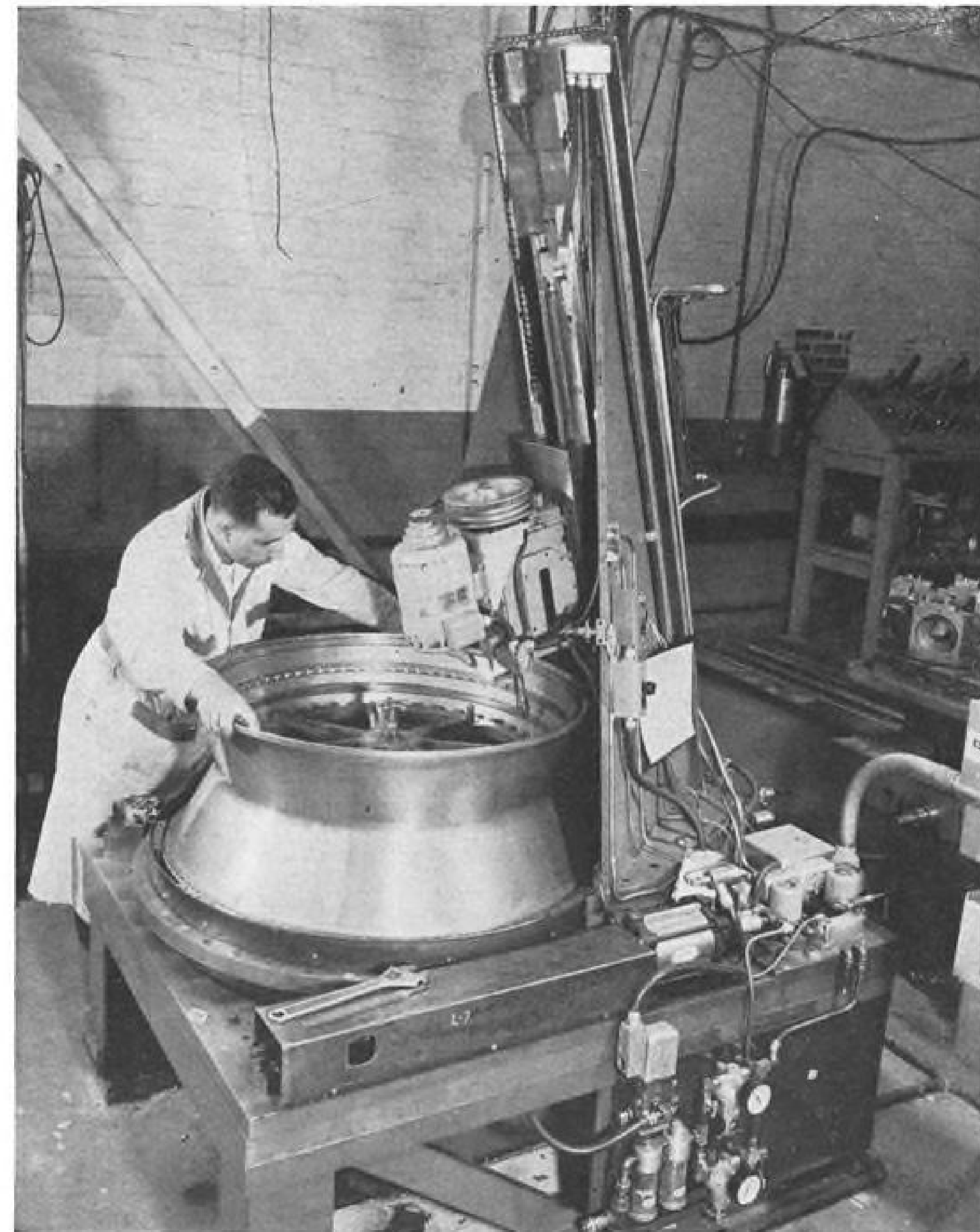
OVERHUNG drill spindle drills and reams blind holes from inside out. The indexing table floats on a cushion of air while turning. Pre-production tooling will tend to require more original creative engineering effort and will be important in cost, time estimates.
