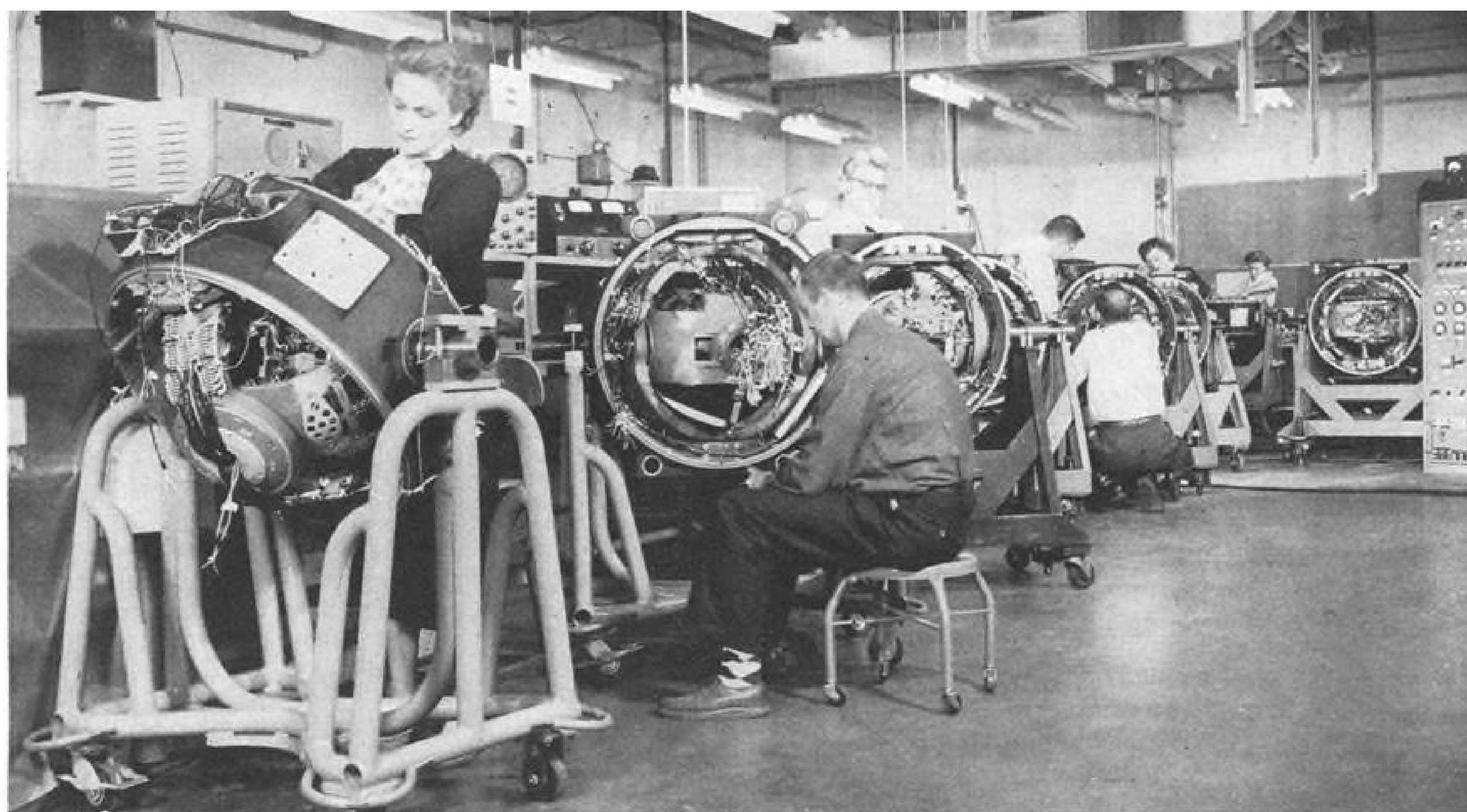
FIRST PHOTOS of inertial guidance systems used in Thor intermediate range ballistic missile, show size and rugged construction of the three-gimbal stabilized platform. Thor guidance system is in quantity production at AC Spark Plug plants in Milwaukee.
