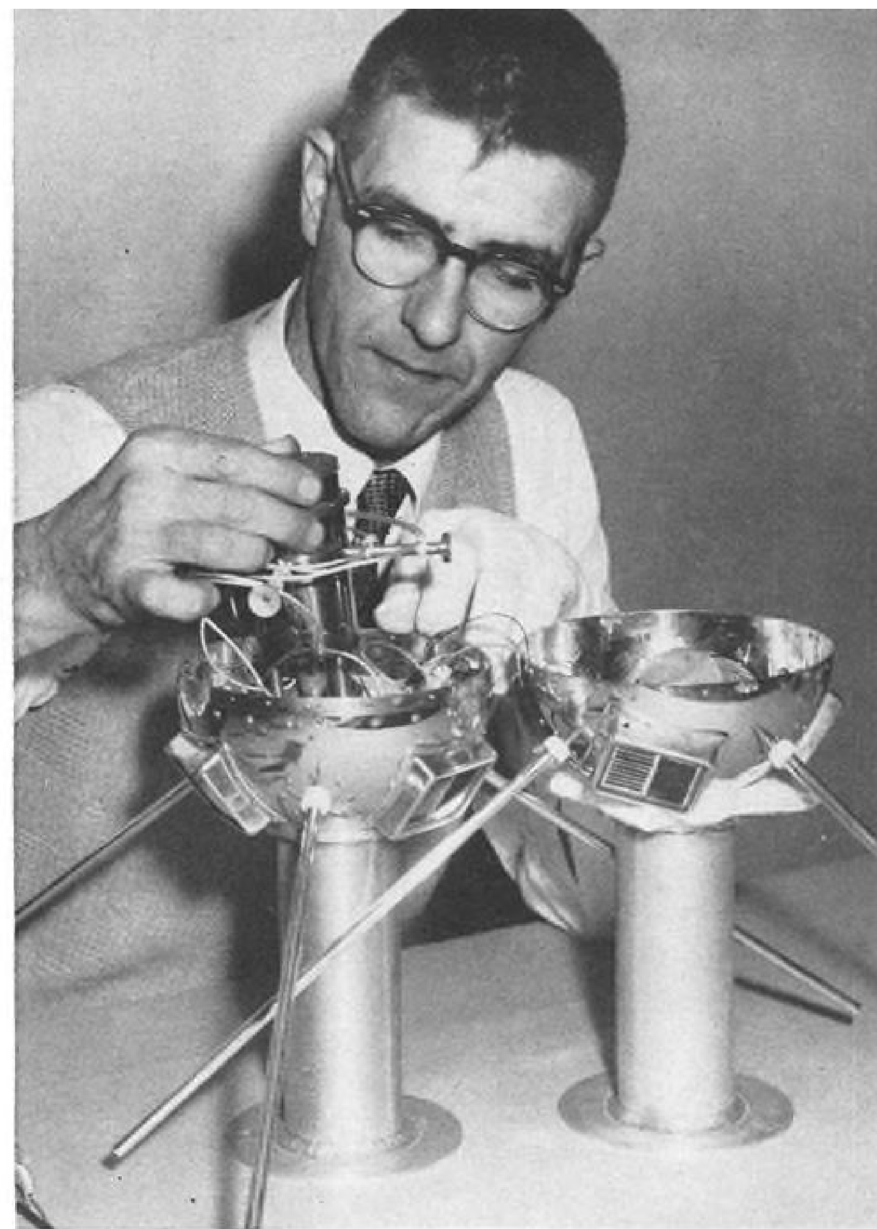
PRELIMINARY testing involves static firing, as illustrated by photograph of the Test Vehicle 3 first-stage engine undergoing static test at night on Cape Canaveral. Naval Research Laboratory machinist (right) inserts instrumentation package in 6.4 in. dia., 3½ lb. test sphere. Baby satellite contains two miniature radio transmitters, one powered by mercury batteries, the other by solar batteries.
