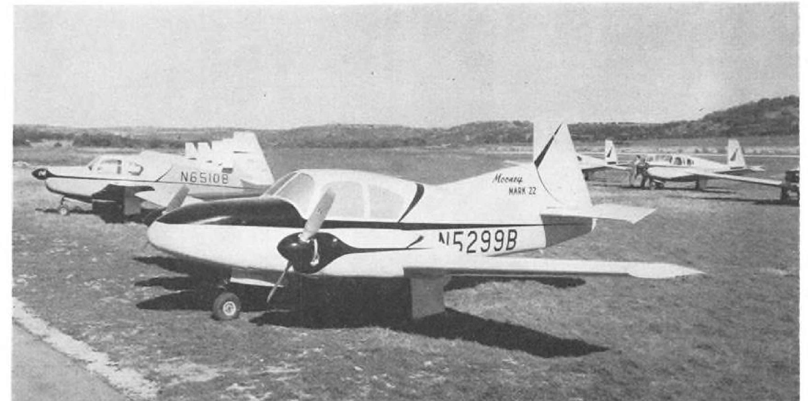
MARK 22 light twin aerodynamic prototype is scheduled to start flight tests in March. Company considers it an early 1960 airplane. Resemblance to single-engine Mark 20s in background is readily apparent. Prototype has 150-hp. engines, but production versions will probably use 180-hp. Lycoming O360s. Large dorsal fin was not on earlier sketches of Mark 22 (AW Dec. 30, p. 23).
