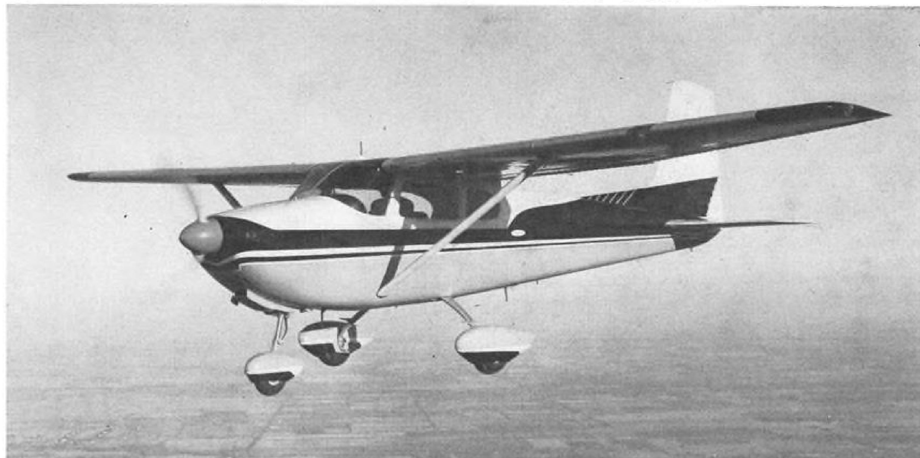
FIBERGLAS WHEEL FAIRINGS set de luxe style note on Skylane, offered to customers as a completely equipped ready-to-use package.
