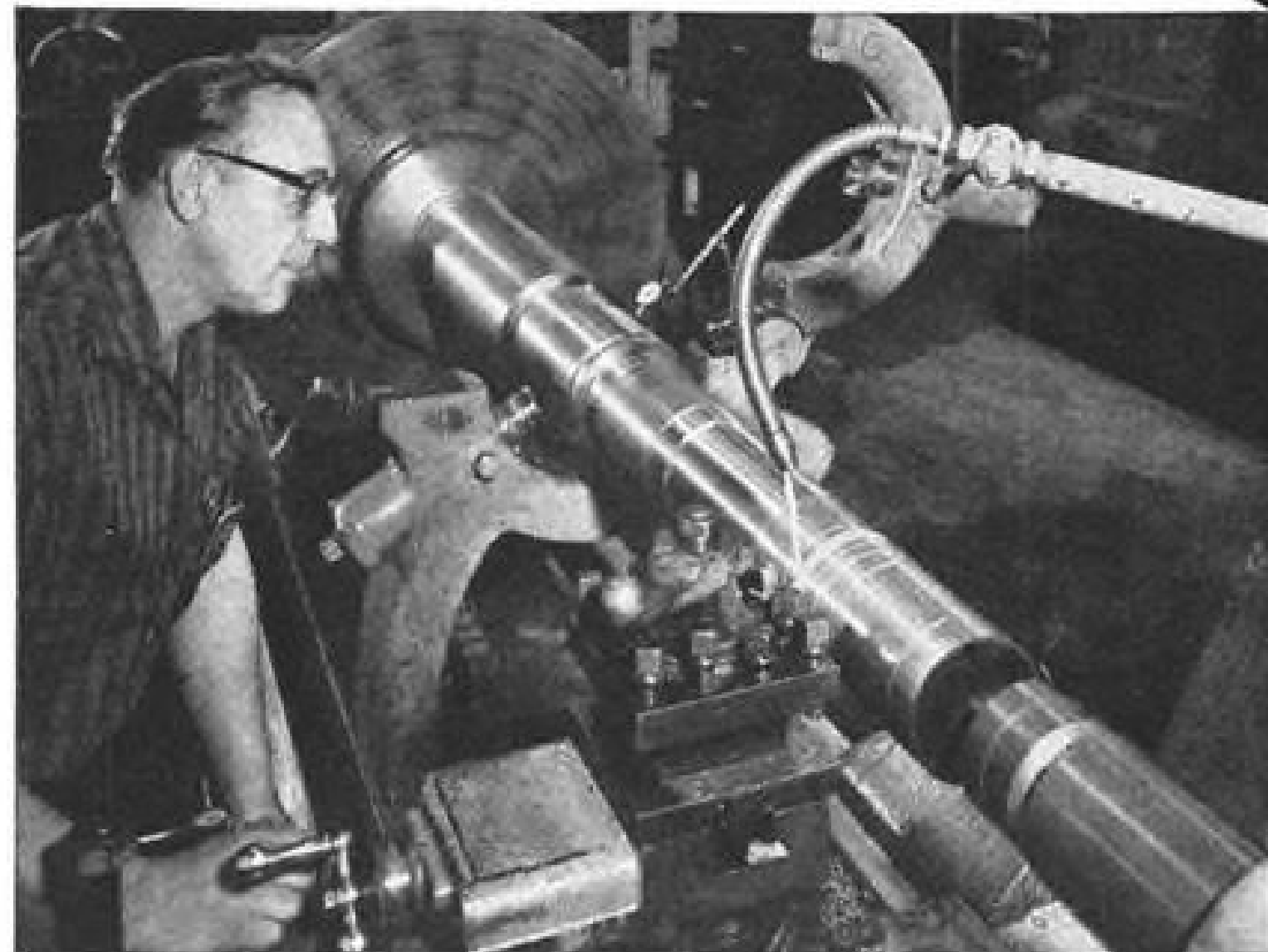
Machining a solid shaft from 4340 alloy for compressor of industrial gas turbine used on gas-transmission pipeline.
