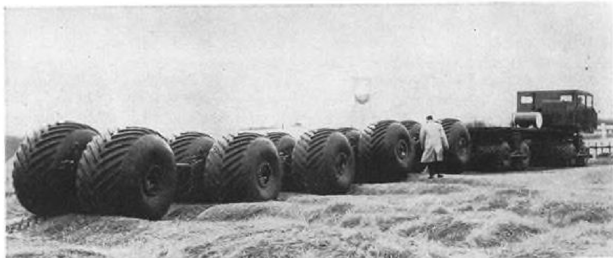
RUBBER TIRE BAGS with a liquid capacity of 500 gal. each are pulled in sets of 10 by all-terrain Teracruzer. Fluid bags carry fuel, liquid chemicals or water.
