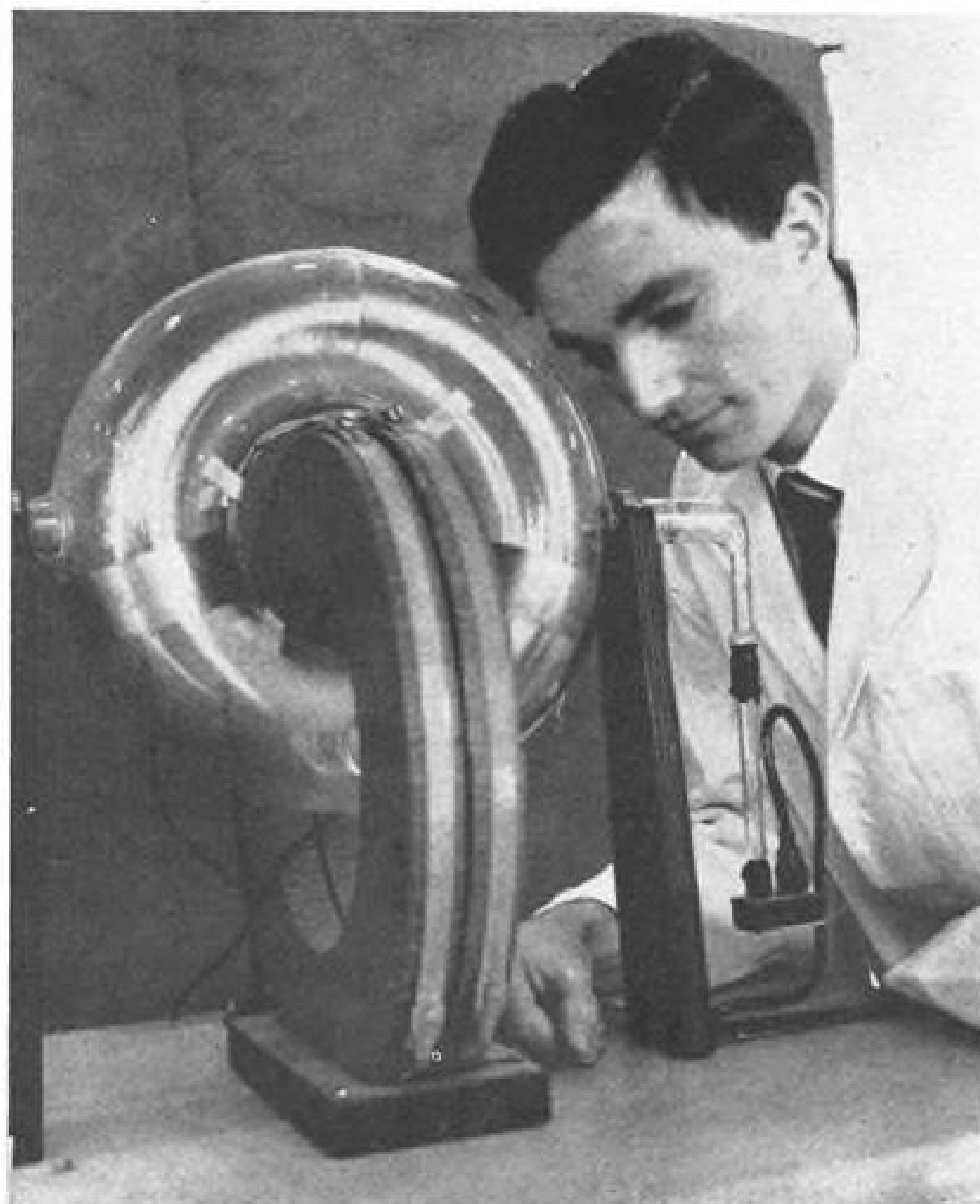
WORKING model shows primary winding of transformer (below) which induces high-current pulse in gas-filled glass tube whose plasma forms short-circuited secondary winding.
