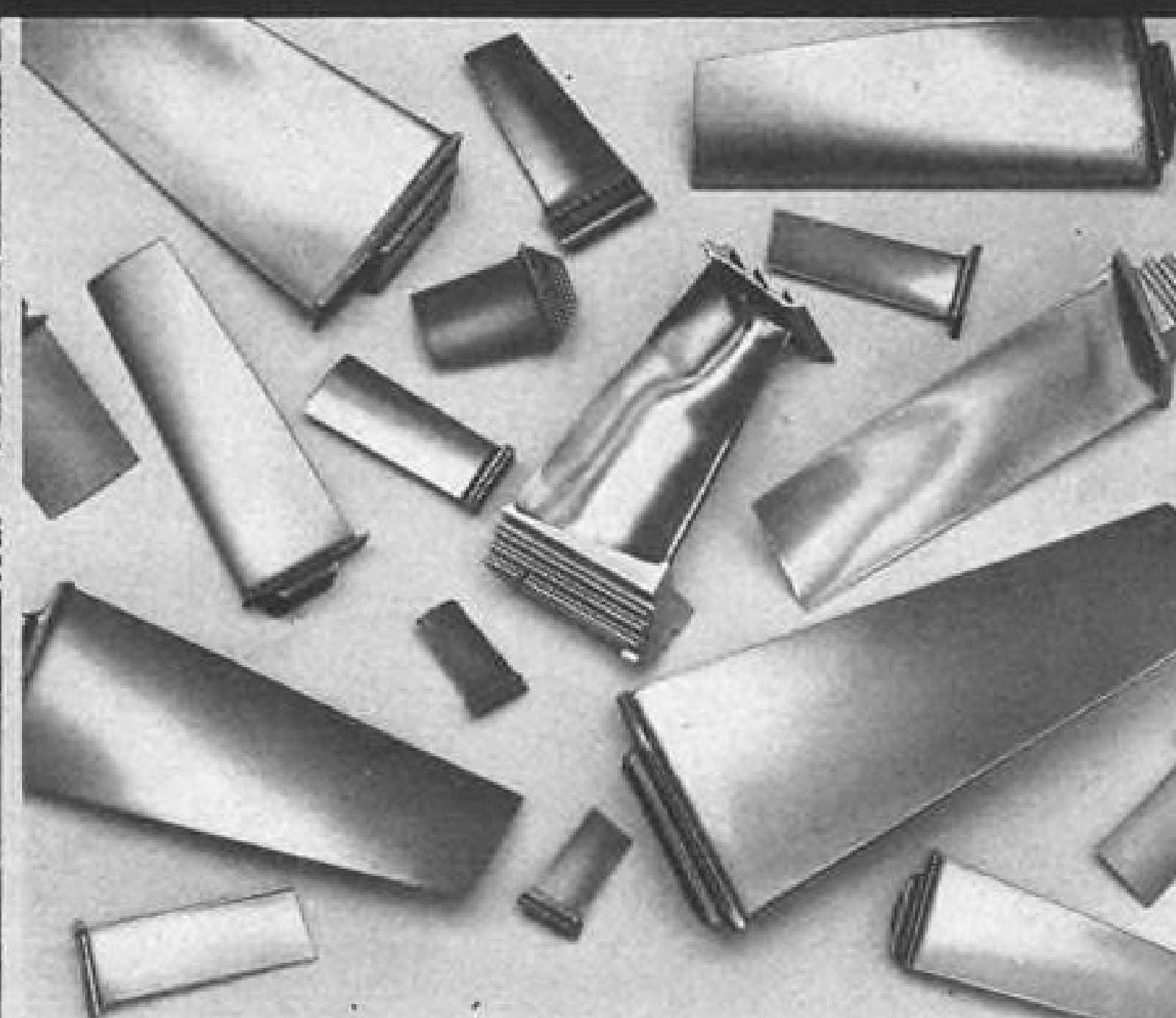
Our experience includes the precision-forging of thousands of jet engine components, with tolerances as close as \pm 0.003'' .
