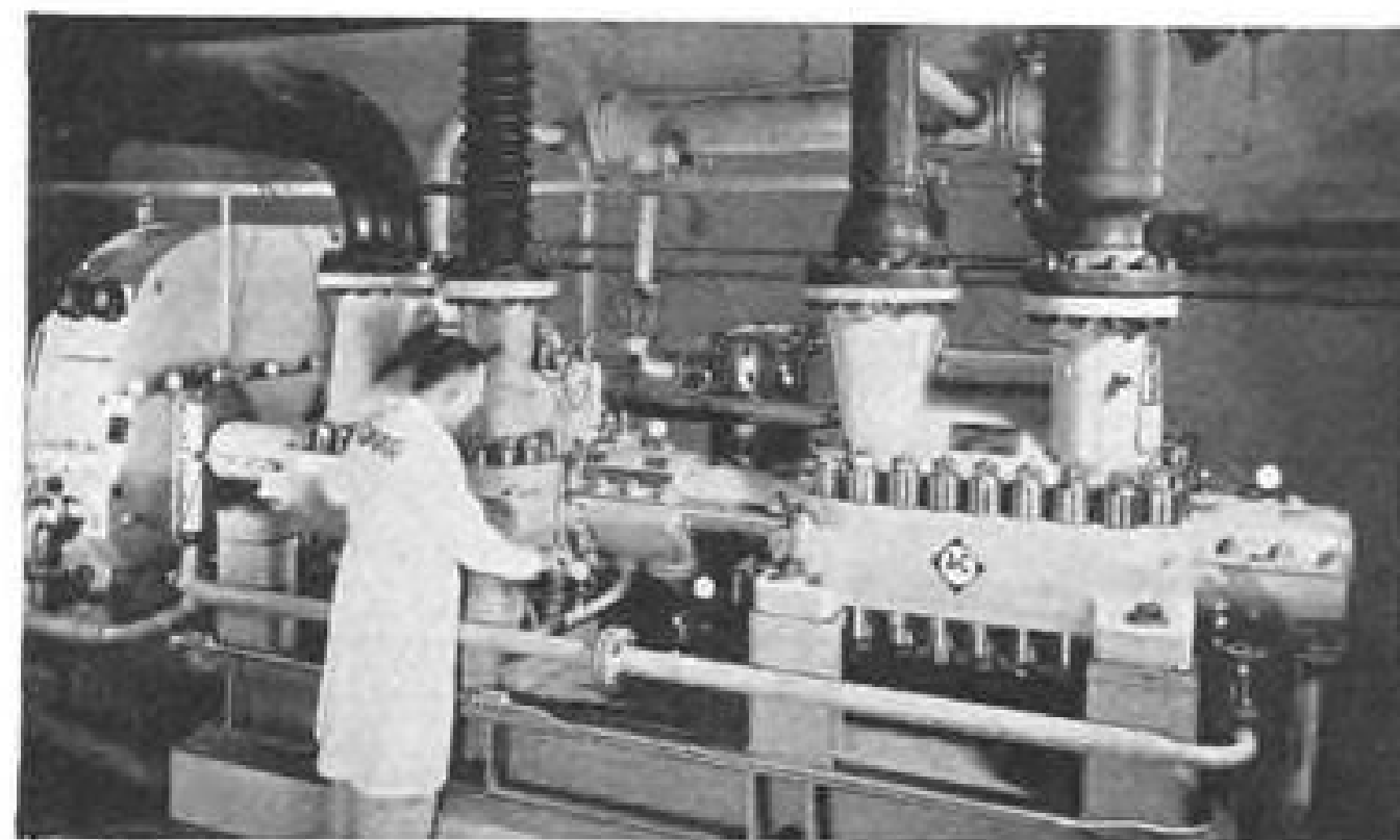
Second and third stage centrifugal compressor driven by the same 8000-hp motor.
