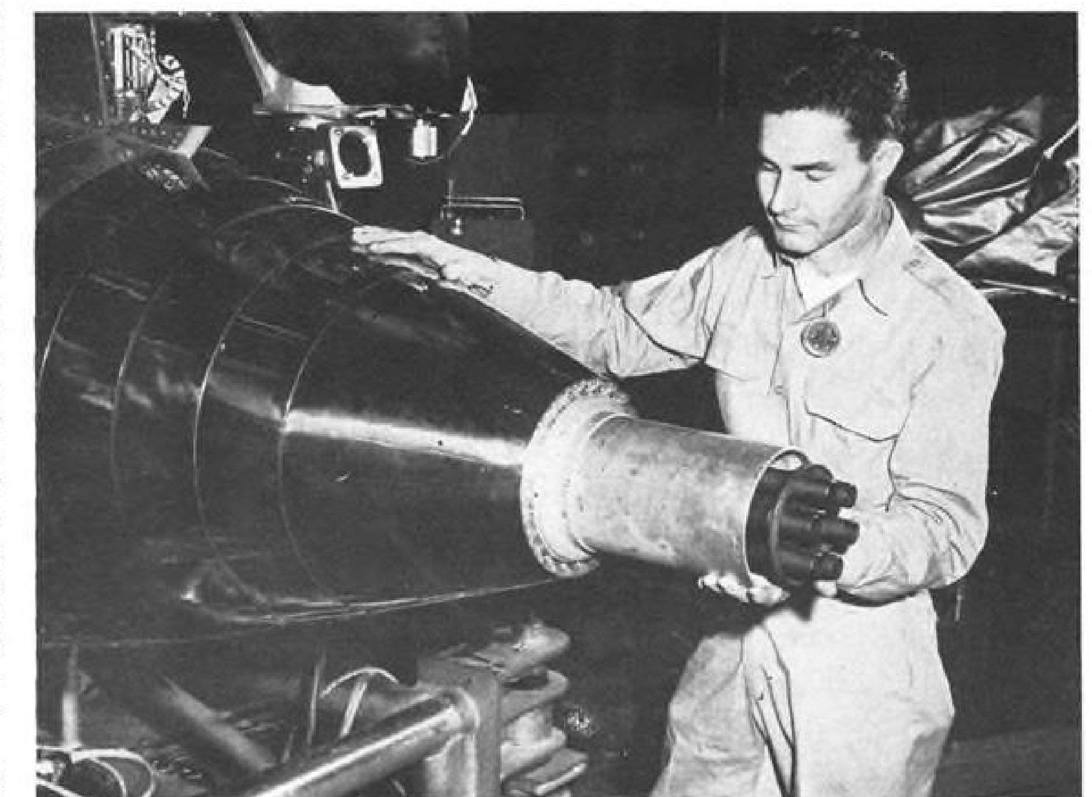
CONVAIR B-58's flexible cone tail turret mounts Vulcan 20 mm. rotating cannon.
