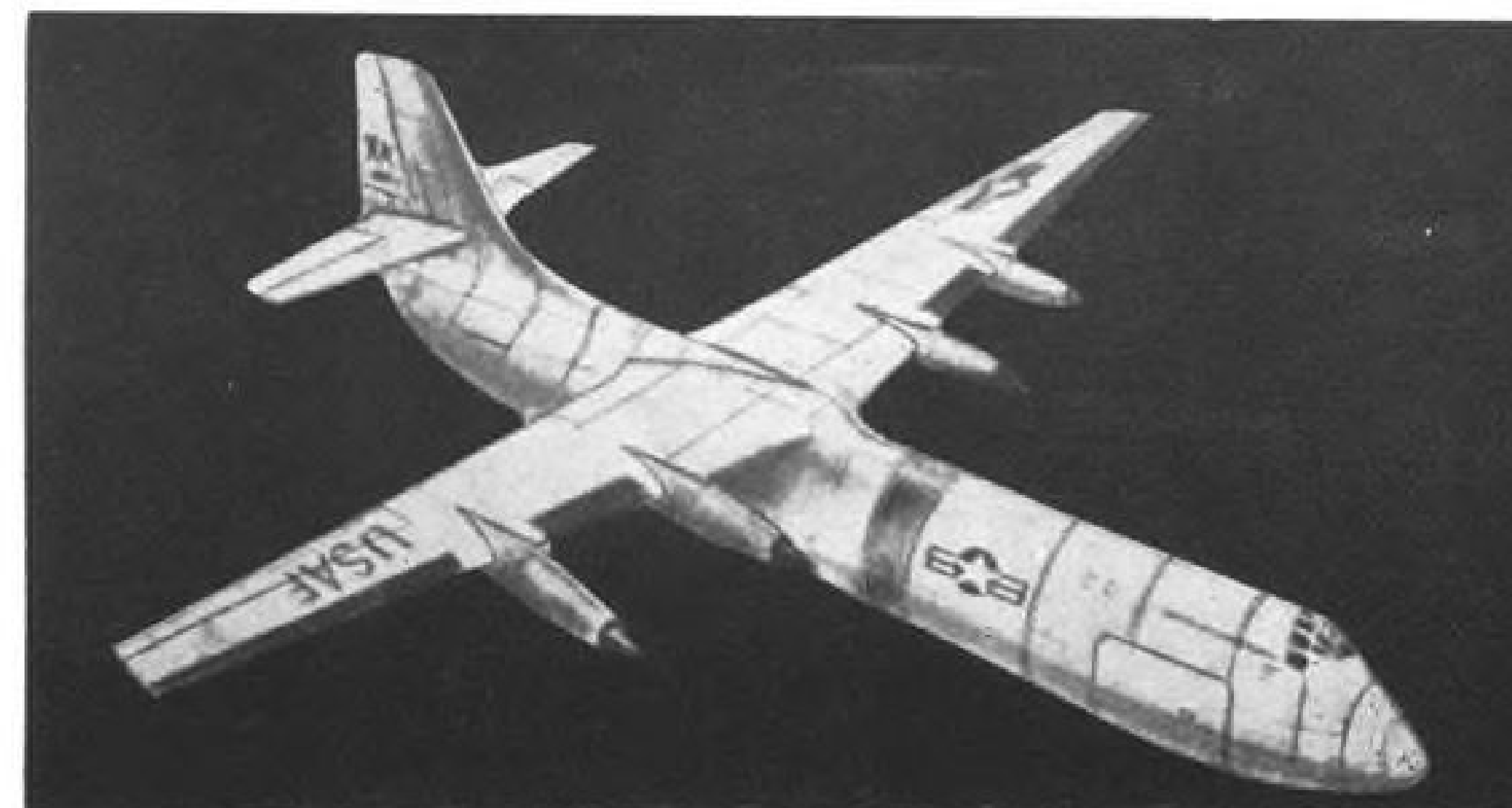
ARTIST'S drawing, left, shows nuclear-powered tanker. Powerplant at right would use helium coolant; reactor would use solid fuel.
