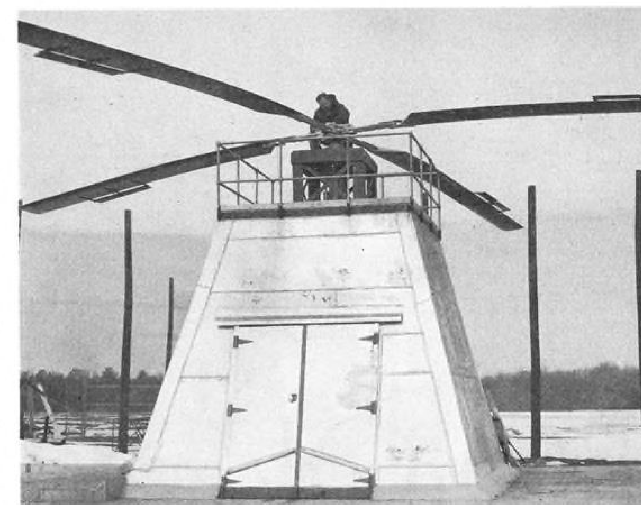
ELECTRIC-POWERED rotor blade test rig delivers constant horsepower to helicopter rotor.
