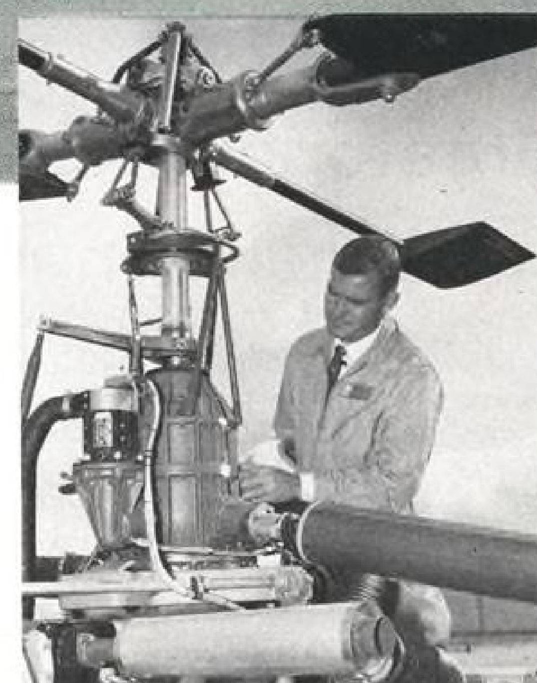
This close-up view of the new Western Gear 1000-hour helicopter transmission emphasizes its ease of maintenance, simplicity and rugged construction. Capable of transmitting 280 HP, the gear box is a double-stage planetary type with power take-offs for the tail rotor drive, fan gear drive and generator drive.
