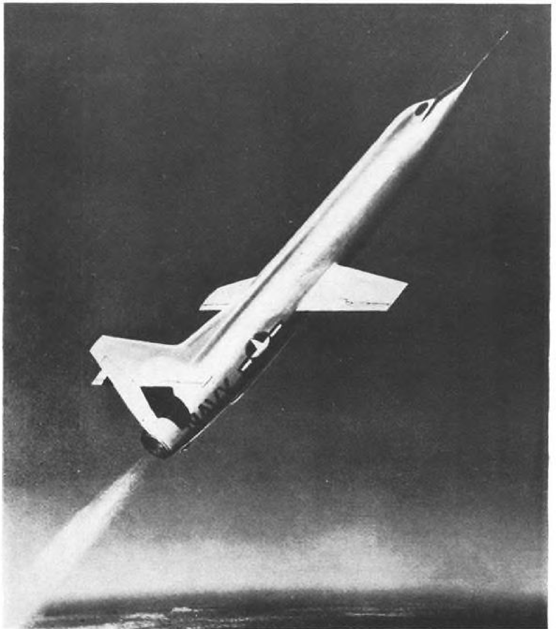
STRAIGHT WINGS characterize this Douglas D-558-III Skyrocket research aircraft first proposed in 1953 to U. S. Navy. Project was dropped because of lack of funds. Artist's conception shows design philosophy of blunt leading edge shapes to reduce skin friction and resultant aerodynamic heating. Plane would be fitted with mono-propellant jet controls for upper atmosphere flight.
