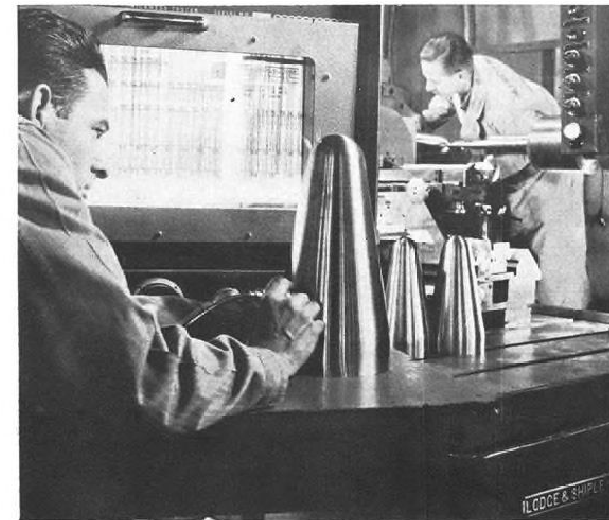
TECHNICAN checks wall thickness of nose cone with a Vidigage ultrasonic probe. Streak of light on instrument panel in rear indicates wall thickness on the chart.
