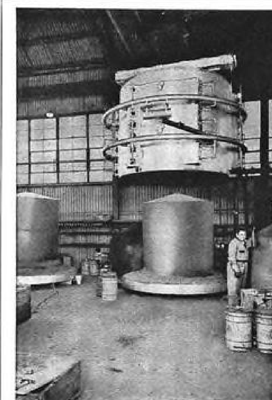
The 72-inch dia. hydrogen atmosphere furnace being lowered over a loaded furnace bell, Detroit plant.
