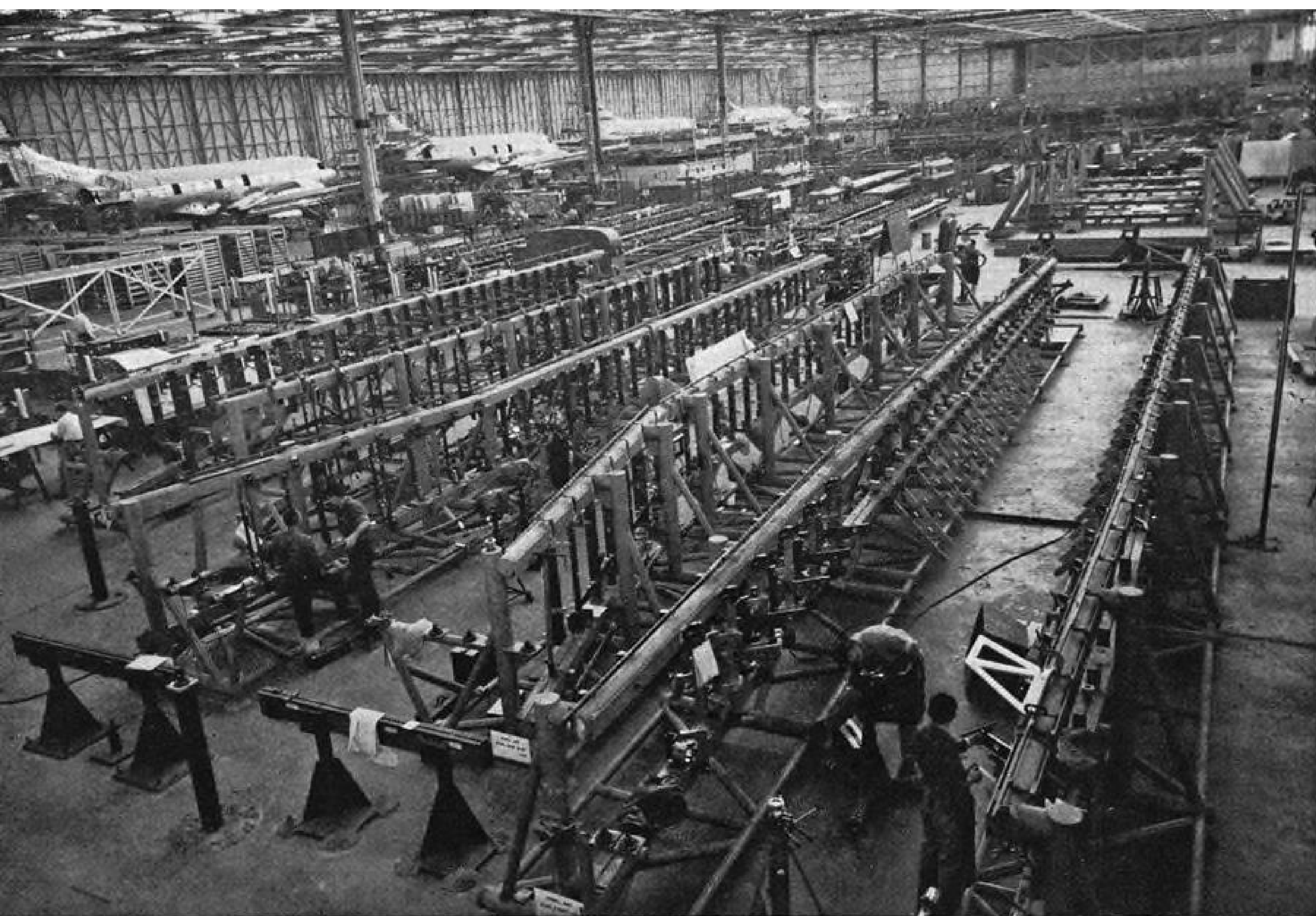
Additional fixtures for wing spar manufacture are completed by tooling crews in part of 632,000-sq. ft. of plant area for Convair 880 production. Convair 440 line is in background.
