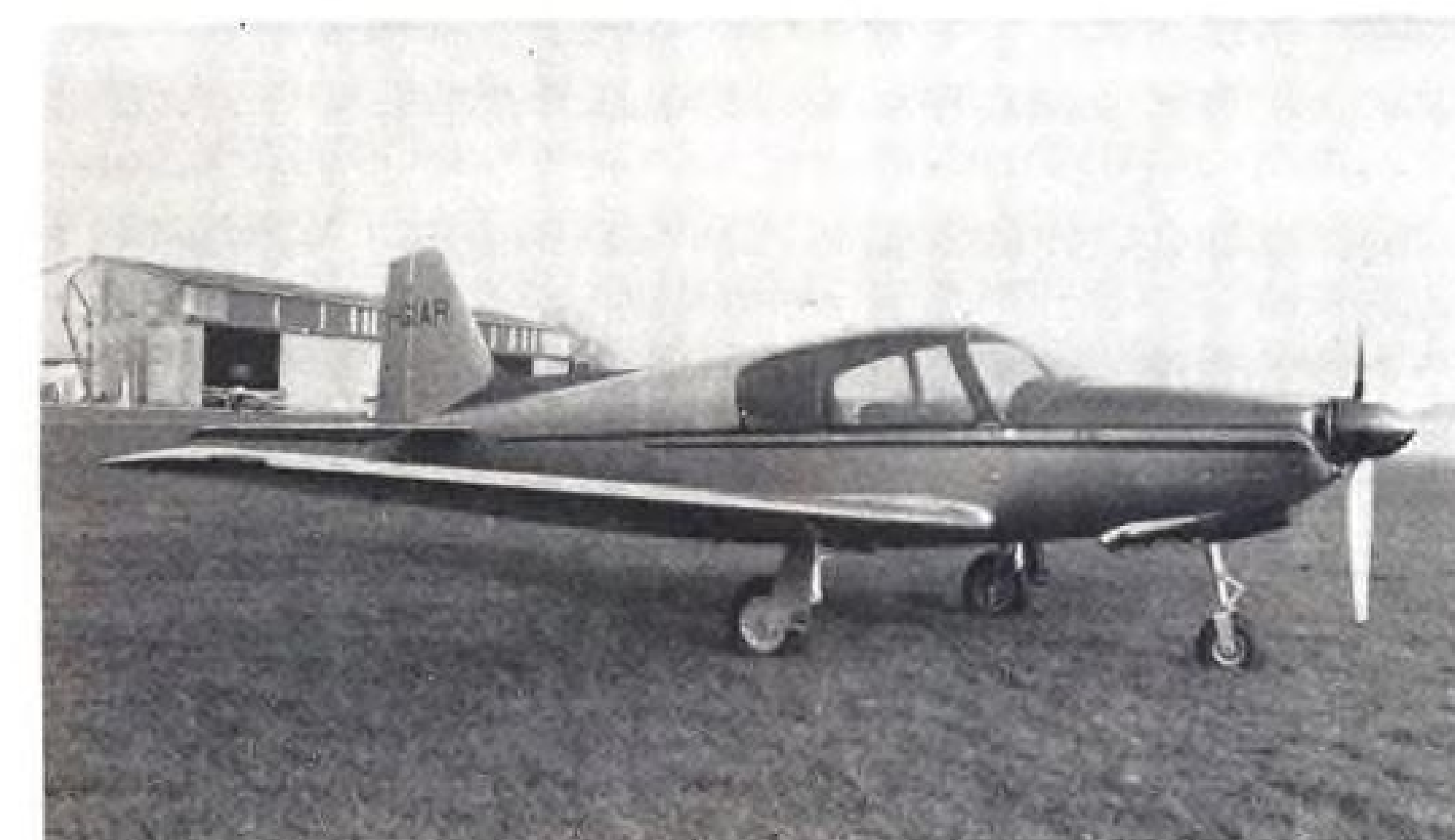
ITALIAN Aviamilano F.14 Nibbio four-placer has a 180-hp. Lycoming O360 and cruises at 180 mph. at 6,500 ft. Range is 621 mi. Gross weight is 2,420 lb. with 40 gal. fuel.
