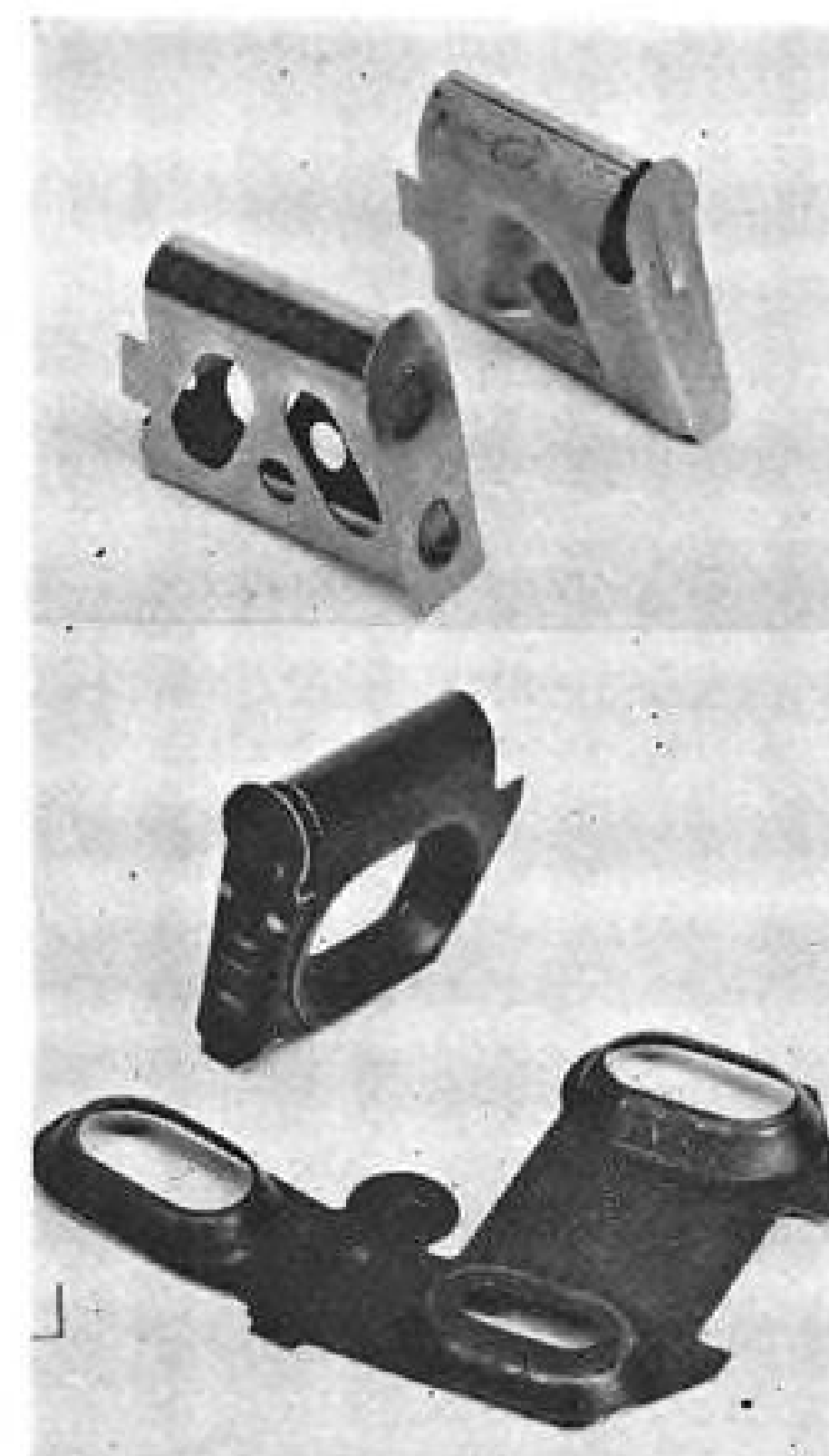
DAMPERS between bucket shanks of power turbine eliminate certain resonance that caused earlier fatigue failures (below). Dark material (photo above) shows final damper configuration.
