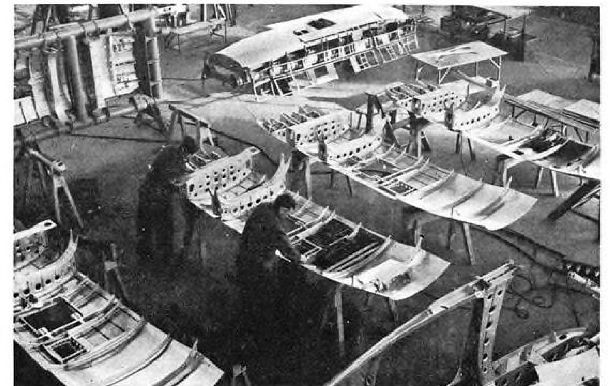
REAR fuselage structure approaches pure monocoque type (left). Finished fuselage bellies (right) await wiring, plumbing installation.
