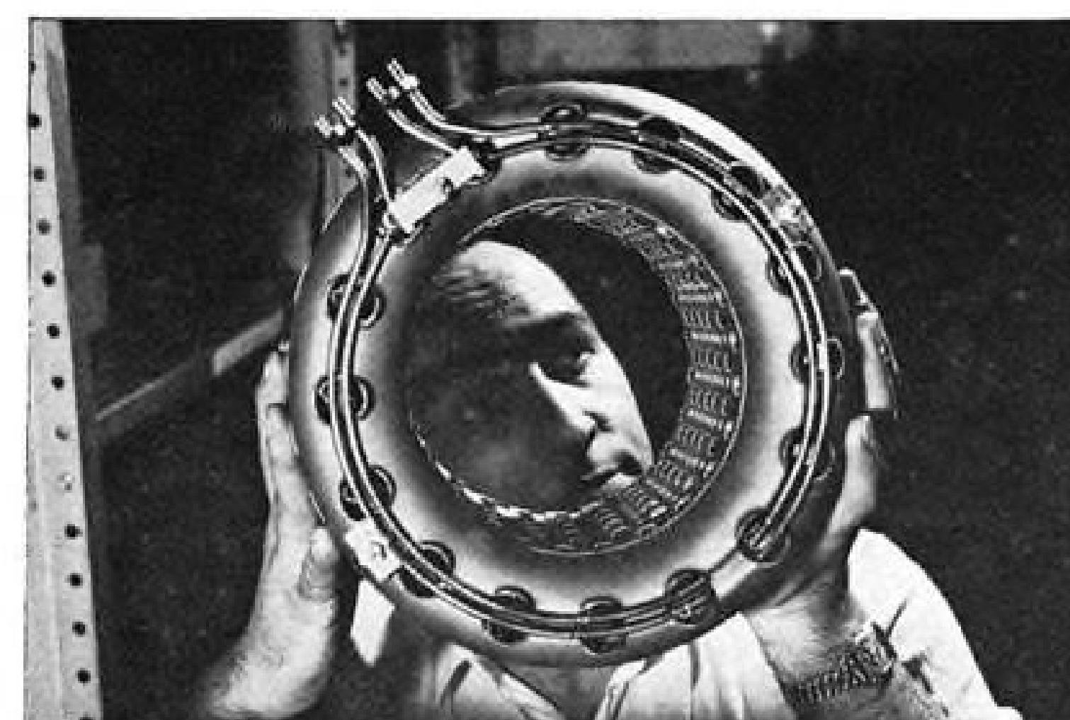
Durable combustion liners have survived 150-hour Model Test without trace of deterioration . . . combustor's altitude re-start ability proven.
