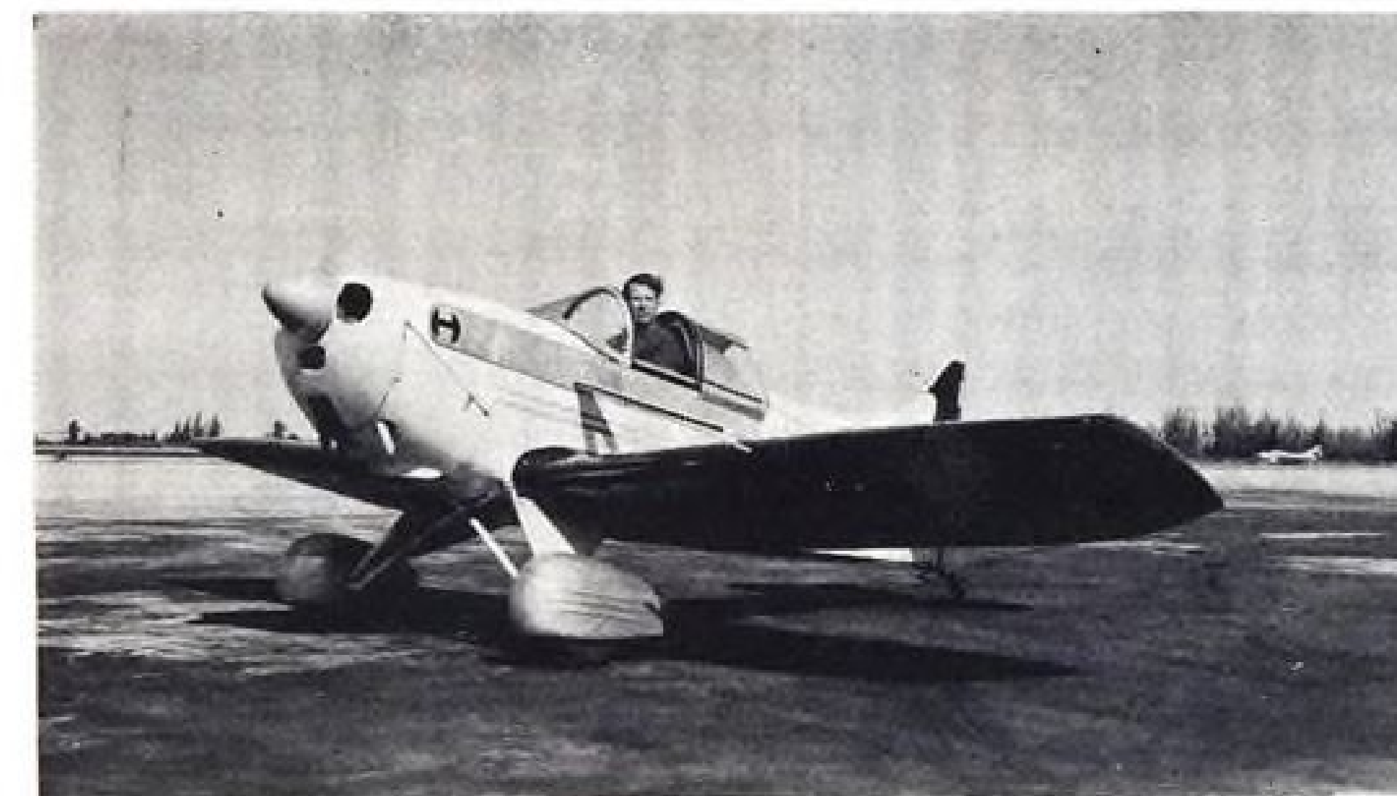
HOMEBUILT single-seater, assembled by Mark Horn, W. Palm Beach, Fla., in spare time for $1,500, has 100-hp. Continental. At 145 mph. it burns 6.2 gph. of 100 octane.
