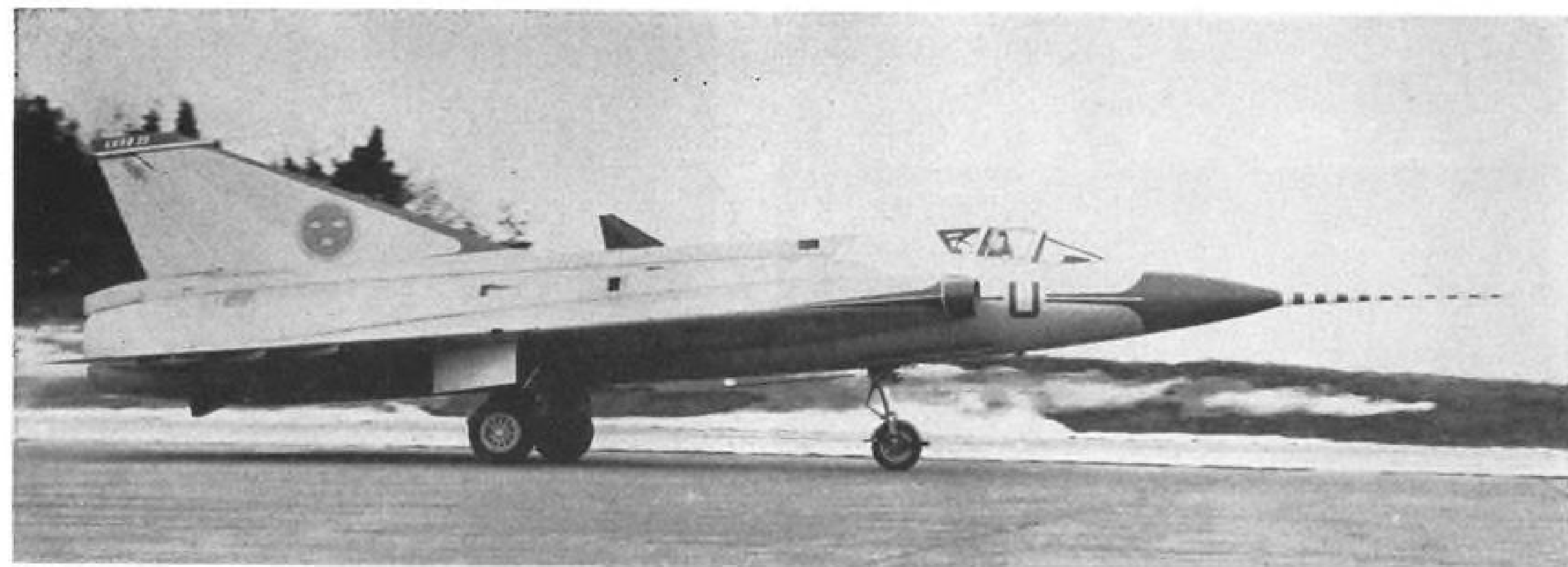
STRUCTURAL changes in first production model of J35 Draken includes major cockpit modification. Tail pipe has been enclosed and VHF antenna is installed on belly. "U" designation denotes aircraft is undergoing experimental flight test.
