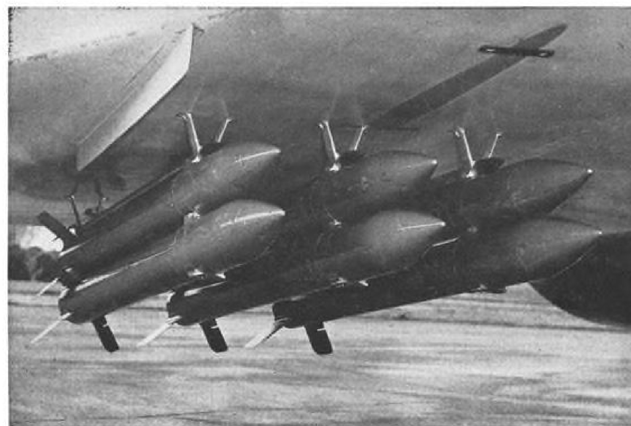
CLUSTER of 12 Bofors rockets, six under each wing, can be carried on Draken. This version is 13.5 cm. air-to-ground type. Inboard fence is at upper left.
