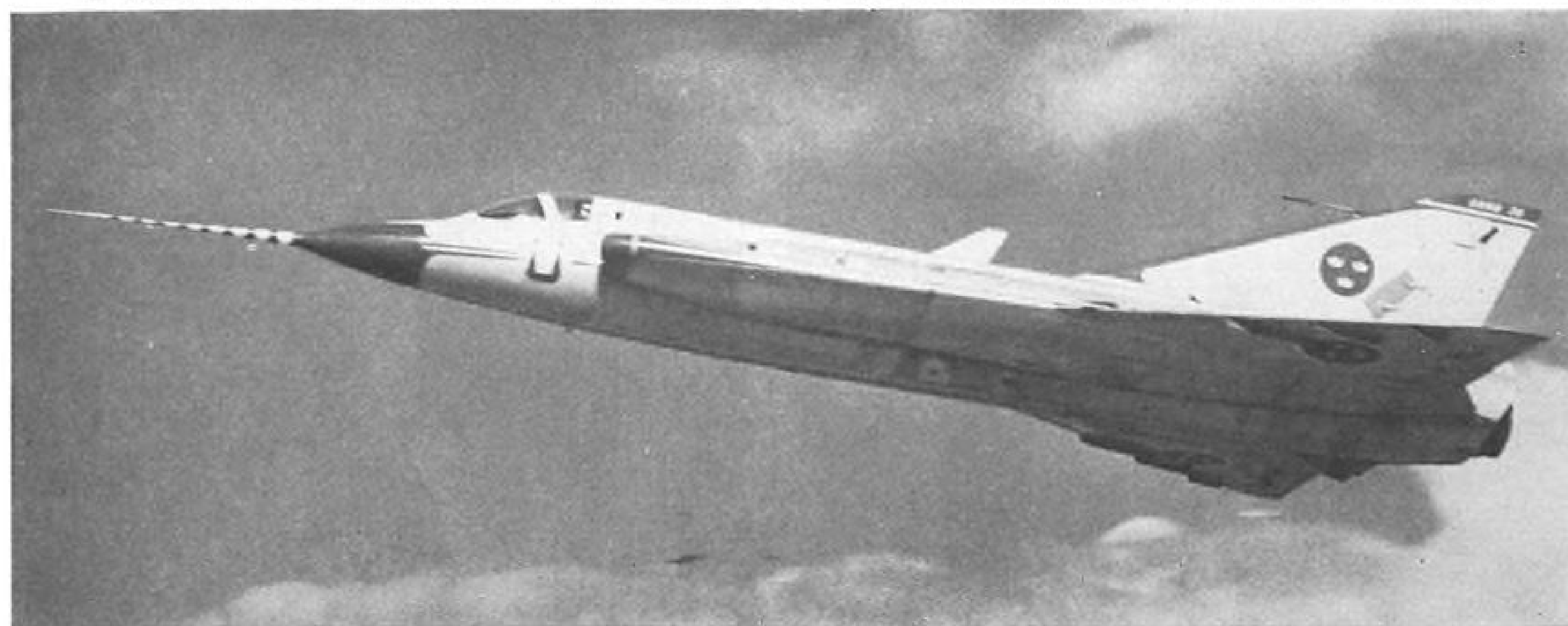
PROTOTYPE Saab J35 Draken has flown at Mach 1.4, can go supersonic in climb. Tail pipe is partly visible on this model.
