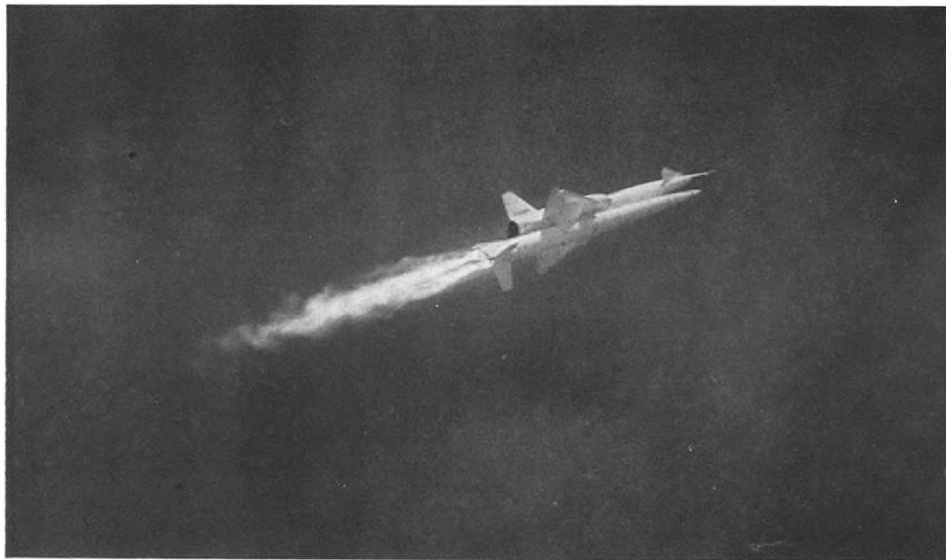
Navaho booster, pushing missile higher, develops 270,000 lb. thrust, is called most powerful of its kind. Project has been canceled.
