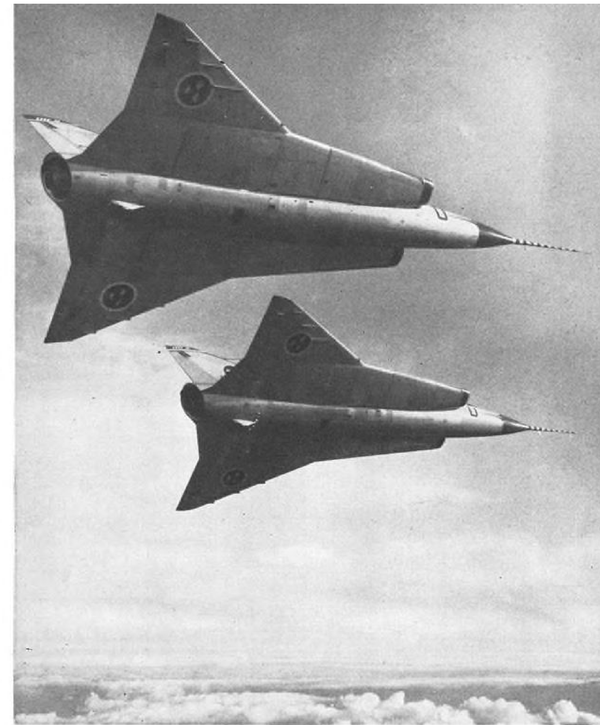
DOUBLE-DELTA configuration and tail cone forward sweep is shown in this prototype formation picture. Fences under delta wings reduce buffeting and give stability augmentation. Cambered surface tests may eliminate the fences.
