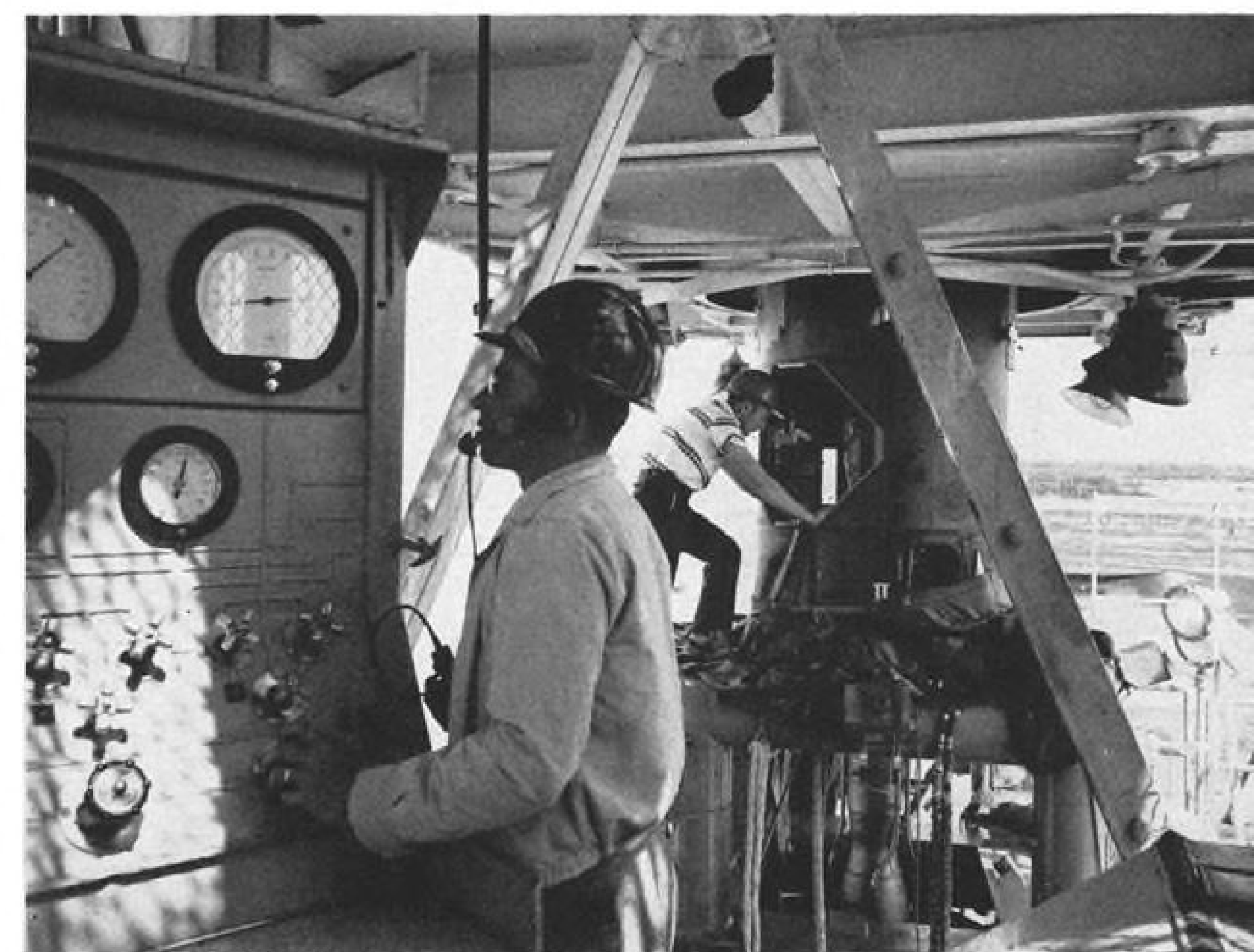
CONTROLS of the Navy Vanguard TV-4 satellite vehicle are checked by Martin Co. engineers at Cape Canaveral, Fla., launching site. Rocket was equipped with a backup ground system to take control of the guidance located in the second stage if it failed.
