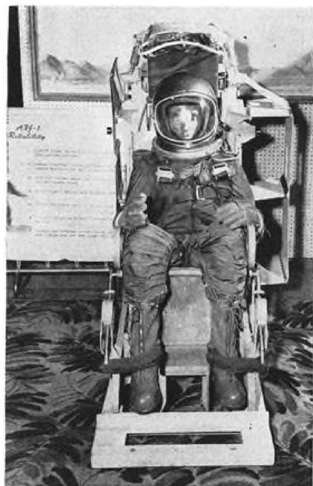
NORTH AMERICAN Columbus Division A3J ejection seat is similar to McDonnell F4H seat division is building. Stabilizing fin on pilot's right (left) is retracted. Rear view, right.
