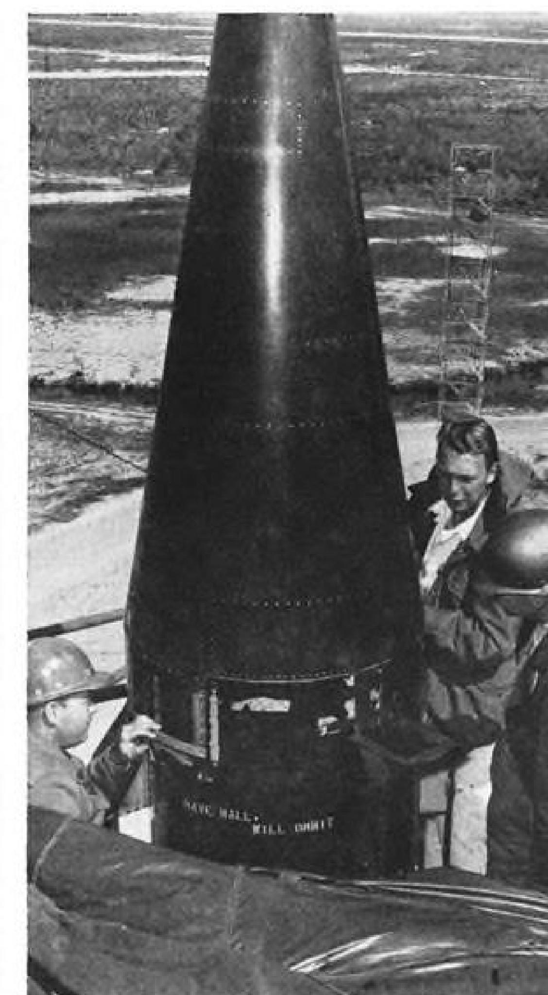
Vanguard nose cone is lowered into position (left), and inspected (center) by technicians. Nose cone is made of plastic phenolic; it streamlines vehicle and insulates sphere from heat. At right the gantry crane moves back and the satellite vehicle is cleared for firing.
