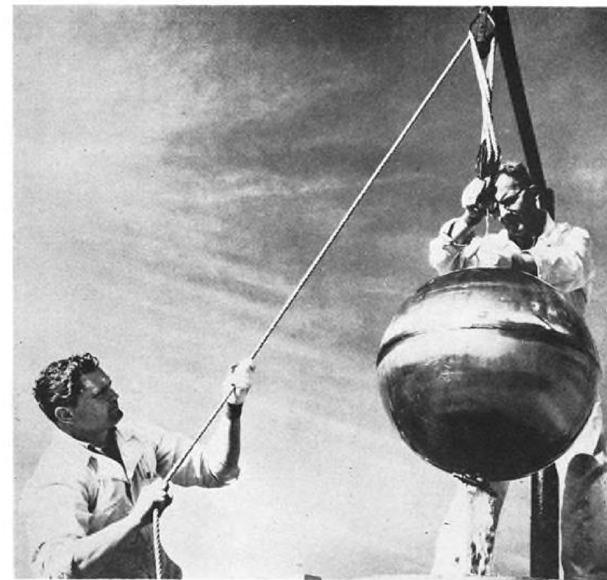
TITANIUM tank, designed for Atlas missile, is rinsed prior to heat treatment. Tank will hold helium which is used to pressurize the missile's propellant fuel.
