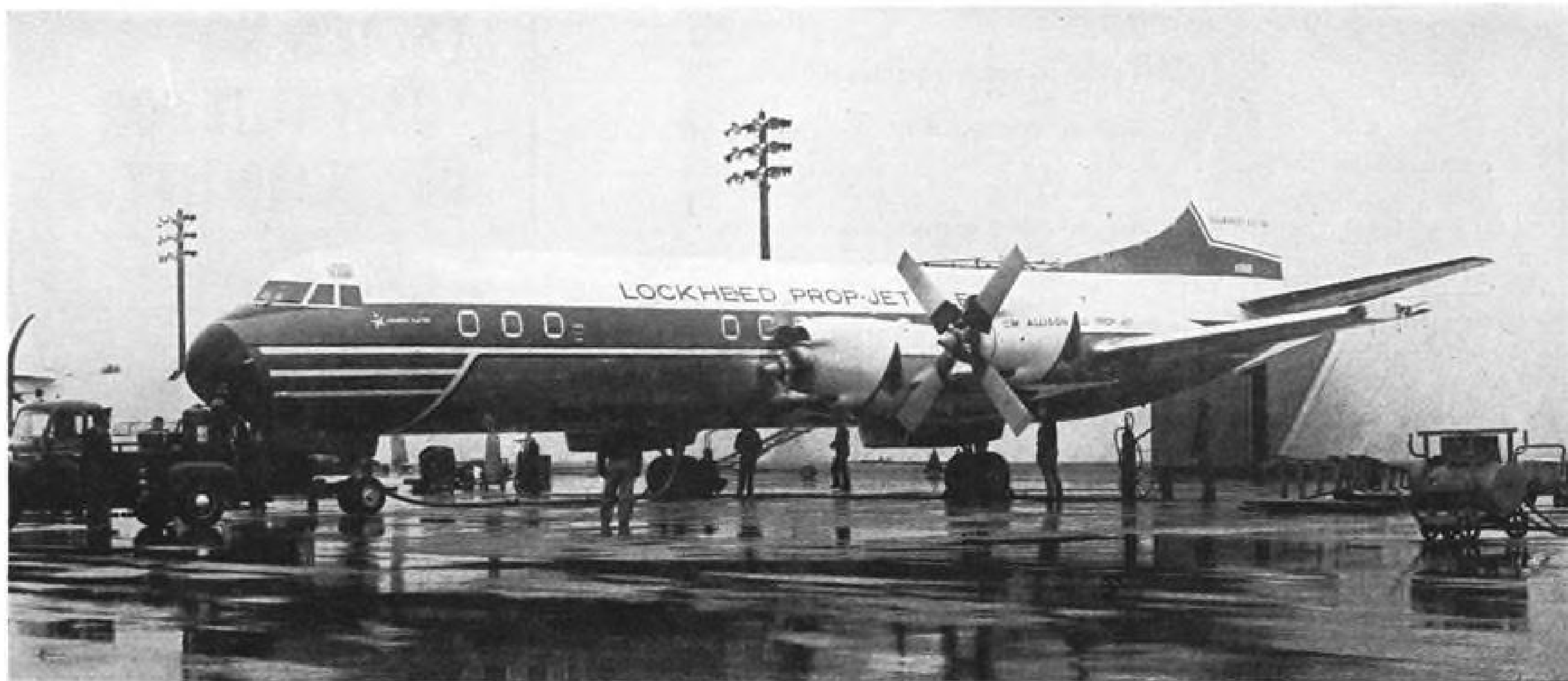
ENGINE runup starts on second Lockheed project Electra at Burbank, Calif., flight line. Each engine develops 3,750 eshp.
