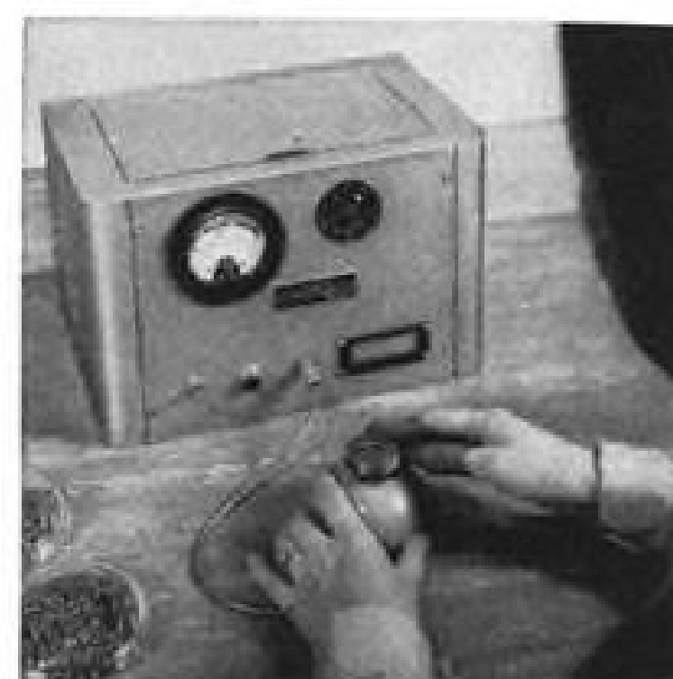
The SmoothRator, an electronic performance tester, was developed by Barden to check vibration as a measure of overall functional quality. A standard quality control instrument at Barden, the SmoothRator is also used by many leading component and systems manufacturers.
